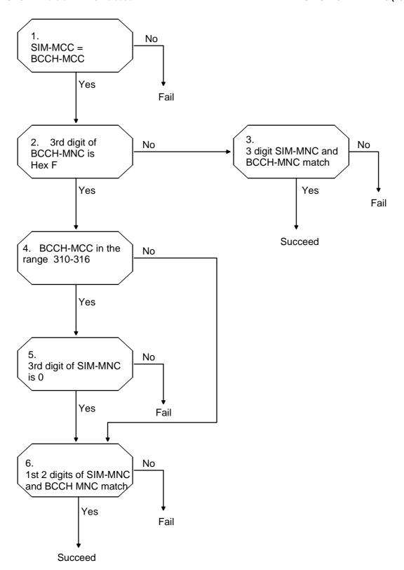
Figure A.2: HPLMN Matching Criteria Logic Flow for mobiles which support PCS1900 for NA (informative)
