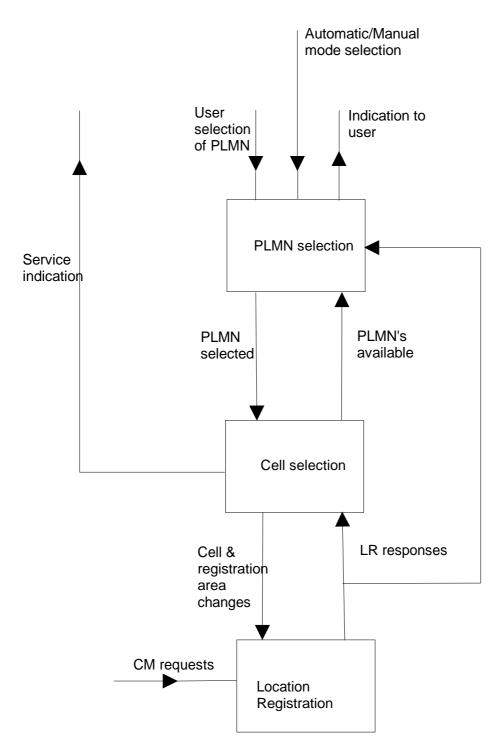
Figure 1: Overall Idle Mode process
