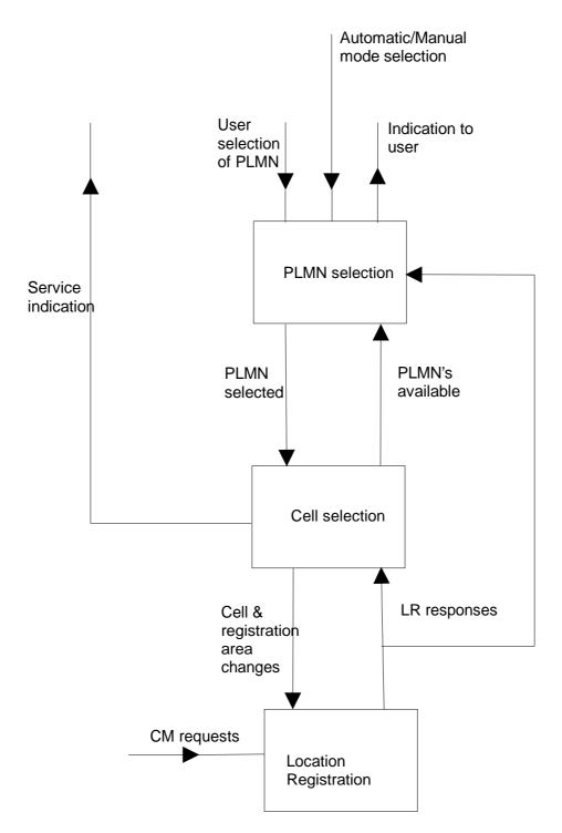
Figure 1: Overall Idle Mode process
