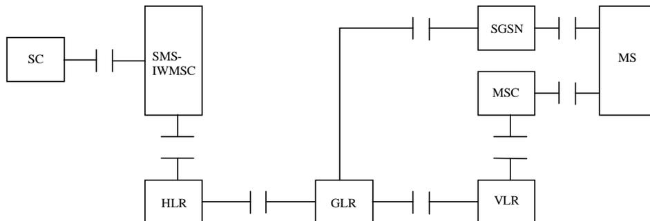
**Figure 7.7/9: Interfaces involved in the Alert procedure with GLR**
