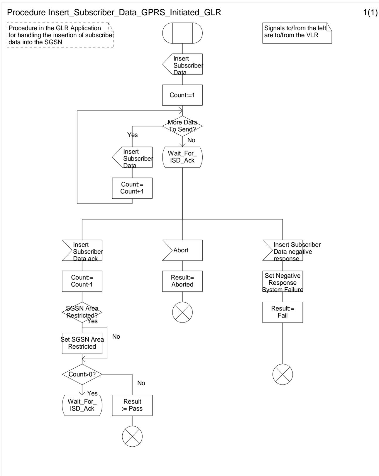
Figure7.3/7: Procedure Insert\_Subscriber\_Data\_GPRS\_Initiated\_GLR
