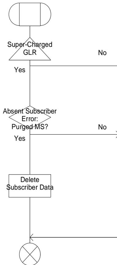
Figure 7.2/14: Procedure Super\_Charged\_PRN\_Error\_GLR
