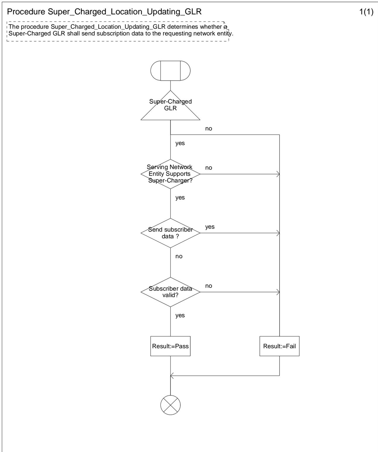
Figure 7.13/5: Procedure Super\_Charged\_Location\_Updating\_GLR
