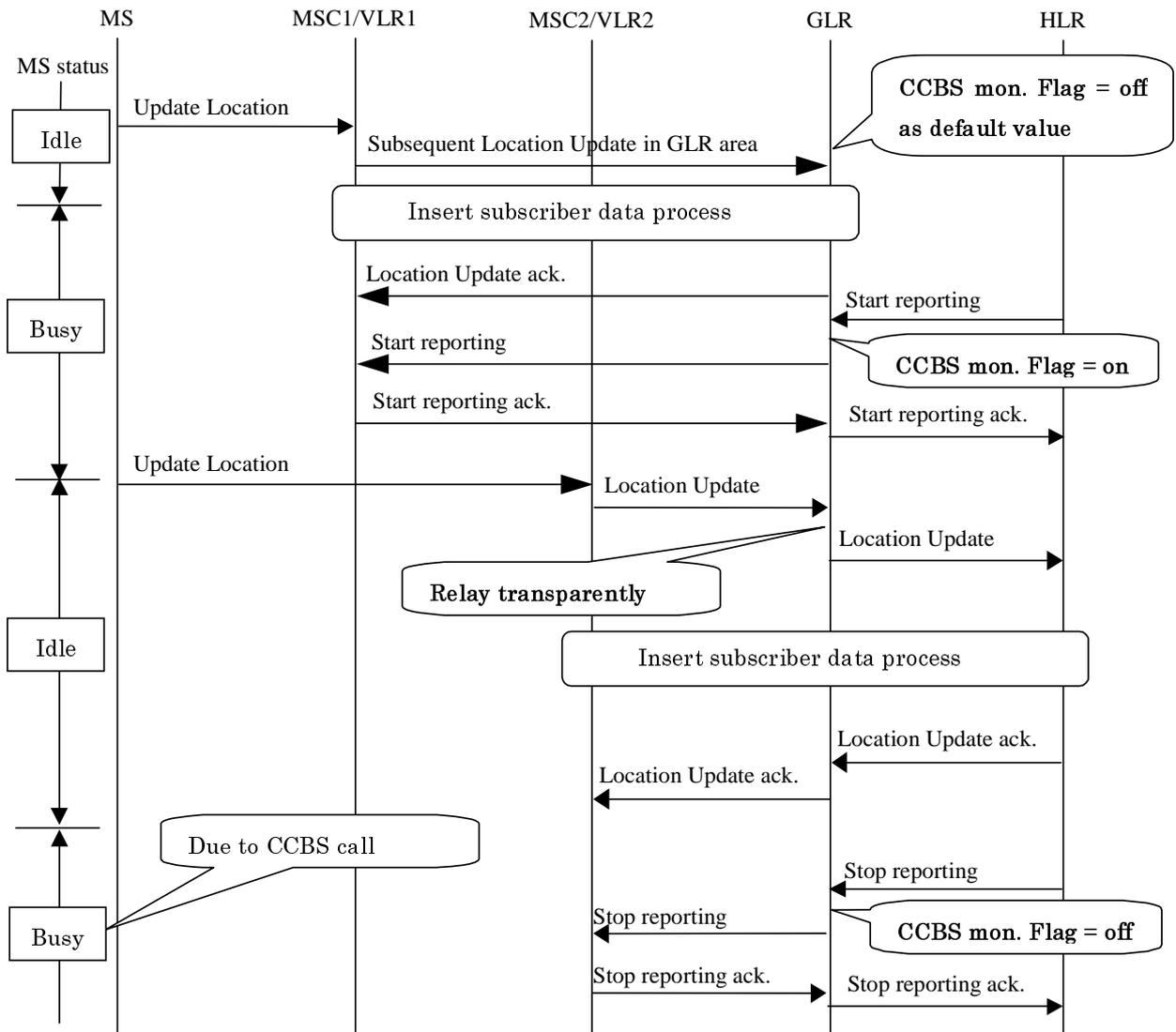
Figure 7.10/1: Update Location request signal handling for CCBS in the GLR (Alternative 1)
