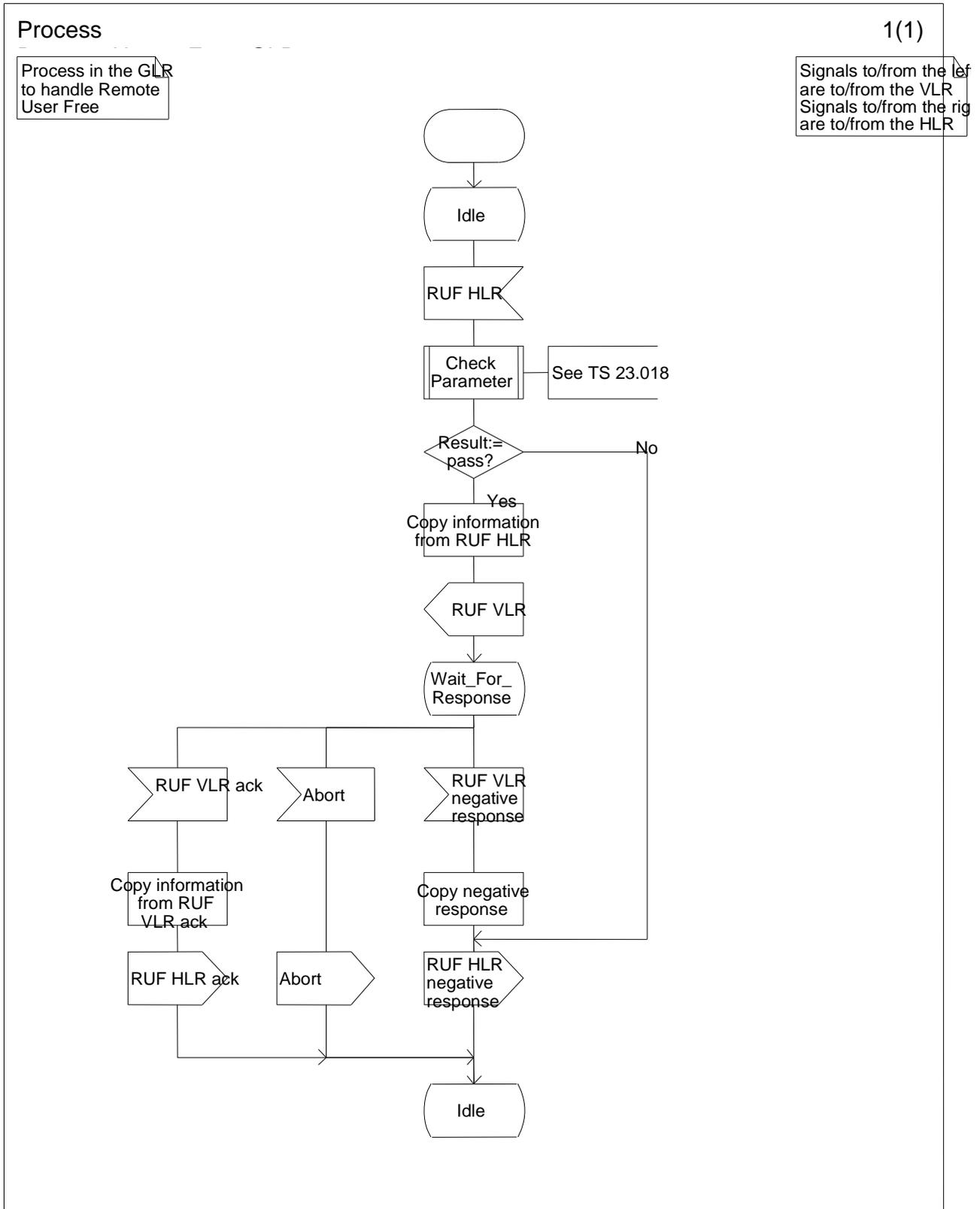
Figure 7.10/5: Process Remote\_User\_Free\_GLR
