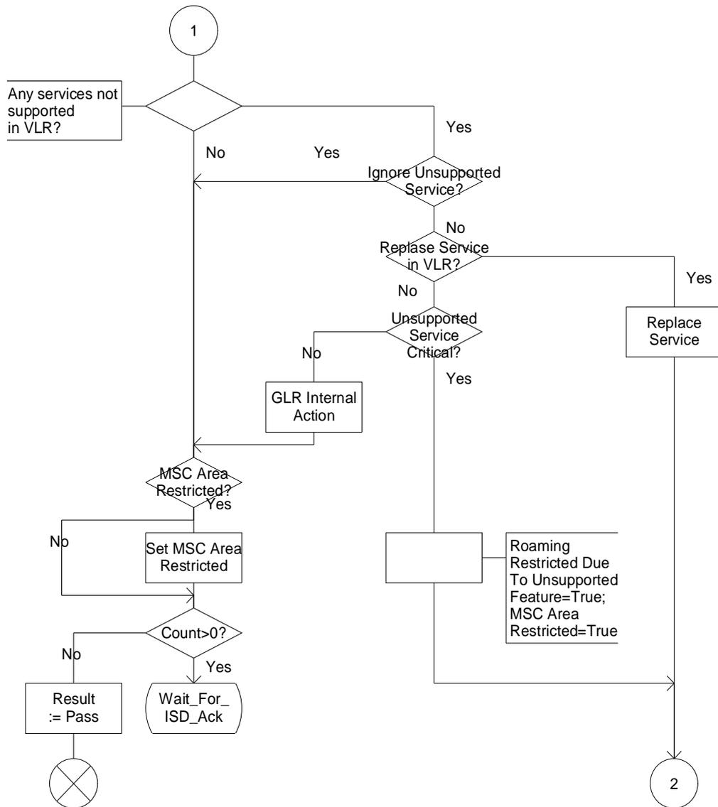
Figure7.2/6(2): Procedure Insert\_Subscriber\_Data\_Initiated\_GLR
