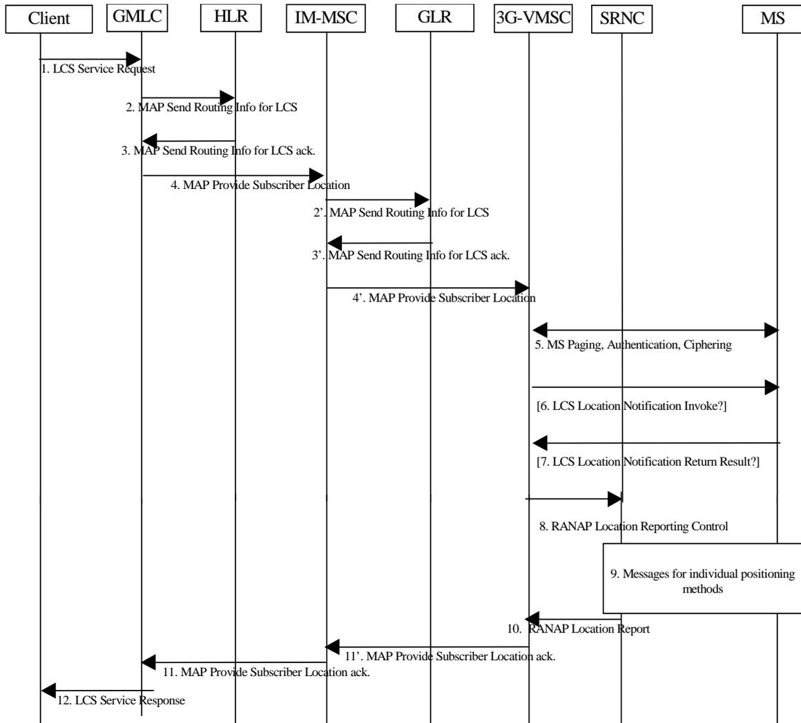
Figure 7.11/1: General Network Positioning for a MT-LR
