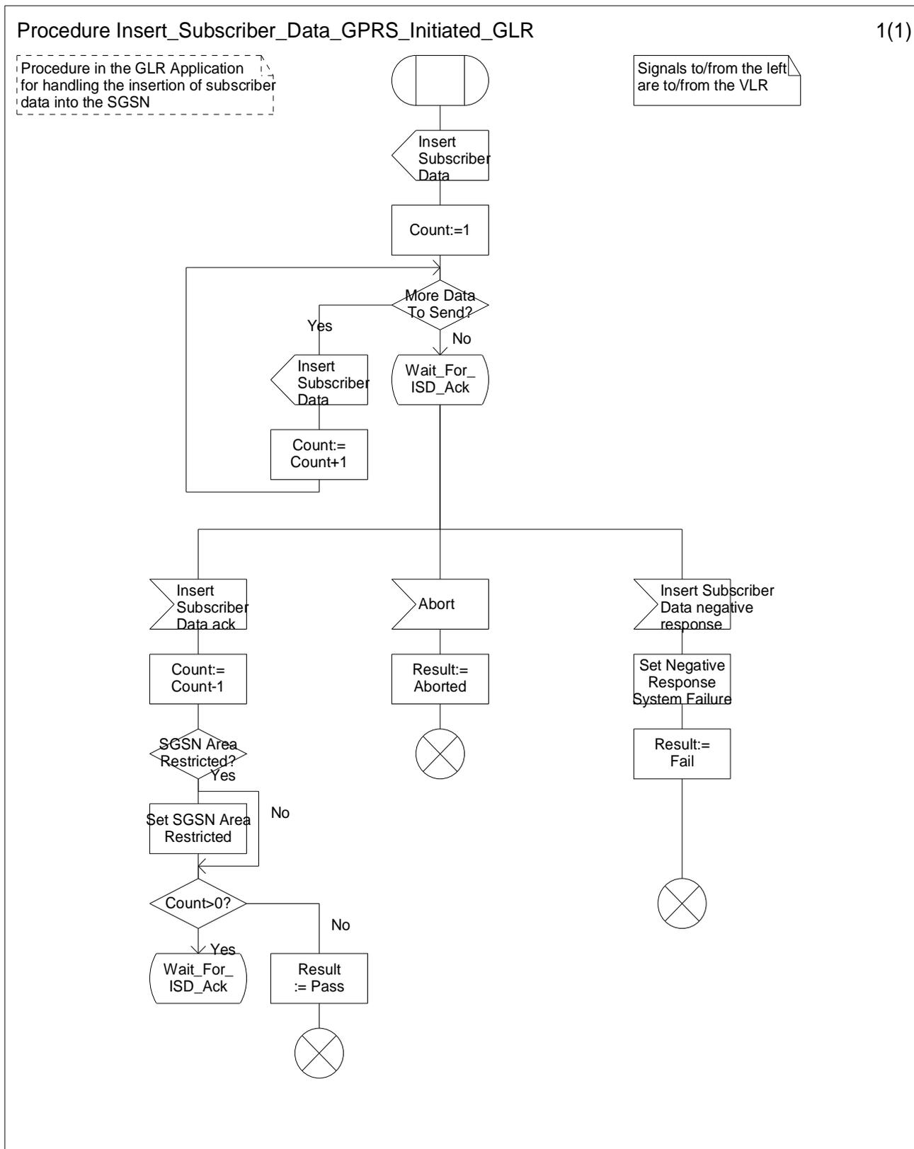
Figure7.3/7: Procedure Insert\_Subscriber\_Data\_GPRS\_Initiated\_GLR
