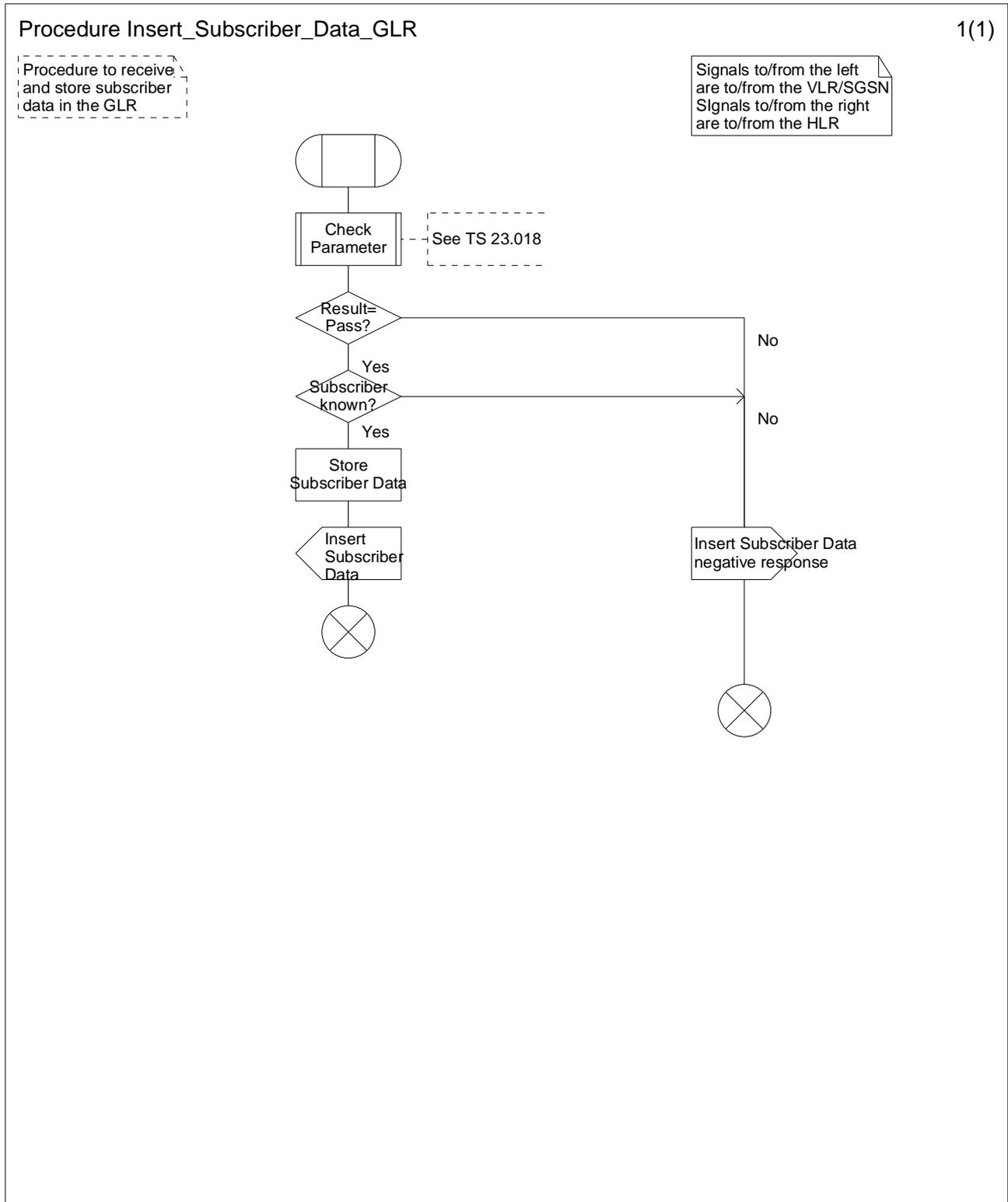
Figure7.2/5: Procedure Insert\_Subscriber\_Data\_GLR
