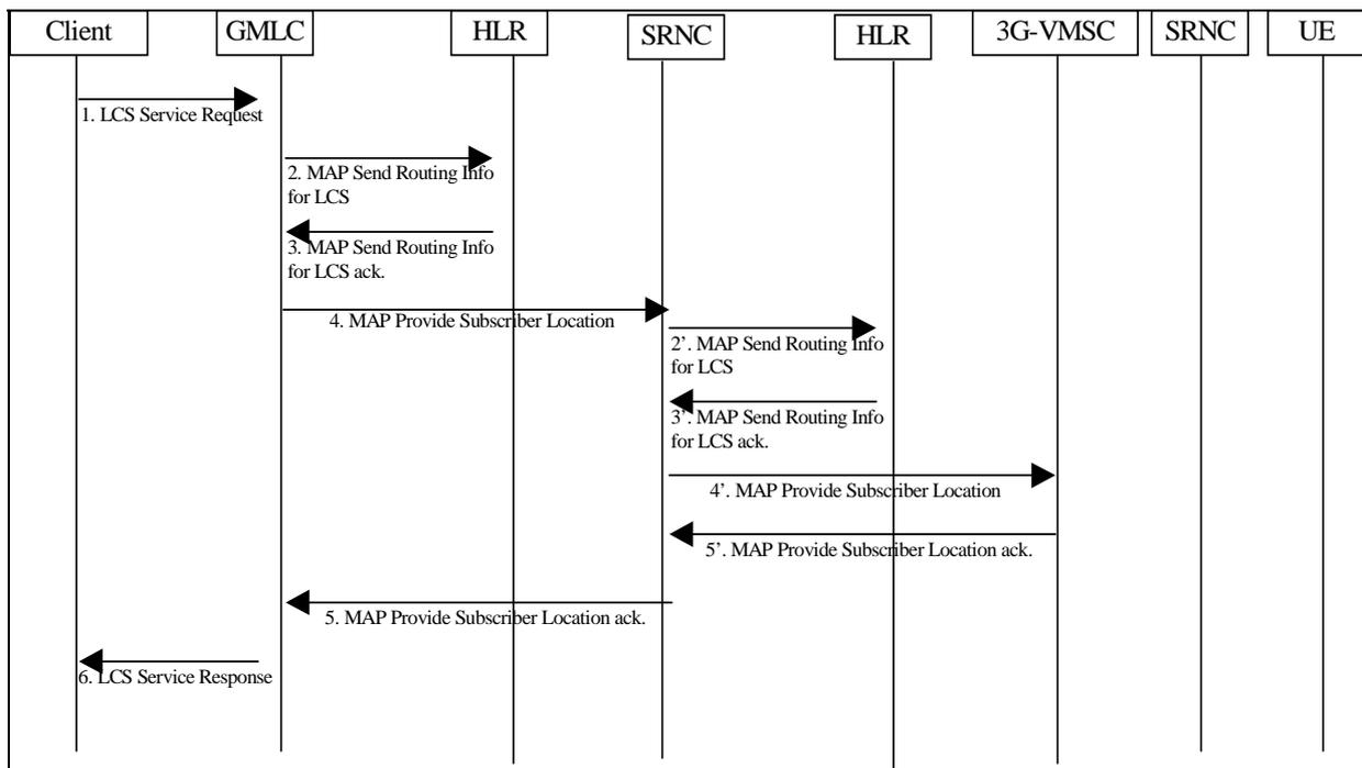
**Figure 7.11/2: MT-LR for a previously obtained location estimate**
