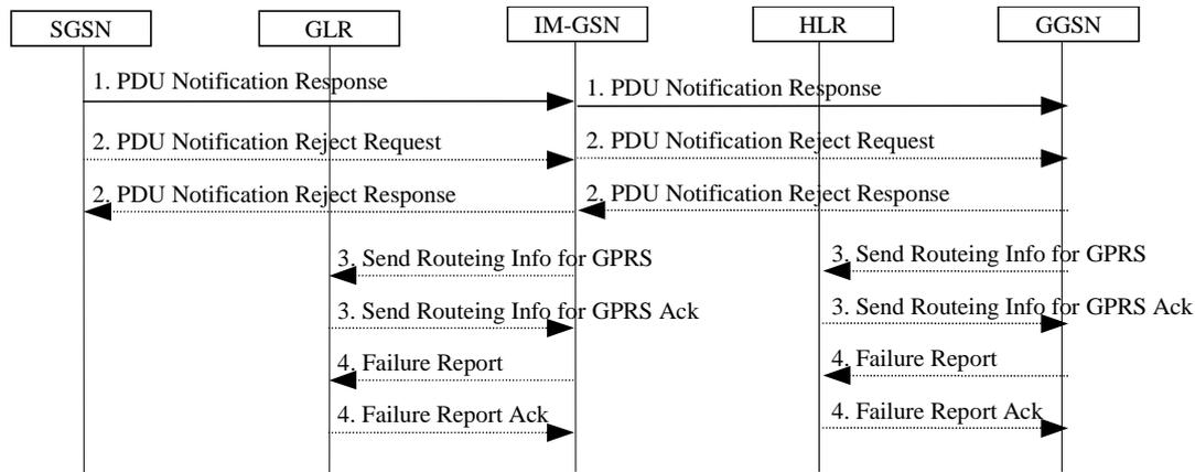
**Figure 7.3/16: Protection Procedure**
