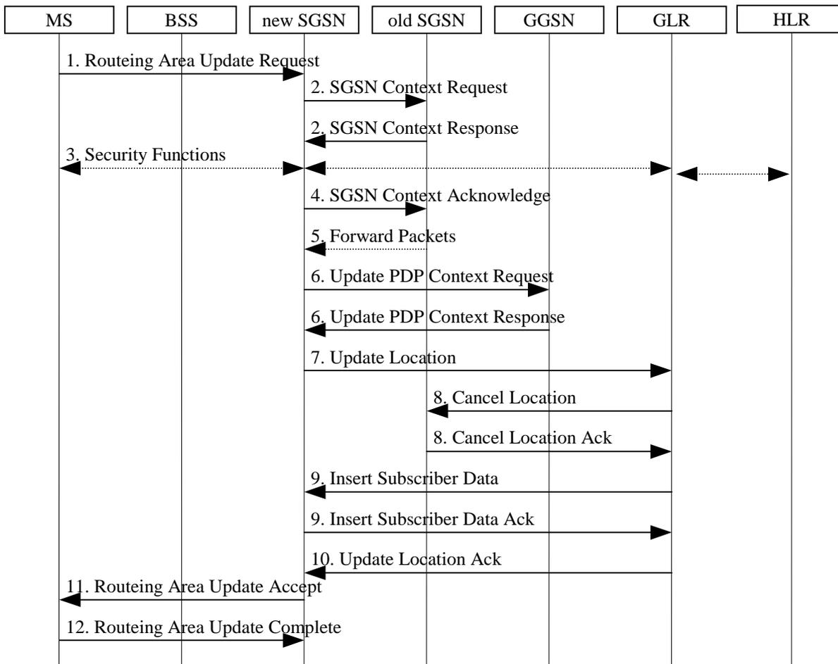
**Figure 7.3/12: Inter SGSN Routing Area Update Procedure**
