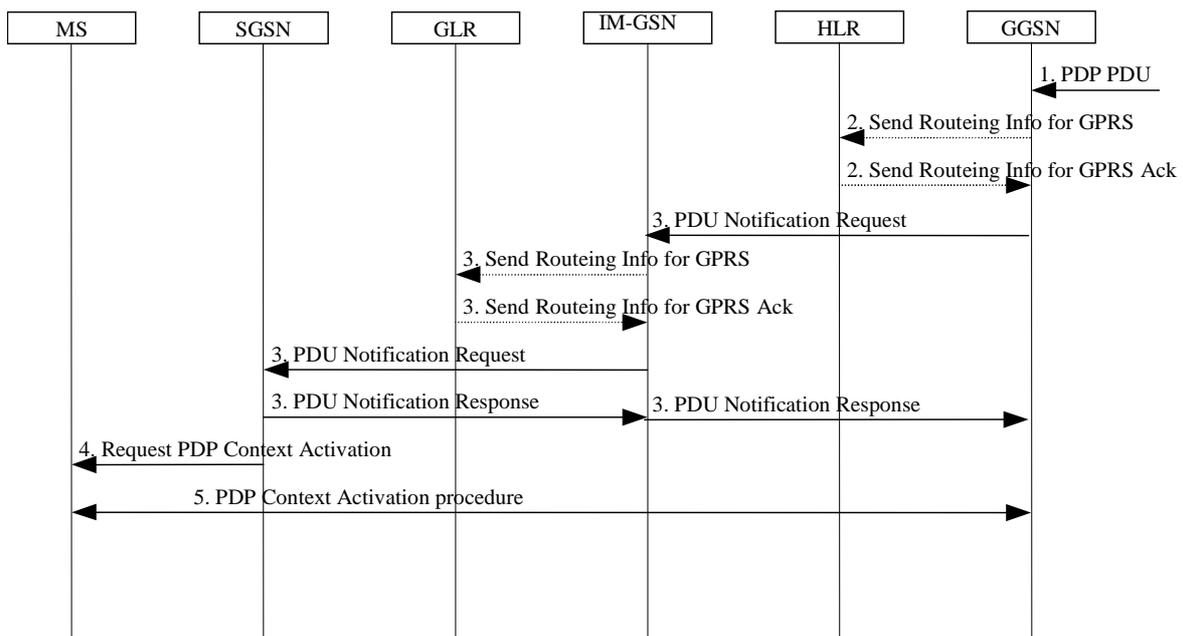
**Figure 7.3/15: Successful Network-Requested PDP Context Activation Procedure**
