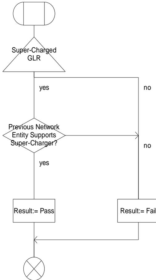
Figure 7.13/4: Procedure Super\_Charged\_Cancel\_Location\_GLR
