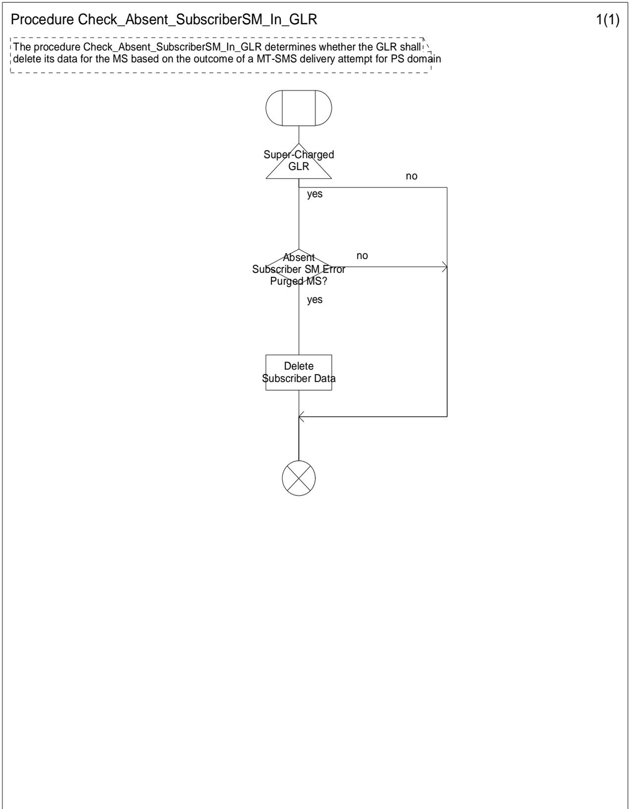
Figure 7.7/8: Procedure Check\_Absent\_SubscriberSM\_In\_GLR
