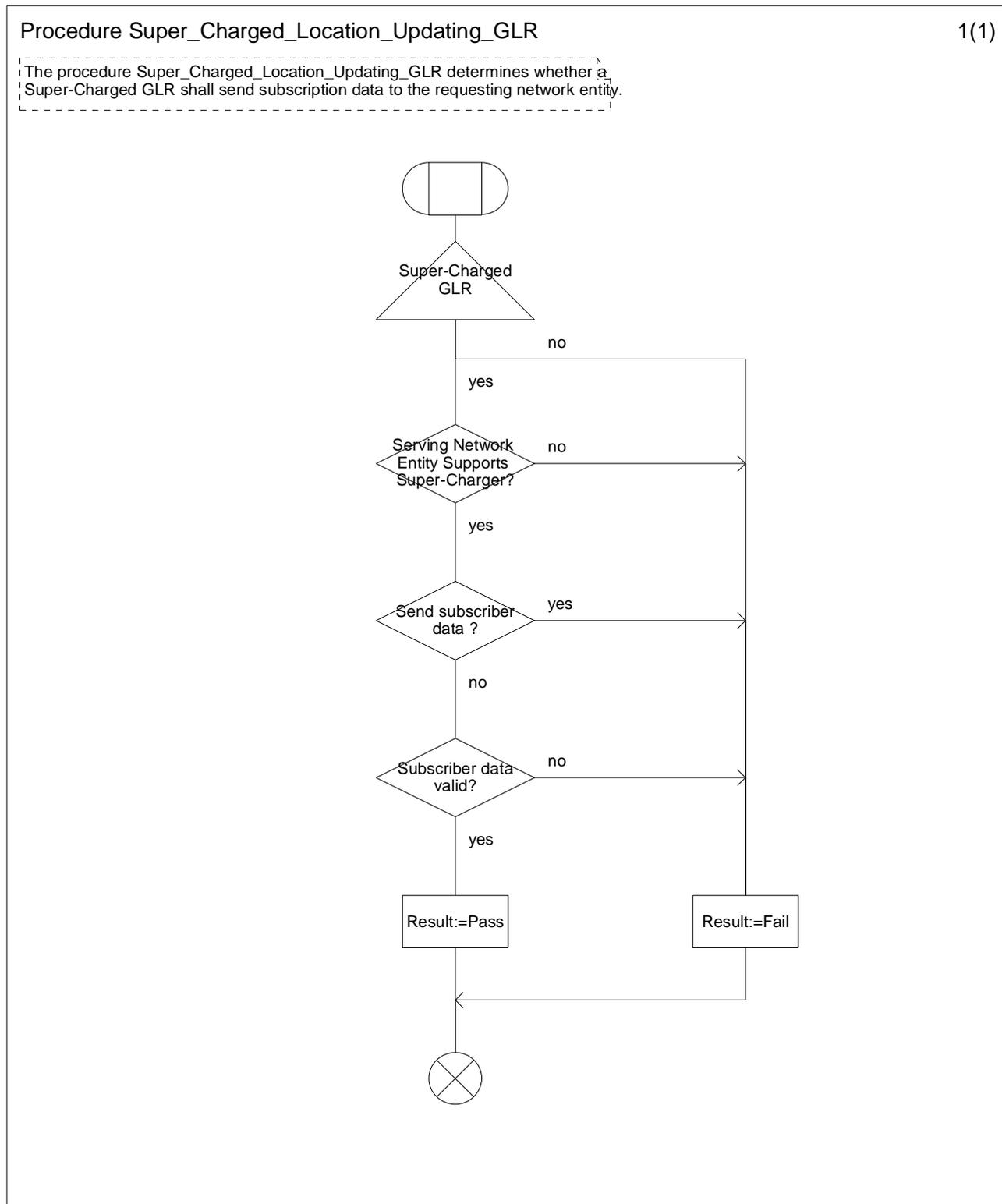
Figure 7.13/5: Procedure Super\_Charged\_Location\_Updating\_GLR
