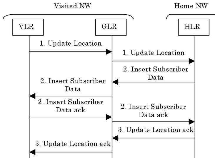
**Figure 7.2/1: First Location Updating Procedure in the Network**
