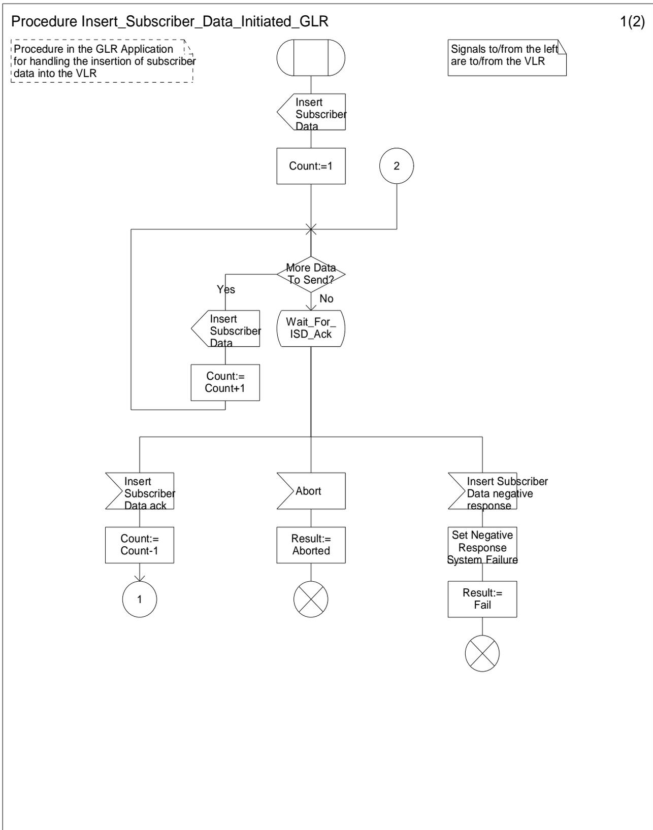
Figure7.2/6(1): Procedure Insert\_Subscriber\_Data\_Initiated\_GLR
