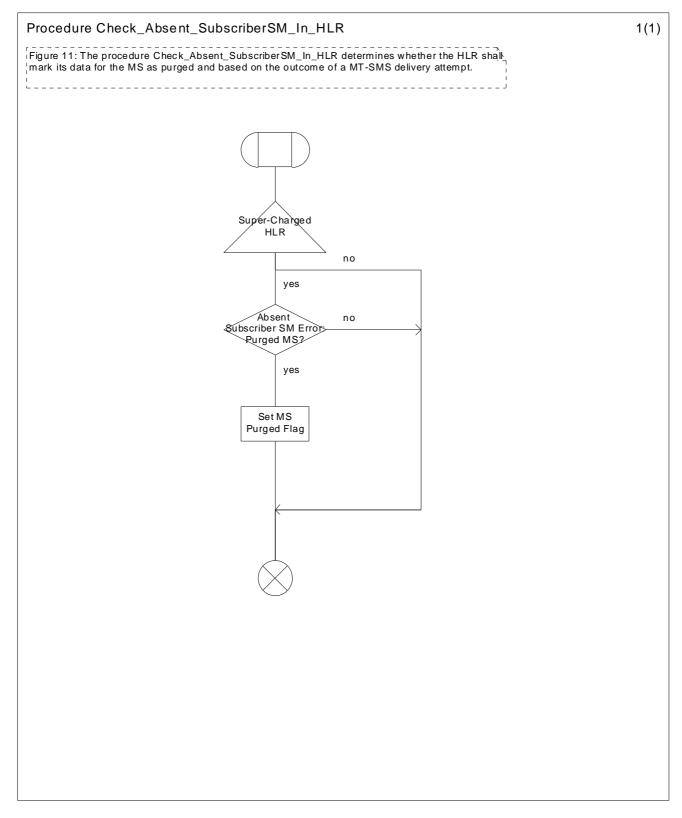
Figure 11: Procedure Check\_Absent\_SubscriberSM\_In\_HLR
