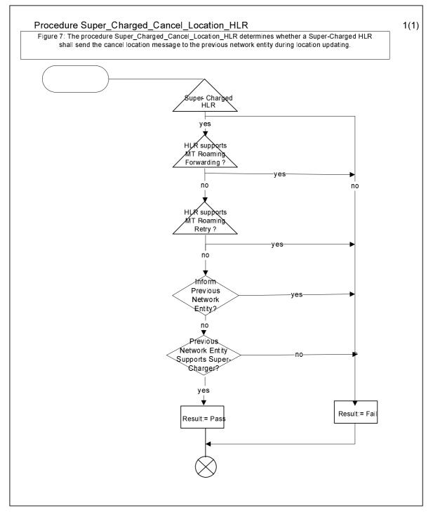
Figure 7: Procedure Super\_Charged\_Cancel\_Location\_HLR
