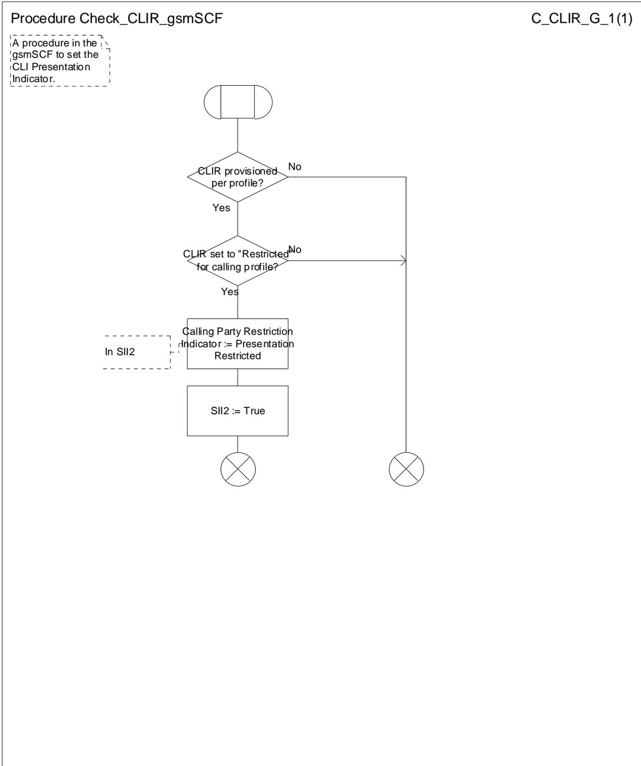
Figure 9: Procedure Check\_CLIR\_gsmSCF
