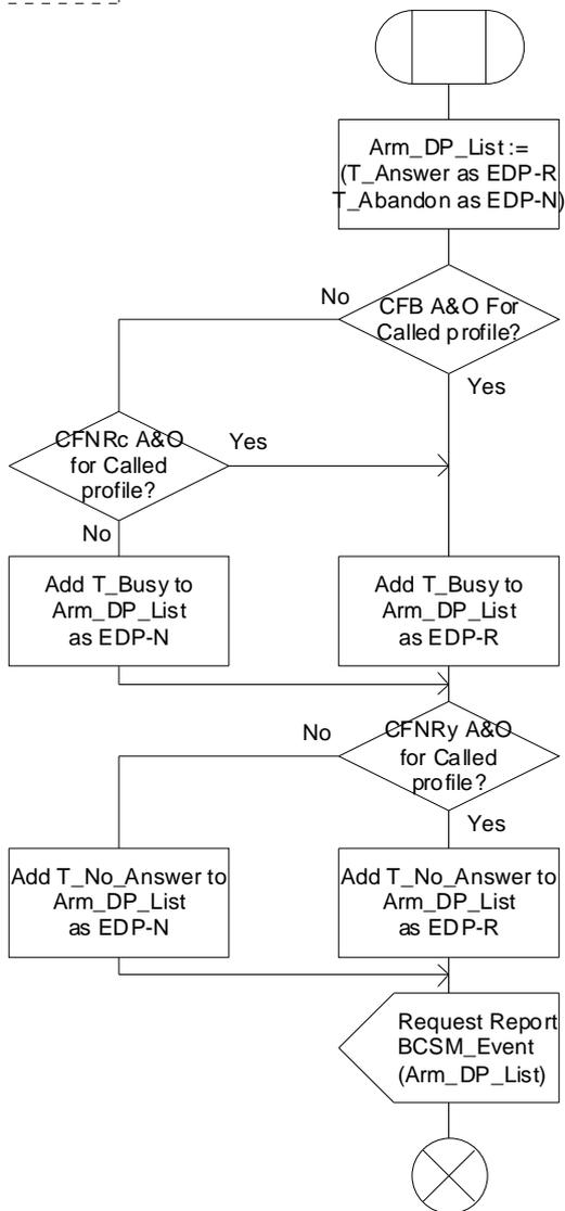
Figure 13: Procedure Check\_Late\_CF\_gsmSCF
