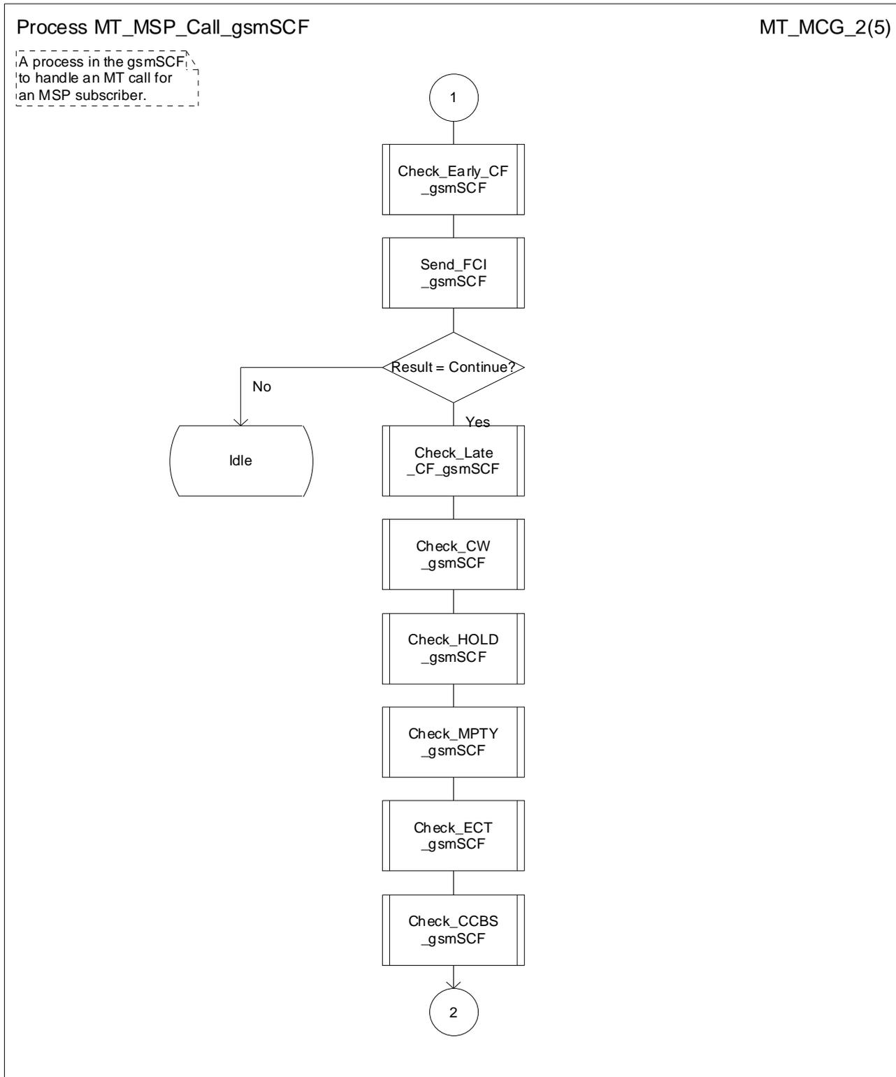
Figure 8b: Process MT\_MSP\_Call\_gsmSCF (sheet 2 of 5)
