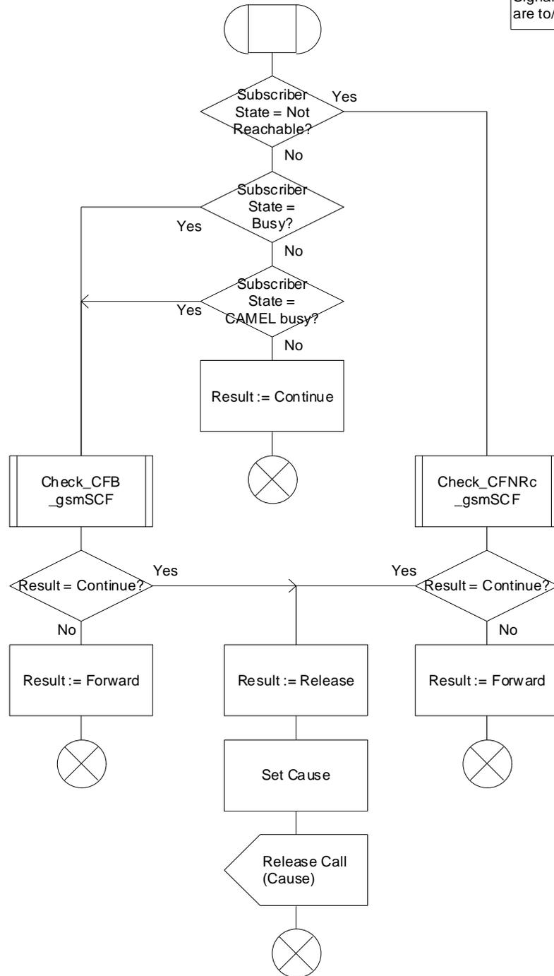
Figure 12: Procedure Check\_Early\_CF\_gsmSCF
