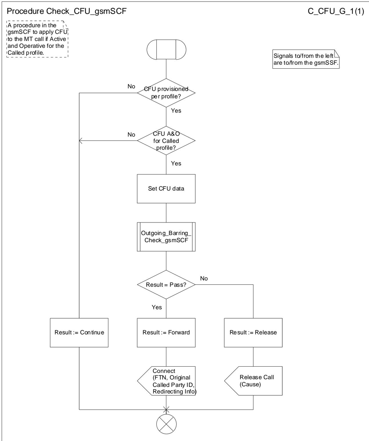
Figure 11: Procedure Check\_CFU\_gsmSCF
