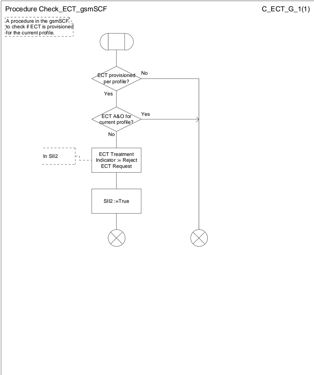
Figure 26: Procedure Check\_ECT\_gsmSCF
