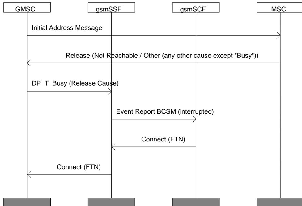
**Figure 36: Information flow for an MT call to a profile with CFNRc active and operative in the gsmSCF, where late CFNRc is invoked**
