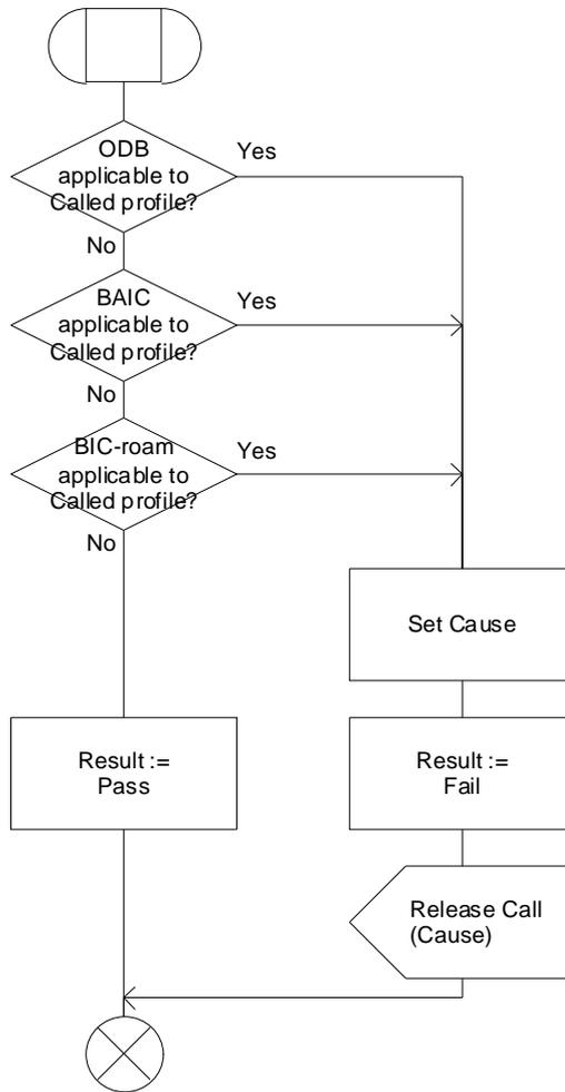
Figure 25: Procedure Incoming\_Barring\_Check\_gsmSCF
