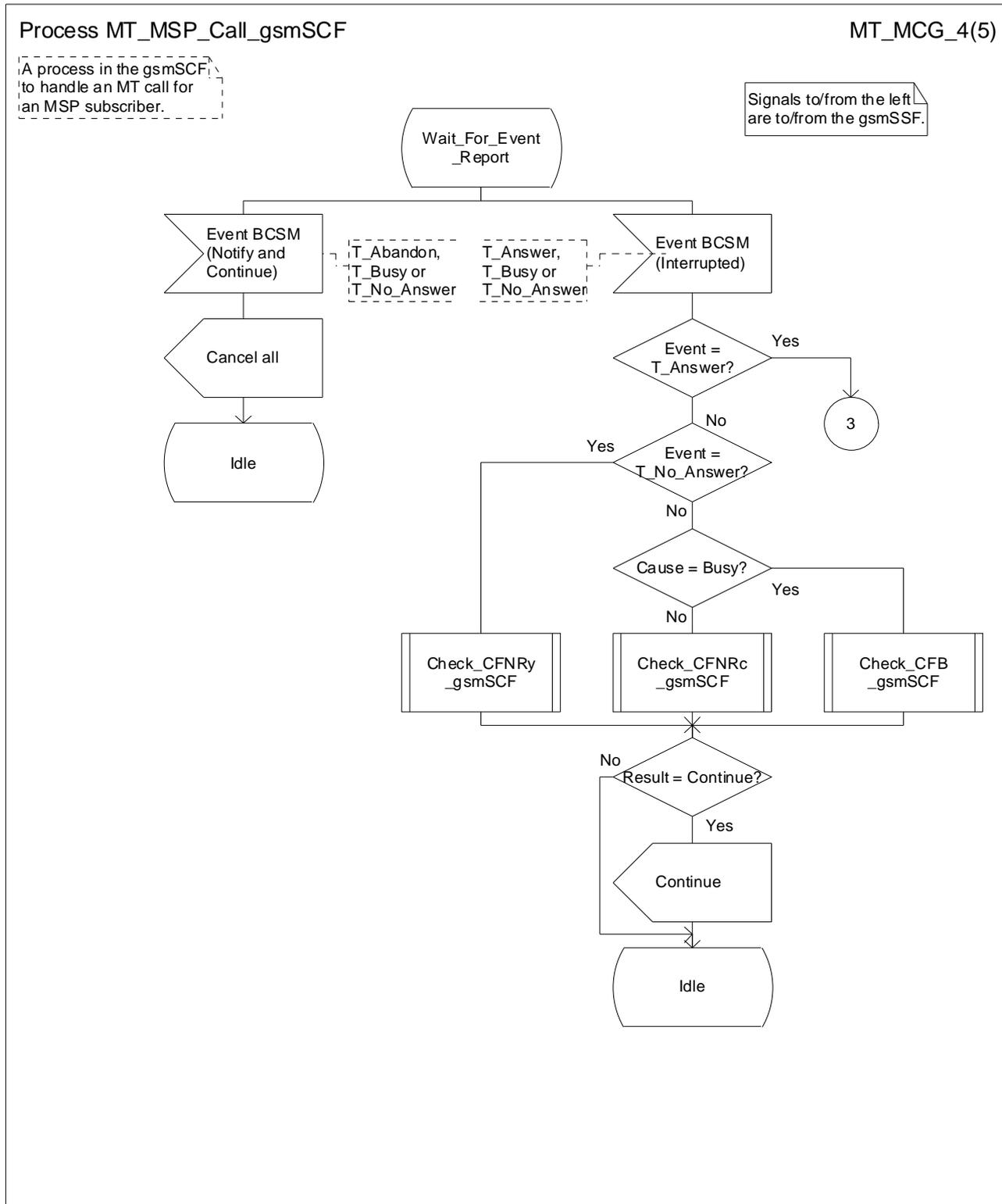
Figure 8d: Process MT\_MSP\_Call\_gsmSCF (sheet 4 of 5)
