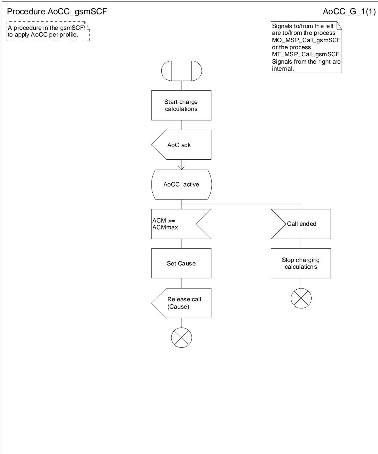
Figure 23: Procedure AoCC\_gsmSCF
