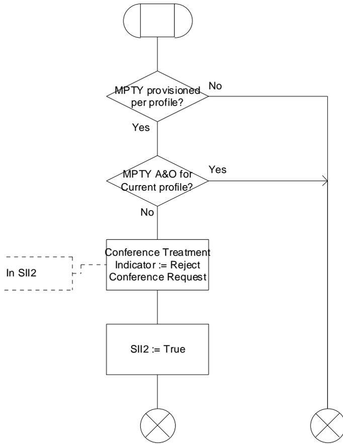
Figure 19: Procedure Check\_MPTY\_gsmSCF
