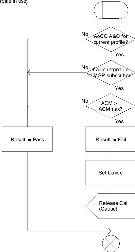
Figure 20: Procedure Check\_ACM\_gsmSCF
