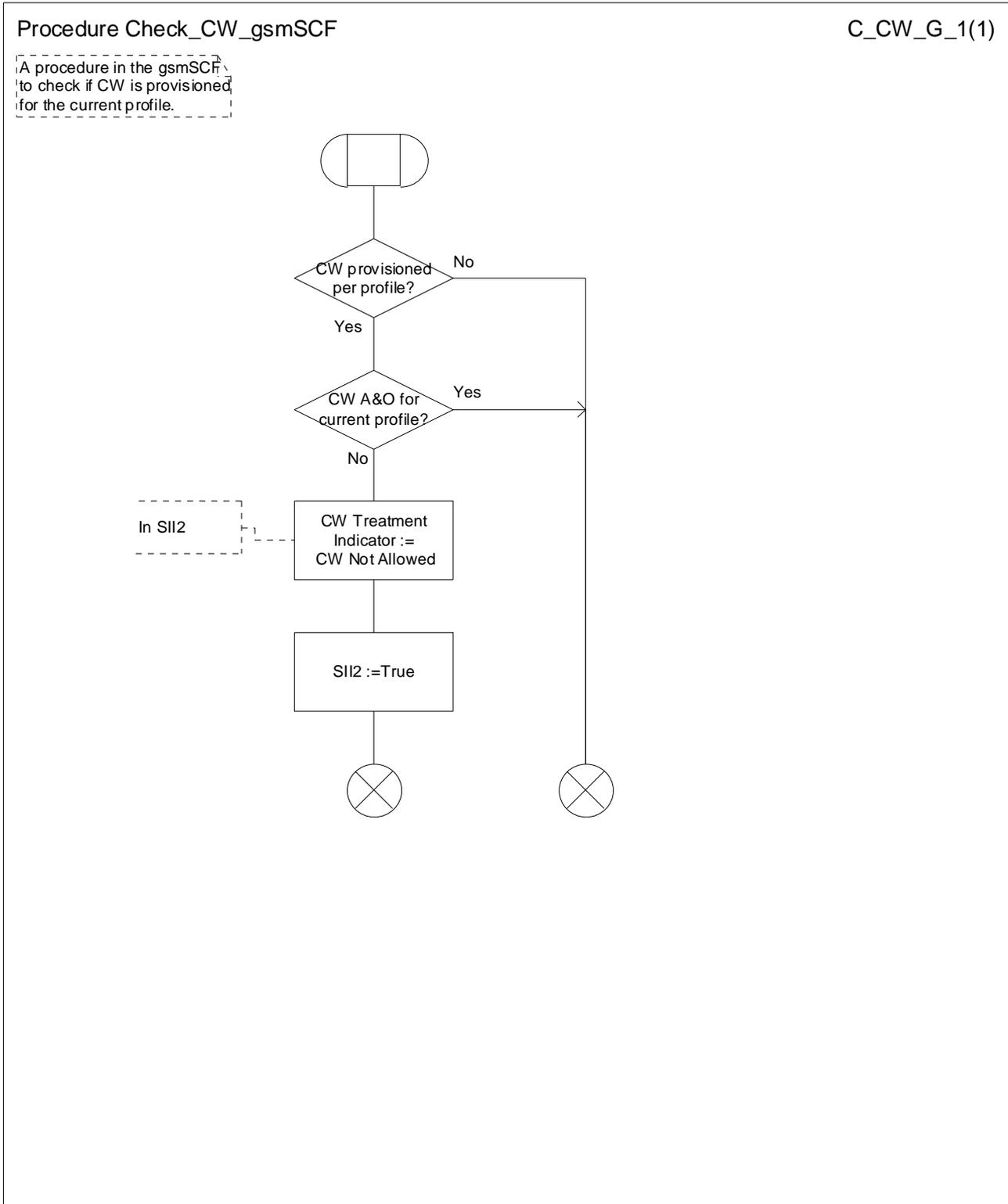
Figure 17: Procedure Check\_CW\_gsmSCF
