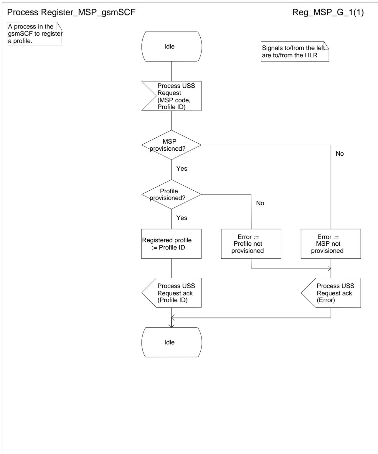
Figure 2: Process Register\_MSP\_gsmSCF
