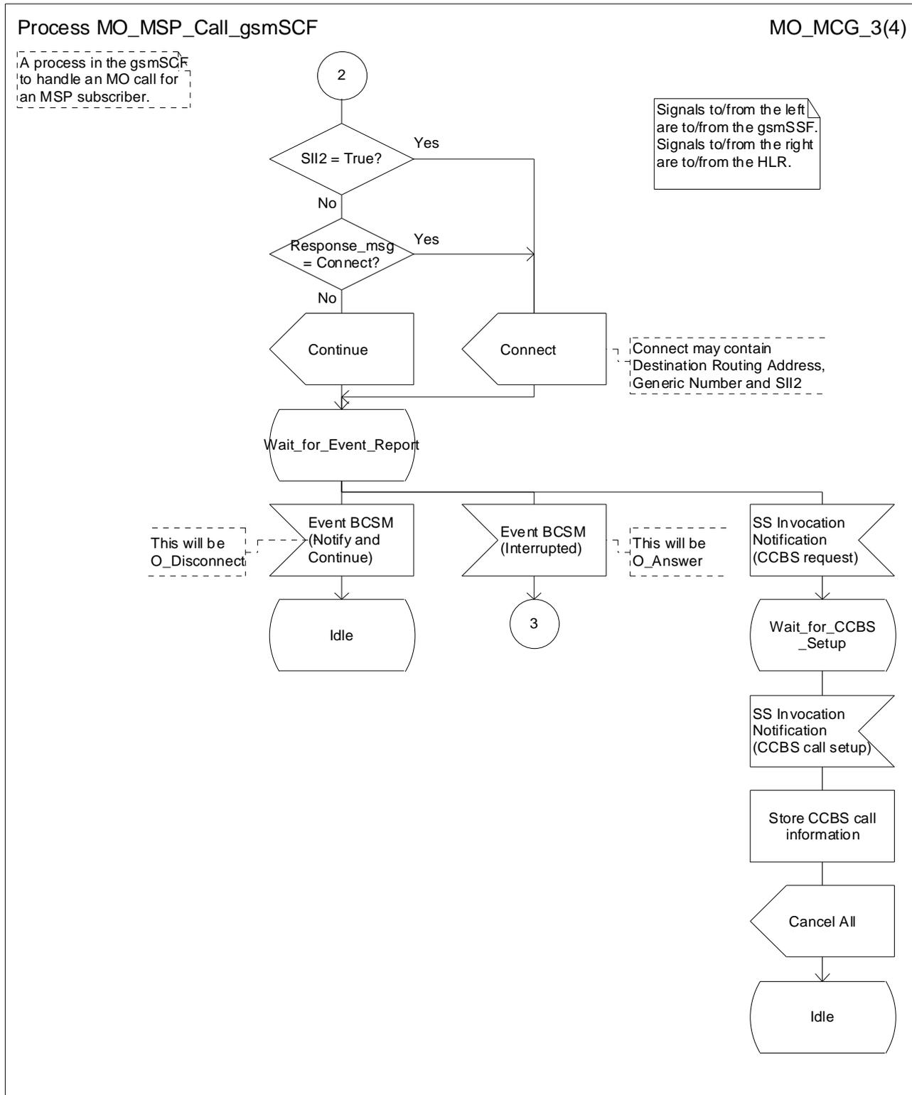
Figure 5c: Process MO\_MSP\_Call\_gsmSCF (sheet 3 of 4)
