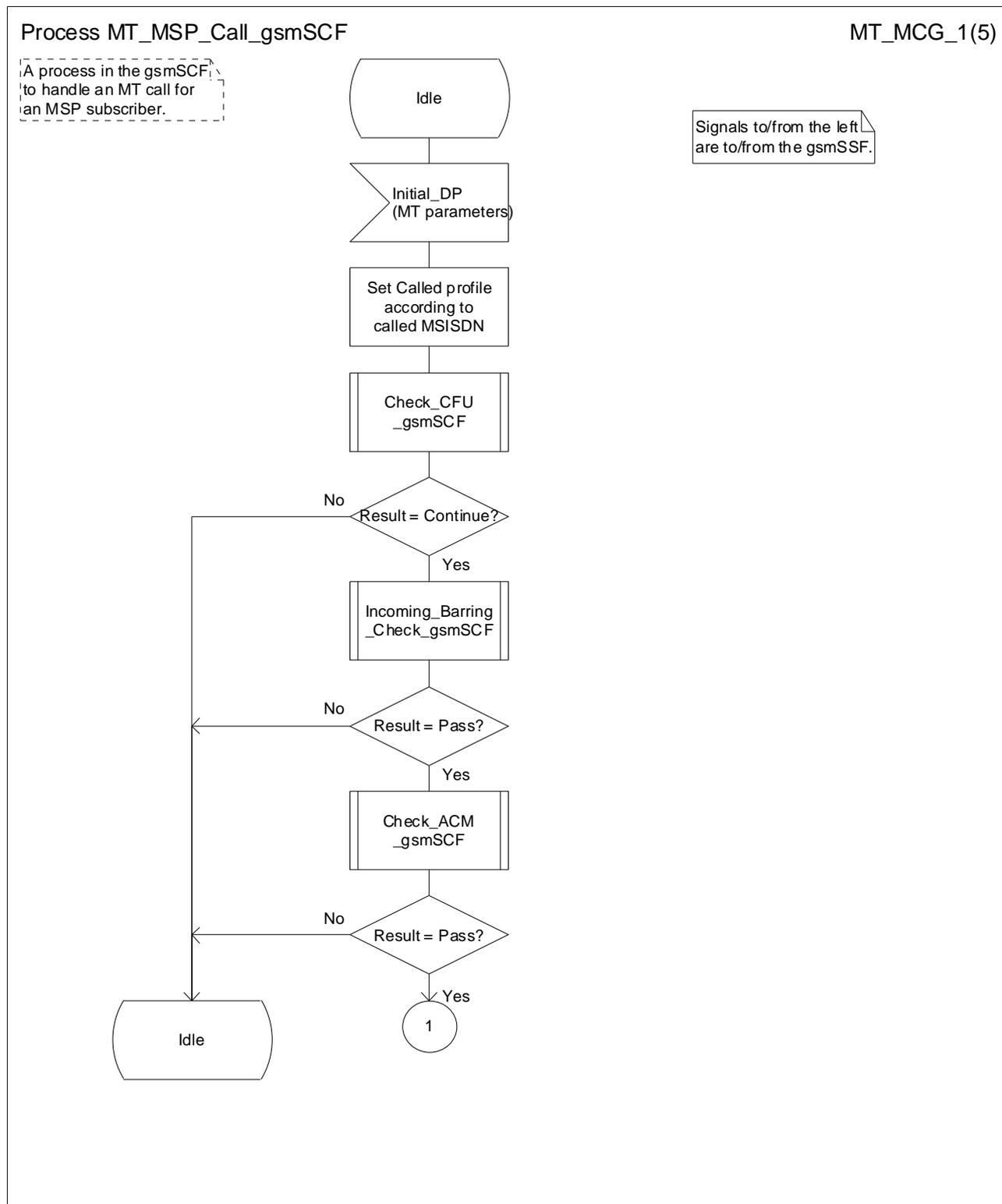
Figure 8a: Process MT\_MSP\_Call\_gsmSCF (sheet 1 of 5)
