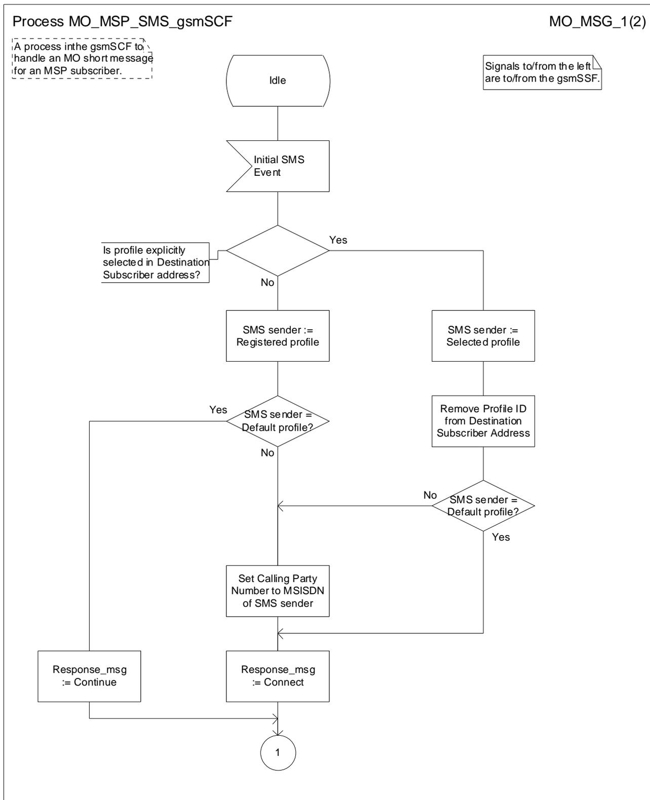
Figure 30a: Process MO\_MSP\_SMS\_gsmSCF (sheet 1 of 2)
