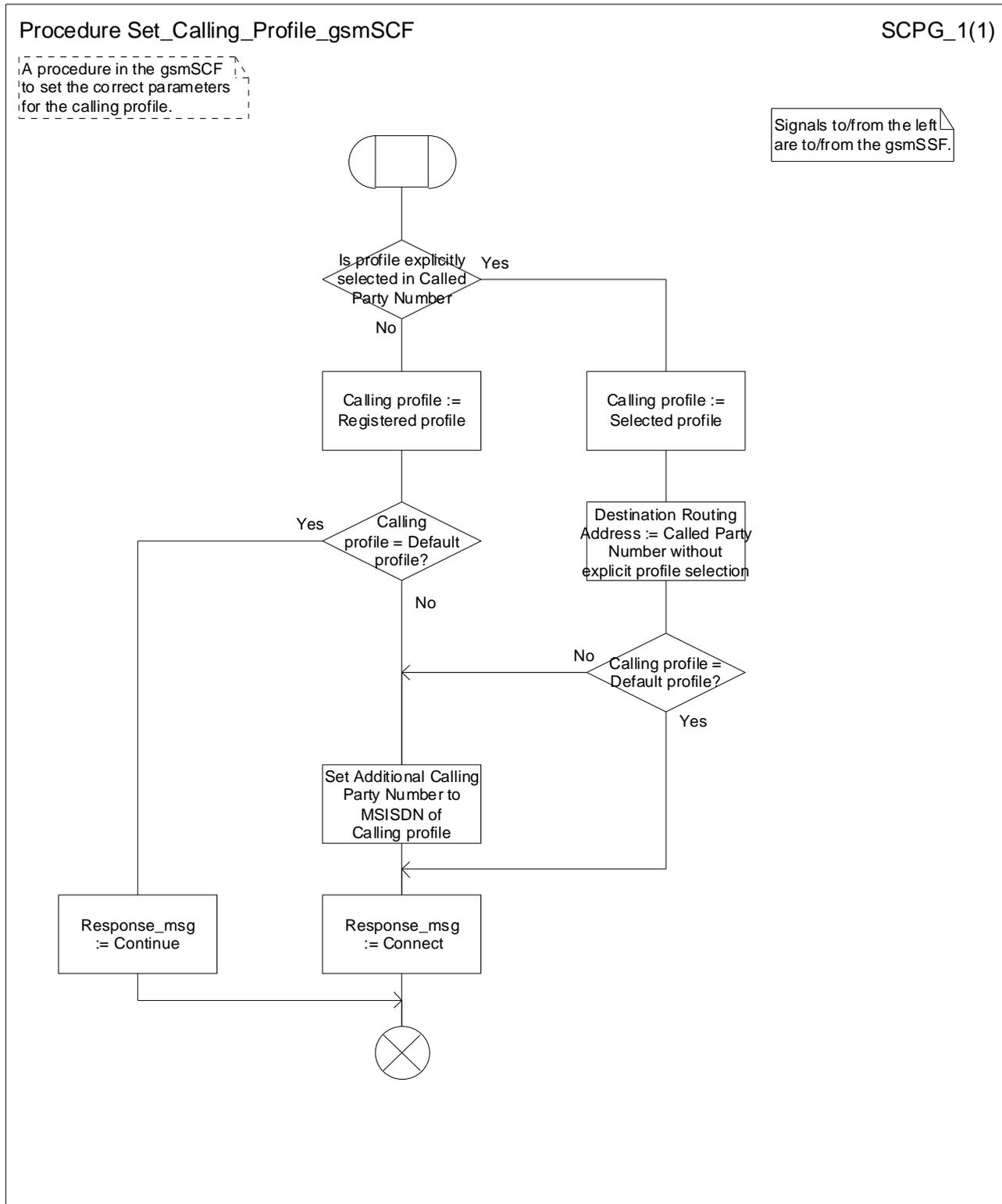
Figure 6: Procedure Set\_Calling\_Profile\_gsmSCF
