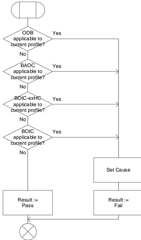
Figure 24: Procedure Outgoing\_Barring\_Check\_gsmSCF
