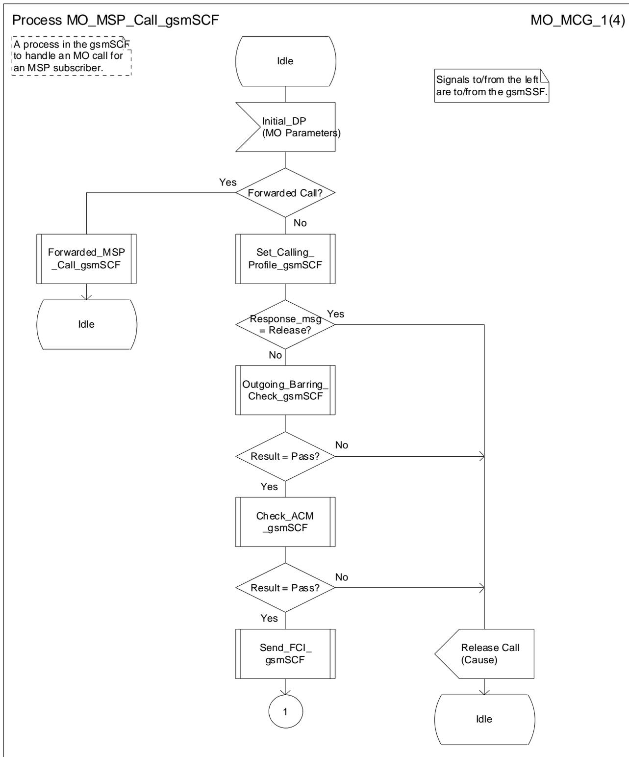
Figure 5a: Process MO\_MSP\_Call\_gsmSCF (sheet 1 of 4)
