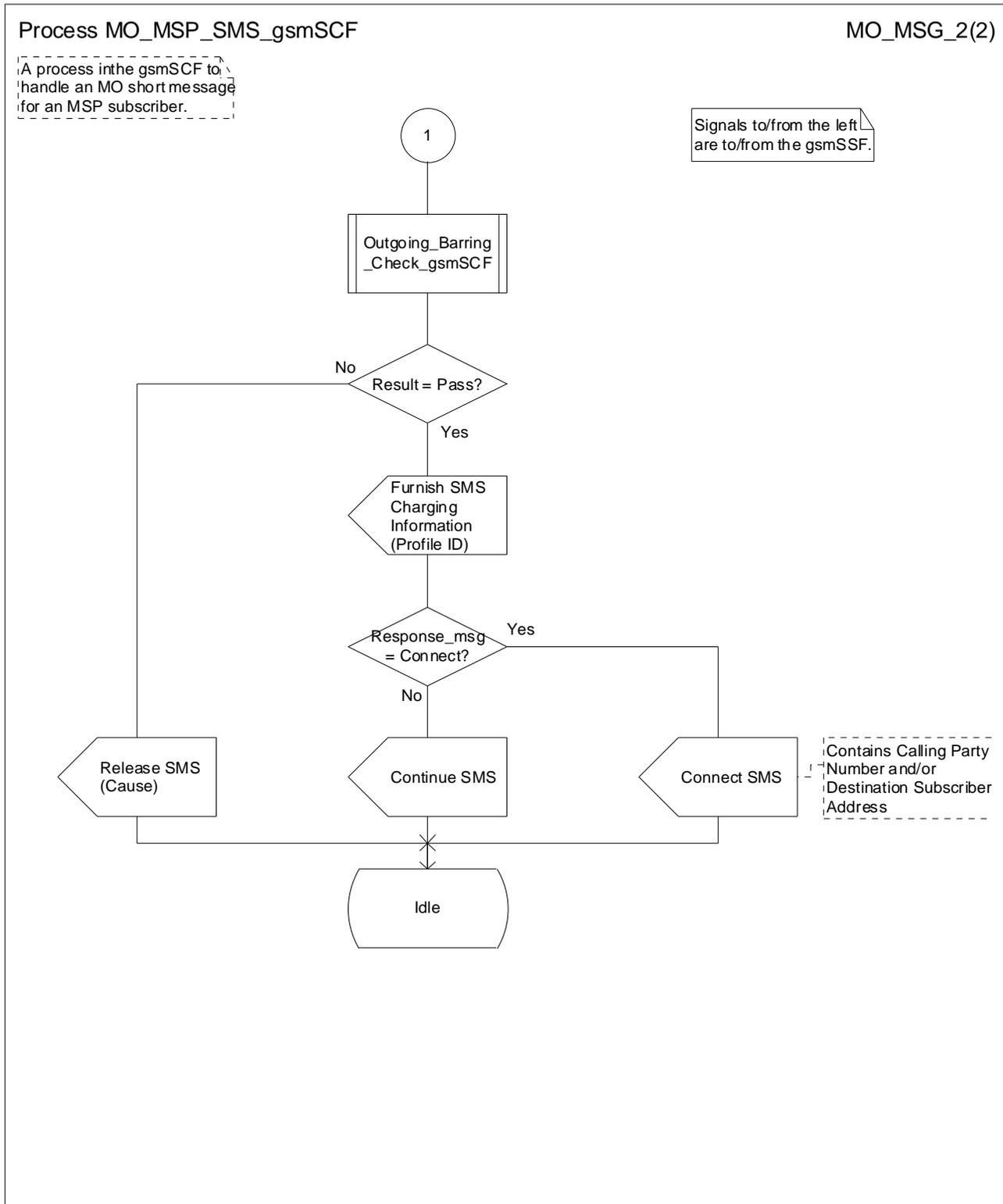
Figure 30b: Process MO\_MSP\_SMS\_gsmSCF (sheet 2 of 2)
