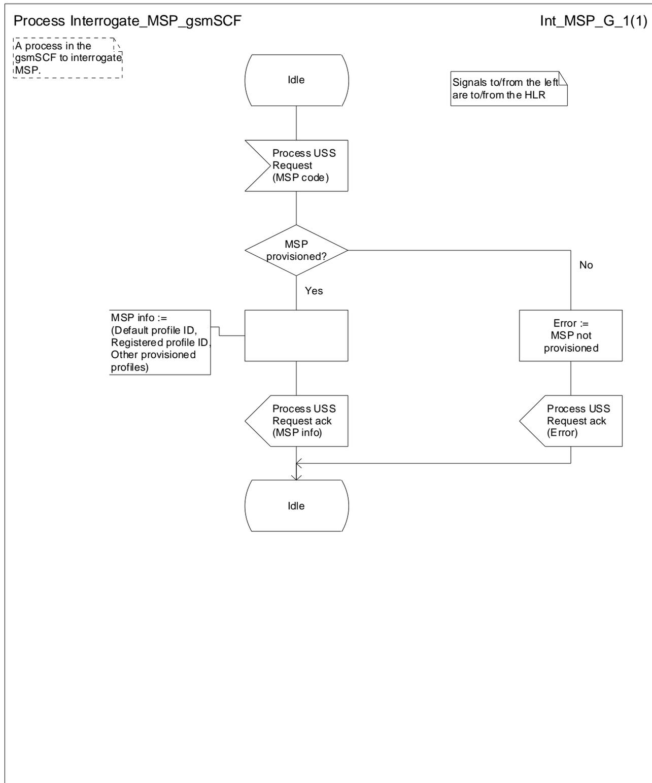
Figure 4: Process Interrogate\_MSP\_gsmSCF
