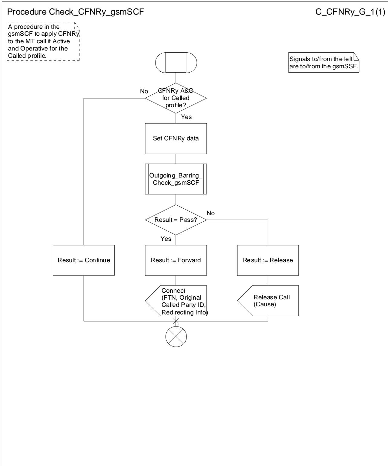
Figure 14: Procedure Check\_CFNRy\_gsmSCF
