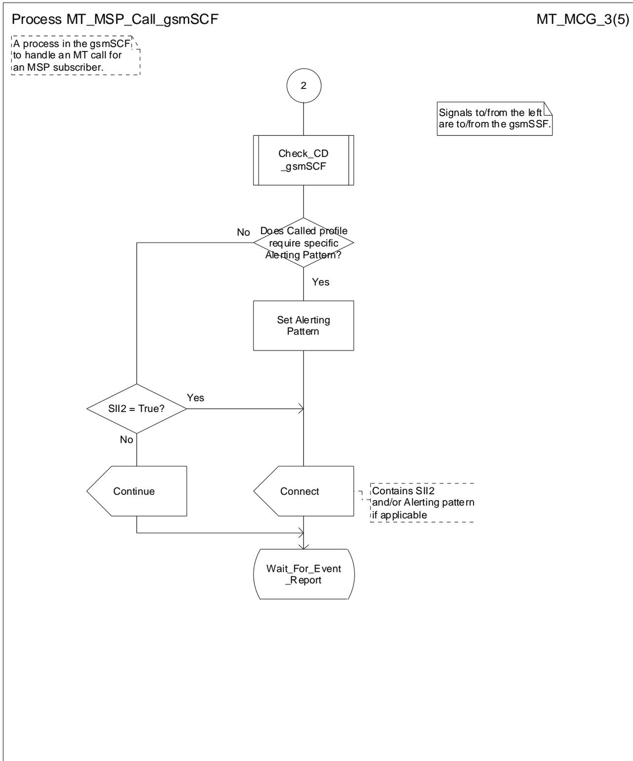
Figure 8c: Process MT\_MSP\_Call\_gsmSCF (sheet 3 of 5)
