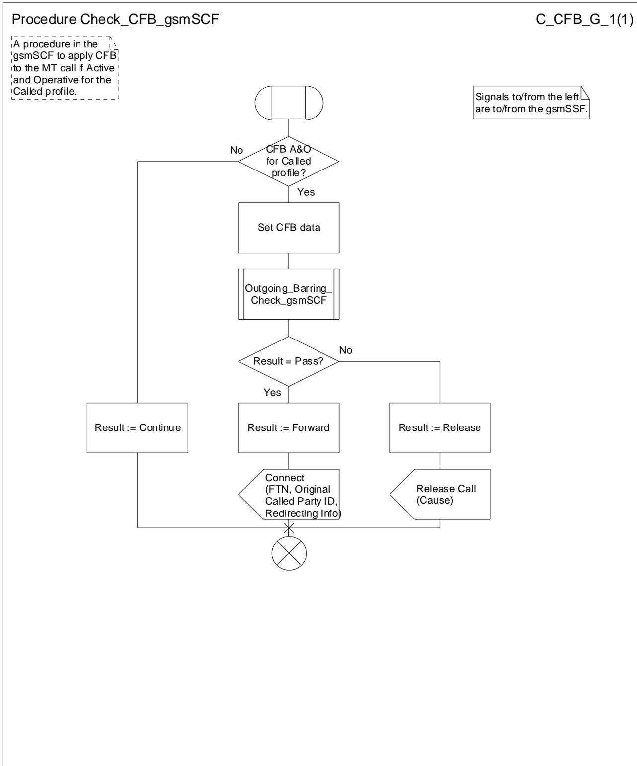
Figure 15: Procedure Check\_CFB\_gsmSCF
