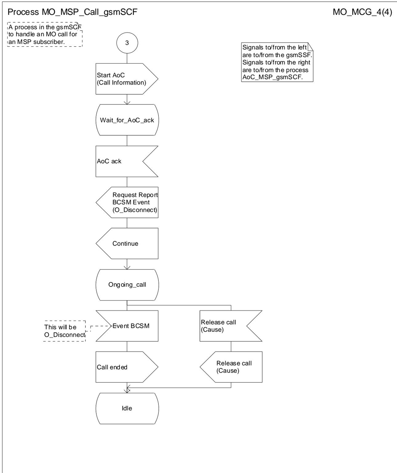
Figure 5d: Process MO\_MSP\_Call\_gsmSCF (sheet 4 of 4)
