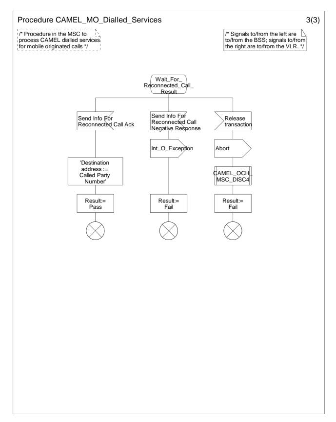
Figure 4.11-3: Procedure CAMEL\_MO\_Dialled\_Services (sheet 3)
