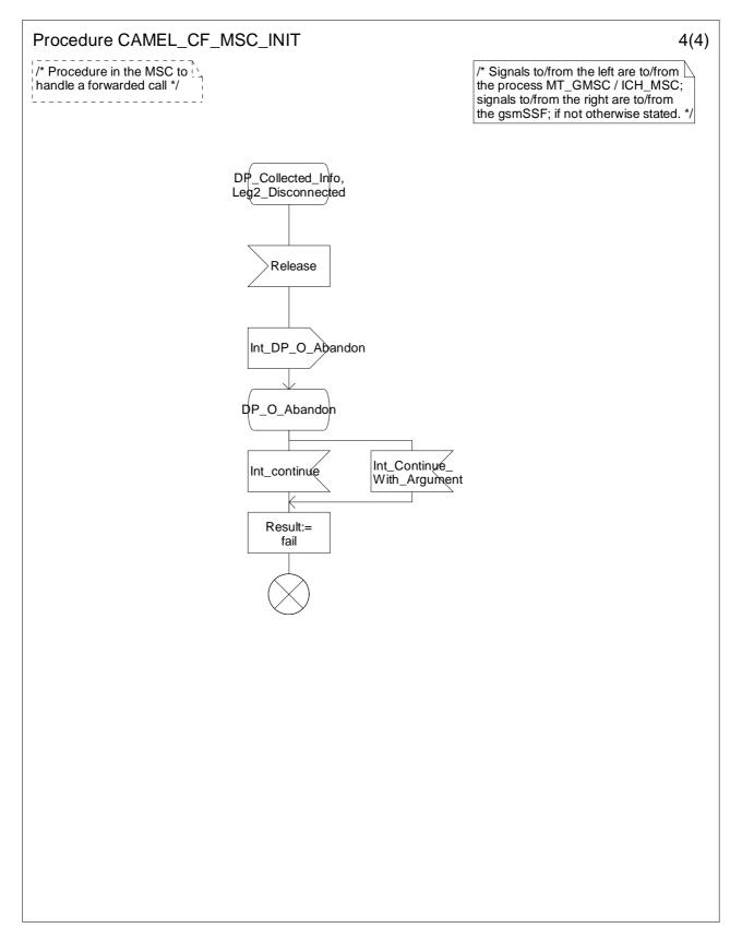
Figure 4.79-4: Procedure CAMEL\_CF\_MSC\_INIT (sheet 4)
