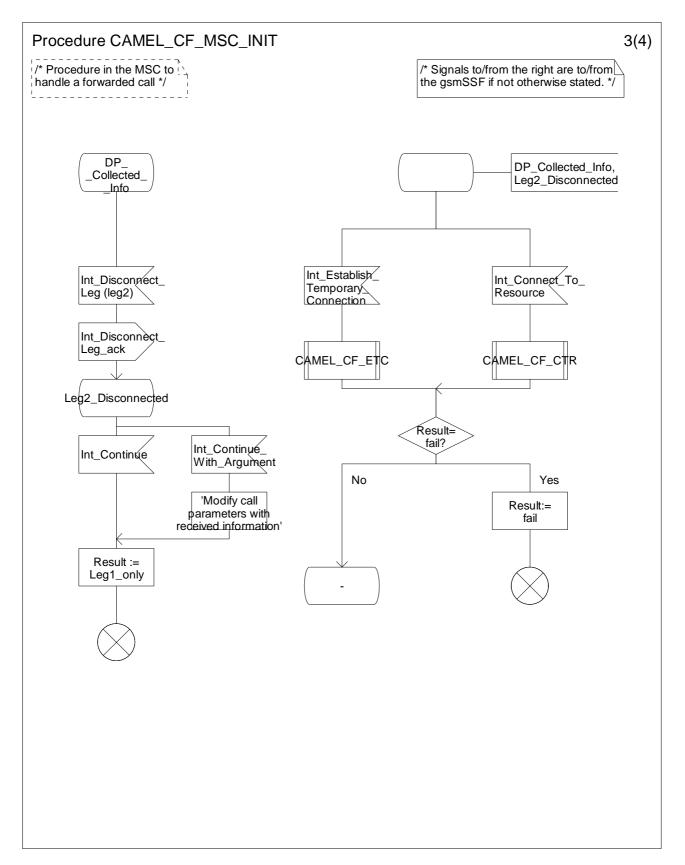
Figure 4.79-3: Procedure CAMEL\_CF\_MSC\_INIT (sheet 3)
