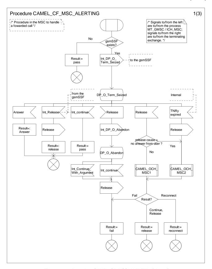
Figure 4.82-1: Procedure CAMEL\_CF\_MSC\_ALERTING (sheet 1)
