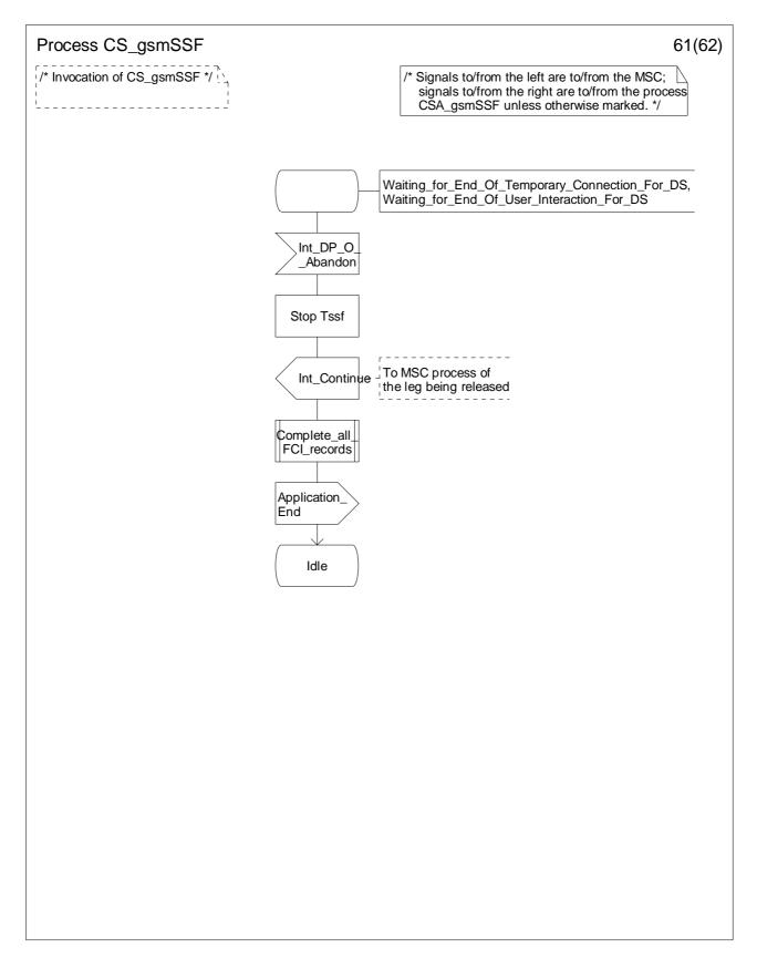
Figure 4.99-61: Process CS\_gsmSSF (sheet 61)
