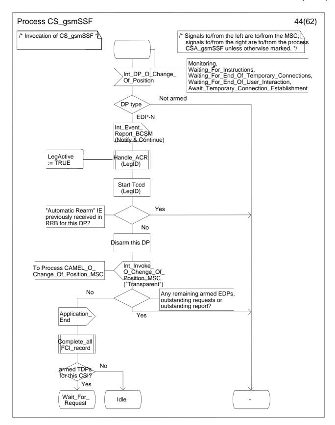
Figure 4.99-44: Process CS\_gsmSSF (sheet 44)
