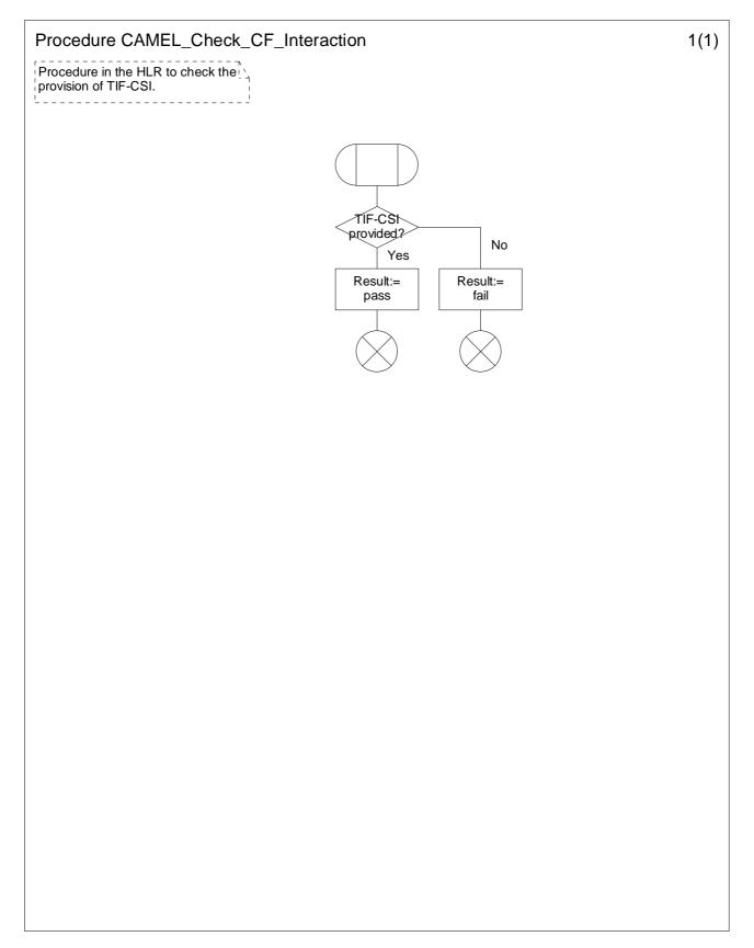
Figure 4.120-1: Procedure CAMEL\_Check\_CF\_Interaction (sheet 1)
