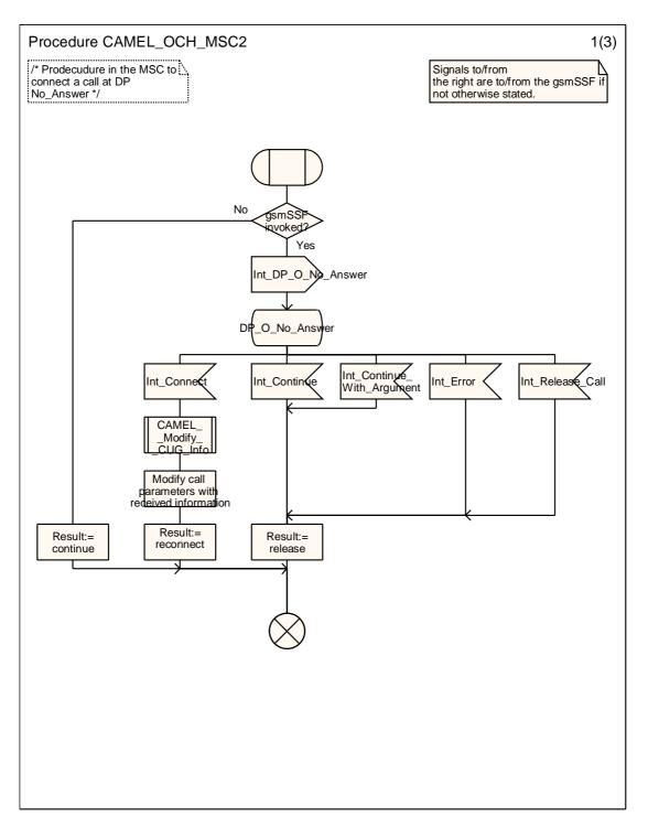
Figure 4.17-1: Procedure CAMEL\_OCH\_MSC2 (sheet 1)
