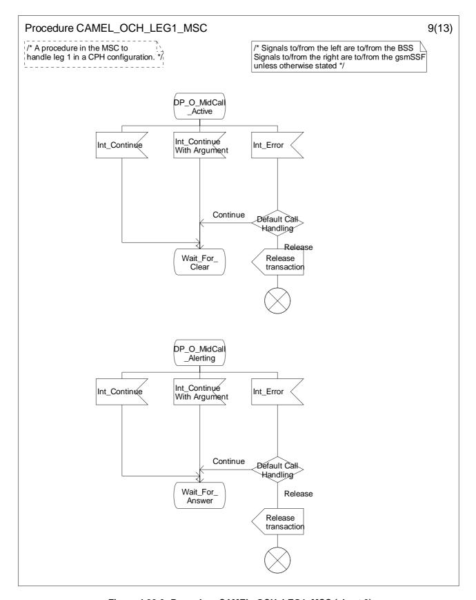
Figure 4.30-9: Procedure CAMEL\_OCH\_LEG1\_MSC (sheet 9)
