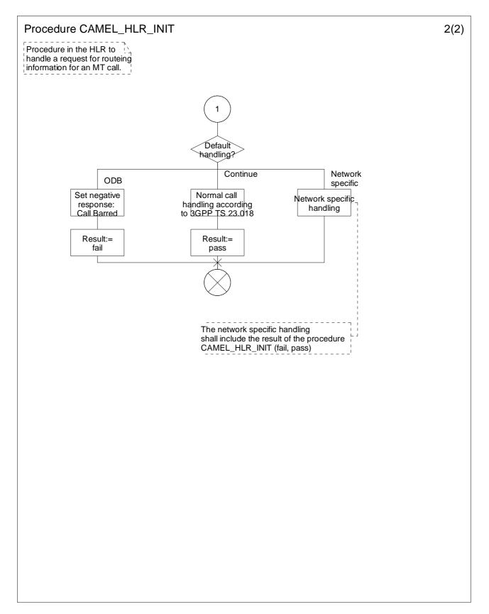
Figure 4.58-2: Procedure CAMEL\_HLR\_INIT (sheet 2)
