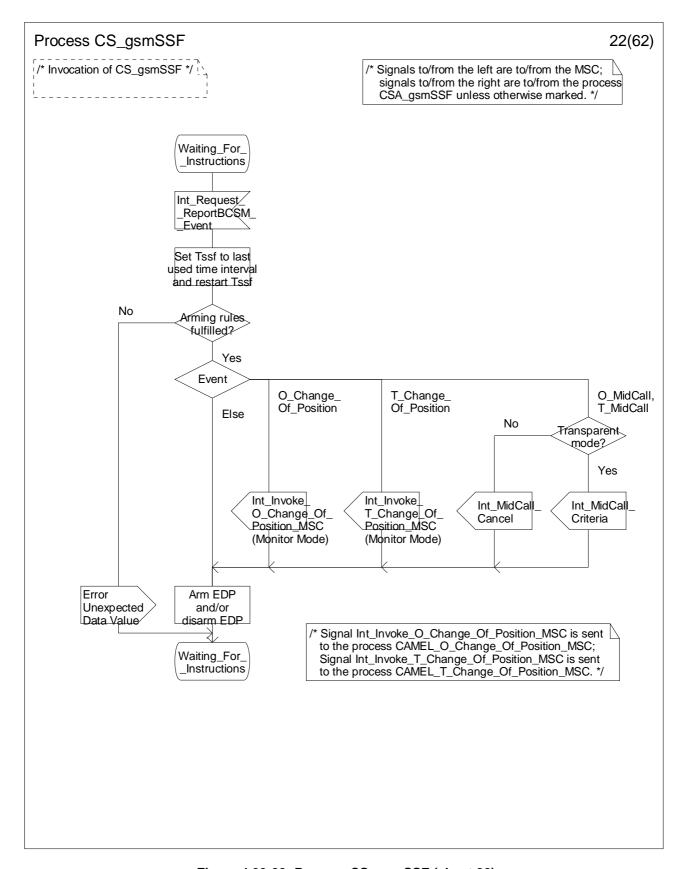
Figure 4.99-22: Process CS\_gsmSSF (sheet 22)
