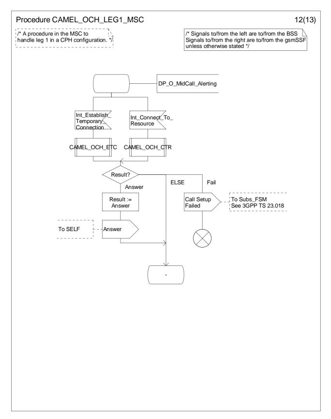
Figure 4.30-12: Procedure CAMEL\_OCH\_LEG1\_MSC (sheet 12)
