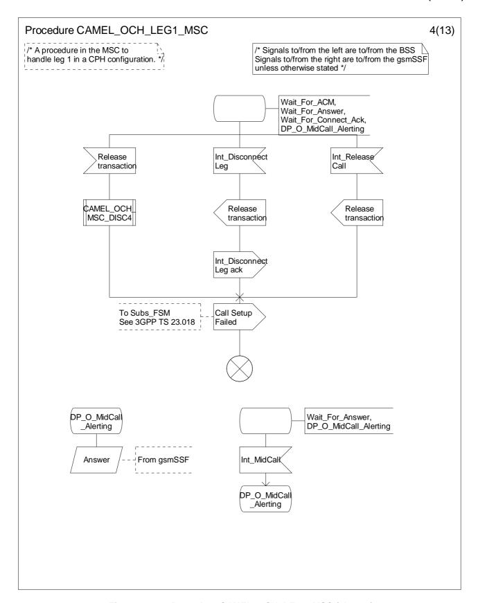
Figure 4.30-4: Procedure CAMEL\_OCH\_LEG1\_MSC (sheet 4)
