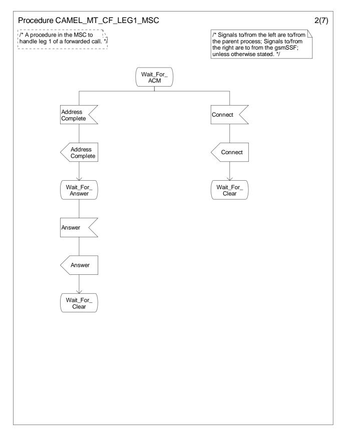
Figure 4.86-2: Procedure CAMEL\_MT\_CF\_LEG1\_MSC (sheet 2)
