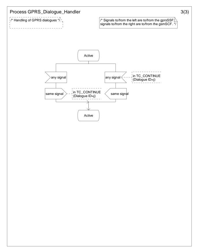
Figure 6.18-3: Process GPRS\_Dialogue\_Handler (sheet 3)
