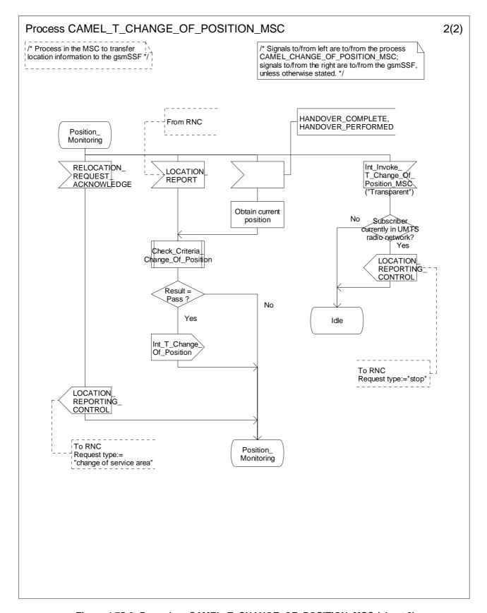
Figure 4.75-2: Procedure CAMEL\_T\_CHANGE\_OF\_POSITION\_MSC (sheet 2)
