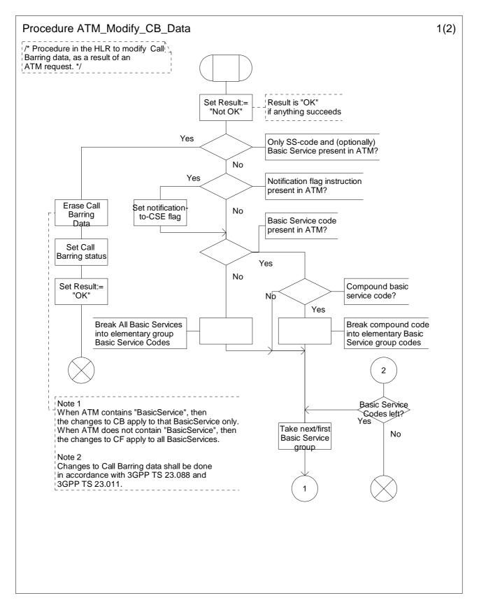
Figure 10.7-1: Procedure ATM\_Modify\_CB\_Data (sheet 1)
