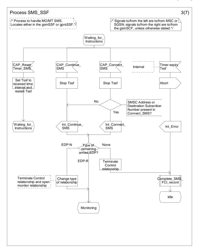
Figure 7.15-3: Process SMS\_SSF (sheet 3)
