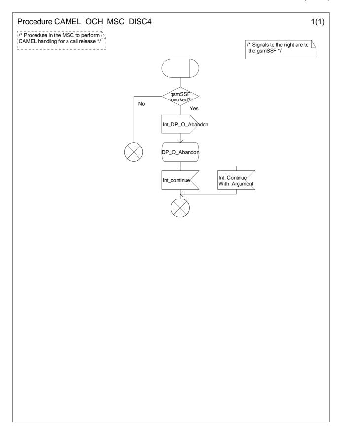
Figure 4.21-1: Procedure CAMEL\_OCH\_MSC\_DISC4 (sheet 1)
