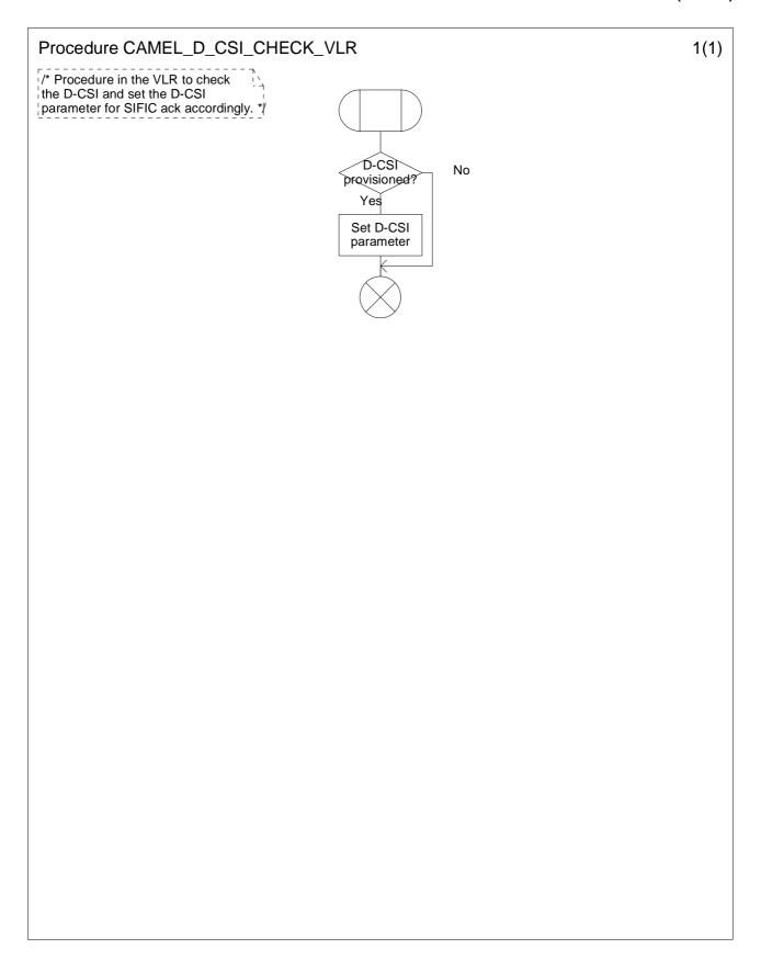
Figure 4.67-1: Procedure CAMEL\_D\_CSI\_Check\_VLR (sheet 1)
