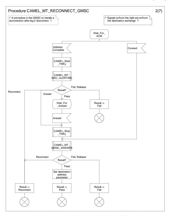
Figure 4.56-2: Procedure CAMEL\_MT\_RECONNECT\_GMSC (sheet 2)
