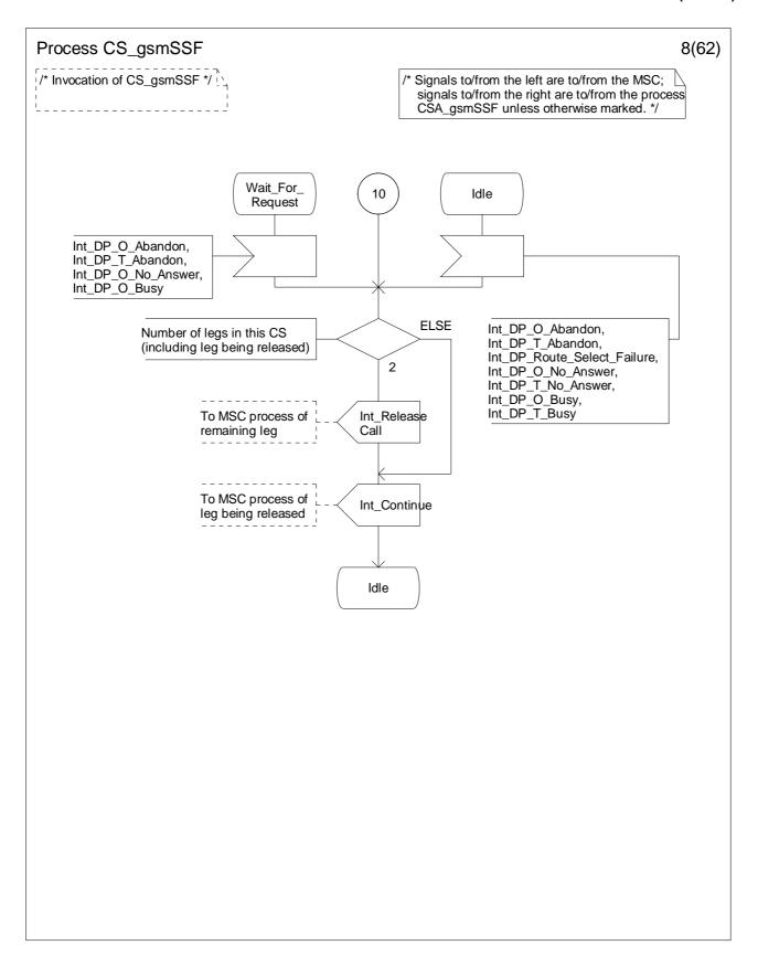
Figure 4.99-8: Process CS\_gsmSSF (sheet 8)
