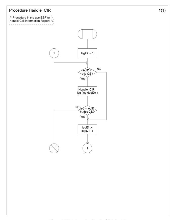
Figure 4.106-1: Procedure Handle\_CIR (sheet 1)
