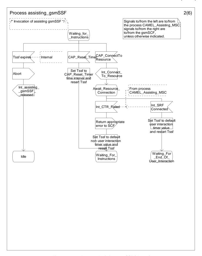
Figure 4.118-2: Process Assisting\_gsmSSF (sheet 2)
