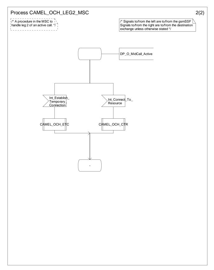
Figure 4.32-2: Process CAMEL\_OCH\_LEG2\_MSC (sheet 2)
