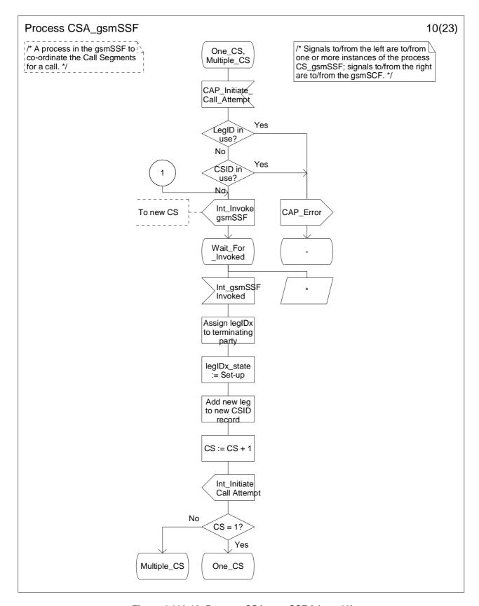
Figure 4.116-10: Process CSA\_gsmSSF (sheet 10)
