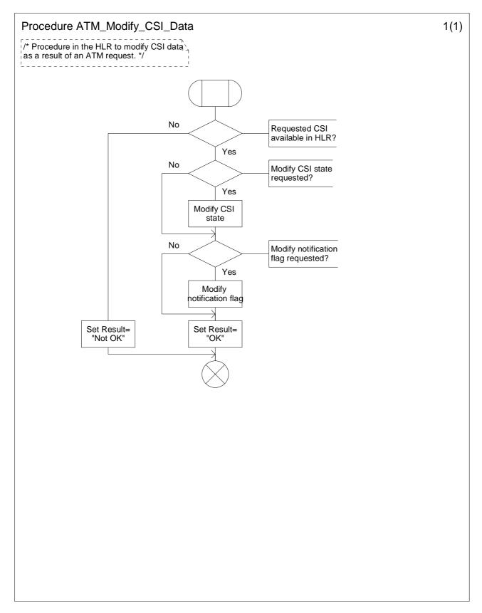
Figure 10.5-1: Procedure ATM\_Modify\_CSI\_Data (sheet 1)
