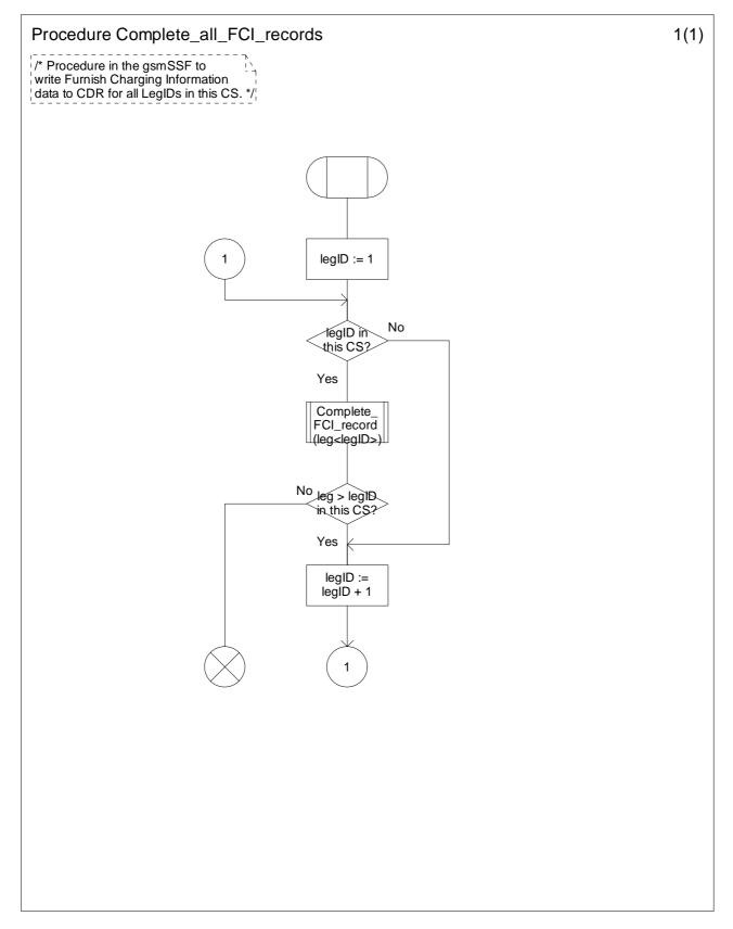
Figure 4.109-1: Procedure Complete\_all\_FCI\_records (sheet 1)
