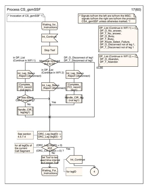
Figure 4.99-17: Process CS\_gsmSSF (sheet 17)
