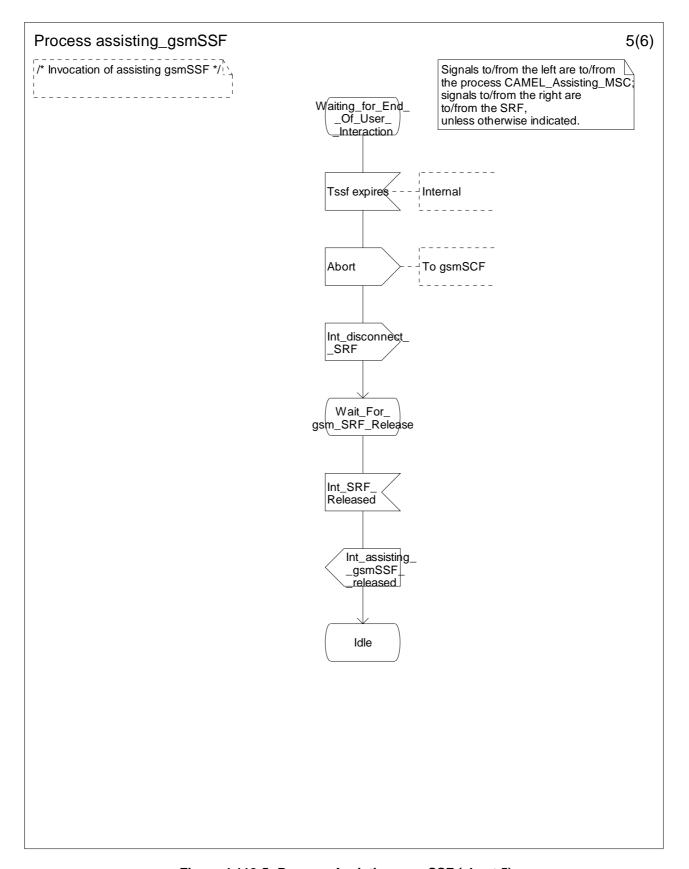
Figure 4.118-5: Process Assisting\_gsmSSF (sheet 5)
