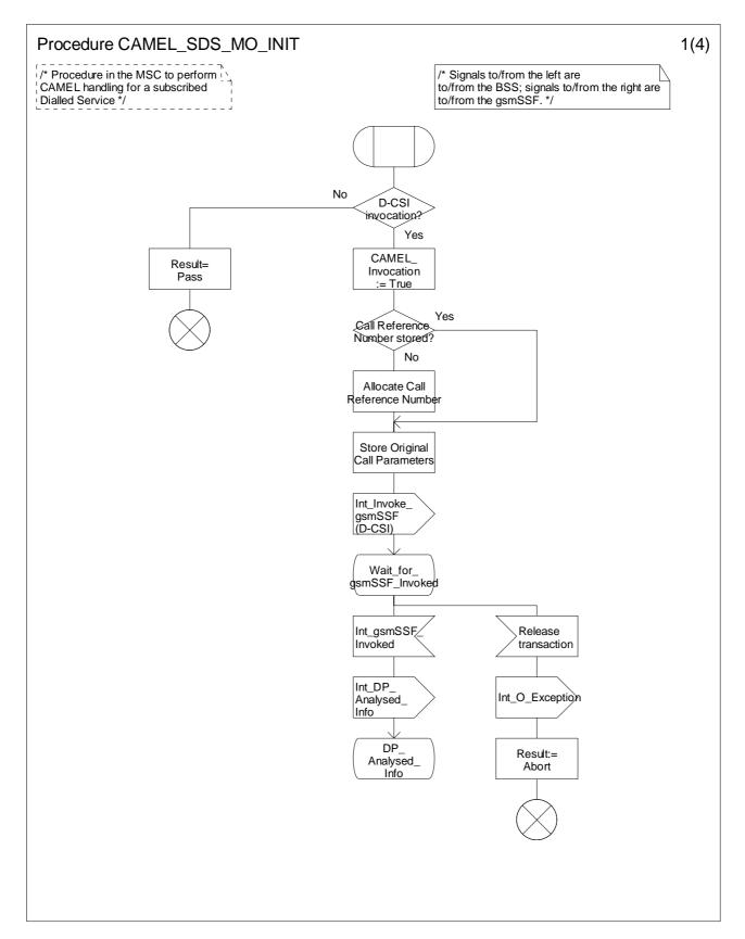
Figure 4.12-1: Procedure CAMEL\_SDS\_MO\_Init (sheet 1)
