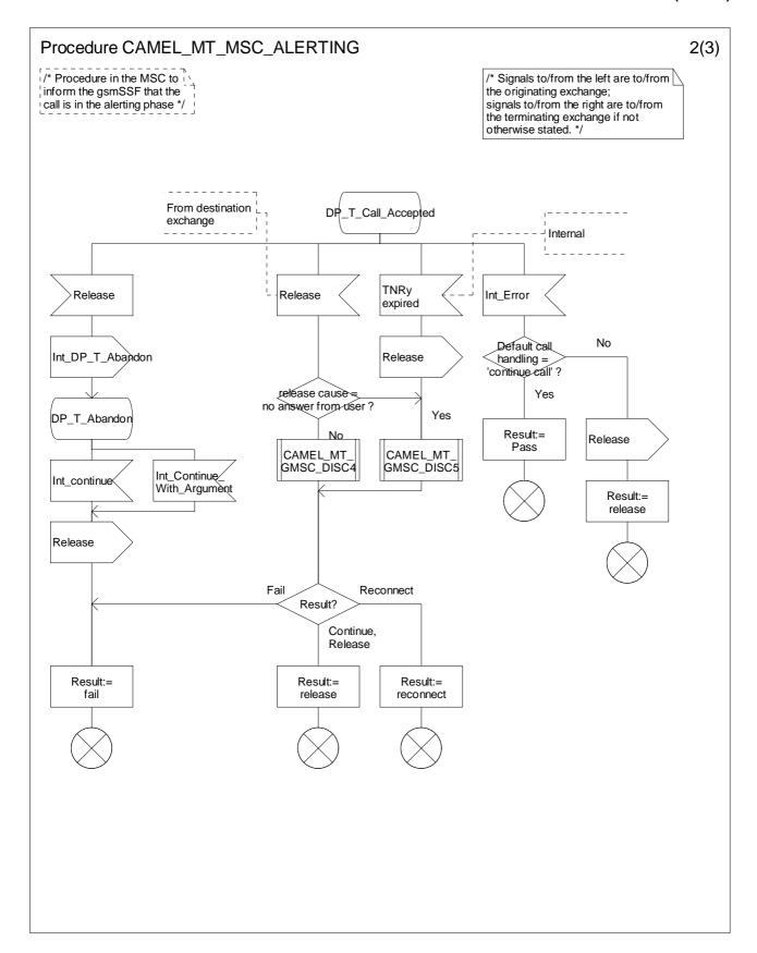
Figure 4.43-2: Procedure CAMEL\_MT\_MSC\_ALERTING (sheet 2)
