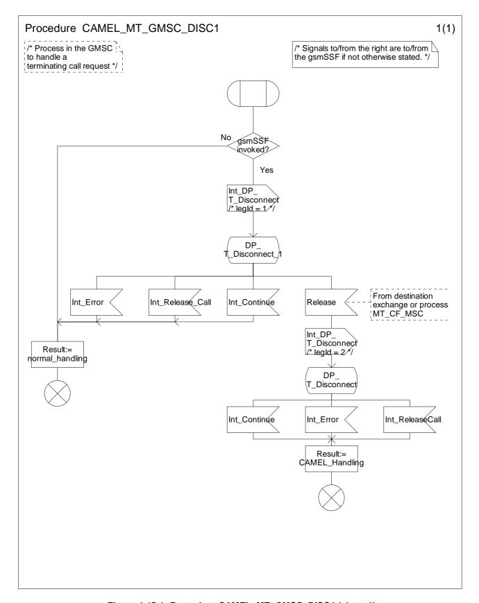
Figure 4.45-1: Procedure CAMEL\_MT\_GMSC\_DISC1 (sheet 1)
