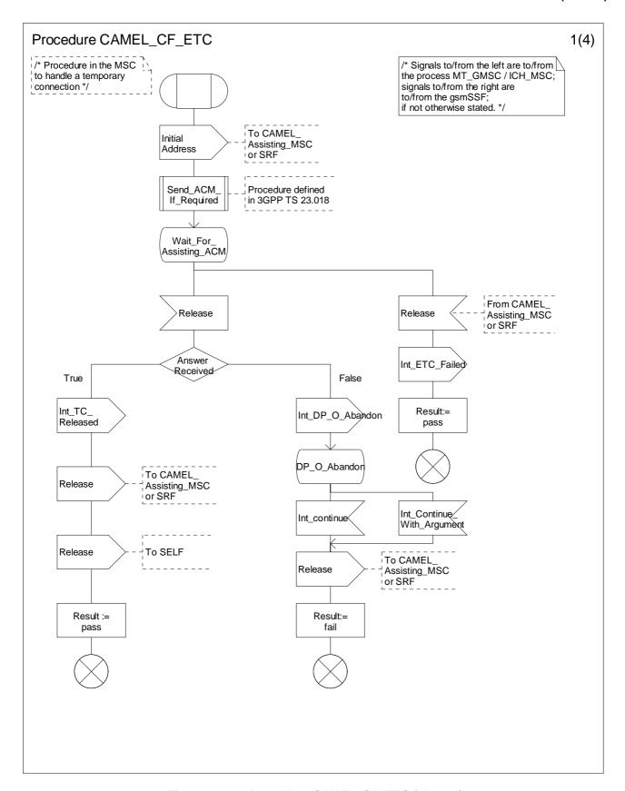
Figure 4.84-1: Procedure CAMEL\_CF\_ETC (sheet 1)
