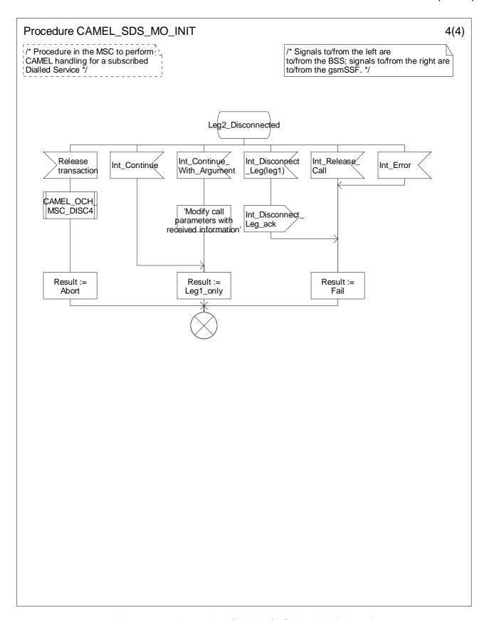
Figure 4.12-4: Procedure CAMEL\_SDS\_MO\_INIT (sheet 4)
