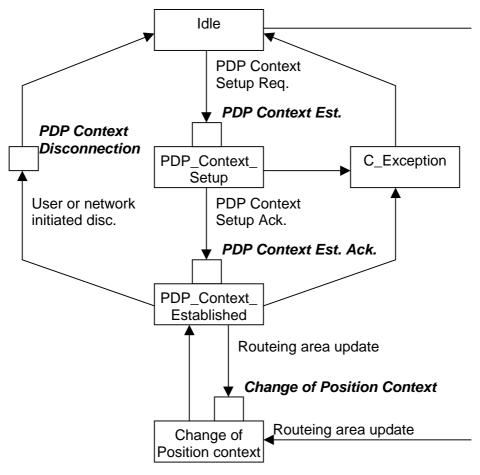
Figure 6.4: GPRS PDP Context State Model
