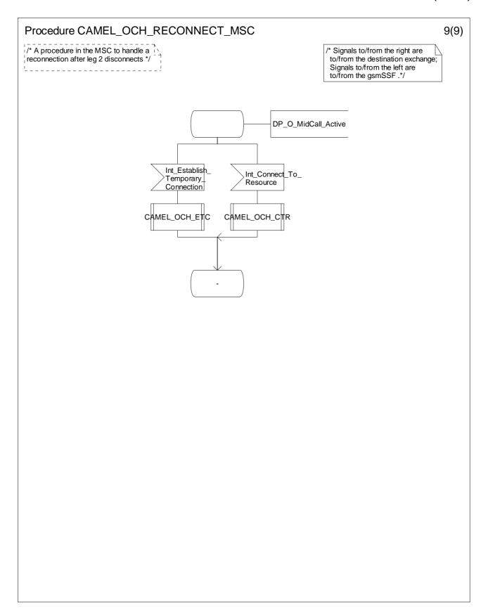
Figure 4.33-9: Procedure CAMEL\_OCH\_RECONNECT\_MSC (sheet 9)
