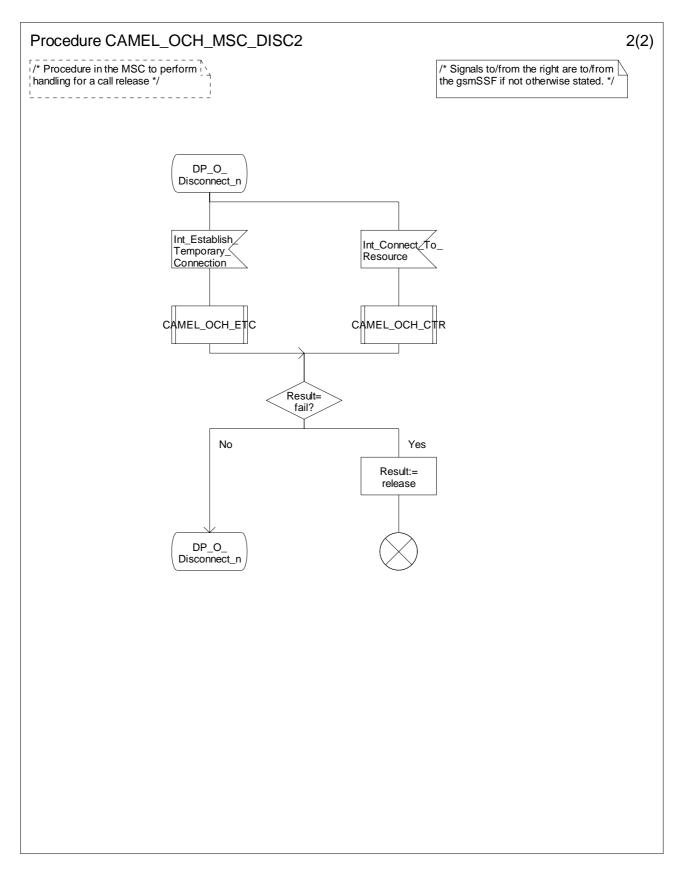
Figure 4.19-2: Procedure CAMEL\_OCH\_MSC\_DISC2 (sheet 2)
