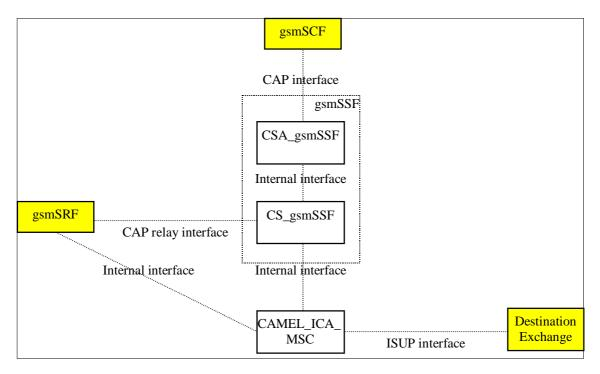
Figure 4.9-8: gsmSCF initiated call case (gsmSSF relay)
