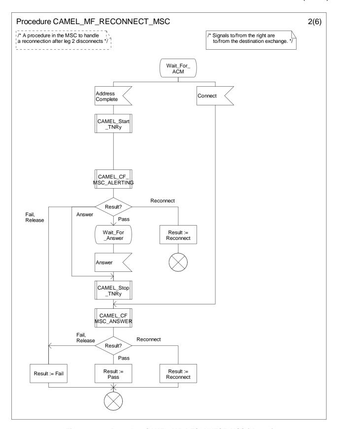
Figure 4.88-2: Procedure CAMEL\_MF\_RECONNECT\_MSC (sheet 2)
