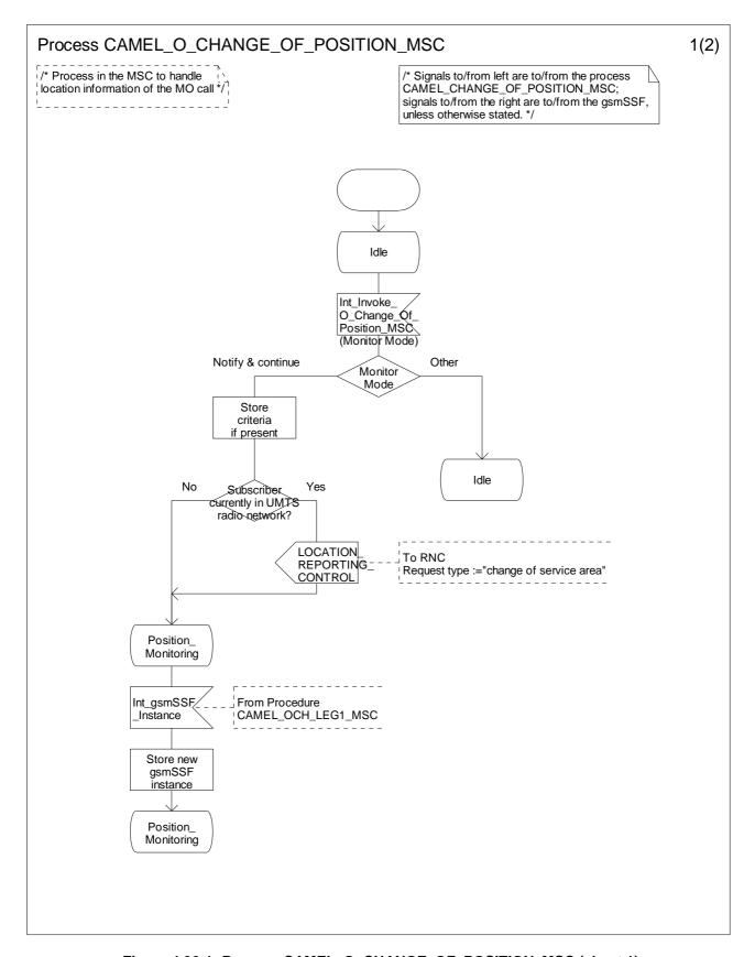
Figure 4.36-1: Process CAMEL\_O\_CHANGE\_OF\_POSITION\_MSC (sheet 1)
