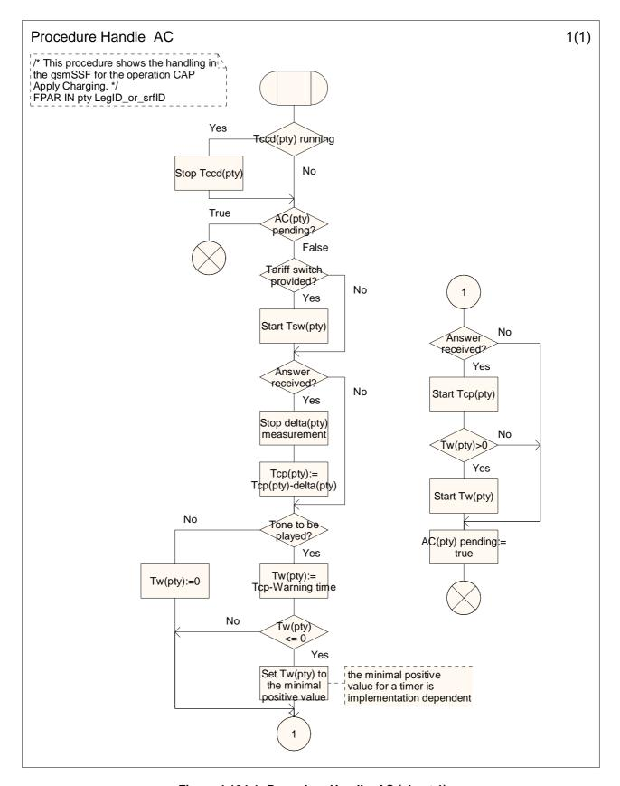
Figure 4.104-1: Procedure Handle\_AC (sheet 1)
