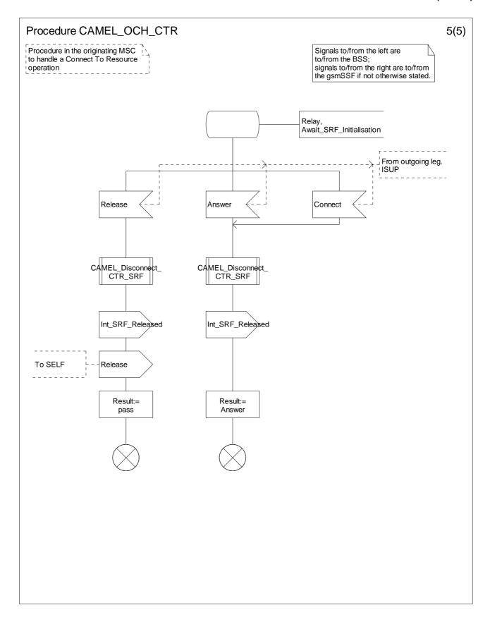
Figure 4.24-5: Procedure CAMEL\_OCH\_CTR (sheet 5)
