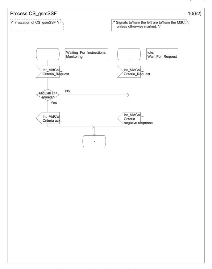
Figure 4.99-10: Process CS\_gsmSSF (sheet 10)
