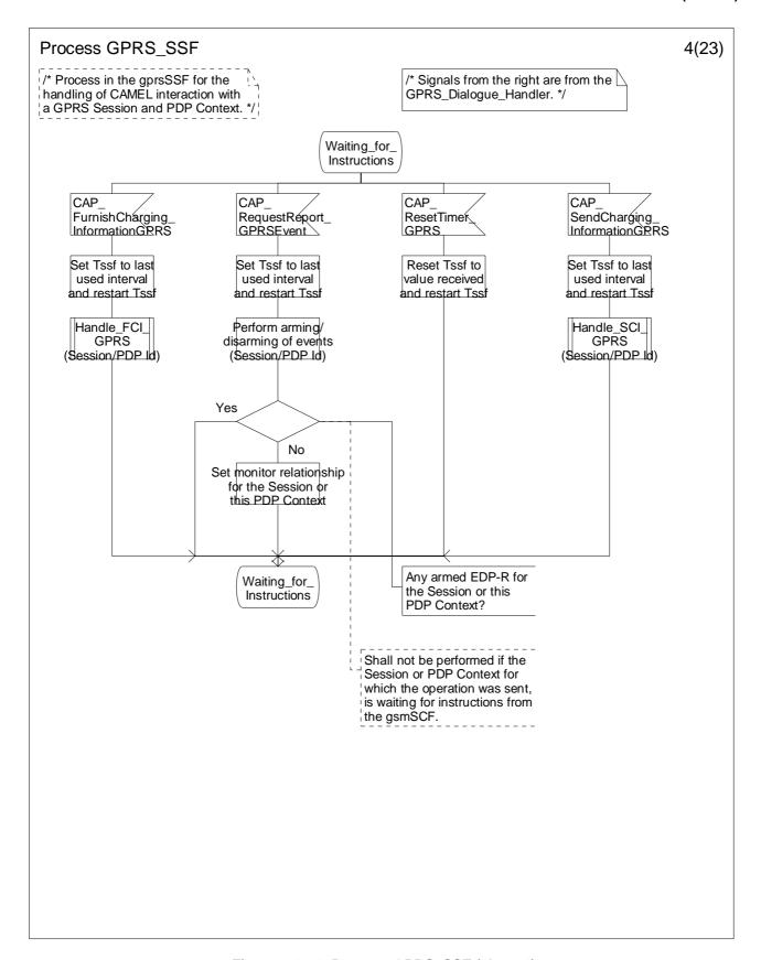
Figure 6.17-4: Process GPRS\_SSF (sheet 4)
