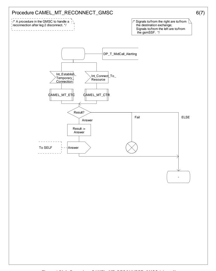
Figure 4.56-6: Procedure CAMEL\_MT\_RECONNECT\_GMSC (sheet 6)
