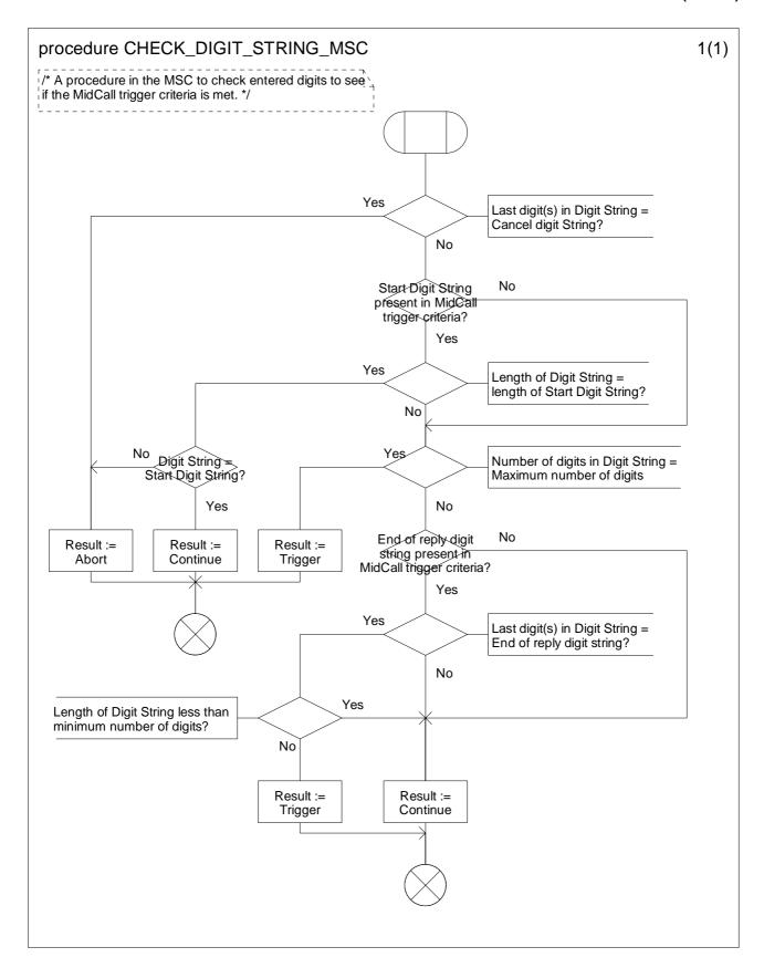
Figure 4.31-1: Procedure CHECK\_DIGIT\_STRING\_MSC (sheet 1)
