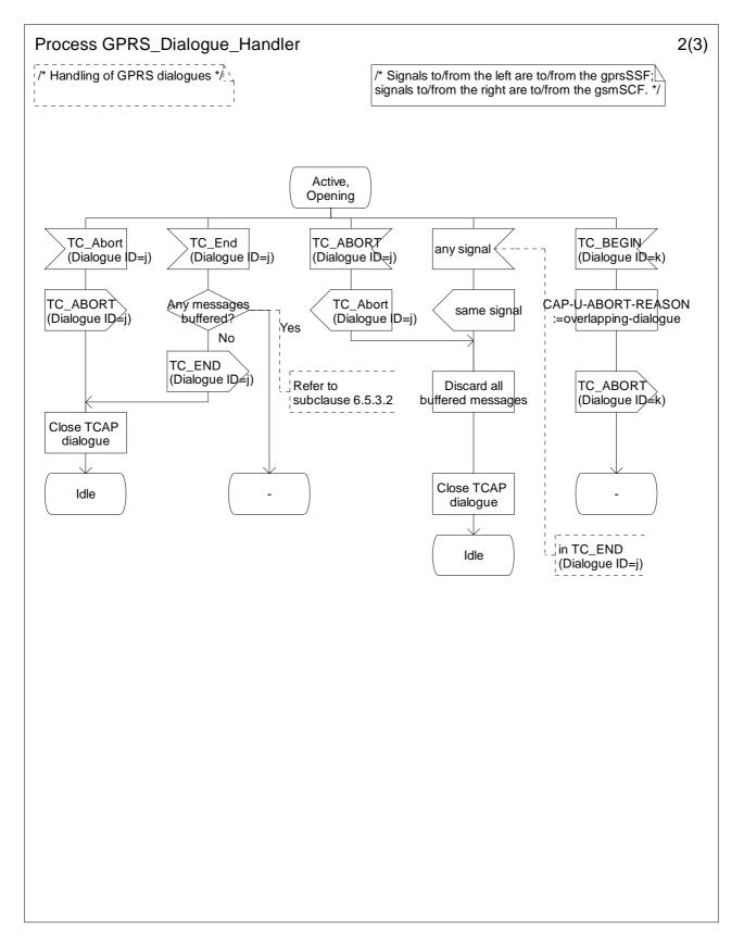
Figure 6.18-2: Process GPRS\_Dialogue\_Handler (sheet 2)
