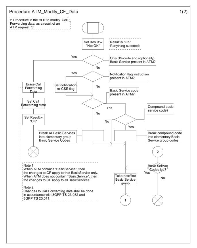
Figure 10.6-1: Procedure ATM\_Modify\_CF\_Data (sheet 1)
