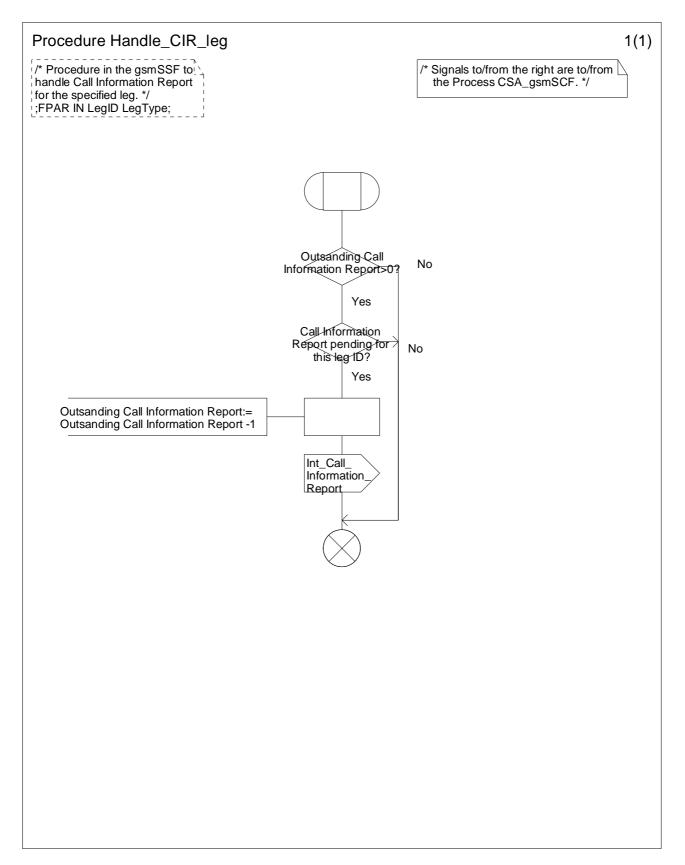
Figure 4.107-1: Procedure Handle\_CIR\_leg (sheet 1)
