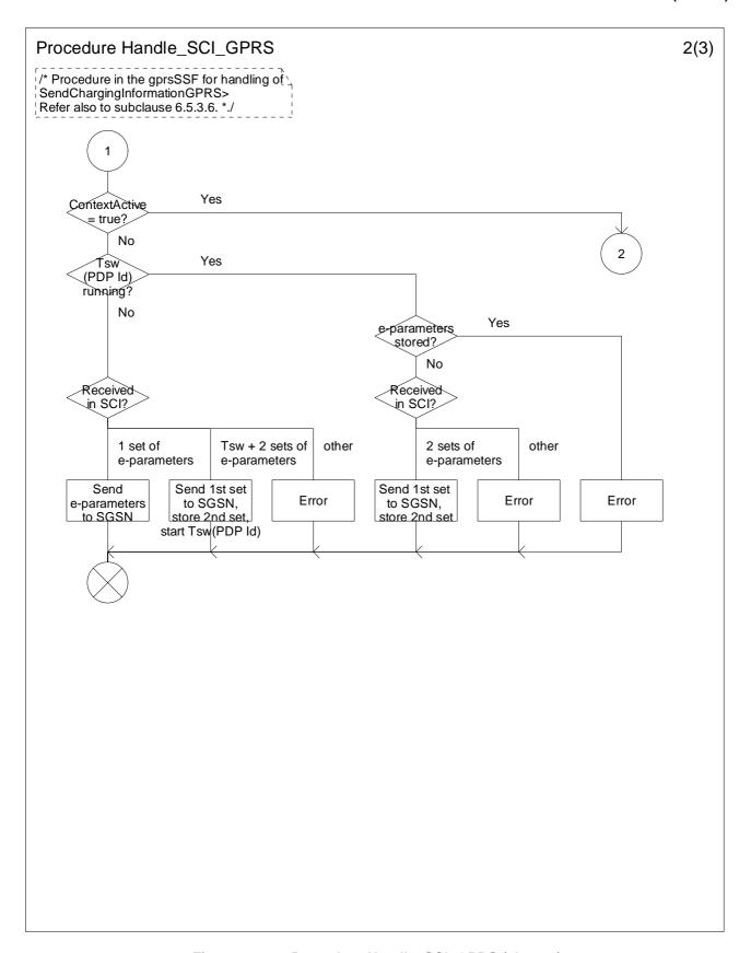
Figure 6.23-2: Procedure Handle\_SCI\_GPRS (sheet 2)
