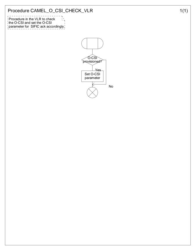
Figure 4.66-1: Procedure CAMEL\_O\_CSI\_Check\_VLR (sheet 1)
