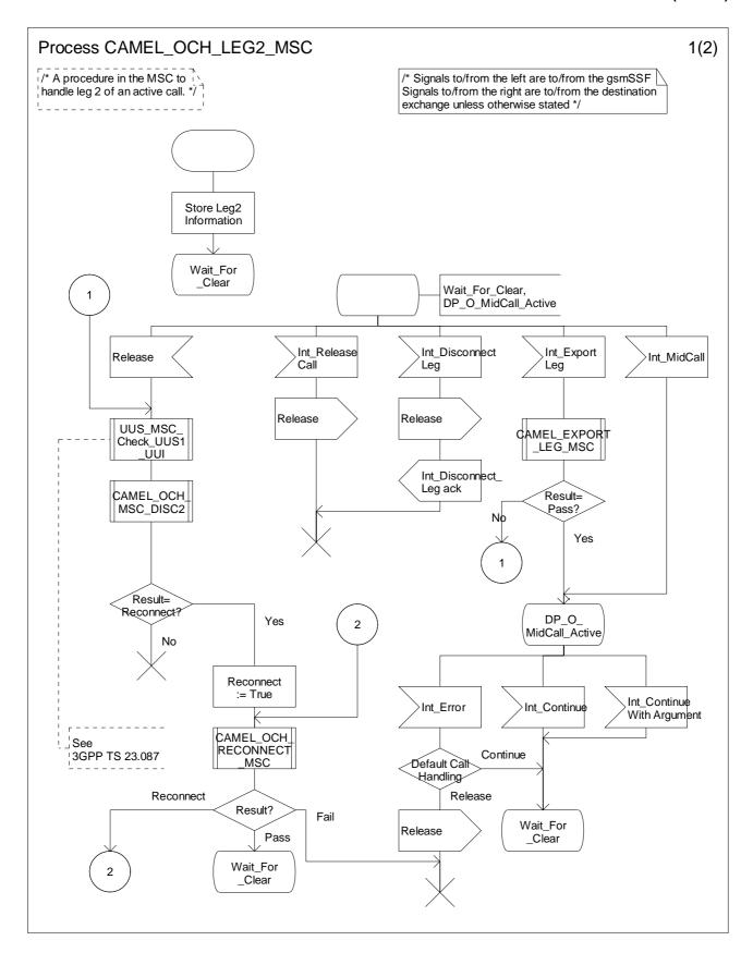
Figure 4.32-1: Process CAMEL\_OCH\_LEG2\_MSC (sheet 1)
