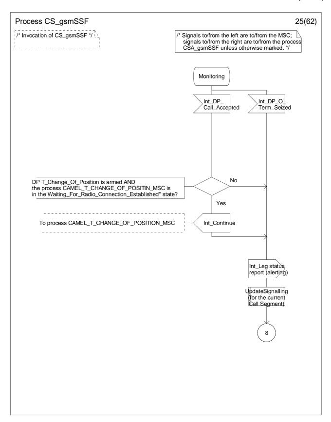
Figure 4.99-25: Process CS\_gsmSSF (sheet 25)
