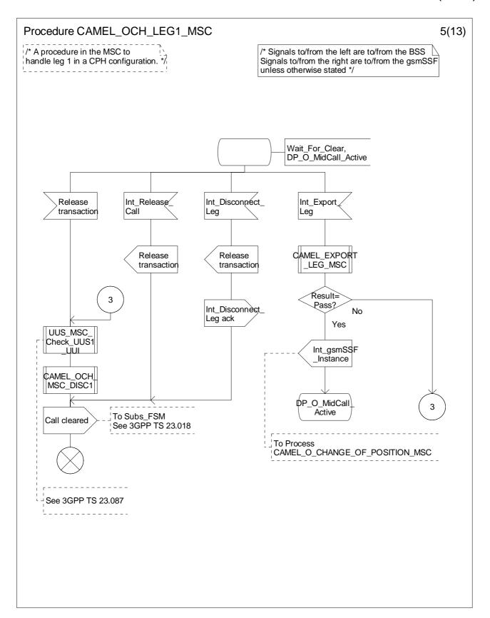
Figure 4.30-5: Procedure CAMEL\_OCH\_LEG1\_MSC (sheet 5)
