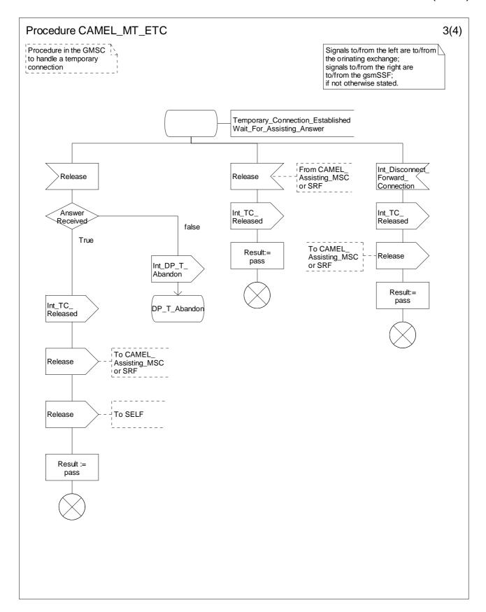
Figure 4.51-3: Procedure CAMEL\_MT\_ETC (sheet 3)
