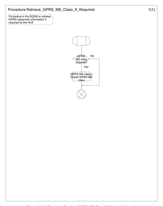
Figure 11.6-1: Procedure Retrieve\_GPRS\_MS\_Class\_If\_Required (sheet 1)
