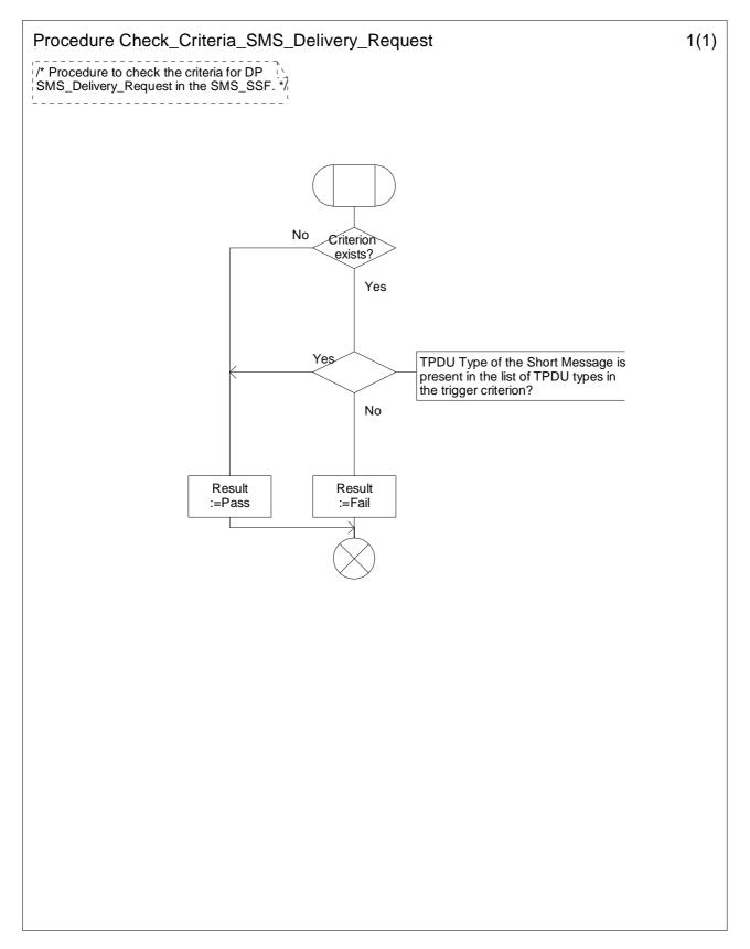
Figure 7.16-1: Procedure Check\_Criteria\_SMS\_Delivery\_Request (Sheet 1)
