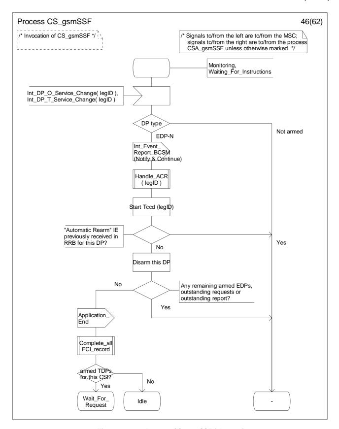
Figure 4.99-46: Process CS\_gsmSSF (sheet 46)
