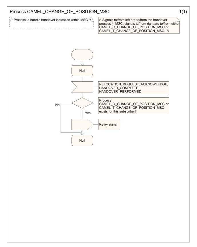
Figure 4.35-1: Process CAMEL\_CHANGE\_OF\_POSITION\_MSC (sheet 1)
