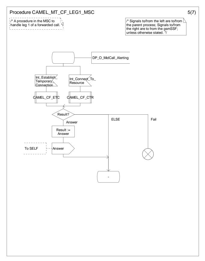
Figure 4.86-5: Procedure CAMEL\_MT\_CF\_LEG1\_MSC (sheet 5)
