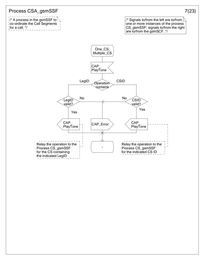
Figure 4.116-7: Process CSA\_gsmSSF (sheet 7)
