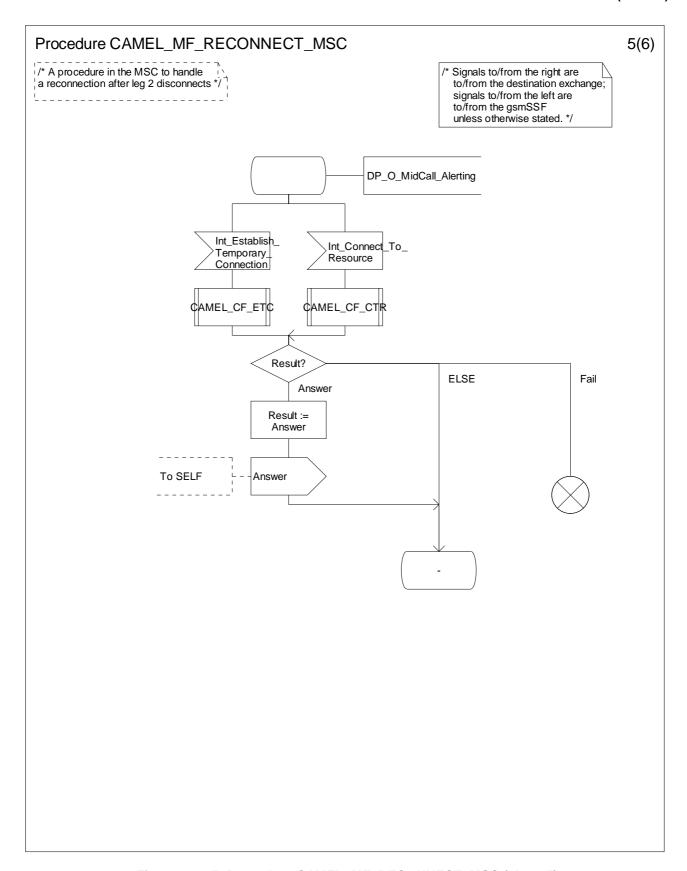
Figure 4.88-5: Procedure CAMEL\_MF\_RECONNECT\_MSC (sheet 5)
