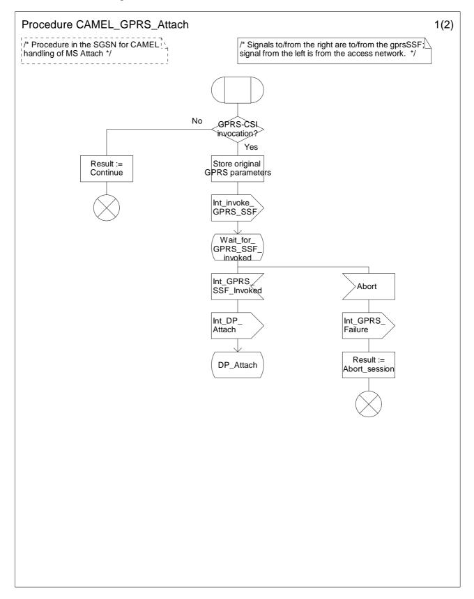
Figure 6.8-1: Procedure CAMEL\_GPRS\_Attach (sheet 1)
