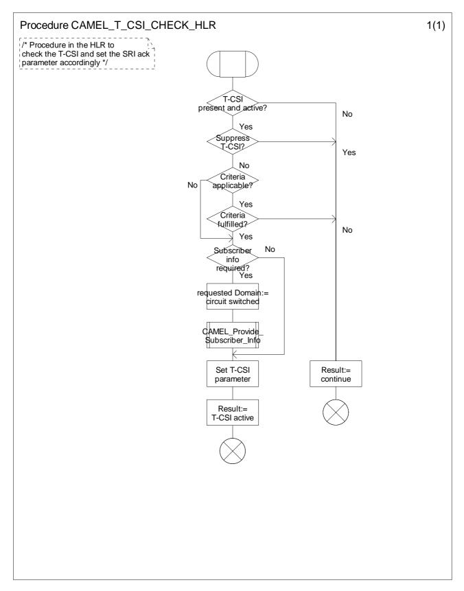
Figure 4.62-1: Procedure CAMEL\_T\_CSI\_CHECK\_HLR (sheet 1)
