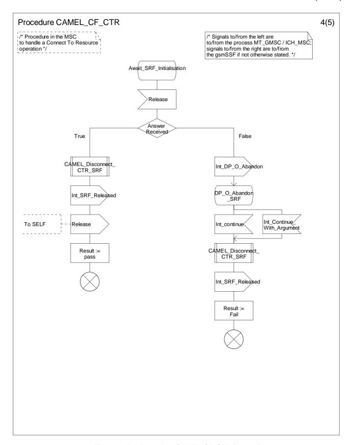
Figure 4.85-4: Procedure CAMEL\_CF\_CTR (sheet 4)
