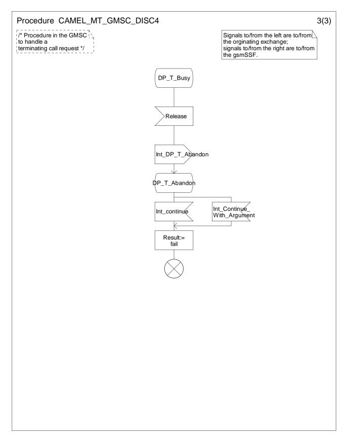
Figure 4.48-3: Procedure CAMEL\_MT\_GMSC\_DISC4 (sheet 3)
