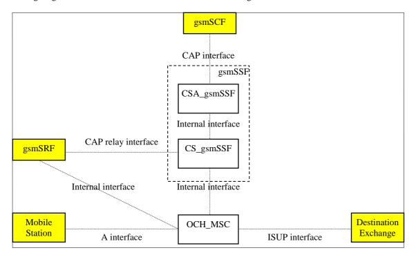
Figure 4.9-1: Outgoing case (gsmSSF relay)
