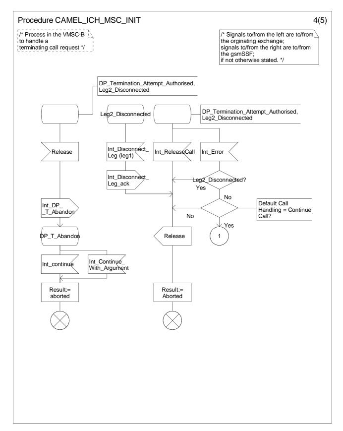
Figure 4.69-4: Procedure CAMEL\_ICH\_MSC\_INIT (sheet 4)
