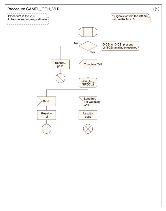
Figure 4.39-1: Procedure CAMEL\_OCH\_VLR (sheet 1)
