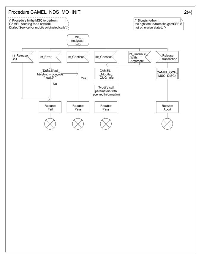
Figure 4.13-2: Procedure CAMEL\_NDS\_MO\_INIT (sheet 2)
