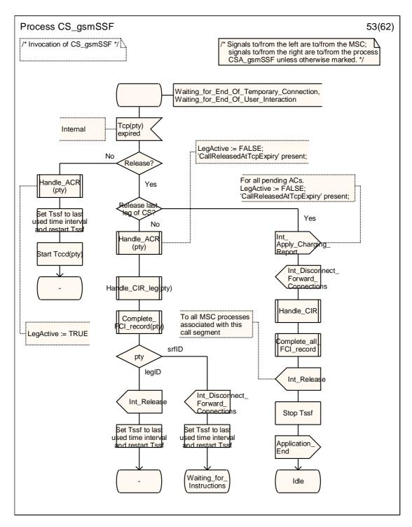
Figure 4.99-53: Process CS\_gsmSSF (sheet 53)
