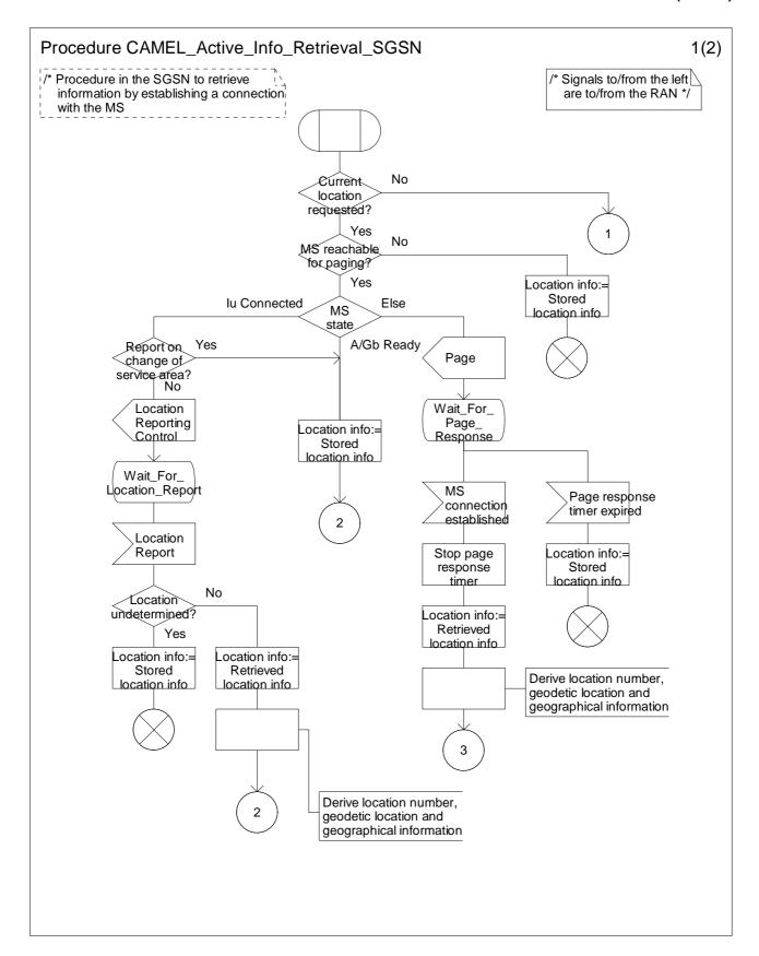
Figure 11.5-1: Procedure CAMEL\_Active\_Info\_Retrieval\_SGSN (sheet 1)
