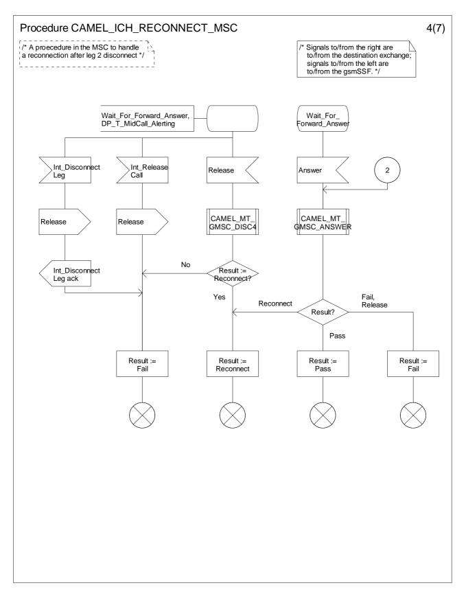
Figure 4.74-4: Procedure CAMEL\_ICH\_RECONNECT\_MSC (sheet 4)
