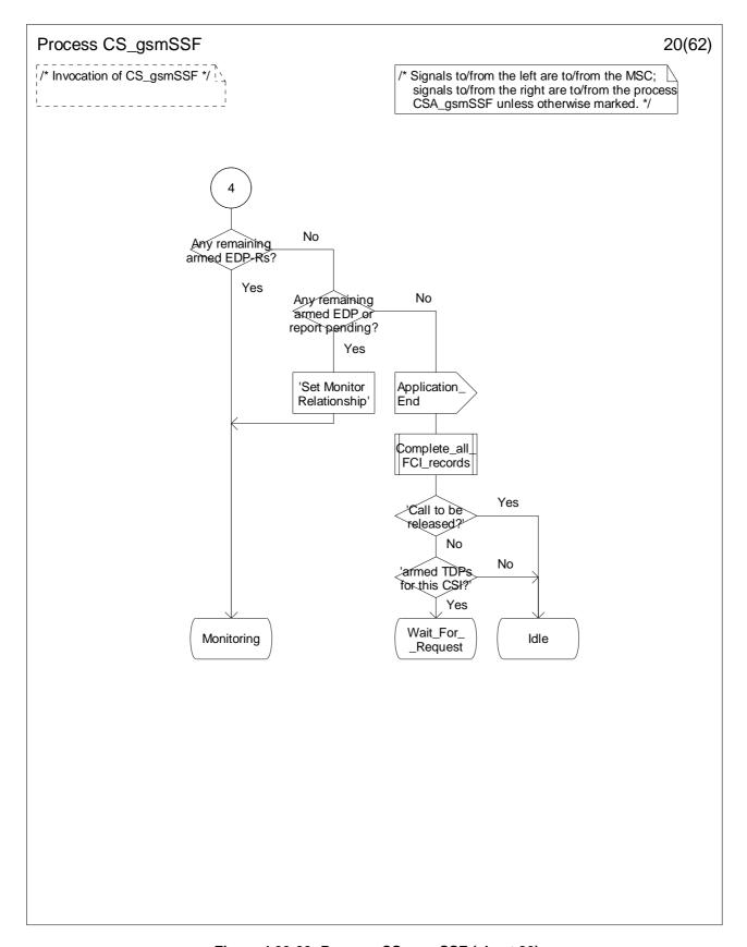
Figure 4.99-20: Process CS\_gsmSSF (sheet 20)
