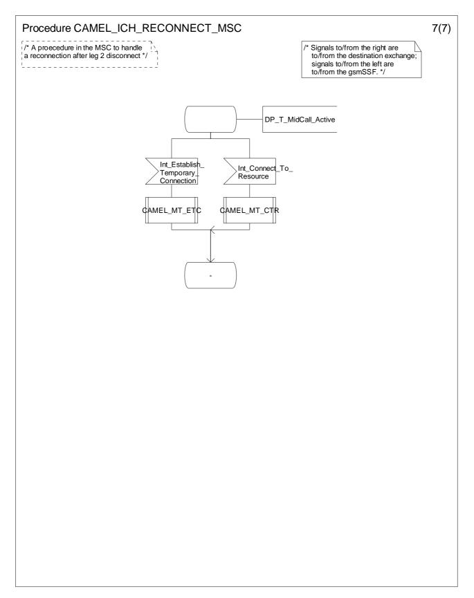
Figure 4.74-7: Procedure CAMEL\_ICH\_RECONNECT\_MSC (sheet 7)
