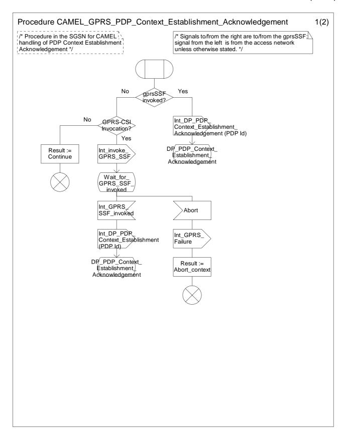
Figure 6.13-1: Procedure CAMEL\_GPRS\_PDP\_Context\_Establishment\_Acknowledgement (sheet 1)
