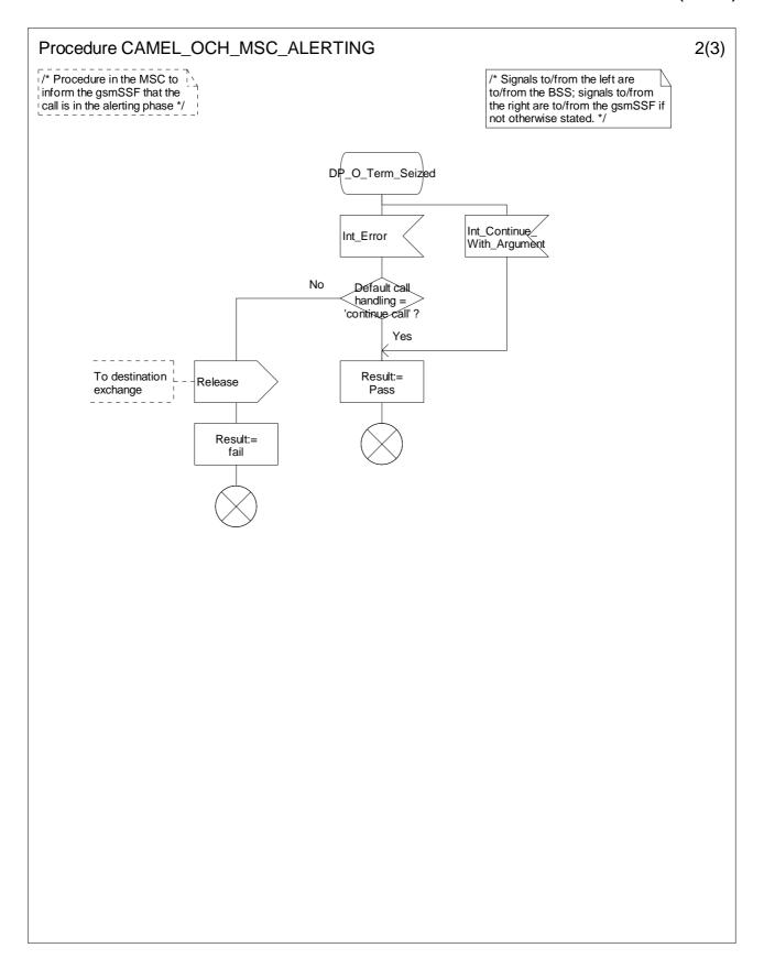
Figure 4.14-2: Procedure CAMEL\_OCH\_MSC\_ALERTING (sheet 2)
