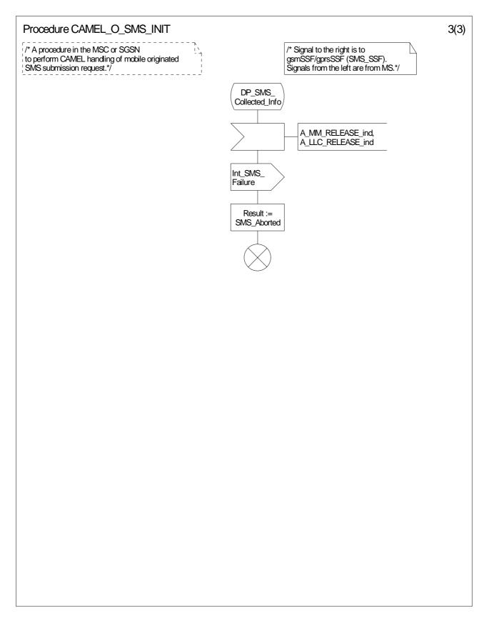
Figure 7.5-3: Procedure CAMEL\_O\_SMS\_INIT (sheet 3)
