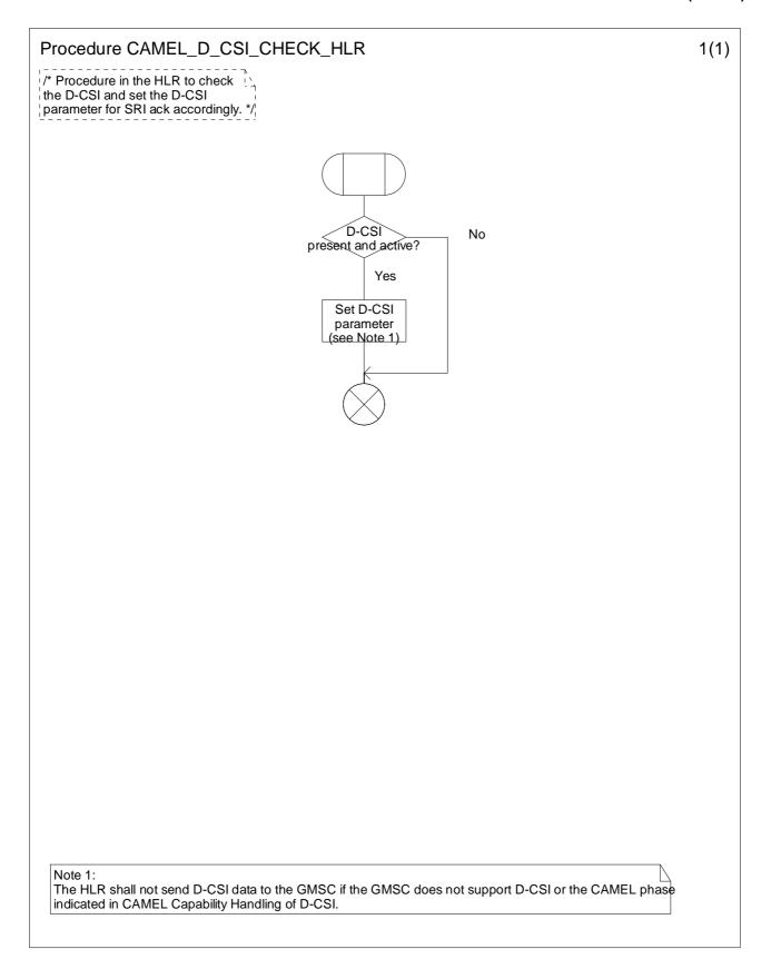
Figure 4.61-1: Procedure CAMEL\_D\_CSI\_CHECK\_HLR (sheet 1)
