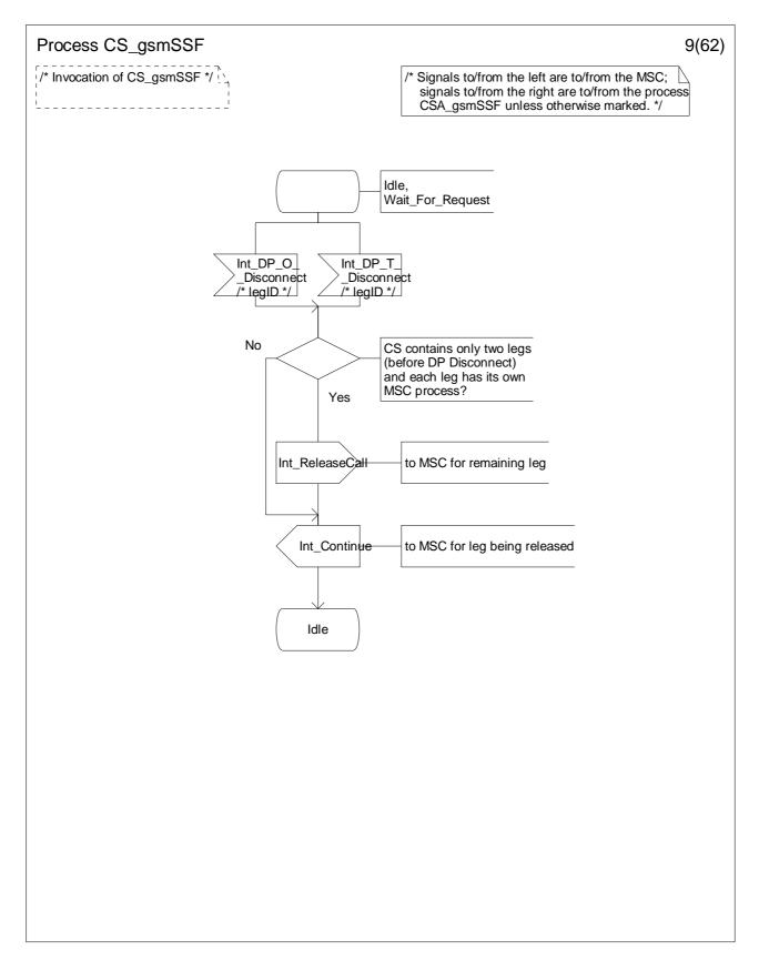
Figure 4.99-9: Process CS\_gsmSSF (sheet 9)
