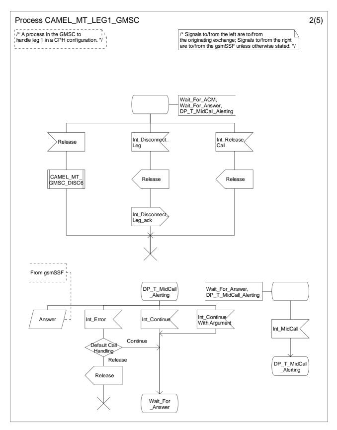
Figure 4.55-2: Process CAMEL\_MT\_LEG1\_GMSC (sheet 2)
