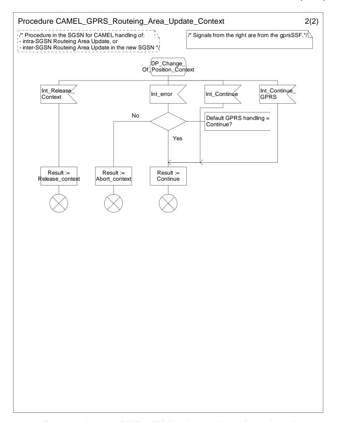
Figure 6.11-2: Procedure CAMEL\_GPRS\_Routeing\_Area\_Update\_Context (sheet 2)
