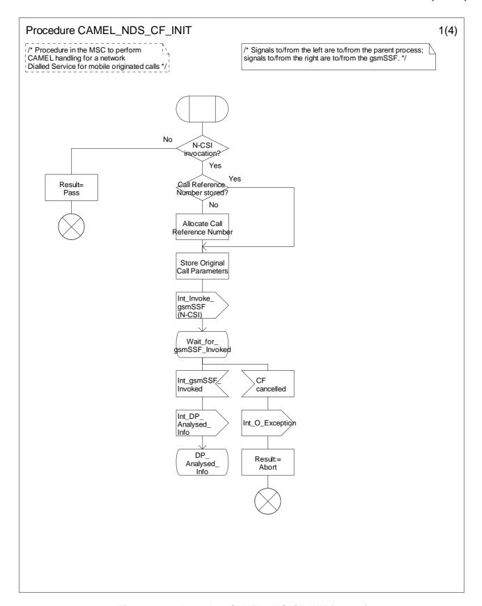
Figure 4.81-1: Procedure CAMEL\_NDS\_CF\_INIT (sheet 1)
