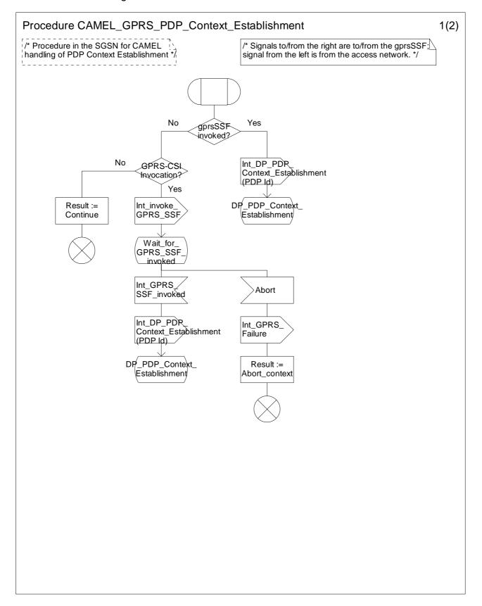
Figure 6.12-1: Procedure CAMEL\_GPRS\_PDP\_Context\_Establishment (sheet 1)
