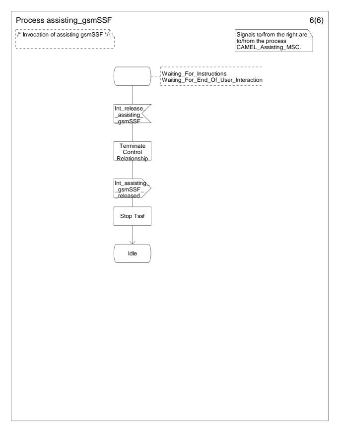
Figure 4.118-6: Process Assisting\_gsmSSF (sheet 6)
