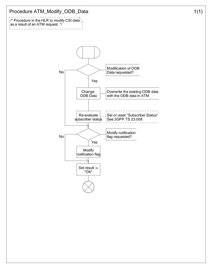
Figure 10.8-1: Procedure ATM\_Modify\_ODB\_Data (sheet 1)
