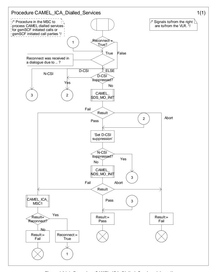
Figure 4.94-1: Procedure CAMEL\_ICA\_Dialled\_Services (sheet 1)
