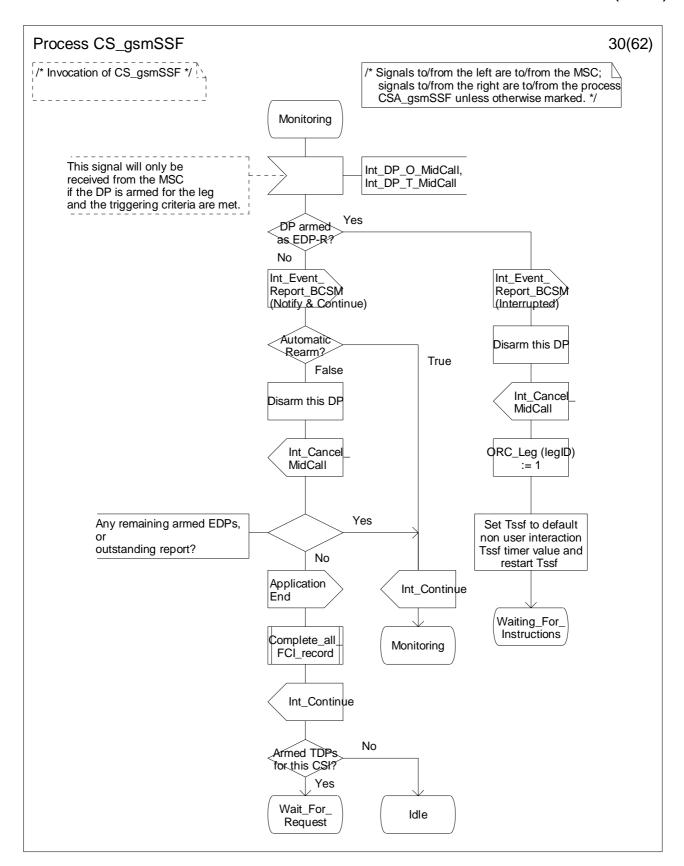
Figure 4.99-30: Process CS\_gsmSSF (sheet 30)
