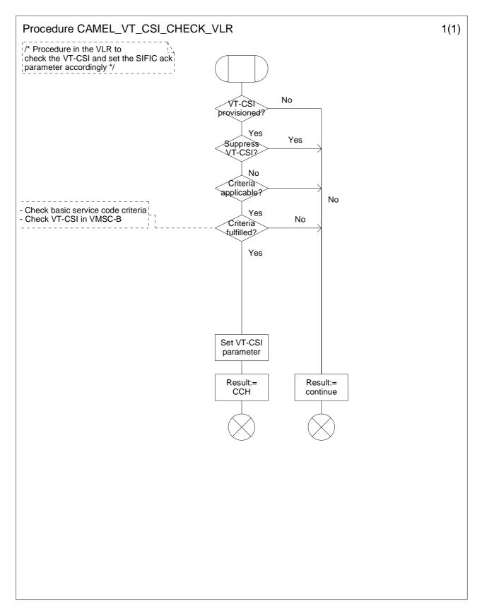
Figure 4.68-1: Procedure CAMEL\_VT\_CSI\_Check\_VLR (sheet 1)
