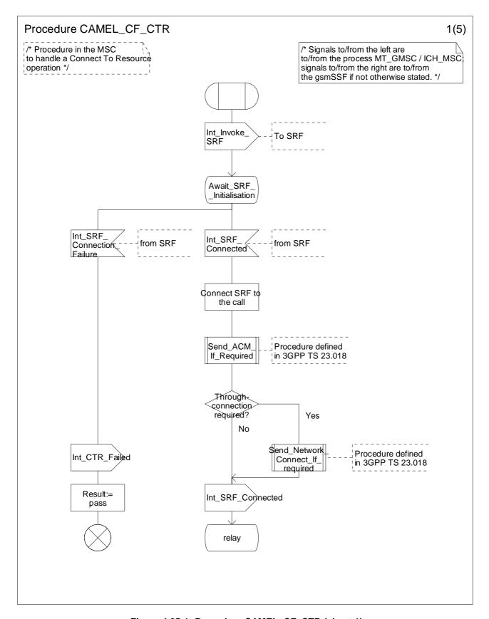
Figure 4.85-1: Procedure CAMEL\_CF\_CTR (sheet 1)
