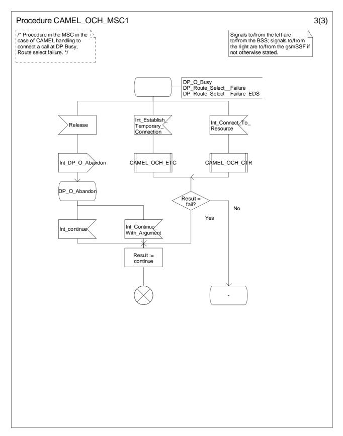
Figure 4.16-3: Procedure CAMEL\_OCH\_MSC1 (sheet 3)
