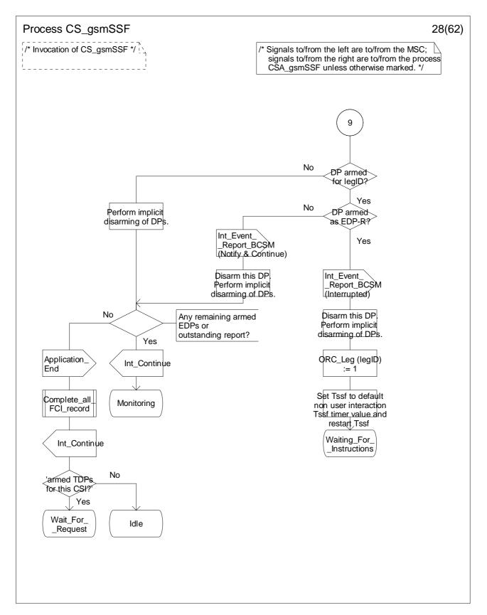
Figure 4.99-28: Process CS\_gsmSSF (sheet 28)
