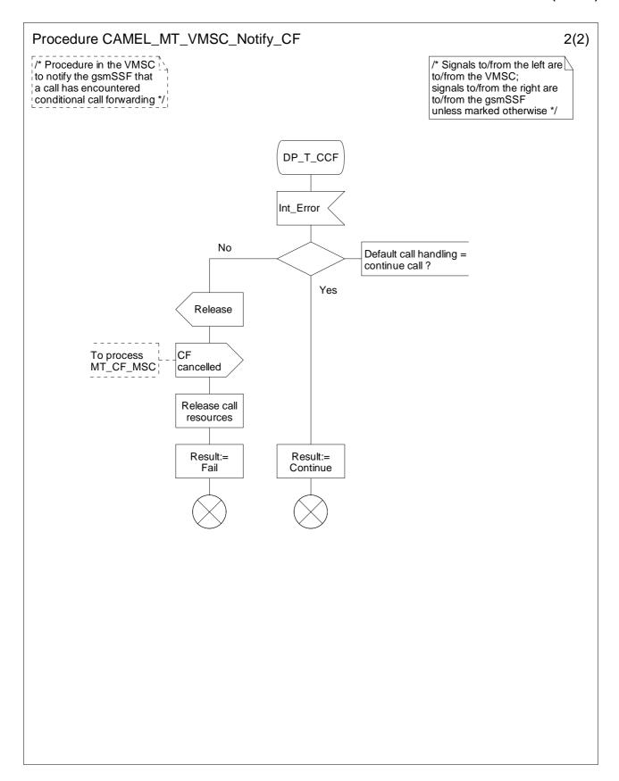
Figure 4.70-2: Procedure CAMEL\_MT\_VMSC\_Notify\_CF (sheet 2)
