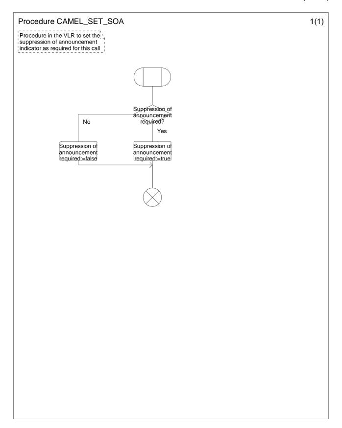
Figure 4.64-1: Procedure CAMEL\_SET\_SOA (sheet 1)
