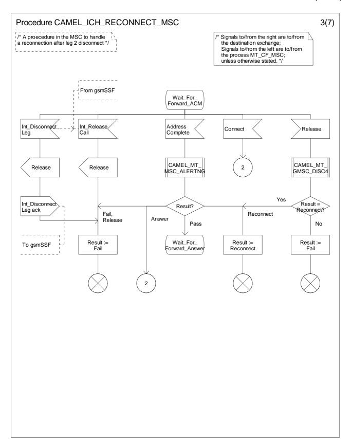
Figure 4.74-3: Procedure CAMEL\_ICH\_RECONNECT\_MSC (sheet 3)
