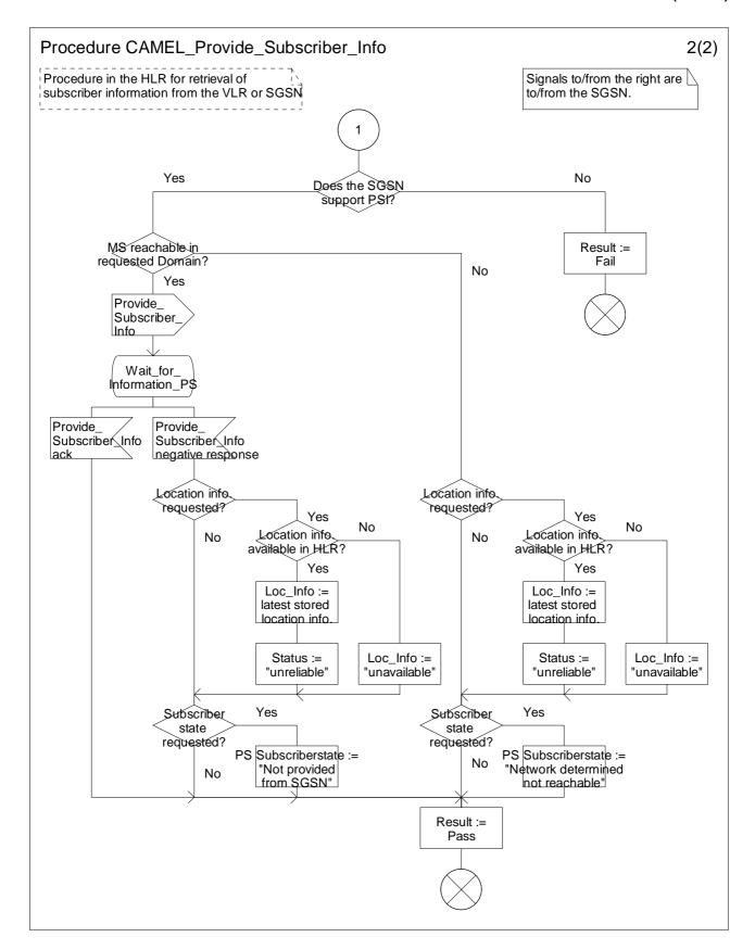
Figure 4.119-2: Procedure CAMEL\_Provide\_Subscriber\_Info (sheet 2)
