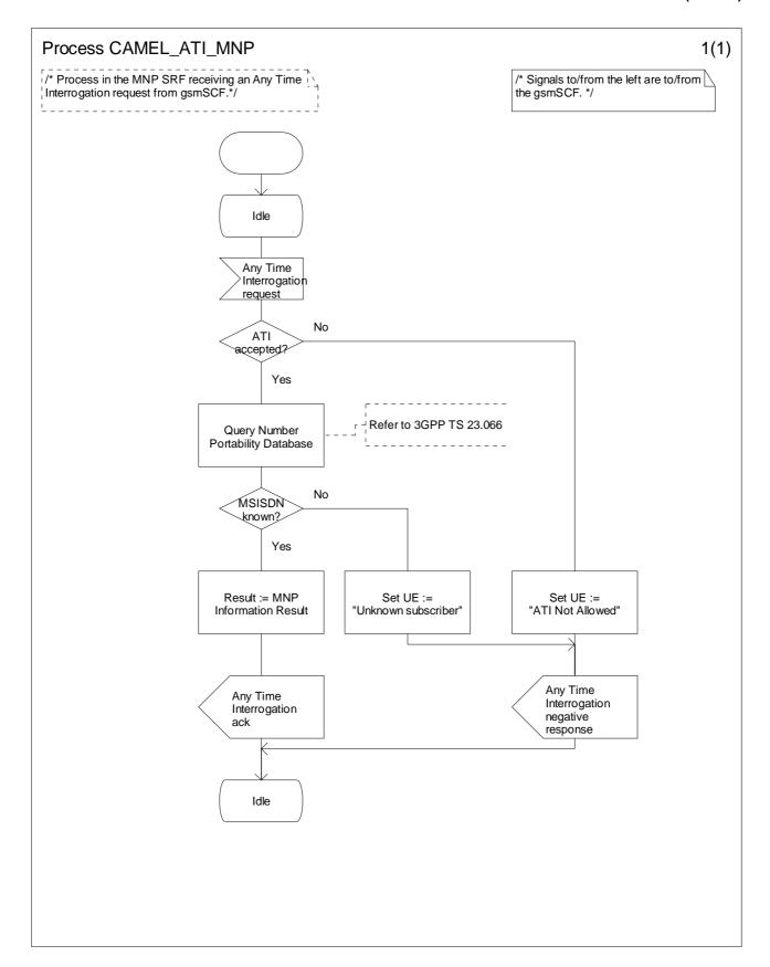
Figure 12.2-1: Process CAMEL\_ATI\_MNP (sheet 1)
