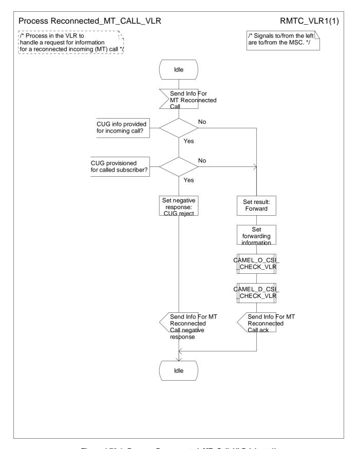
Figure 4.76-1: Process Reconnected\_MT\_Call\_VLR (sheet 1)
