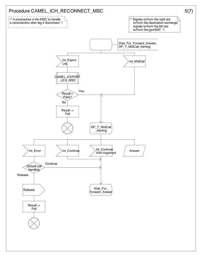
Figure 4.74-5: Procedure CAMEL\_ICH\_RECONNECT\_MSC (sheet 5)
