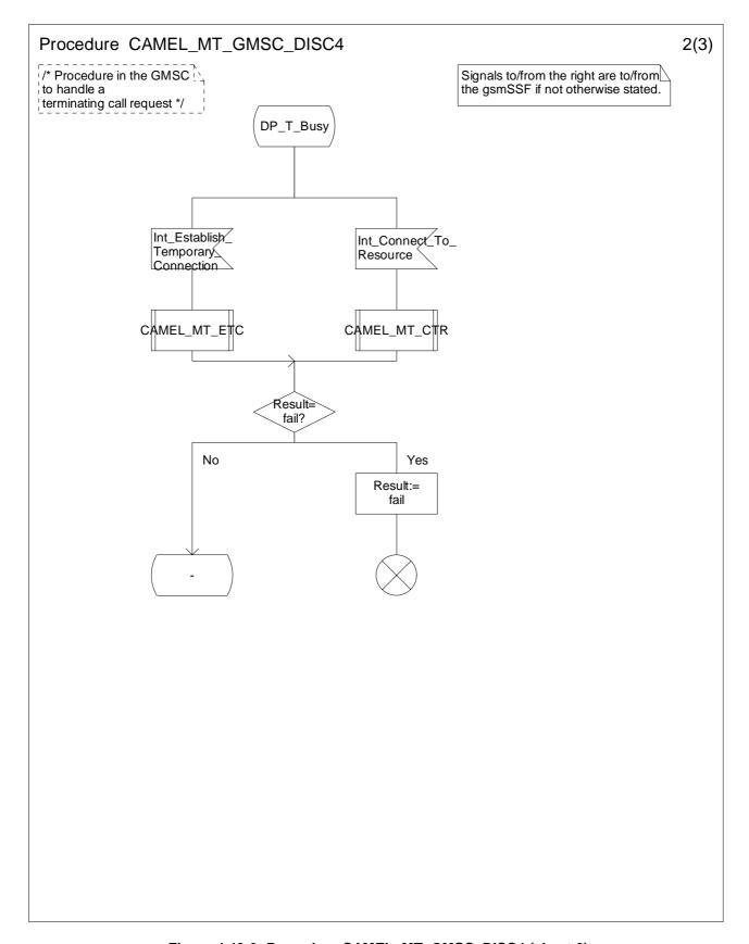
Figure 4.48-2: Procedure CAMEL\_MT\_GMSC\_DISC4 (sheet 2)
