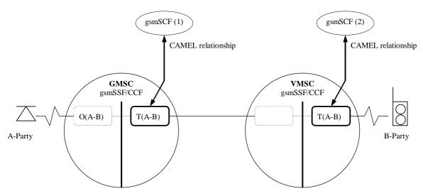
Figure 4.6: BCSM Scenario for Mobile Terminated Calls at the GMSC or VMSC
