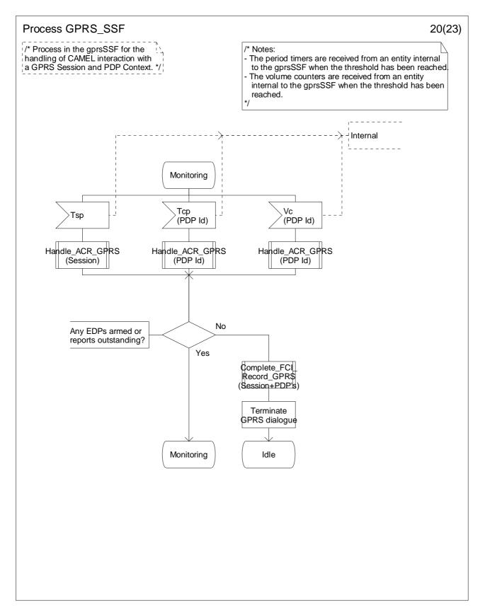
Figure 6.17-20: Process GPRS\_SSF (sheet 20)
