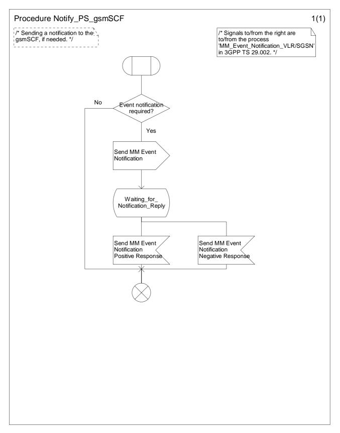
Figure 9.7-1: Procedure Notify\_PS\_gsmSCF (sheet 1)
