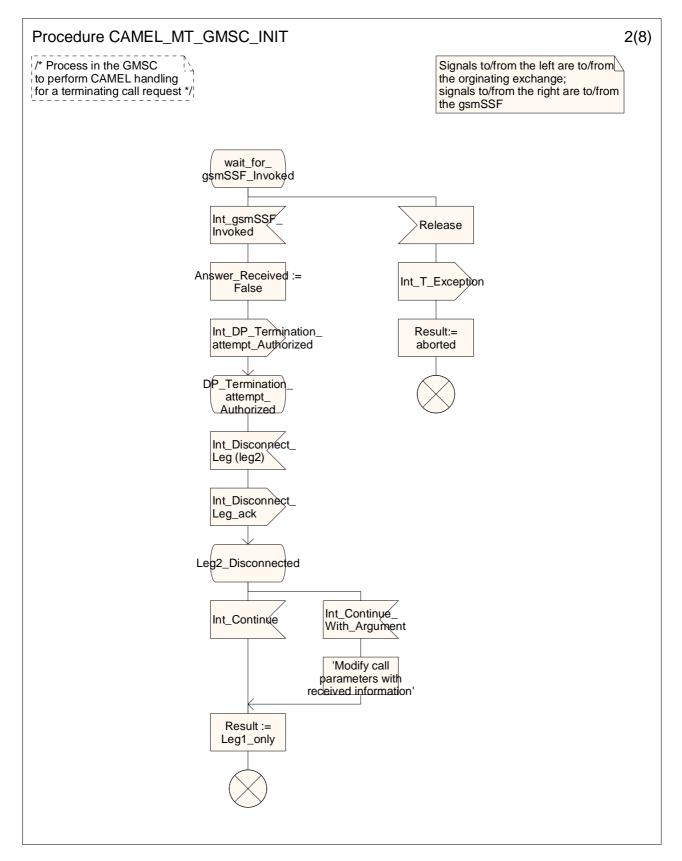
Figure 4.42-2: Procedure CAMEL\_MT\_GMSC\_INIT (sheet 2)
