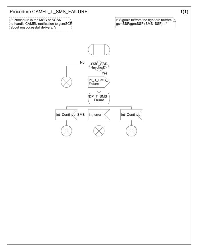
Figure 7.11-1: Procedure CAMEL\_T\_SMS\_FAILURE (sheet 1)
