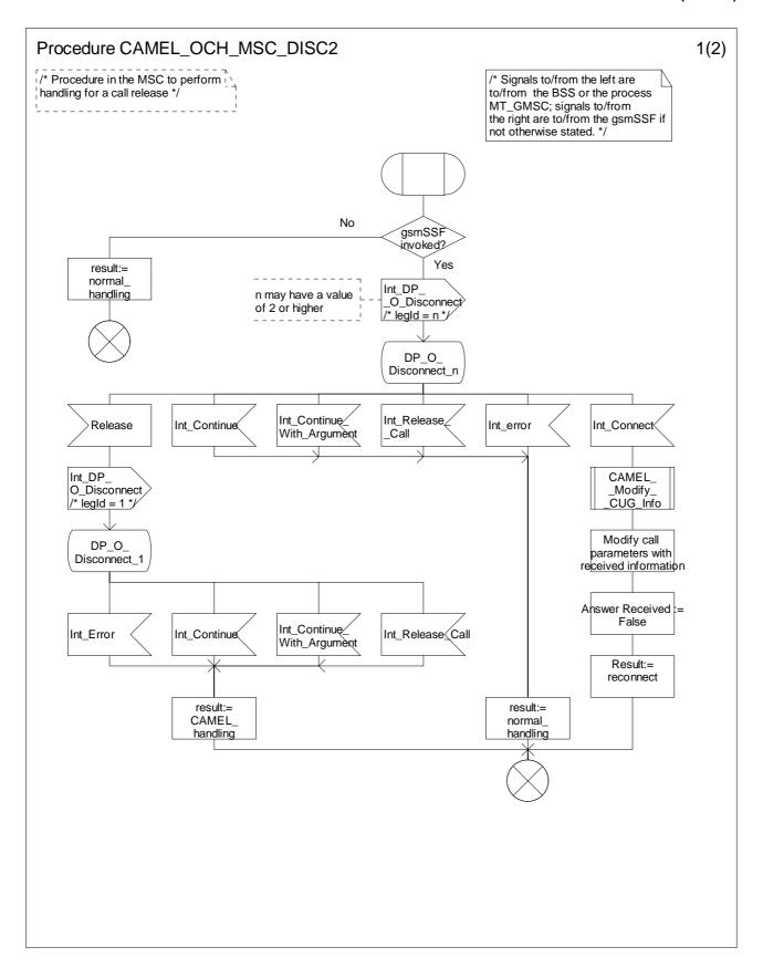
Figure 4.19-1: Procedure CAMEL\_OCH\_MSC\_DISC2 (sheet 1)
