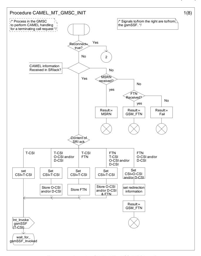
Figure 4.42-1: Procedure CAMEL\_MT\_GMSC\_INIT (sheet 1)
