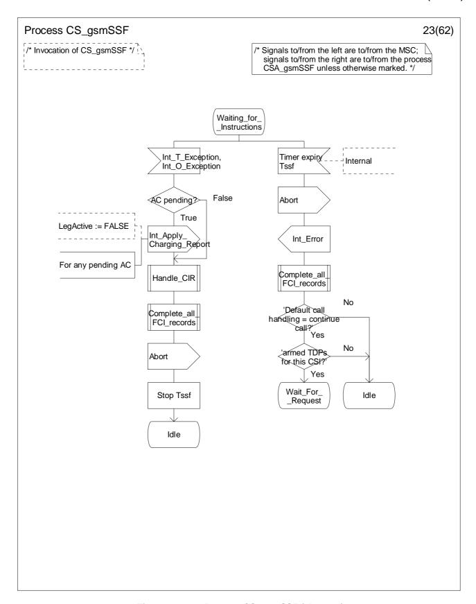
Figure 4.99-23: Process CS\_gsmSSF (sheet 23)
