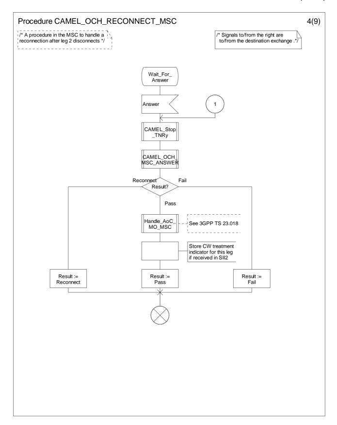
Figure 4.33-4: Procedure CAMEL\_OCH\_RECONNECT\_MSC (sheet 4)
