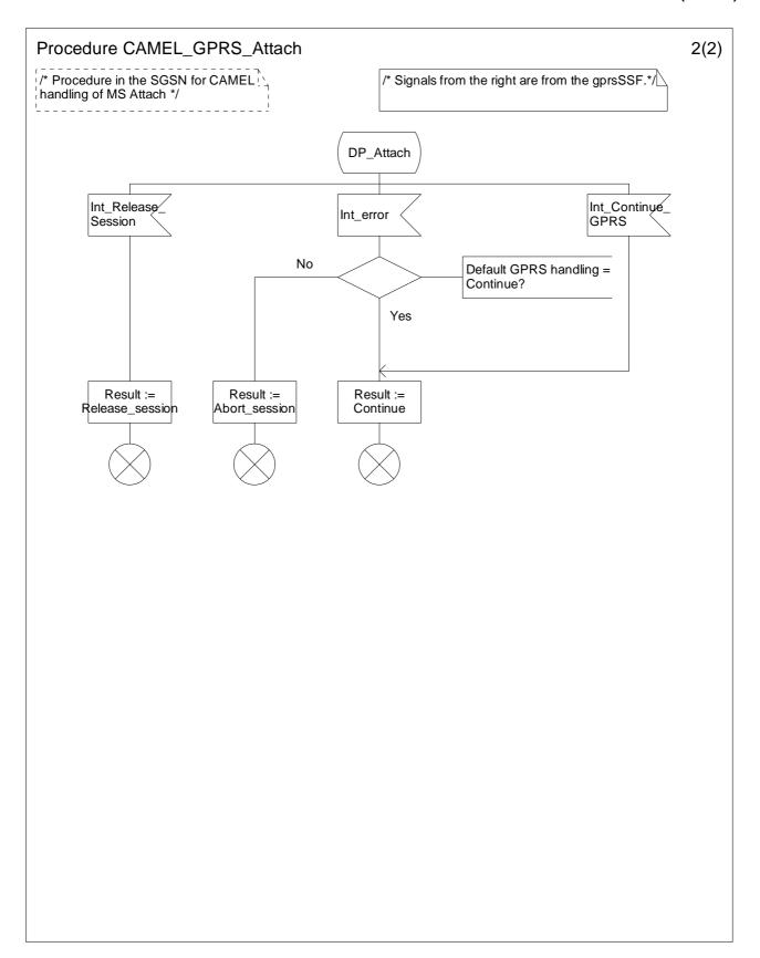
Figure 6.8-2: Procedure CAMEL\_GPRS\_Attach (sheet 2)
