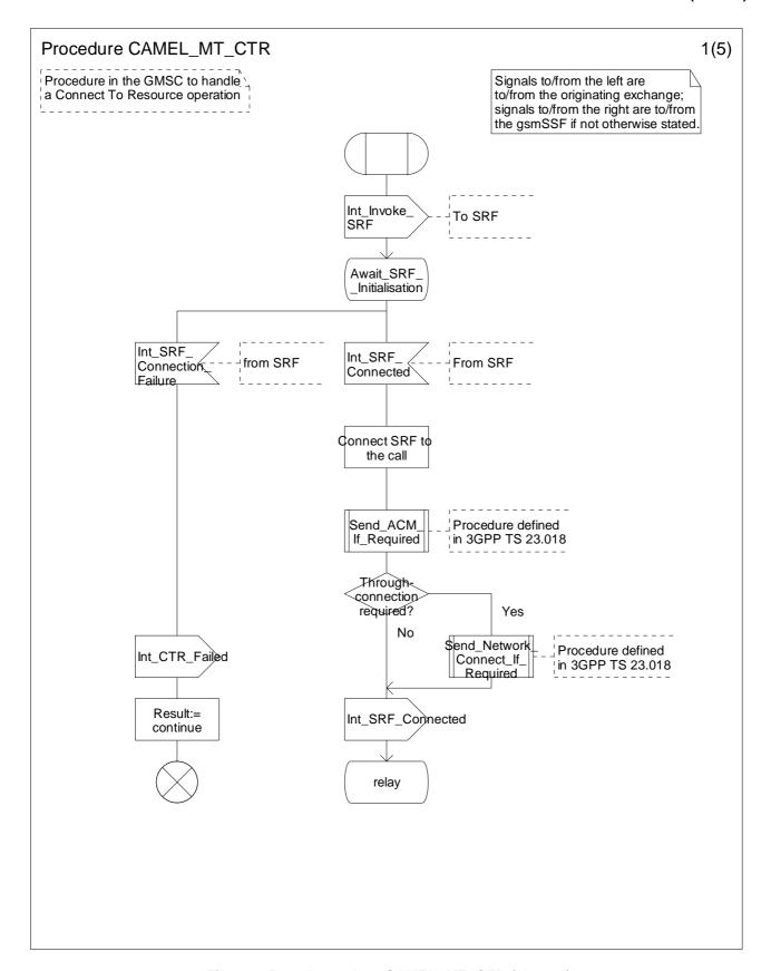
Figure 4.52-1: Procedure CAMEL\_MT\_CTR (sheet 1)
