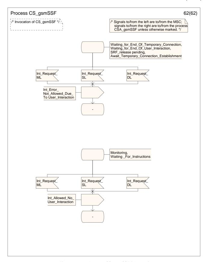
Figure 4.99-62: Process CS\_gsmSSF (sheet 62)
