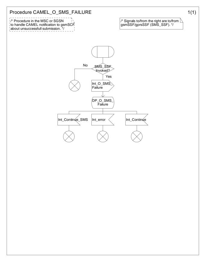
Figure 7.7-1: Procedure CAMEL\_O\_SMS\_FAILURE (sheet 1)
