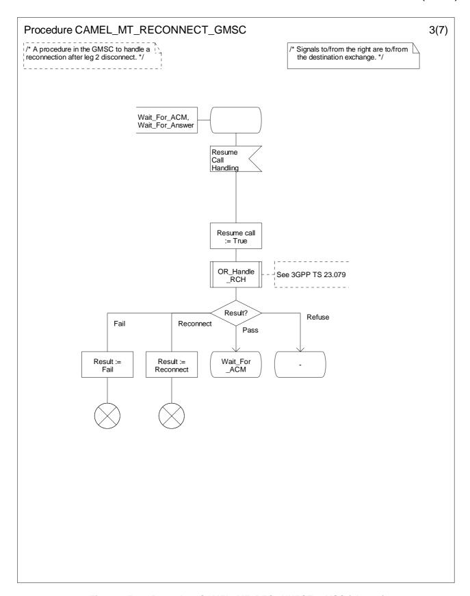
Figure 4.56-3: Procedure CAMEL\_MT\_RECONNECT\_GMSC (sheet 3)
