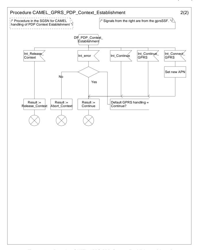
Figure 6.12-2: Procedure CAMEL\_GPRS\_PDP\_Context\_Establishment (sheet 2)
