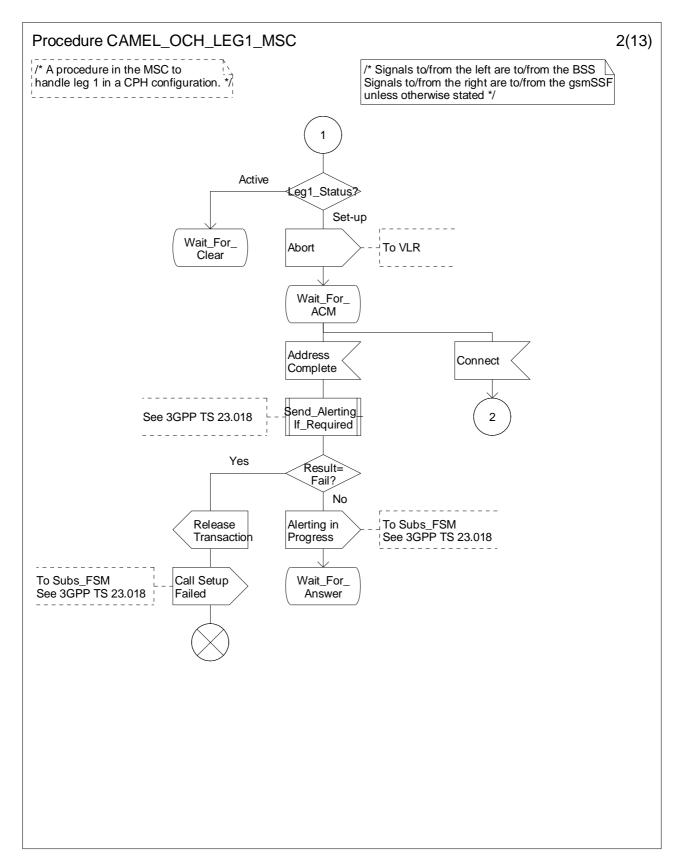
Figure 4.30-2: Procedure CAMEL\_OCH\_LEG1\_MSC (sheet 2)
