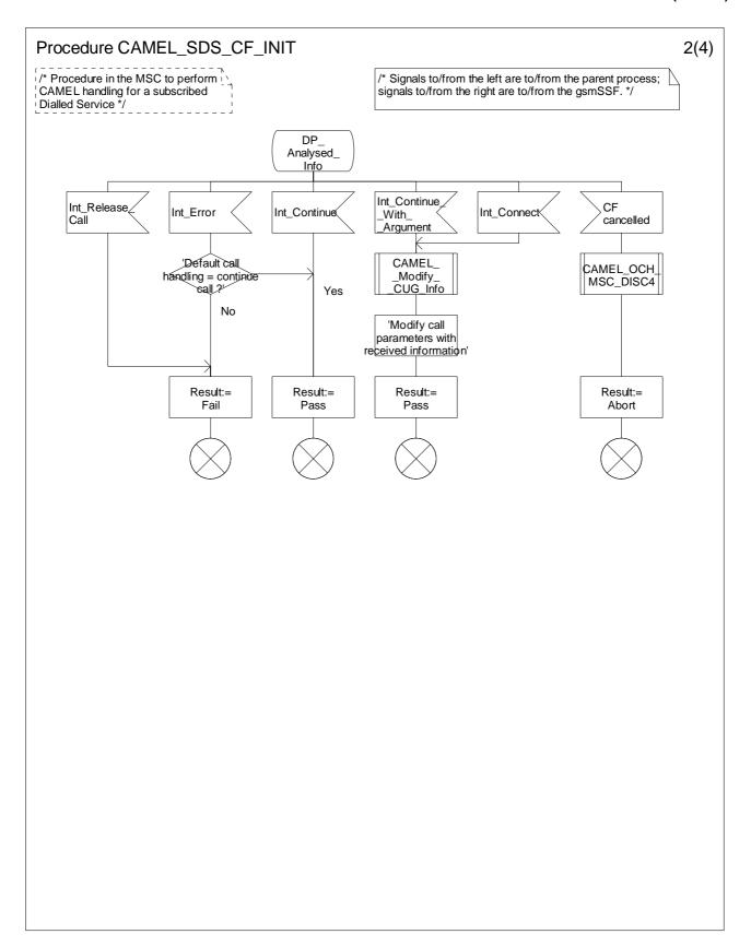
Figure 4.80-2: Procedure CAMEL\_SDS\_CF\_INIT (sheet 2)
