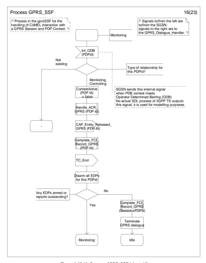
Figure 6.17-16: Process GPRS\_SSF (sheet 16)
