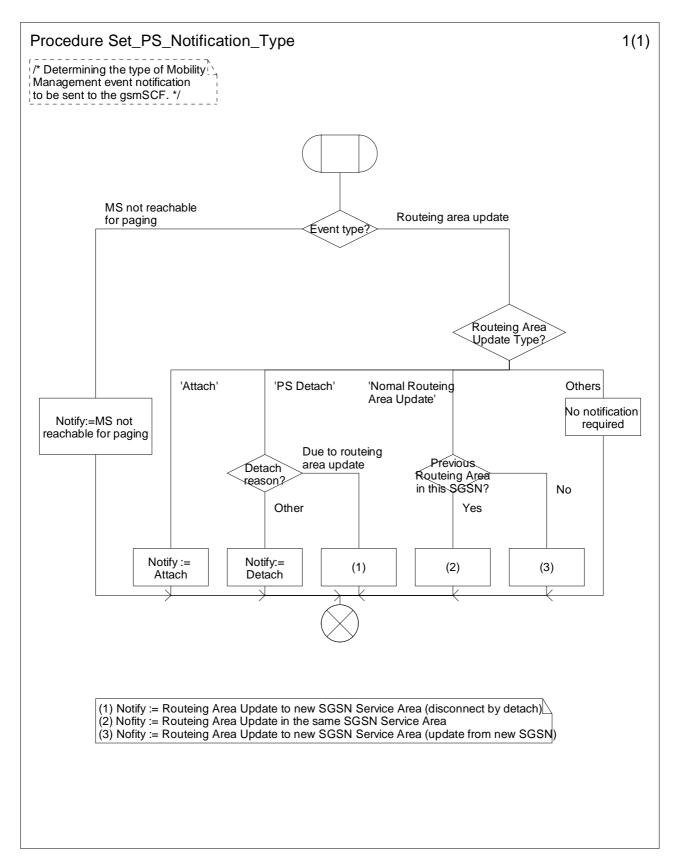
Figure 9.6-1: Procedure Set\_PS\_Notification\_Type (sheet 1)
