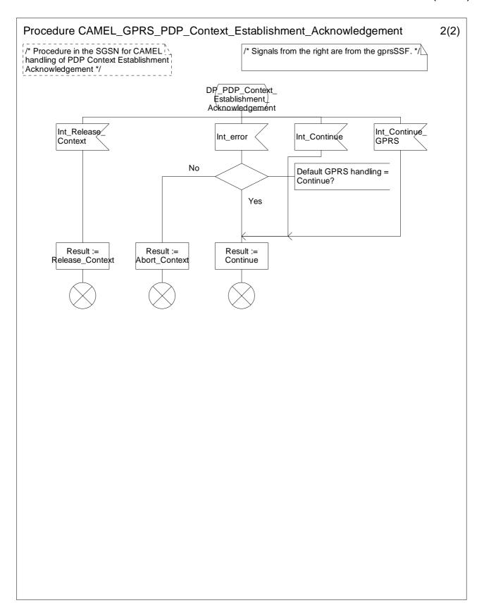
Figure 6.13-2: Procedure CAMEL\_GPRS\_PDP\_Context\_Establishment\_Acknowledgement (sheet 2)
