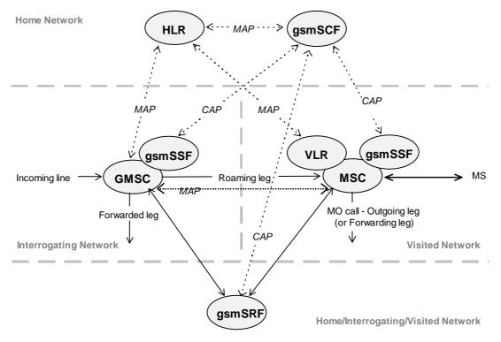
Figure 4.1: Functional architecture for support of CAMEL
