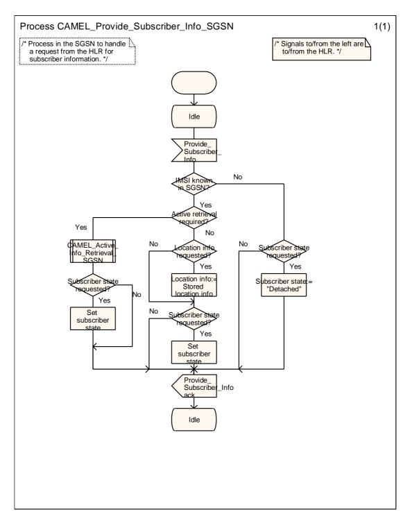
Figure 11.4-1: Process CAMEL\_Provide\_Subscriber\_Info\_SGSN (sheet 1)
