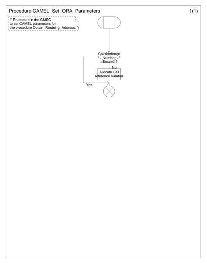
Figure 4.41-1: Procedure CAMEL\_Set\_ORA\_Parameters (sheet 1)
