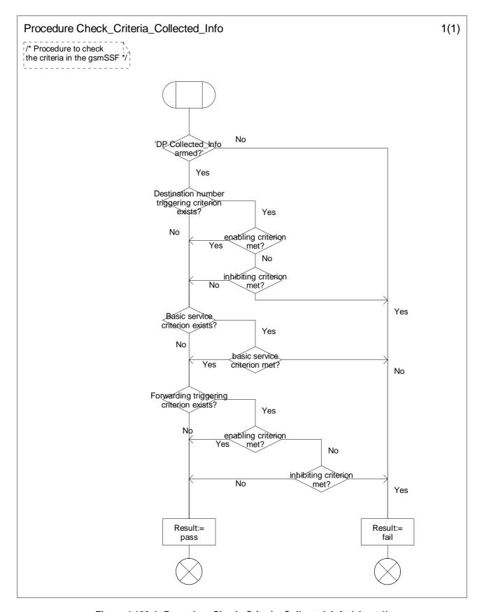
Figure 4.100-1: Procedure Check\_Criteria\_Collected\_Info (sheet 1)
