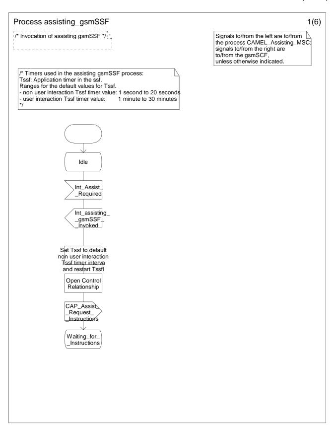
Figure 4.118-1: Process Assisting\_gsmSSF (sheet 1)
