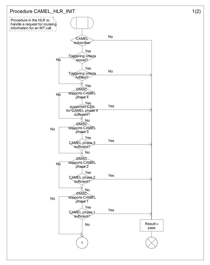
Figure 4.58-1: Procedure CAMEL\_HLR\_INIT (sheet 1)
