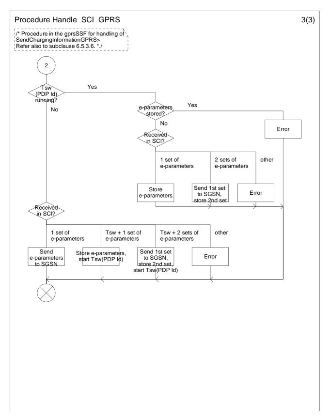
Figure 6.23-3: Procedure Handle\_SCI\_GPRS (sheet 3)
