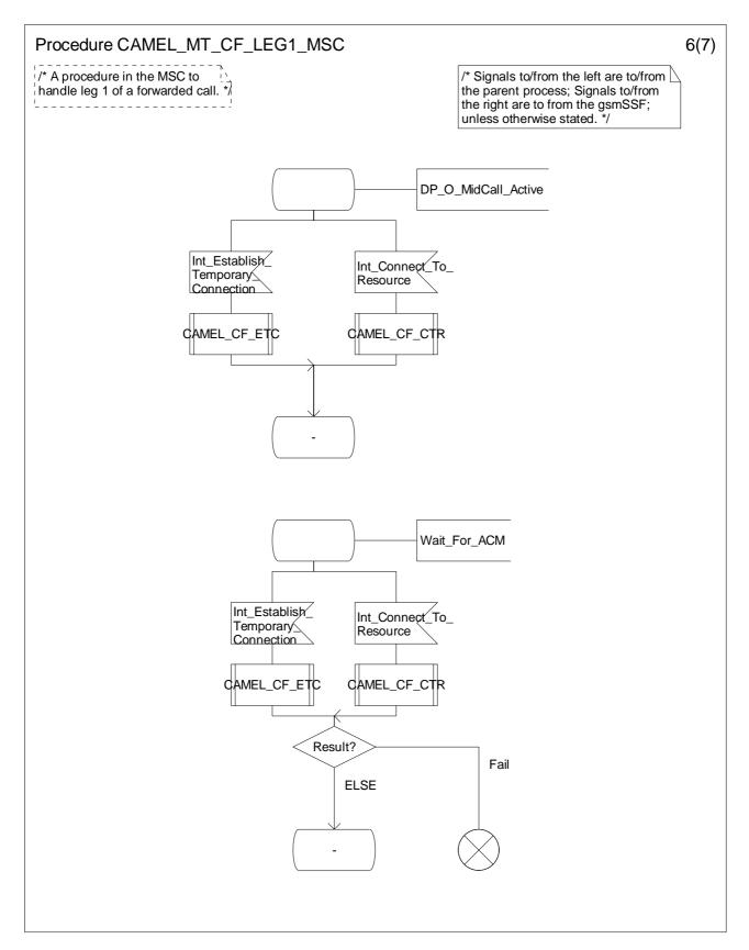
Figure 4.86-6: Procedure CAMEL\_MT\_CF\_LEG1\_MSC (sheet 6)
