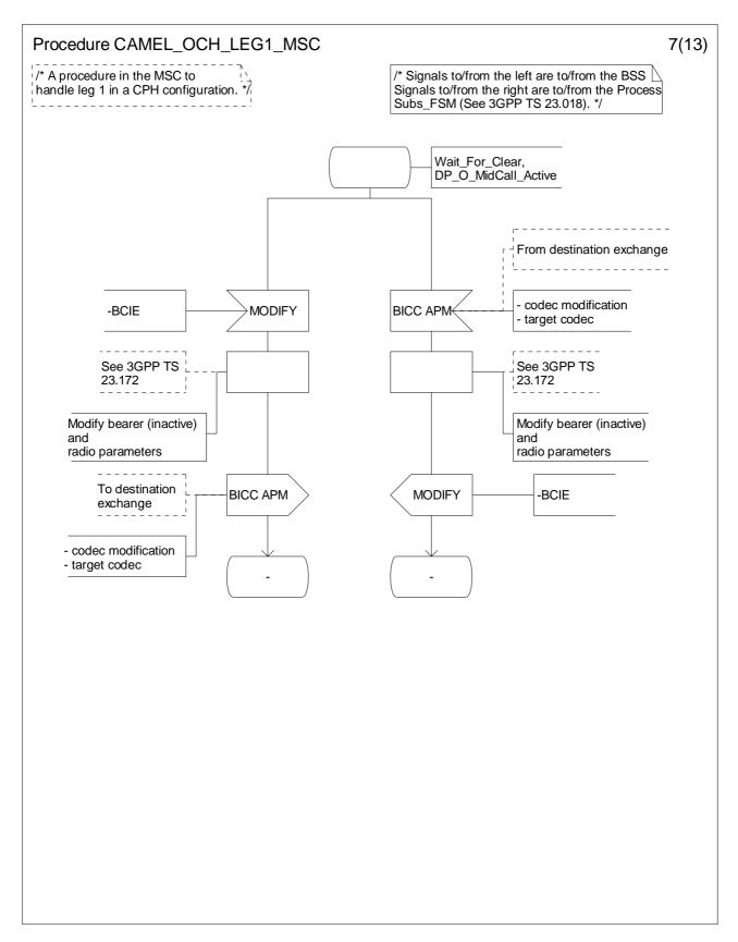
Figure 4.30-7: Procedure CAMEL\_OCH\_LEG1\_MSC (sheet 7)
