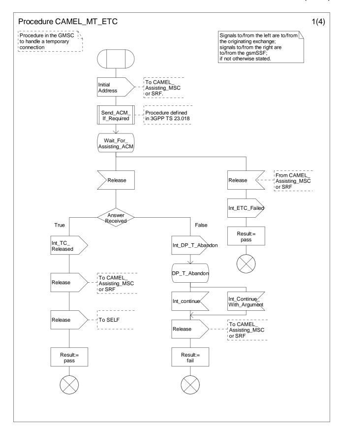
Figure 4.51-1: Procedure CAMEL\_MT\_ETC (sheet 1)
