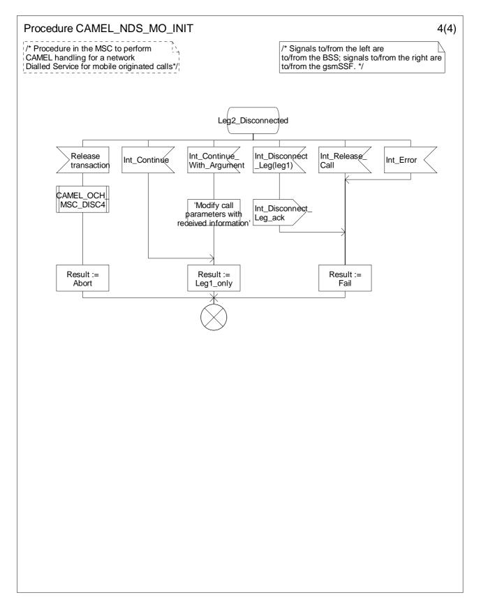
Figure 4.13-4: Procedure CAMEL\_NDS\_MO\_INIT (sheet 4)
