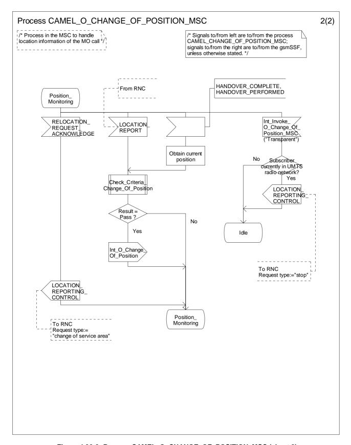
Figure 4.36-2: Process CAMEL\_O\_CHANGE\_OF\_POSITION\_MSC (sheet 2)
