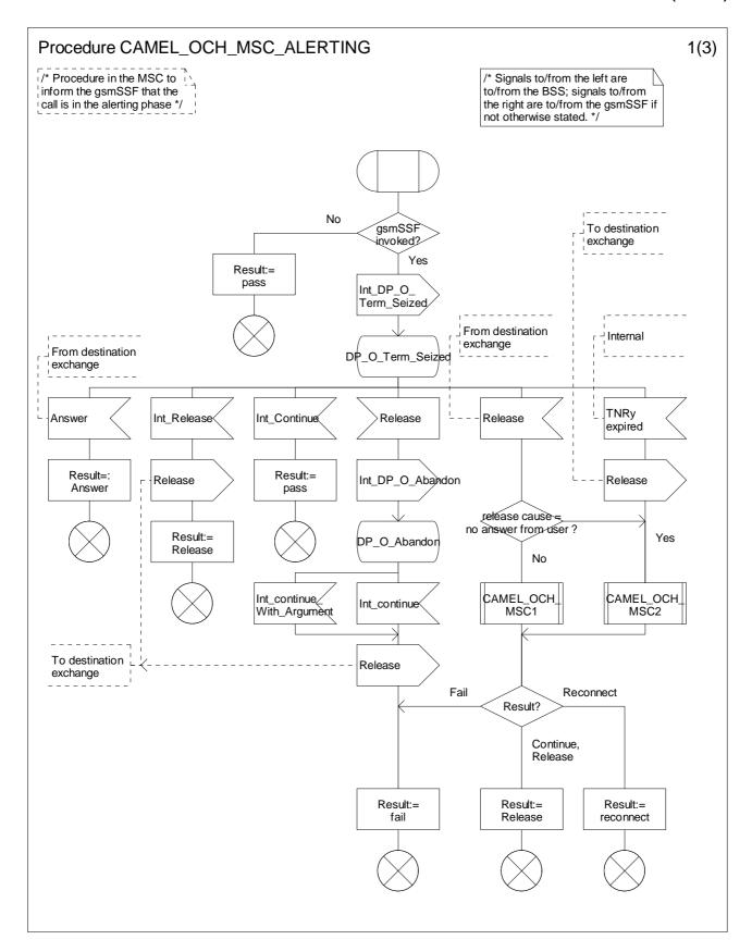
Figure 4.14-1: Procedure CAMEL\_OCH\_MSC\_ALERTING (sheet 1)
