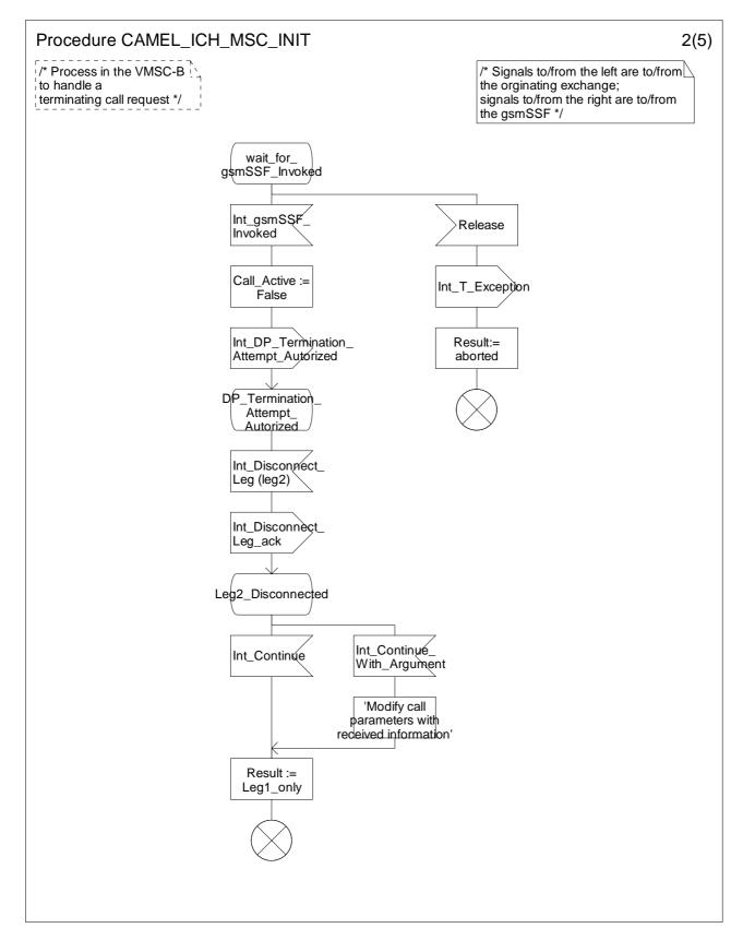
Figure 4.69-2: Procedure CAMEL\_ICH\_MSC\_INIT (sheet 2)
