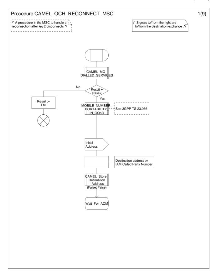
Figure 4.33-1: Procedure CAMEL\_OCH\_RECONNECT\_MSC (sheet 1)
