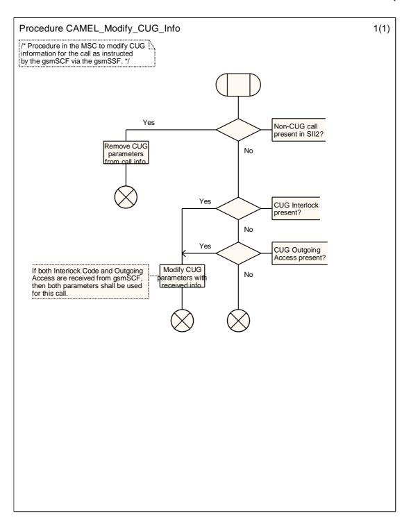
Figure 4.28-1: Procedure CAMEL\_Modify\_CUG\_Info (sheet 1)
