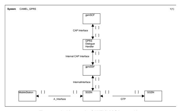
Figure 6.7: Architecture for CAMEL/GPRS interworking
