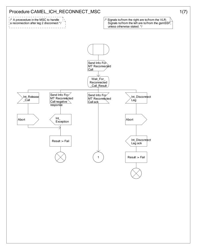
Figure 4.74-1: Procedure CAMEL\_ICH\_RECONNECT\_MSC (sheet 1)
