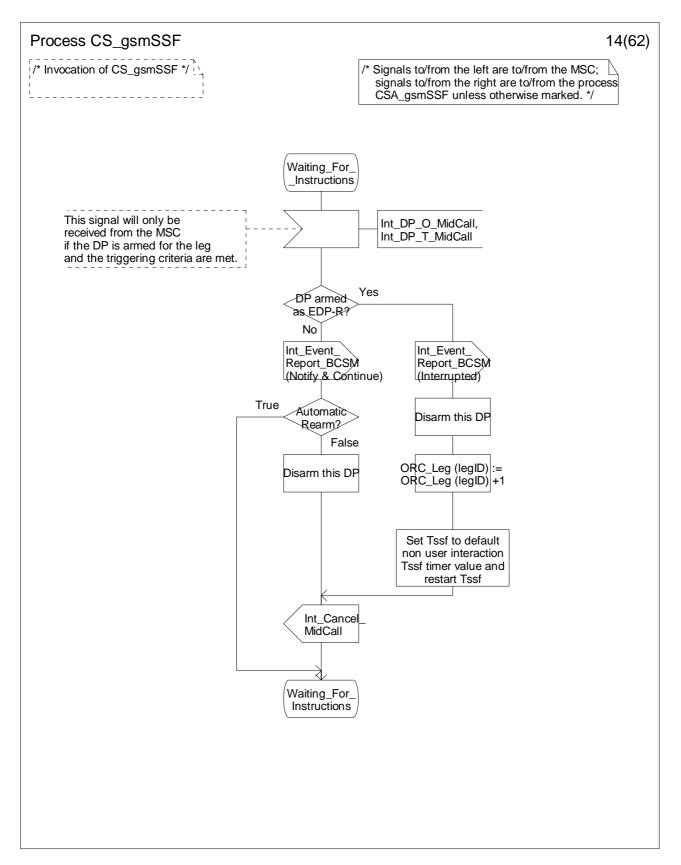
Figure 4.99-14: Process CS\_gsmSSF (sheet 14)
