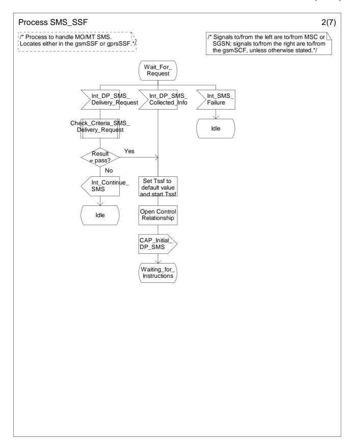
Figure 7.15-2: Process SMS\_SSF (sheet 2)
