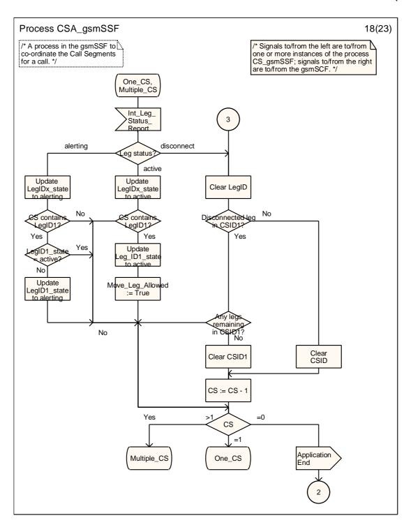
Figure 4.116-18: Process CSA\_gsmSSF (sheet 18)
