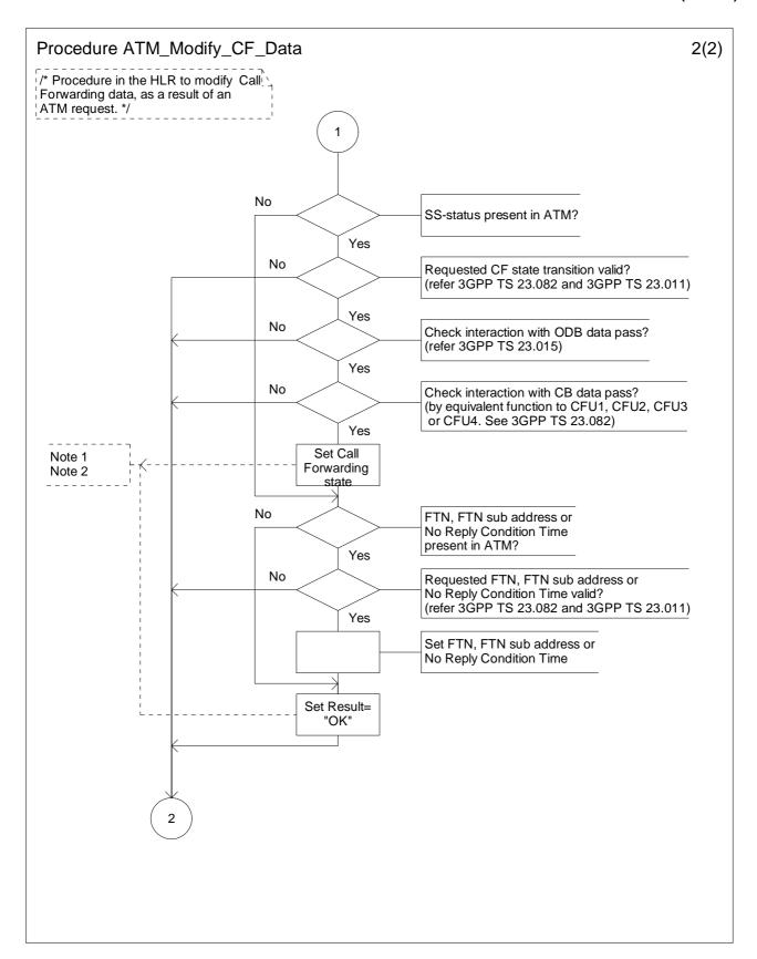
Figure 10.6-2: Procedure ATM\_Modify\_CF\_Data (sheet 2)
