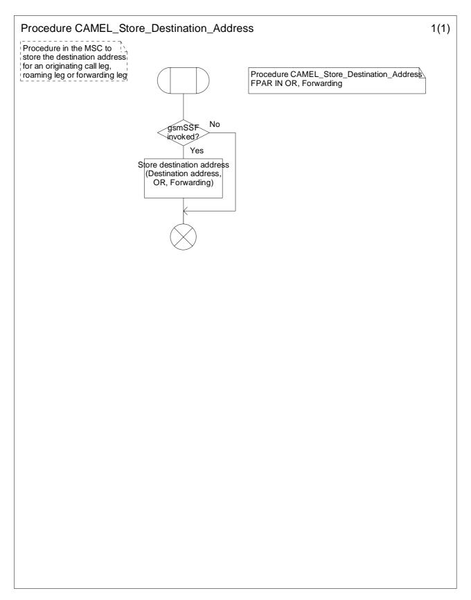
Figure 4.27-1: Procedure CAMEL\_Store\_Destination\_Address (sheet 1)
