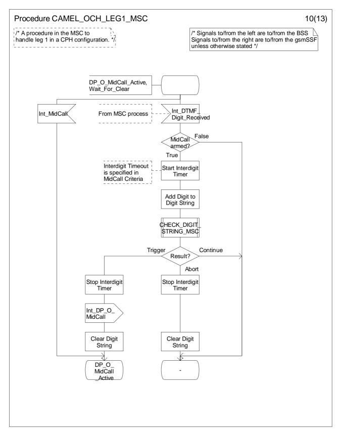
Figure 4.30-10: Procedure CAMEL\_OCH\_LEG1\_MSC (sheet 10)
