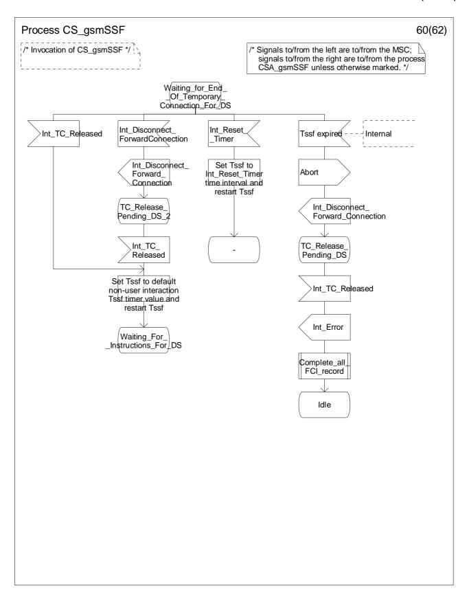
Figure 4.99-60: Process CS\_gsmSSF (sheet 60)
