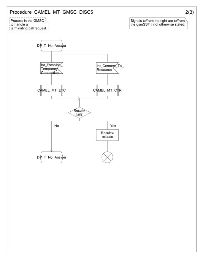
Figure 4.49-2: Procedure CAMEL\_MT\_GMSC\_DISC5 (sheet 2)
