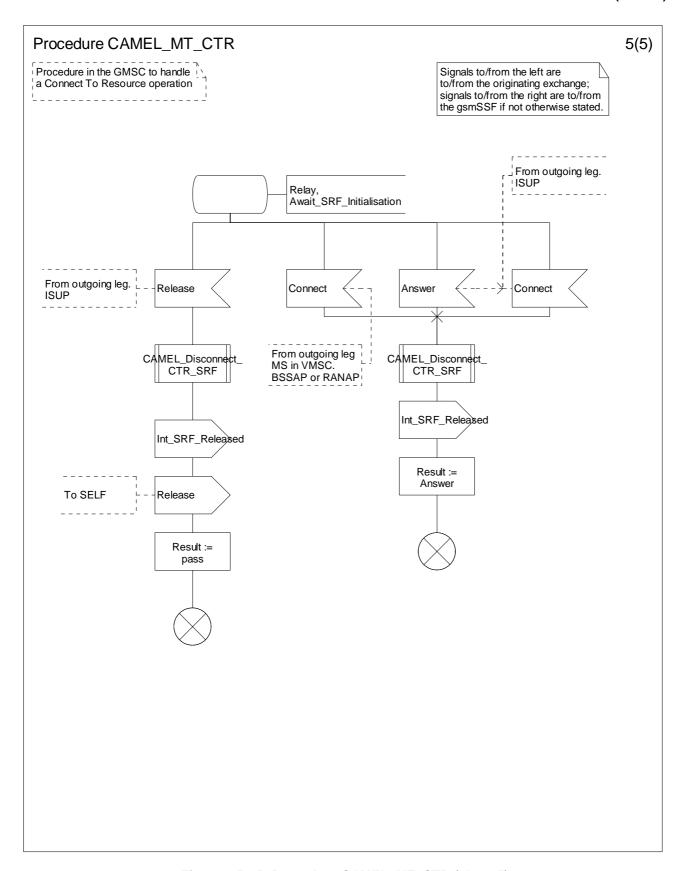
Figure 4.52-5: Procedure CAMEL\_MT\_CTR (sheet 5)
