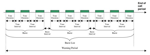
Figure 4.97: Representation of burst list
