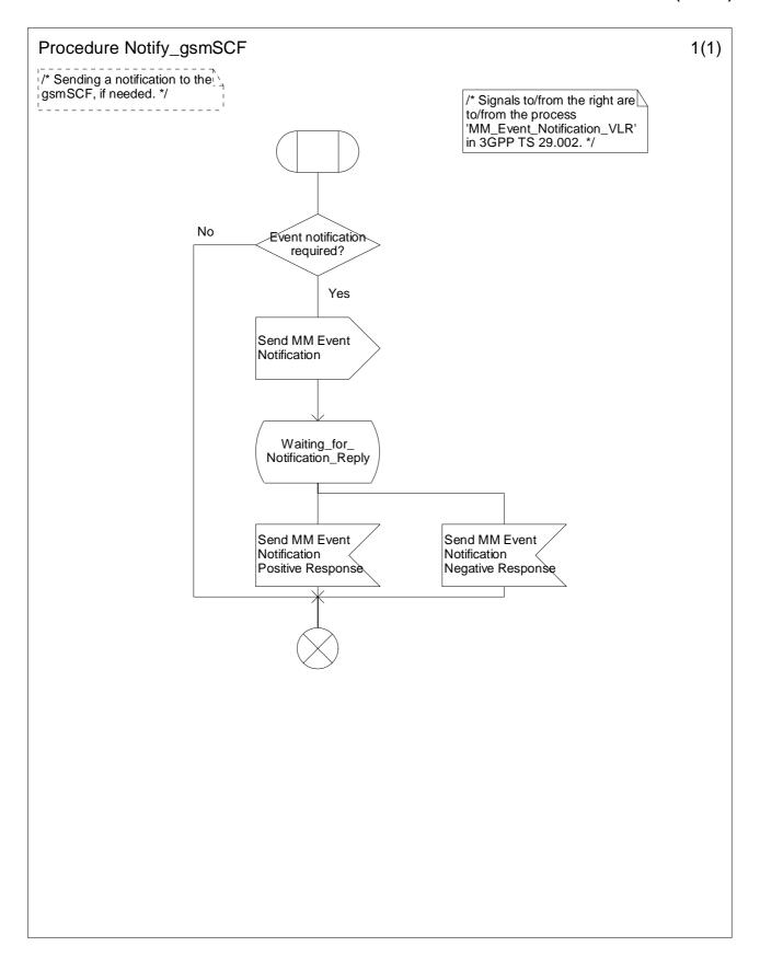
Figure 9.3-1: Procedure Notify\_gsmSCF (sheet 1)
