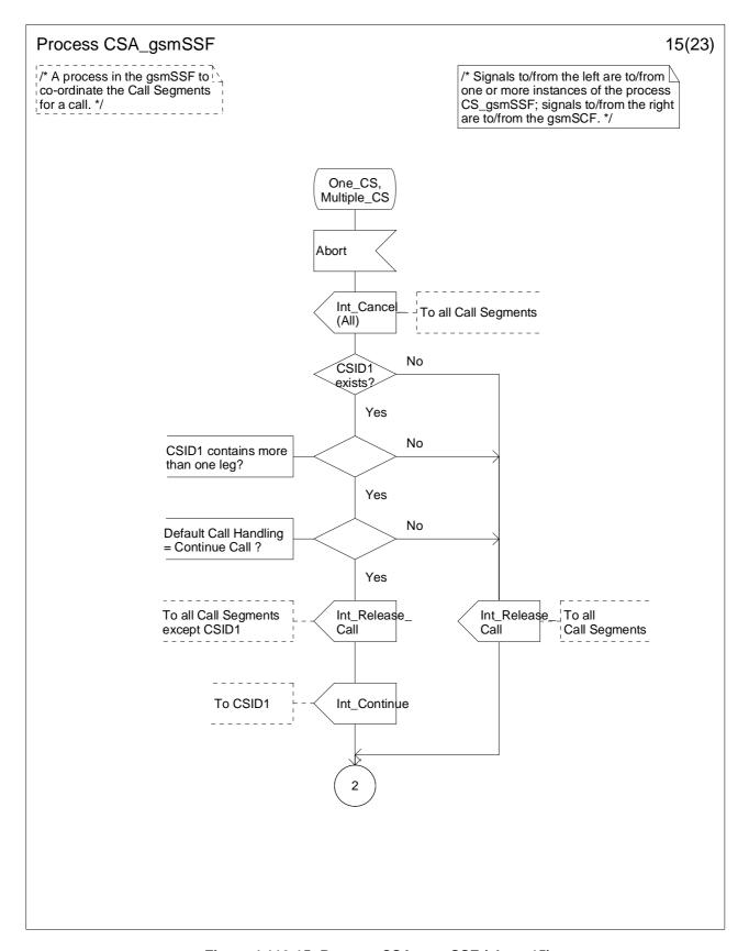
Figure 4.116-15: Process CSA\_gsmSSF (sheet 15)
