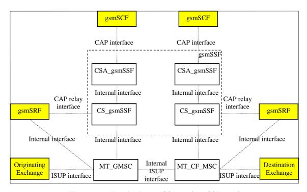
Figure 4.9-3: Terminating GMSC case (gsmSSF relay)
