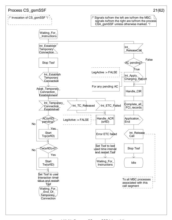
Figure 4.99-21: Process CS\_gsmSSF (sheet 21)
