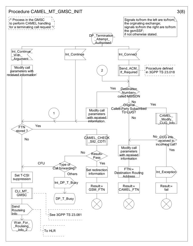
Figure 4.42-3: Procedure CAMEL\_MT\_GMSC\_INIT (sheet 3)
