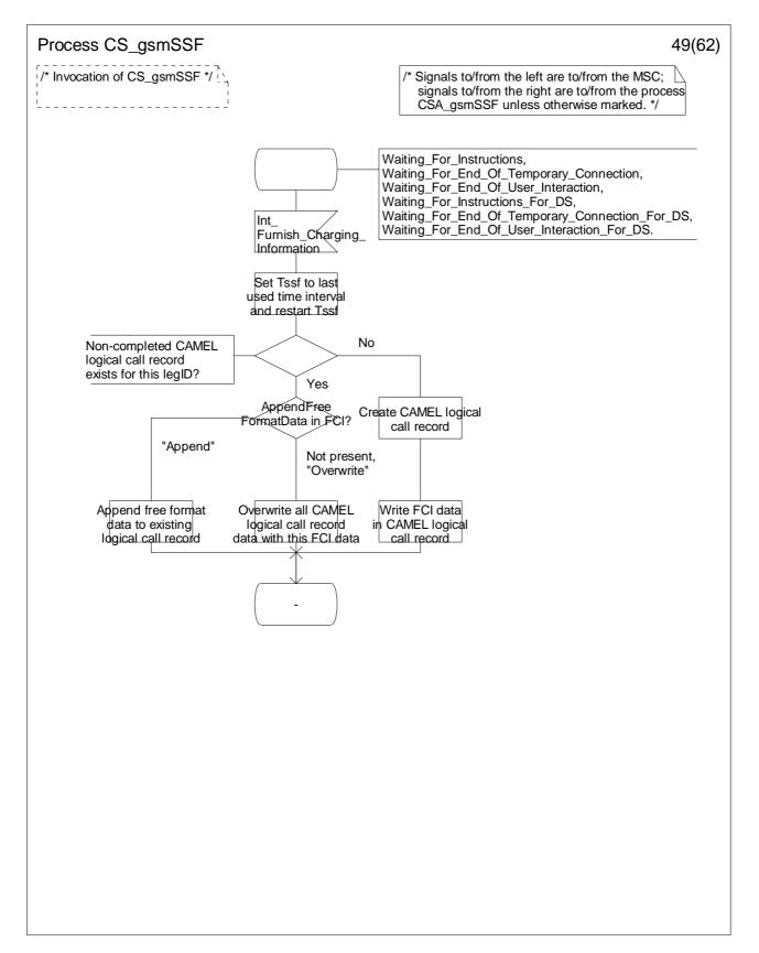
Figure 4.99-49: Process CS\_gsmSSF (sheet 49)
