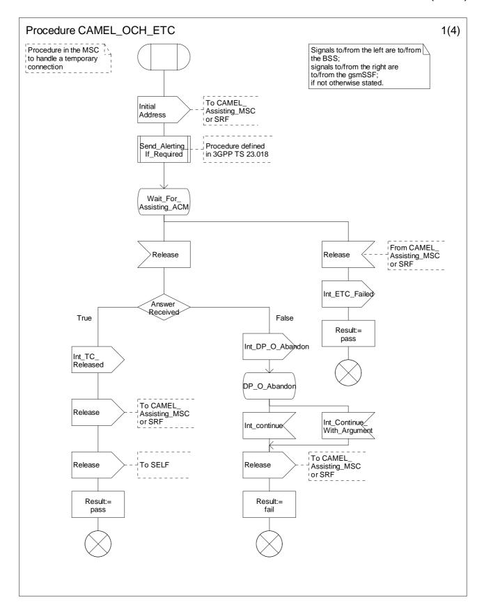
Figure 4.23-1: Procedure CAMEL\_OCH\_ETC (sheet 1)
