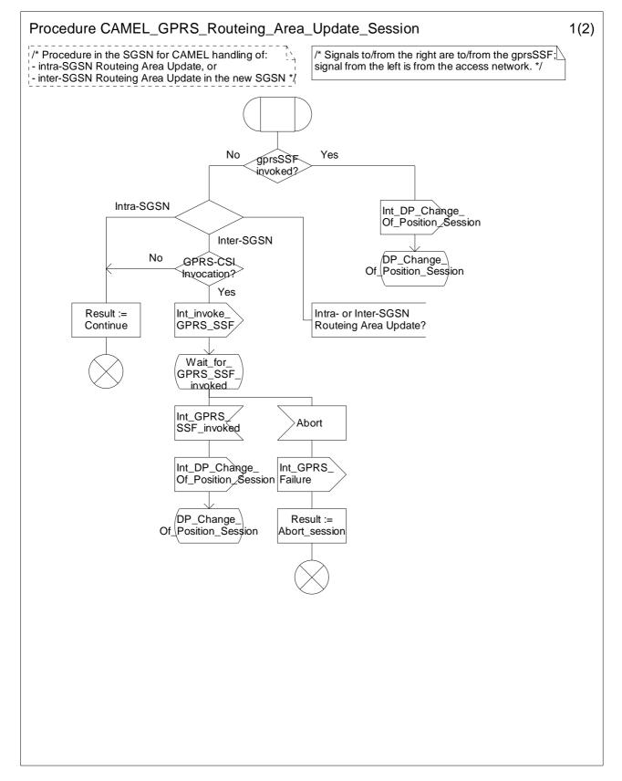
Figure 6.10-1: Procedure CAMEL\_GPRS\_Routeing\_Area\_Update\_Session (sheet 1)
