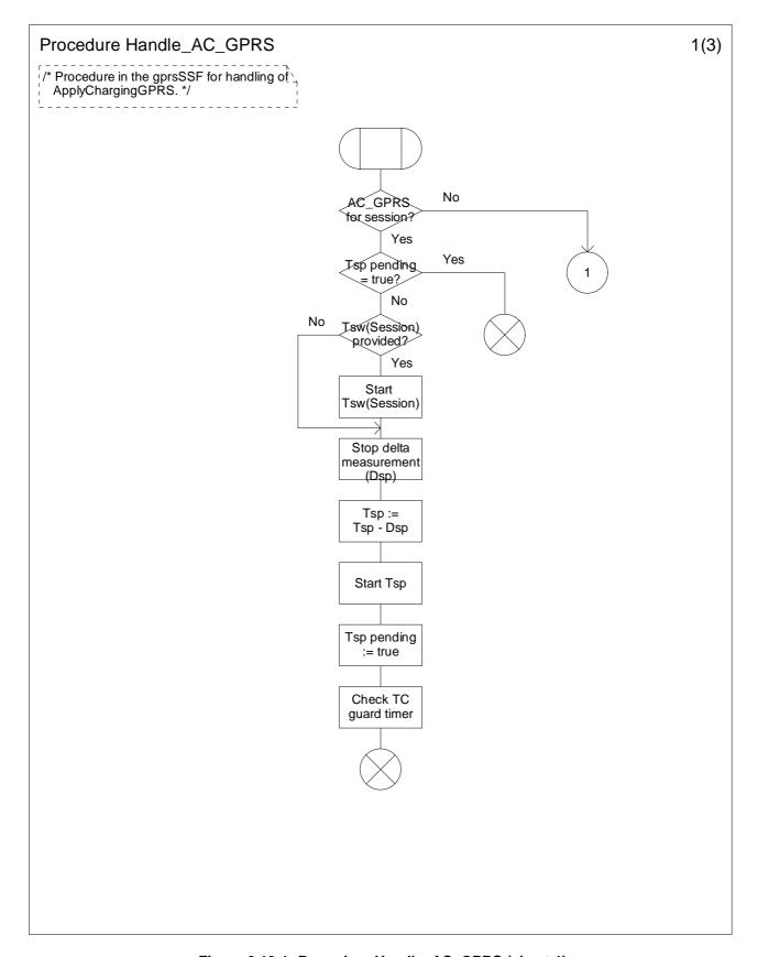
Figure 6.19-1: Procedure Handle\_AC\_GPRS (sheet 1)
