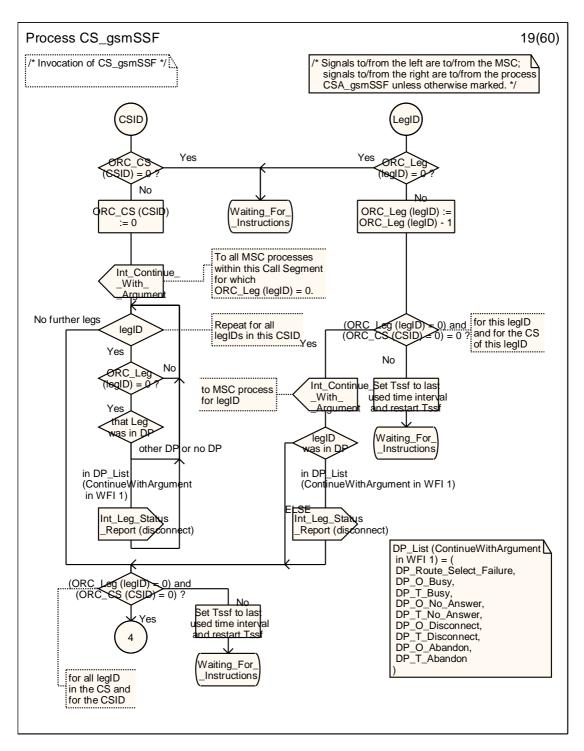
Figure 4.99-19: Process CS\_gsmSSF (sheet 19)
