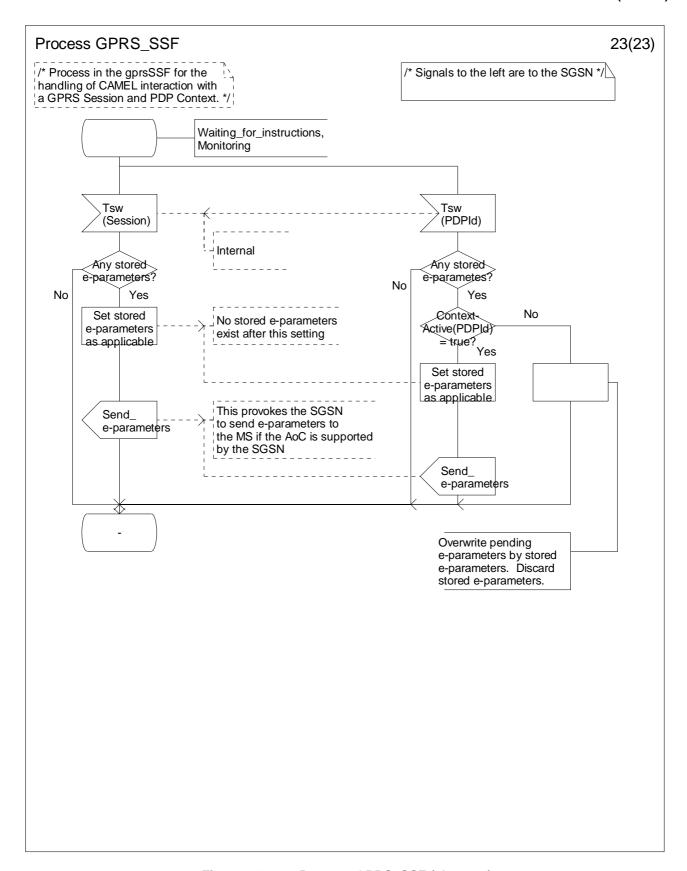
Figure 6.17-23: Process GPRS\_SSF (sheet 23)
