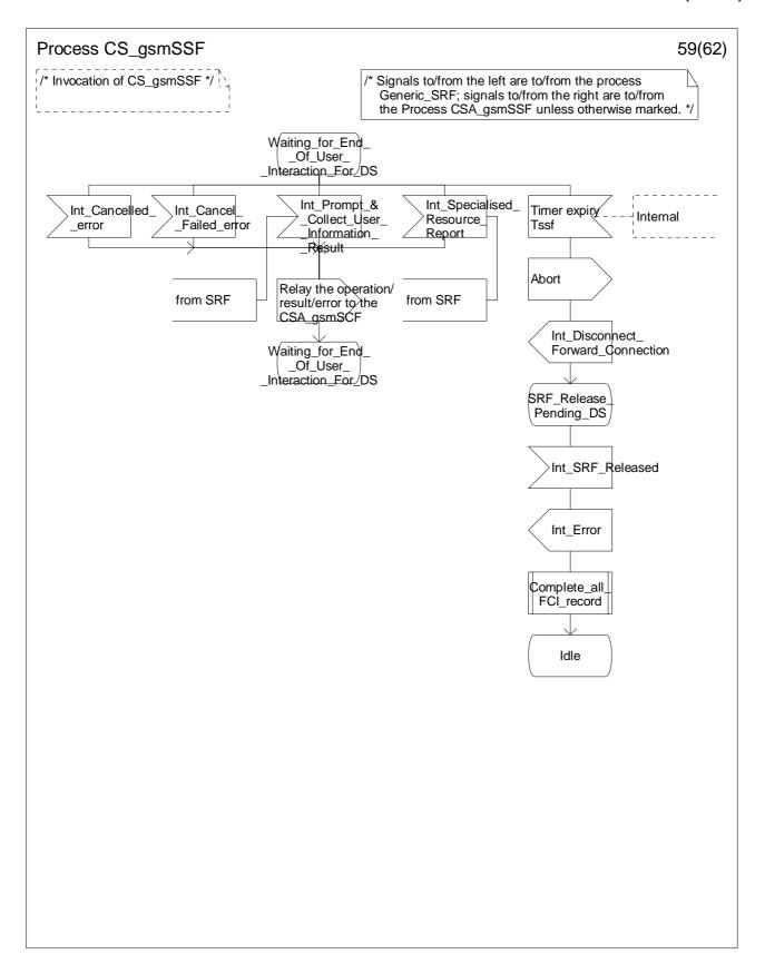
Figure 4.99-59: Process CS\_gsmSSF (sheet 59)
