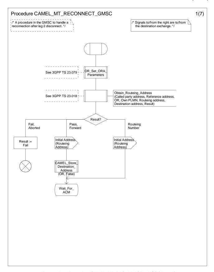
Figure 4.56-1: Procedure CAMEL\_MT\_RECONNECT\_GMSC (sheet 1)
