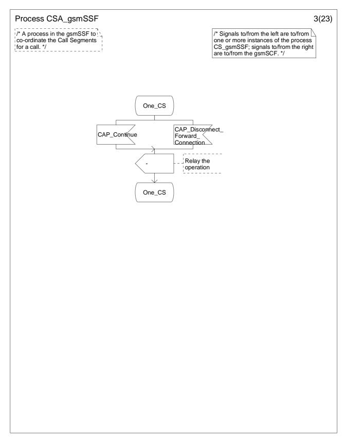
Figure 4.116-3: Process CSA\_gsmSSF (sheet 3)
