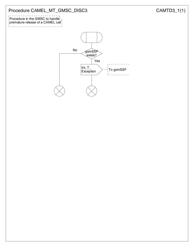
Figure 4.47-1: Procedure CAMEL\_MT\_GMSC\_DISC3 (sheet 1)
