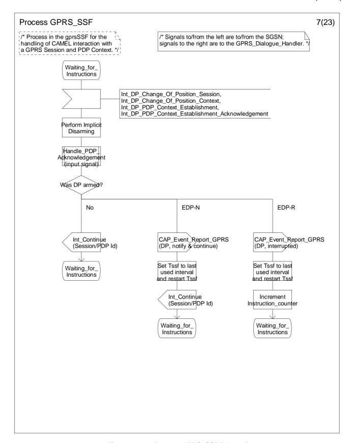
Figure 6.17-7: Process GPRS\_SSF (sheet 7)
