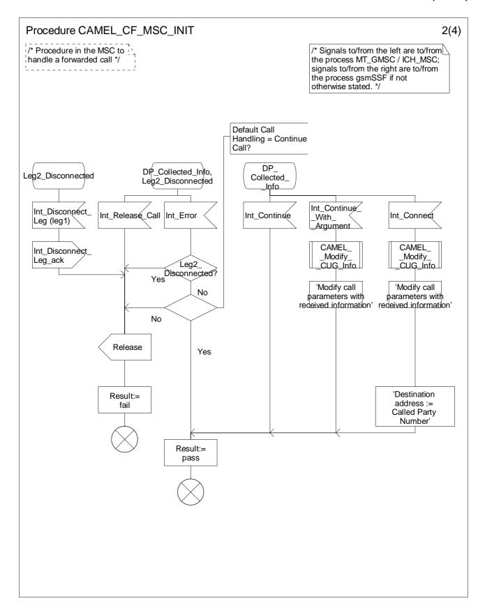
Figure 4.79-2: Procedure CAMEL\_CF\_MSC\_INIT (sheet 2)
