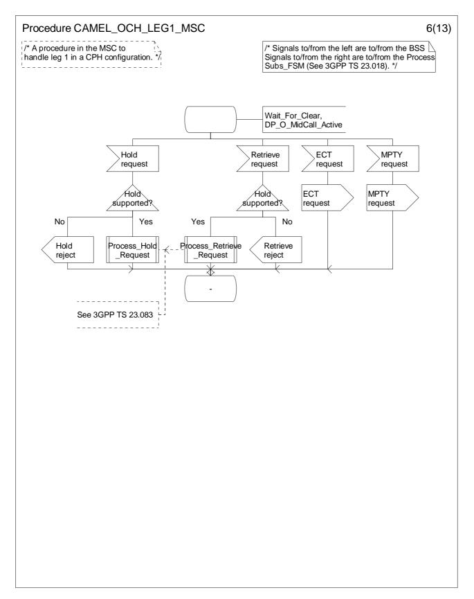
Figure 4.30-6: Procedure CAMEL\_OCH\_LEG1\_MSC (sheet 6)
