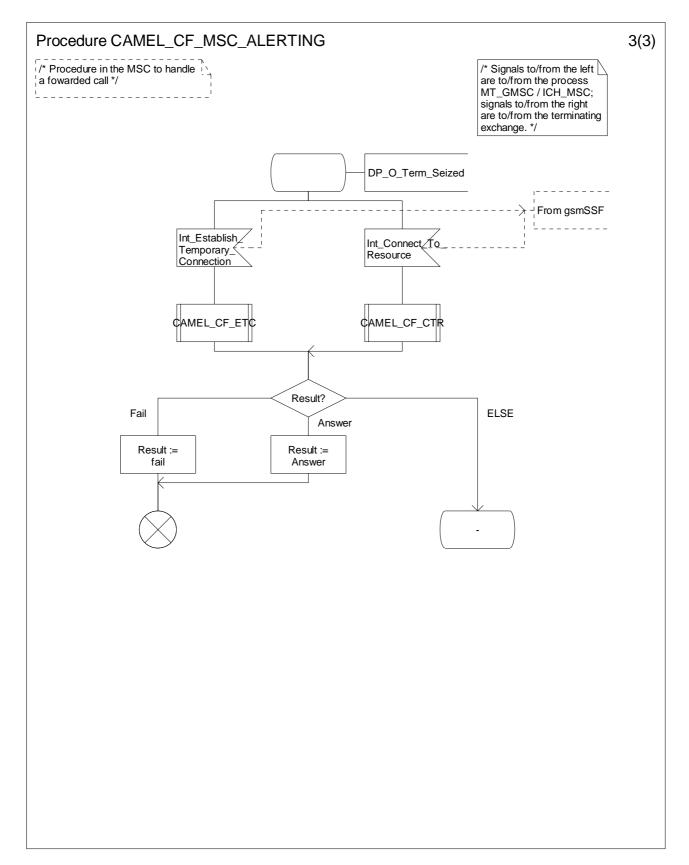
Figure 4.82-3: Procedure CAMEL\_CF\_MSC\_ALERTING (sheet 3)
