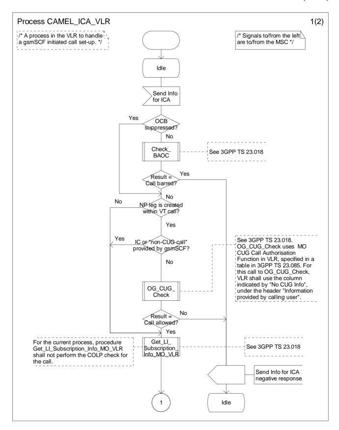
Figure 4.95-1: Process CAMEL\_ICA\_VLR (sheet 1)
