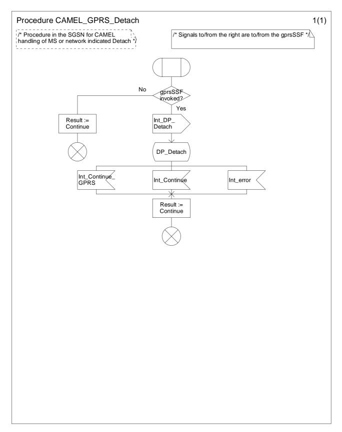
Figure 6.9-1: Procedure CAMEL\_GPRS\_Detach (sheet 1)
