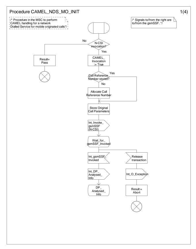
Figure 4.13-1: Procedure CAMEL\_NDS\_MO\_INIT (sheet 1)
