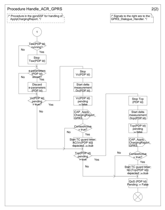
Figure 6.20-2: Procedure Handle\_ACR\_GPRS (sheet 2)
