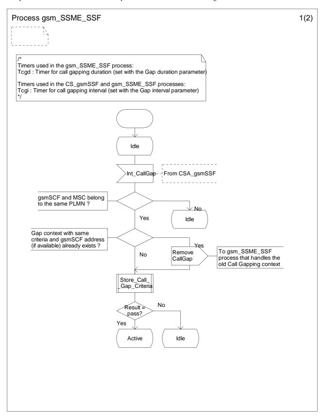
Figure 4.113-1: Process gsm\_SSME\_SSF (sheet 1)
