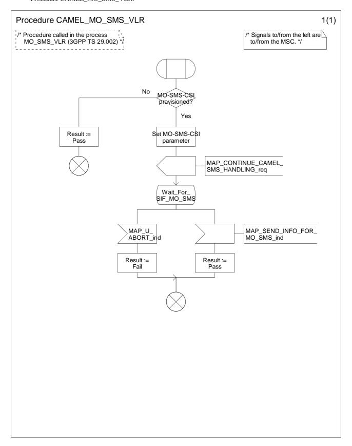
Figure 7.8-1: Procedure CAMEL\_MO\_SMS\_VLR (sheet 1)
