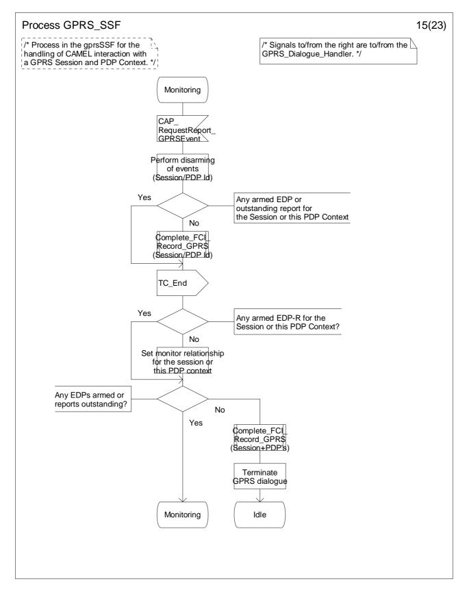
Figure 6.17-15: Process GPRS\_SSF (sheet 15)
