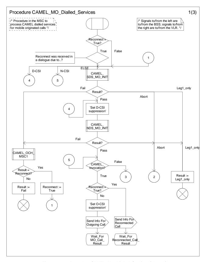
Figure 4.11-1: Procedure CAMEL\_MO\_Dialled\_Services (sheet 1)
