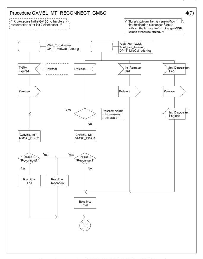
Figure 4.56-4: Procedure CAMEL\_MT\_RECONNECT\_GMSC (sheet 4)
