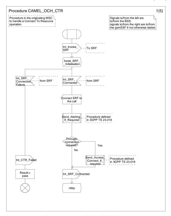
Figure 4.24-1: Procedure CAMEL\_OCH\_CTR (sheet 1)
