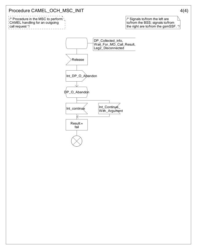
Figure 4.10-4: Procedure CAMEL\_OCH\_MSC\_INIT (sheet 4)
