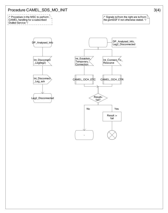
Figure 4.12-3: Procedure CAMEL\_SDS\_MO\_INIT (sheet 3)
