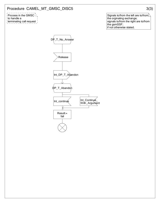
Figure 4.49-3: Procedure CAMEL\_MT\_GMSC\_DISC5 (sheet 3)
