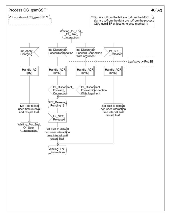
Figure 4.99-40: Process CS\_gsmSSF (sheet 40)
