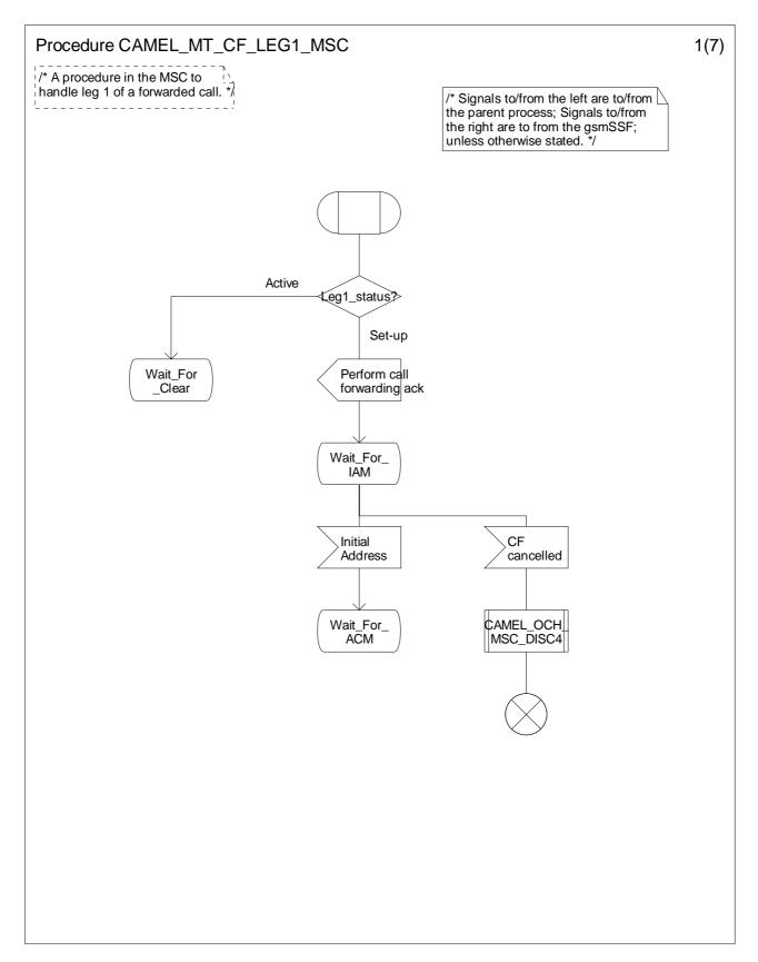
Figure 4.86-1: Procedure CAMEL\_MT\_CF\_LEG1\_MSC (sheet 1)
