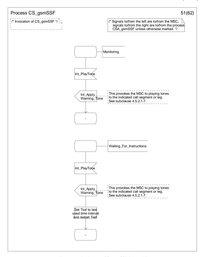
Figure 4.99-51: Process CS\_gsmSSF (sheet 51)
