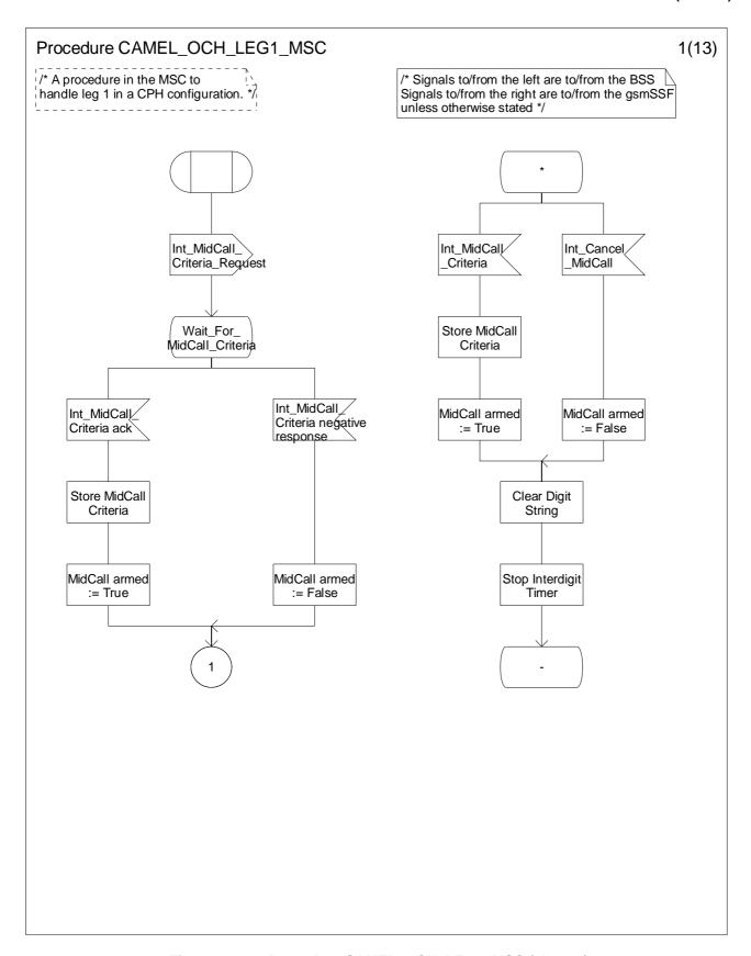
Figure 4.30-1: Procedure CAMEL\_OCH\_LEG1\_MSC (sheet 1)
