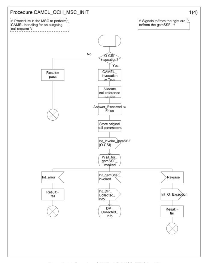
Figure 4.10-1: Procedure CAMEL\_OCH\_MSC\_INIT (sheet 1)
