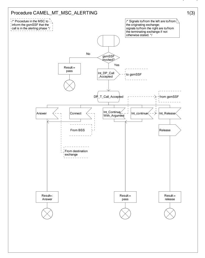
Figure 4.43-1: Procedure CAMEL\_MT\_MSC\_ALERTING (sheet 1)
