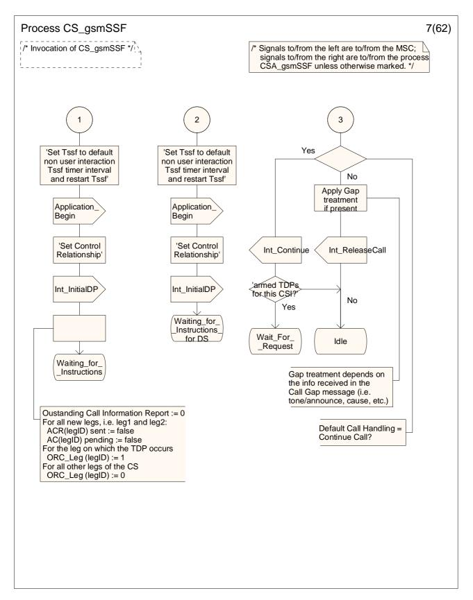
Figure 4.99-7: Process CS\_gsmSSF (sheet 7)
