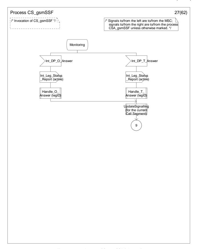
Figure 4.99-27: Process CS\_gsmSSF (sheet 27)
