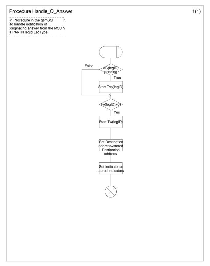
Figure 4.110-1: Procedure Handle\_O\_Answer (sheet 1)
