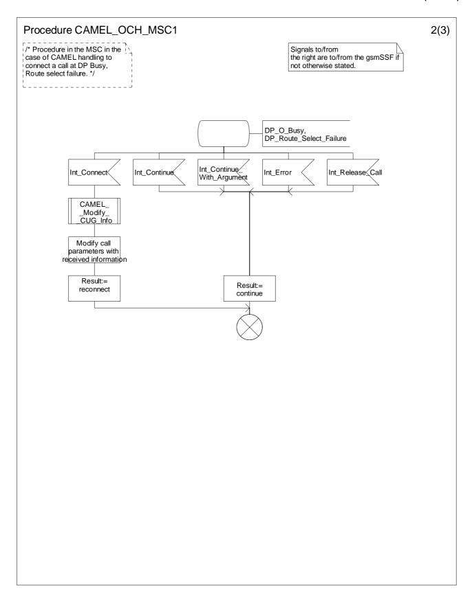
Figure 4.16-2: Procedure CAMEL\_OCH\_MSC1 (sheet 2)
