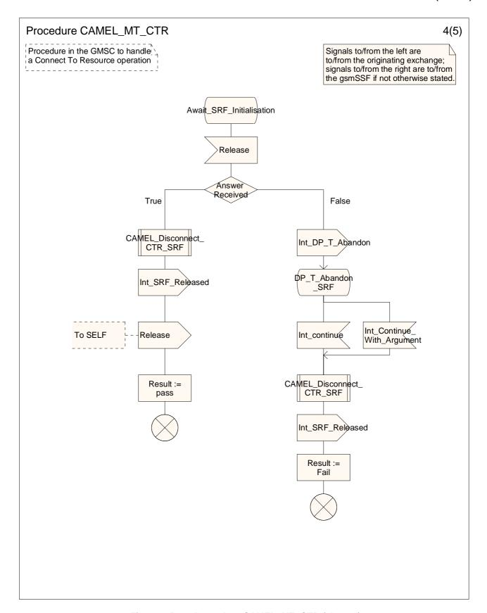
Figure 4.52-4: Procedure CAMEL\_MT\_CTR (sheet 4)
