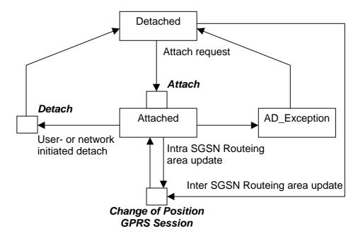
Figure 6.3: GPRS Attach/Detach State Model
