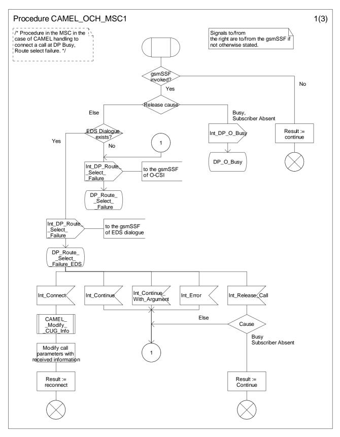
Figure 4.16-1: Procedure CAMEL\_OCH\_MSC1 (sheet 1)
