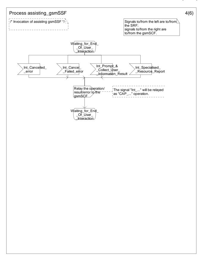
Figure 4.118-4: Process Assisting\_gsmSSF (sheet 4)
