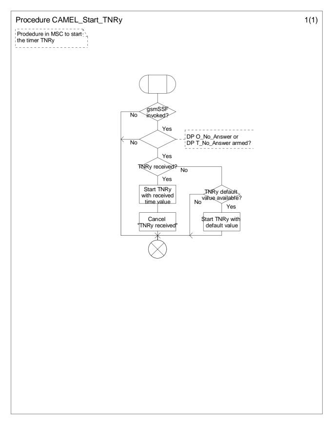
Figure 4.25-1: Procedure CAMEL\_Start\_TNRy (sheet 1)
