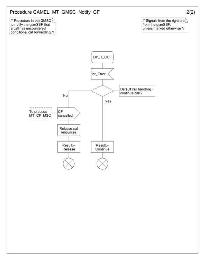
Figure 4.53-2: Procedure CAMEL\_MT\_GMSC\_Notify\_CF (sheet 2)
