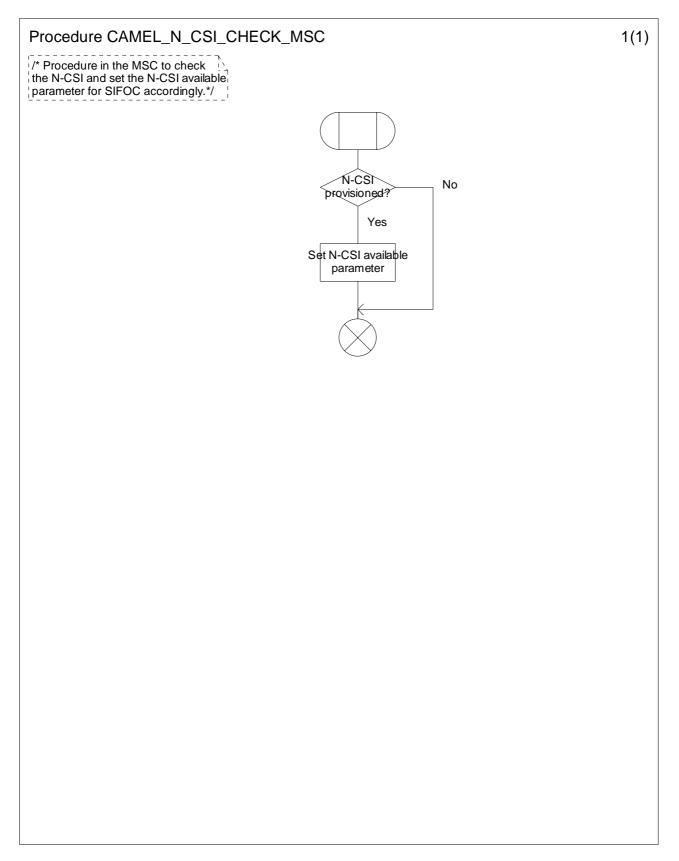
Figure 4.29-1: Procedure CAMEL\_N\_CSI\_CHECK\_MSC (sheet 1)
