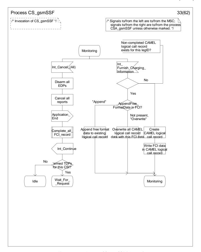
Figure 4.99-33: Process CS\_gsmSSF (sheet 33)
