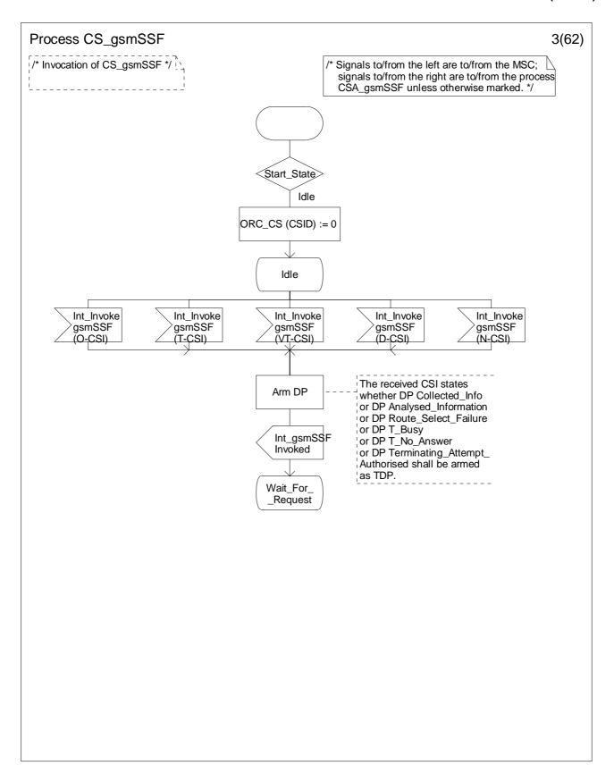
Figure 4.99-3: Process CS\_gsmSSF (sheet 3)
