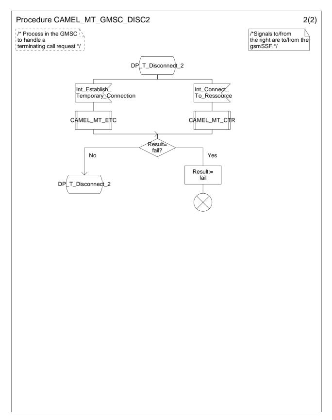
Figure 4.46-2: Procedure CAMEL\_MT\_GMSC\_DISC2 (sheet 2)
