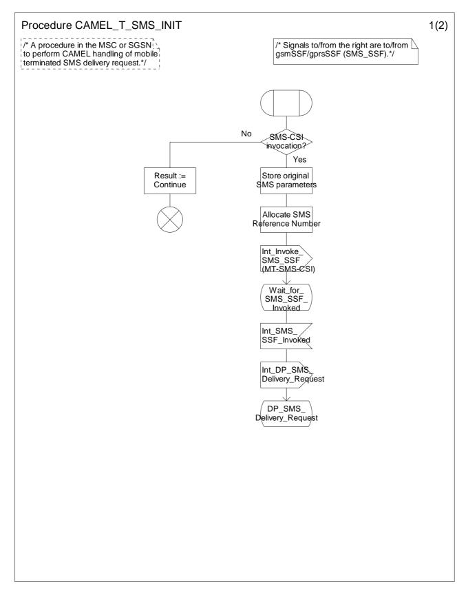
Figure 7.10-1: Procedure CAMEL\_T\_SMS\_INIT (sheet 1)
