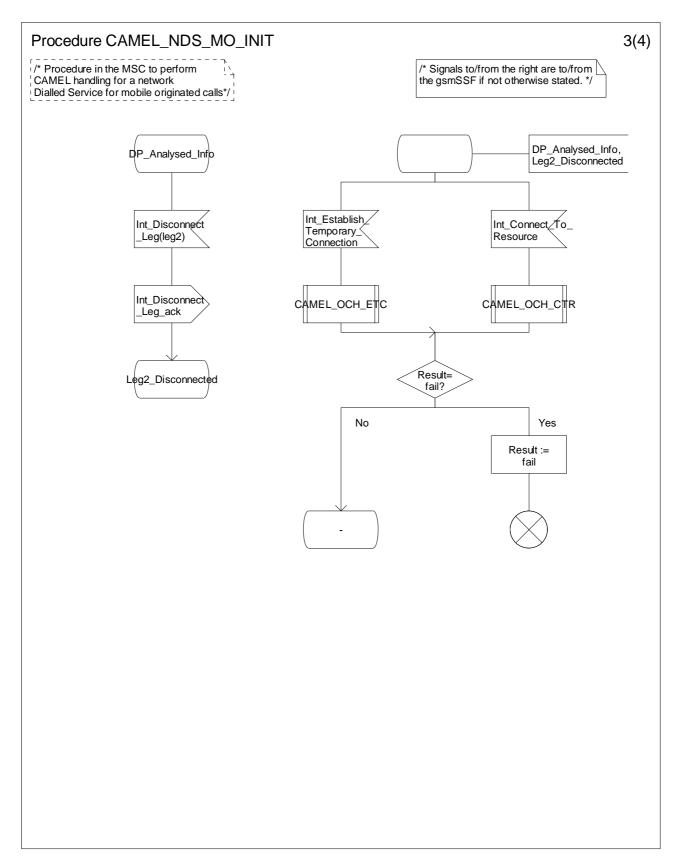
Figure 4.13-3: Procedure CAMEL\_NDS\_MO\_INIT (sheet 3)
