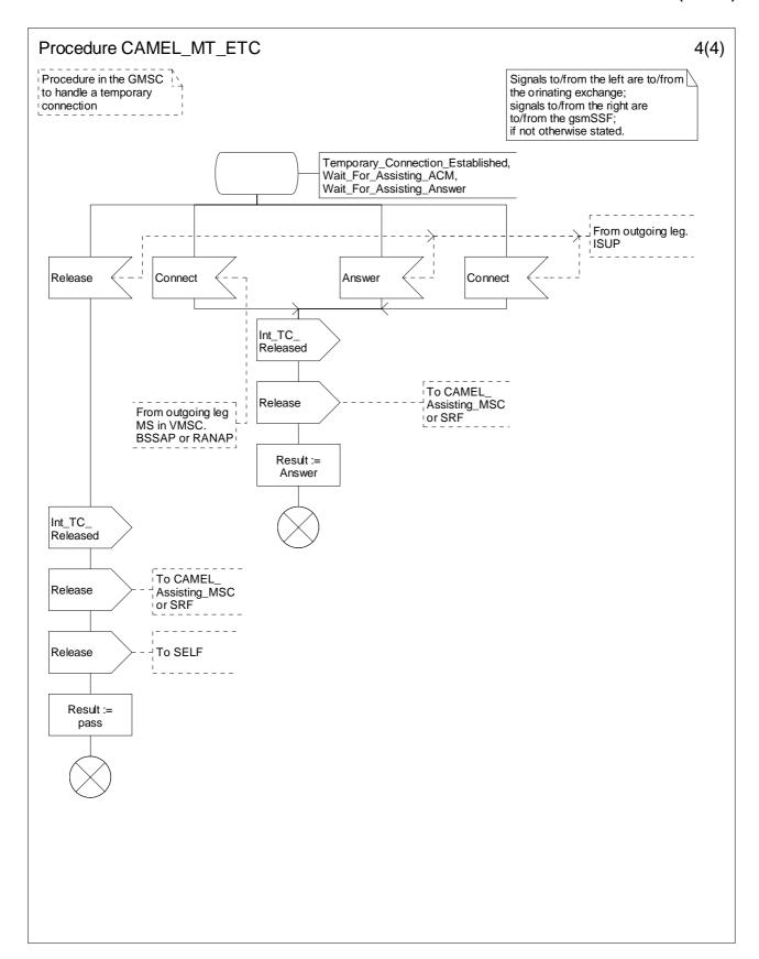
Figure 4.51-4: Procedure CAMEL\_MT\_ETC (sheet 4)
