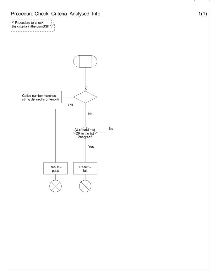
Figure 4.101-1: Procedure Check\_Criteria\_Analysed\_Info (sheet 1)
