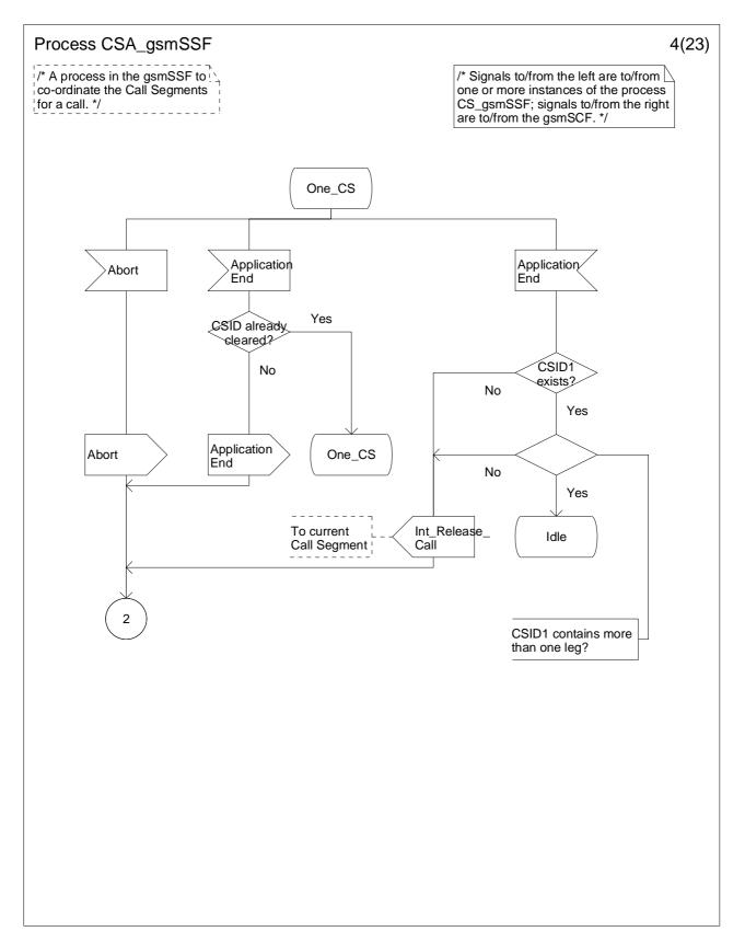
Figure 4.116-4: Process CSA\_gsmSSF (sheet 4)
