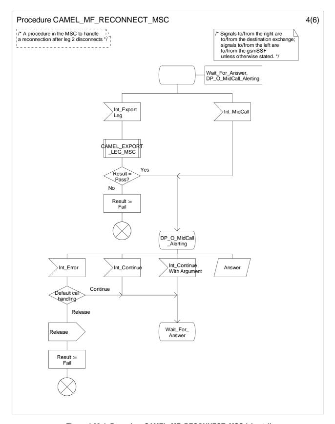
Figure 4.88-4: Procedure CAMEL\_MF\_RECONNECT\_MSC (sheet 4)
