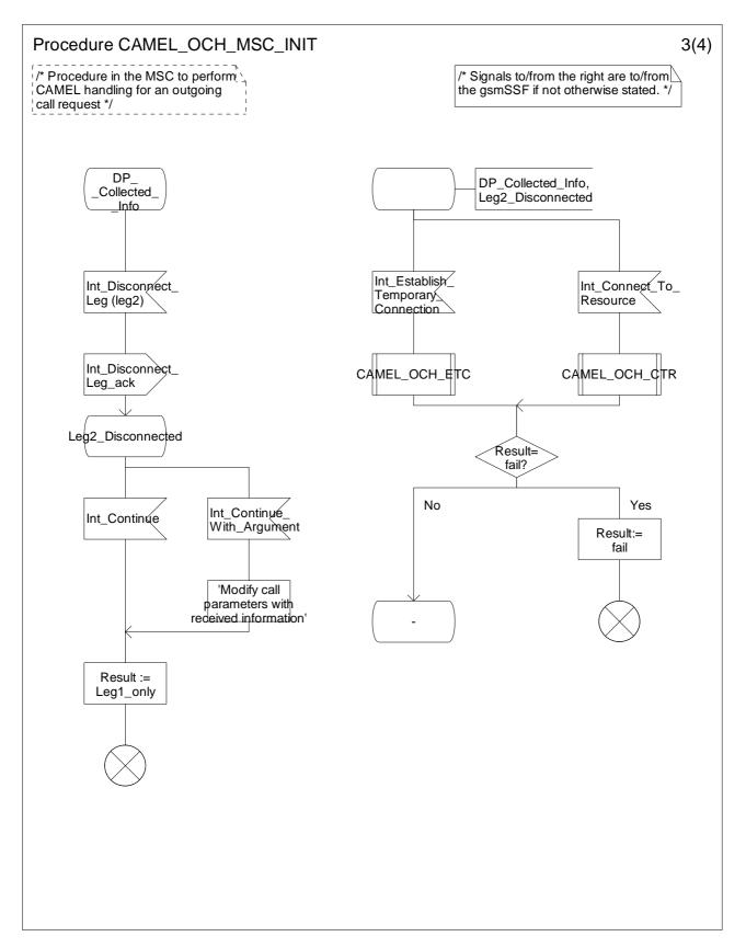
Figure 4.10-3: Procedure CAMEL\_OCH\_MSC\_INIT (sheet 3)
