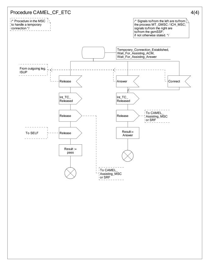
Figure 4.84-4: Procedure CAMEL\_CF\_ETC (sheet 4)
