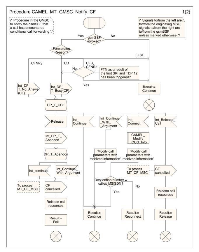
Figure 4.53-1: Procedure CAMEL\_MT\_GMSC\_Notify\_CF (sheet 1)
