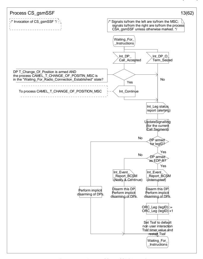
Figure 4.99-13: Process CS\_gsmSSF (sheet 13)
