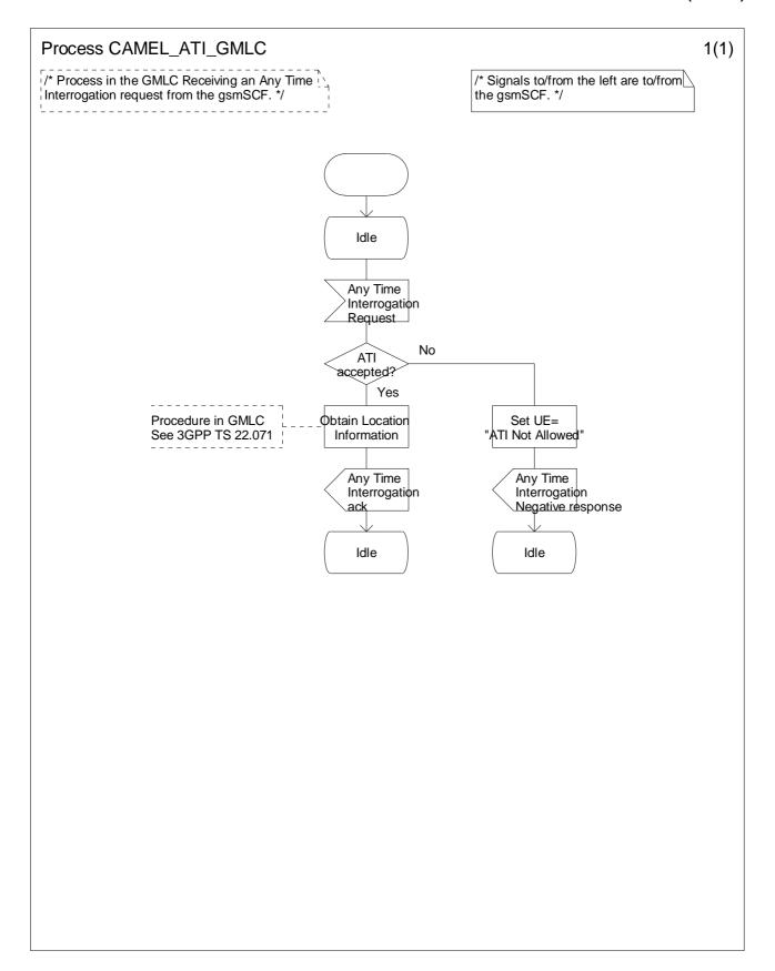
Figure 11.2-1: Process CAMEL\_ATI\_GMLC (sheet 1)
