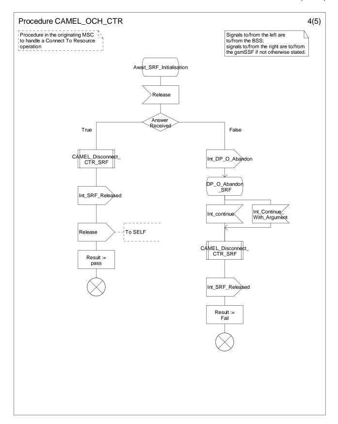
Figure 4.24-4: Procedure CAMEL\_OCH\_CTR (sheet 4)
