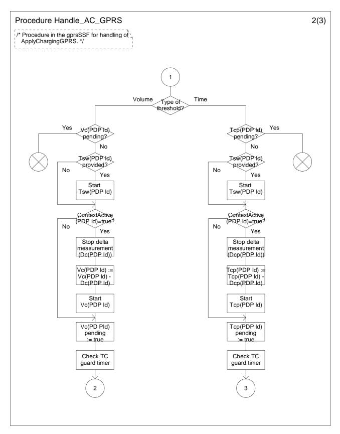
Figure 6.19-2: Procedure Handle\_AC\_GPRS (sheet 2)
