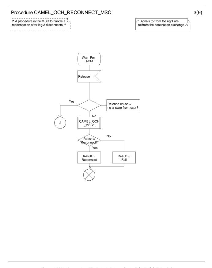
Figure 4.33-3: Procedure CAMEL\_OCH\_RECONNECT\_MSC (sheet 3)
