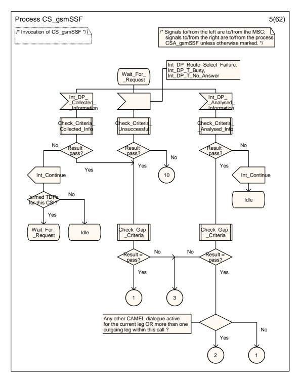
Figure 4.99-5: Process CS\_gsmSSF (sheet 5)
