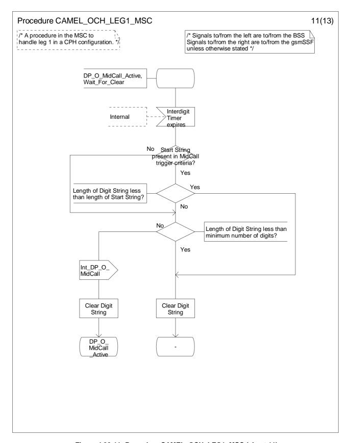
Figure 4.30-11: Procedure CAMEL\_OCH\_LEG1\_MSC (sheet 11)
