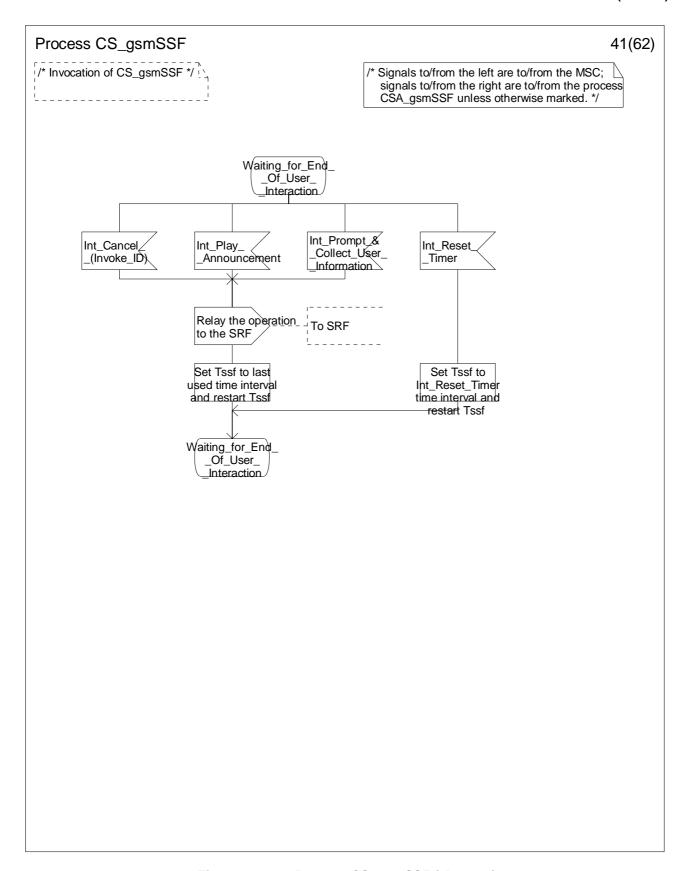
Figure 4.99-41: Process CS\_gsmSSF (sheet 41)
