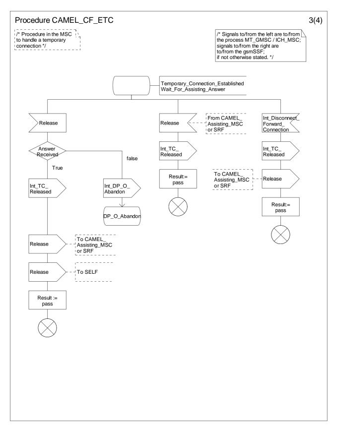
Figure 4.84-3: Procedure CAMEL\_CF\_ETC (sheet 3)
