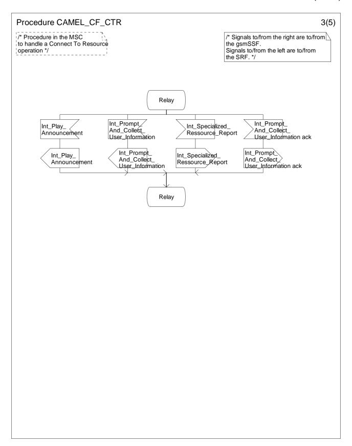
Figure 4.85-3: Procedure CAMEL\_CF\_CTR (sheet 3)
