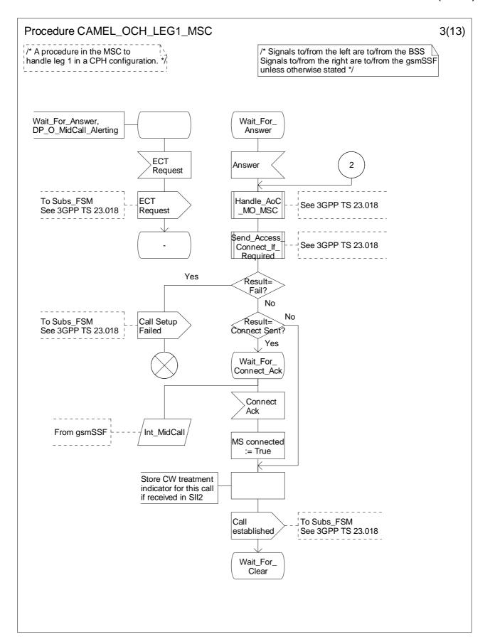
Figure 4.30-3: Procedure CAMEL\_OCH\_LEG1\_MSC (sheet 3)
