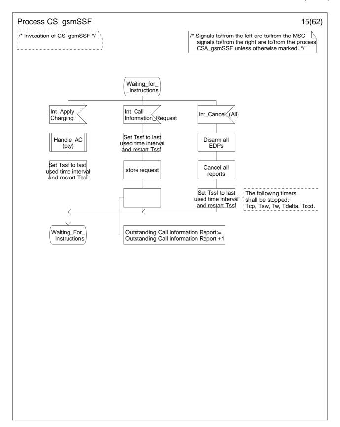
Figure 4.99-15: Process CS\_gsmSSF (sheet 15)
