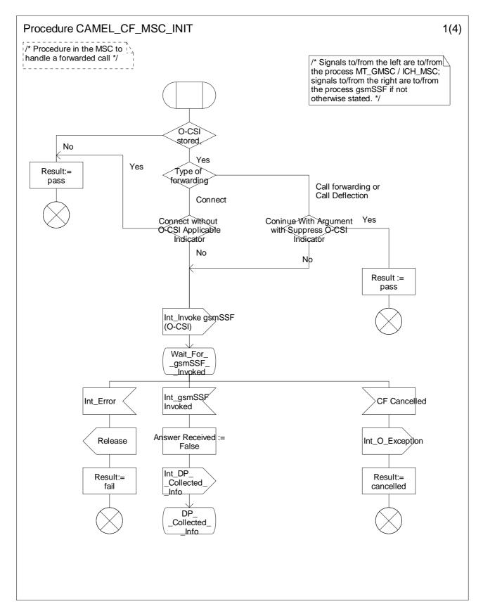
Figure 4.79-1: Procedure CAMEL\_CF\_MSC\_INIT (sheet 1)
