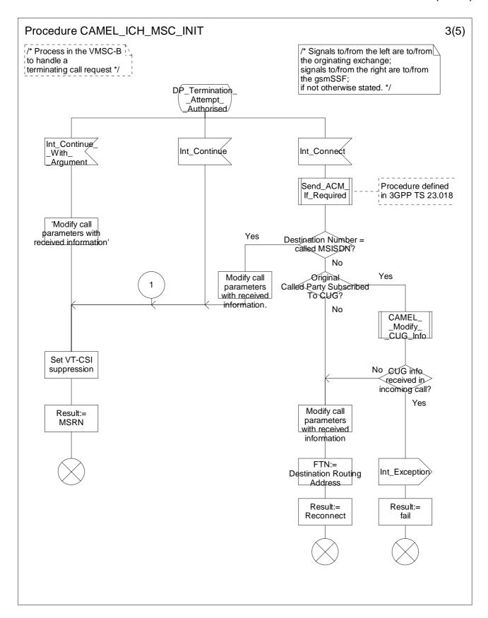
Figure 4.69-3: Procedure CAMEL\_ICH\_MSC\_INIT (sheet 3)
