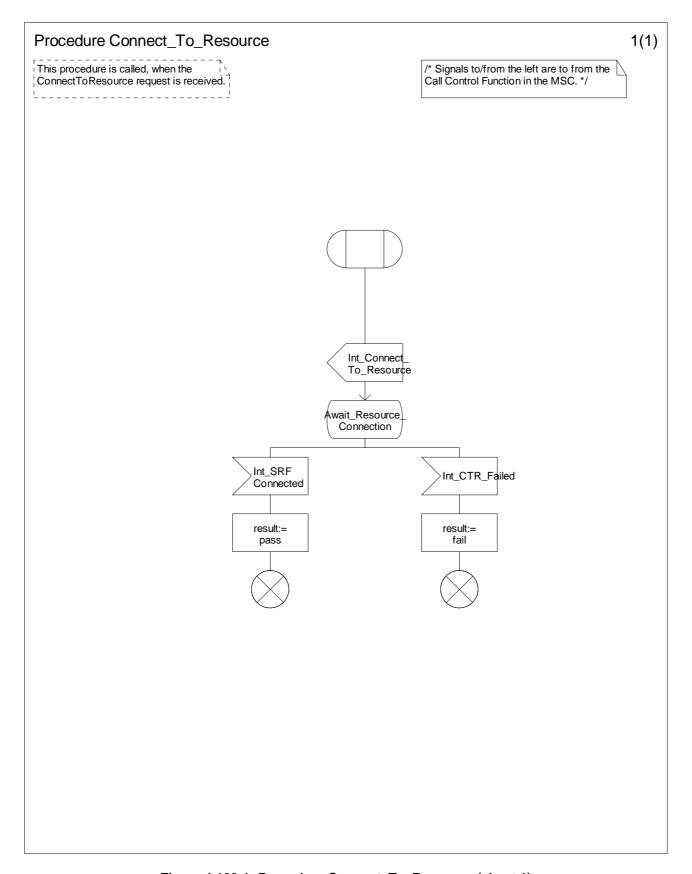
Figure 4.103-1: Procedure Connect\_To\_Resource (sheet 1)
