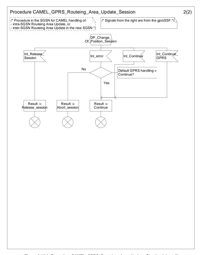
Figure 6.10-2: Procedure CAMEL\_GPRS\_Routeing\_Area\_Update\_Session (sheet 2)
