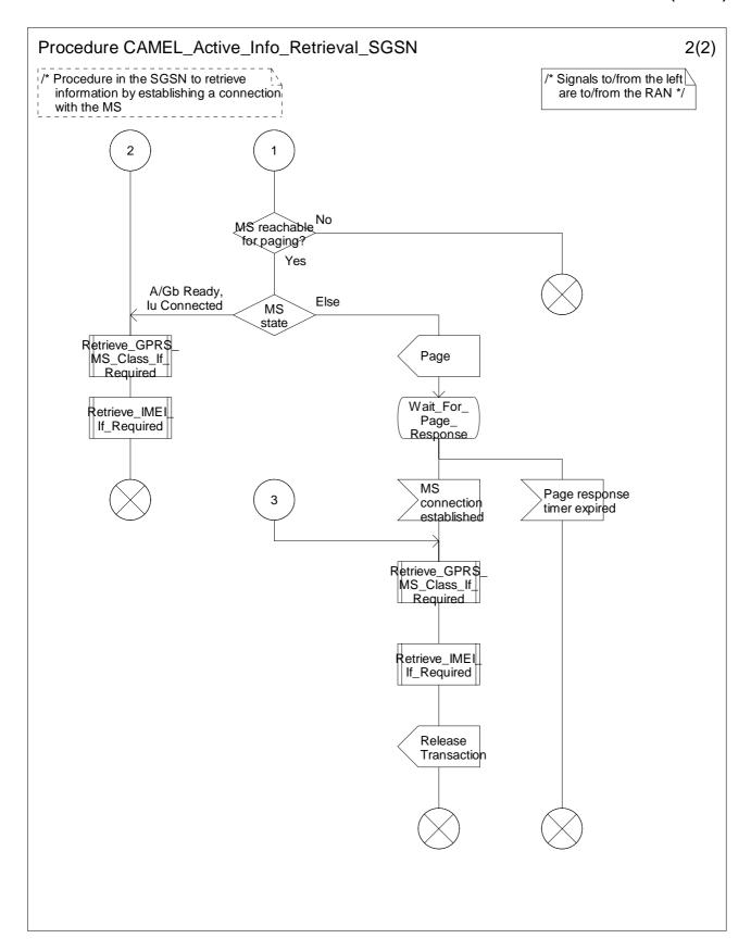
Figure 11.5-2: Procedure CAMEL\_Active\_Info\_Retrieval\_SGSN (sheet 2)
