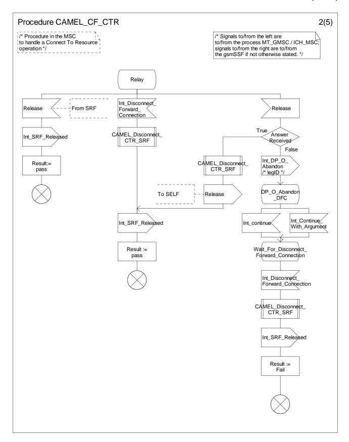
Figure 4.85-2: Procedure CAMEL\_CF\_CTR (sheet 2)
