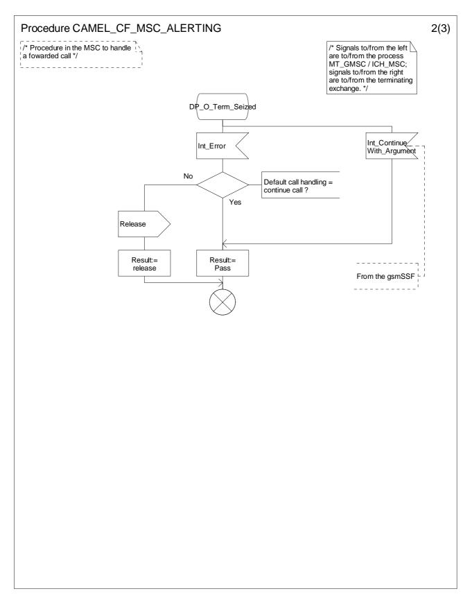
Figure 4.82-2: Procedure CAMEL\_CF\_MSC\_ALERTING (sheet 2)
