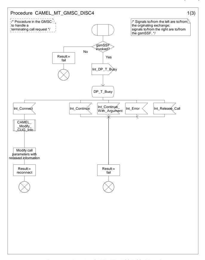
Figure 4.48-1: Procedure CAMEL\_MT\_GMSC\_DISC4 (sheet 1)
