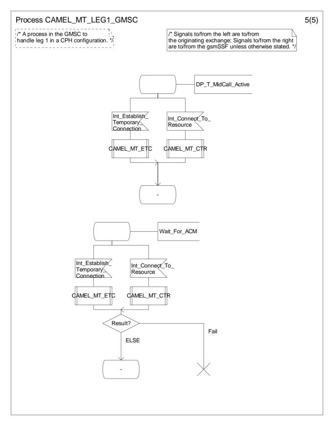
Figure 4.55-5: Process CAMEL\_MT\_LEG1\_GMSC (sheet 5)
