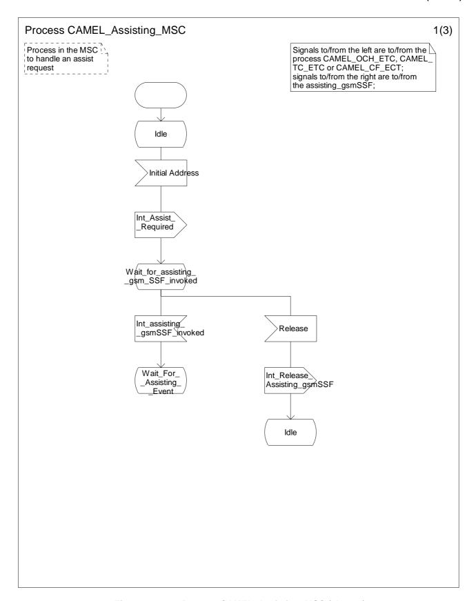
Figure 4.117-1: Process CAMEL\_Assisting\_MSC (sheet 1)
