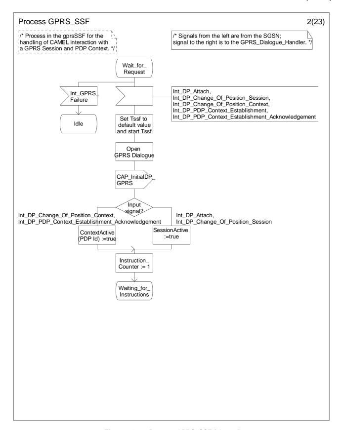
Figure 6.17-2: Process GPRS\_SSF (sheet 2)
