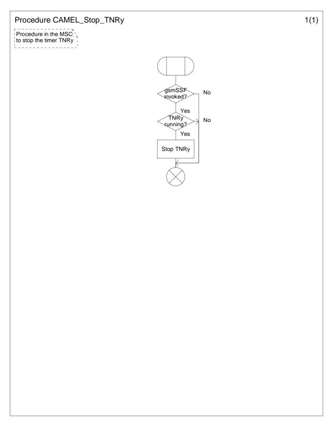
Figure 4.26-1: Procedure CAMEL\_Stop\_TNRy (sheet 1)
