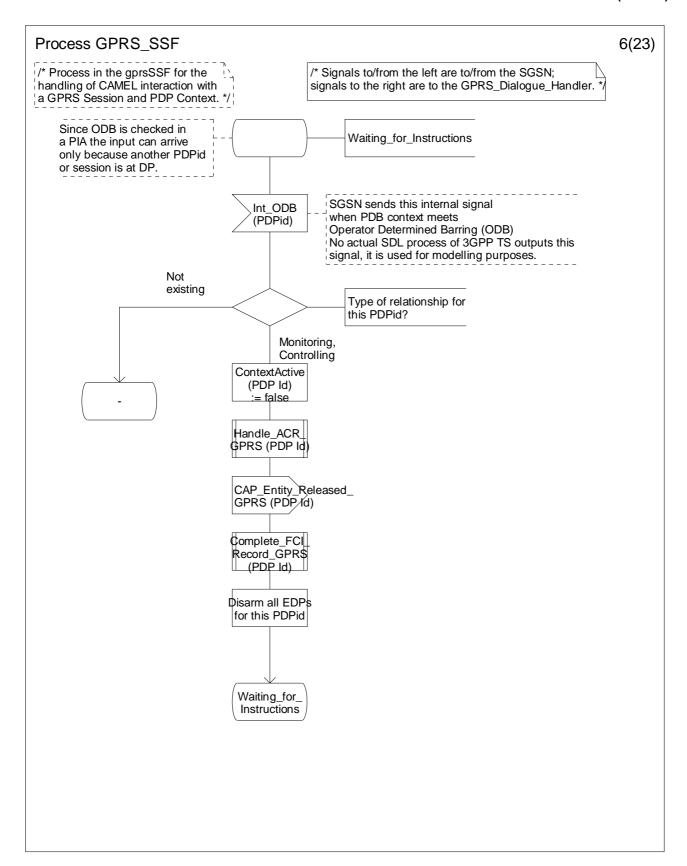
Figure 6.17-6: Process GPRS\_SSF (sheet 6)
