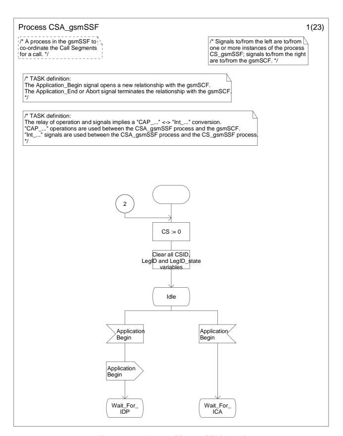
Figure 4.116-1: Process CSA\_gsmSSF (sheet 1)
