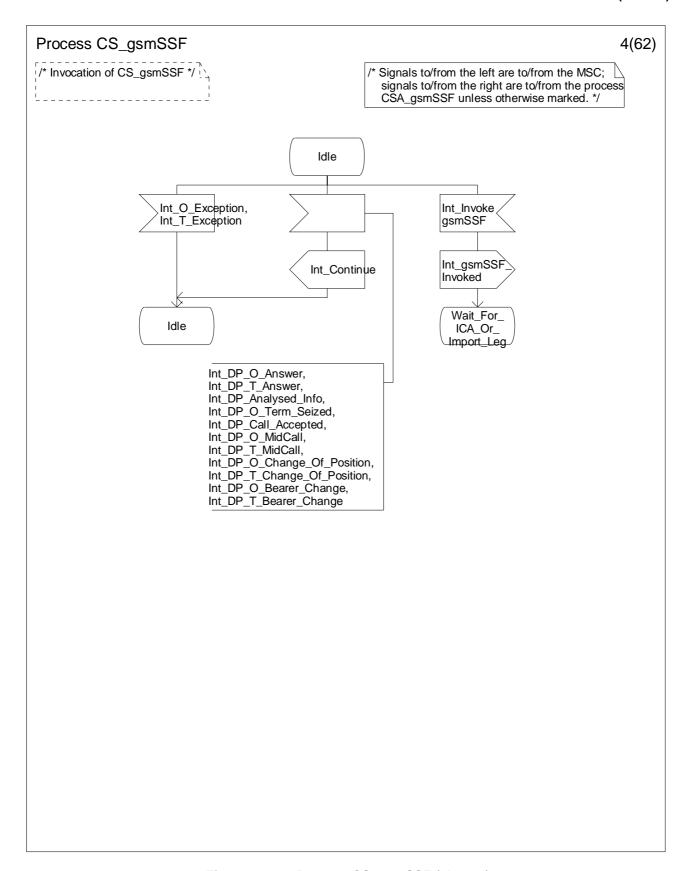
Figure 4.99-4: Process CS\_gsmSSF (sheet 4)
