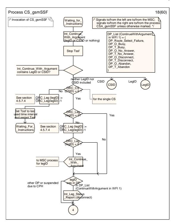
Figure 4.99-18: Process CS\_gsmSSF (sheet 18)
