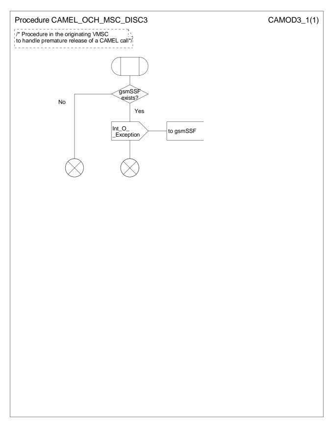
Figure 4.20-1: Procedure CAMEL\_OCH\_MSC\_DISC3 (sheet 1)
