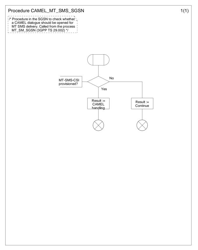
Figure 7.14-1: Procedure CAMEL\_MT\_SMS\_SGSN (sheet 1)
