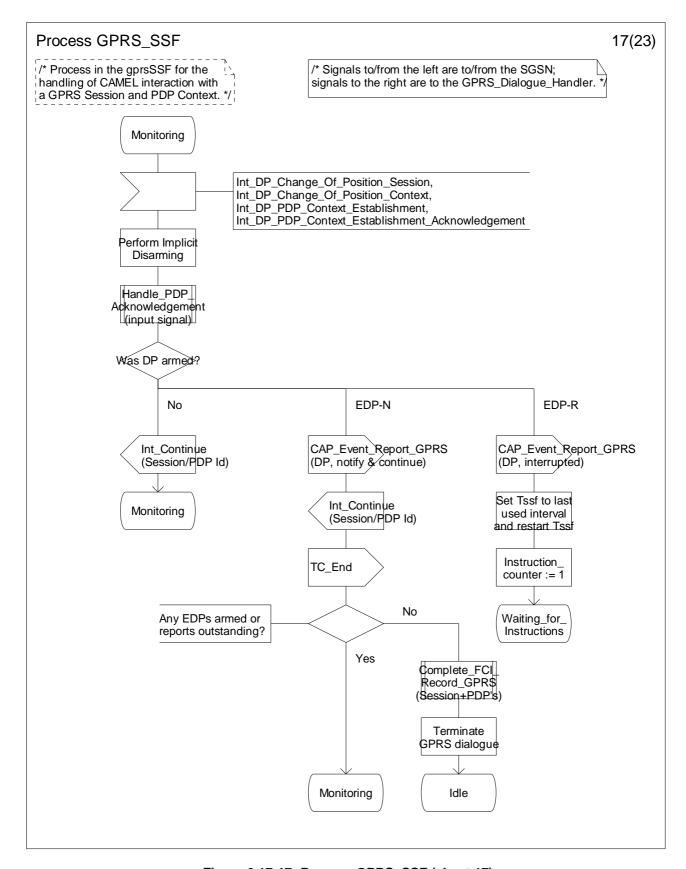
Figure 6.17-17: Process GPRS\_SSF (sheet 17)
