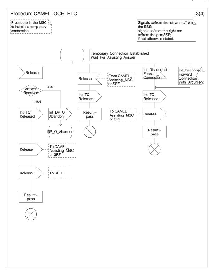
Figure 4.23-3: Procedure CAMEL\_OCH\_ETC (sheet 3)
