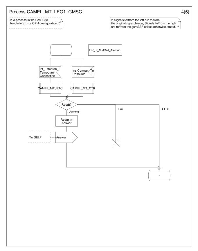
Figure 4.55-4: Process CAMEL\_MT\_LEG1\_GMSC (sheet 4)
