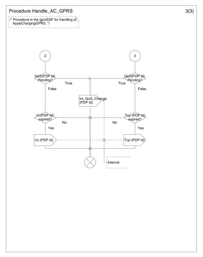
Figure 6.19-3: Procedure Handle\_AC\_GPRS (sheet 3)
