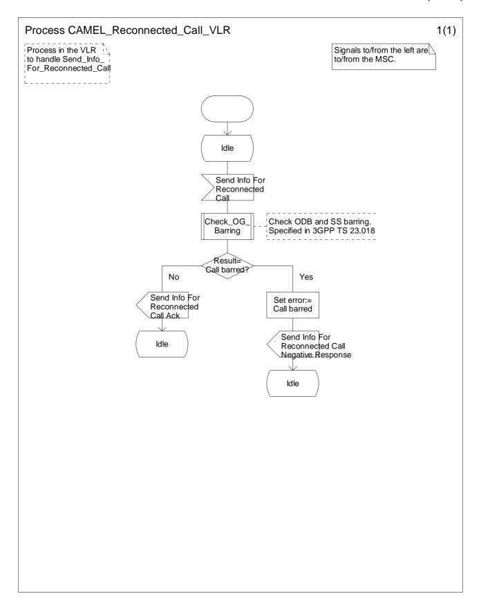
Figure 4.40-1: Process CAMEL\_Reconnected\_Call\_VLR (sheet 1)
