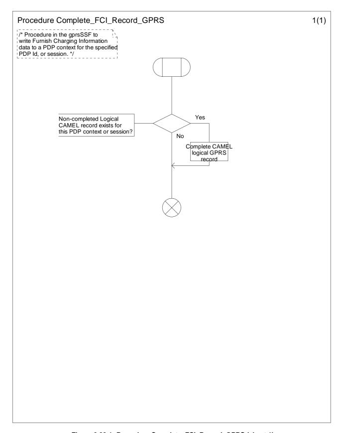
Figure 6.22-1: Procedure Complete\_FCI\_Record\_GPRS (sheet 1)
