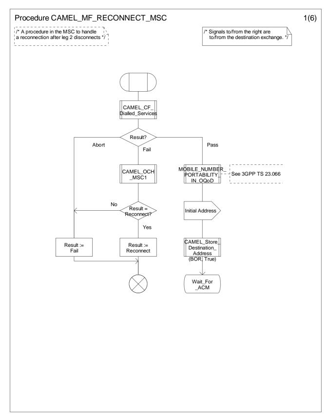
Figure 4.88-1: Procedure CAMEL\_MF\_RECONNECT\_MSC (sheet 1)
