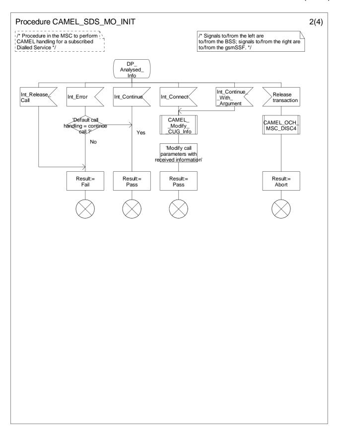
Figure 4.12-2: Procedure CAMEL\_SDS\_MO\_INIT (sheet 2)
