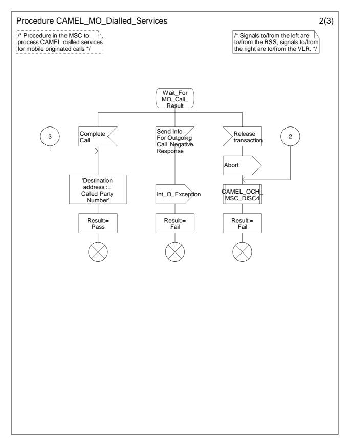
Figure 4.11-2: Procedure CAMEL\_MO\_Dialled\_Services (sheet 2)
