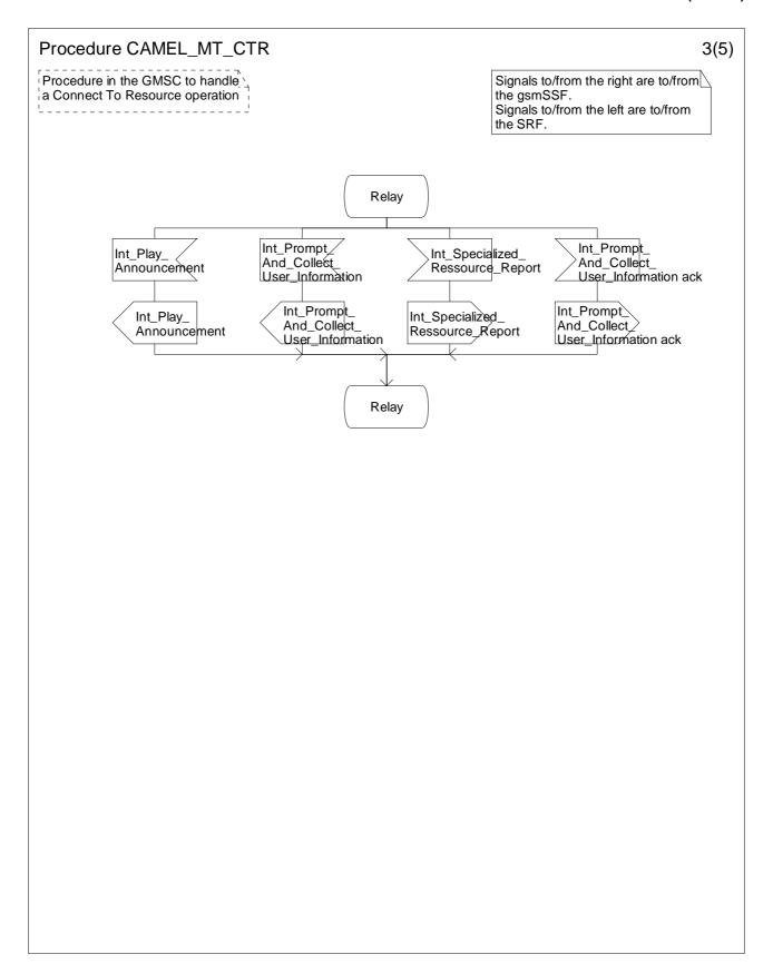
Figure 4.52-3: Procedure CAMEL\_MT\_CTR (sheet 3)
