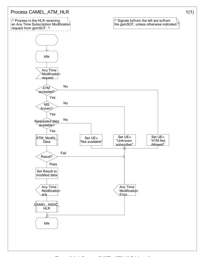
Figure 10.3-1: Process CAMEL\_ATM\_HLR (sheet 1)
