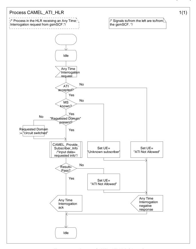
Figure 11.3-1: Process CAMEL\_ATI\_HLR (sheet 1)
