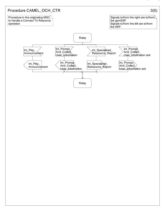
Figure 4.24-3: Procedure CAMEL\_OCH\_CTR (sheet 3)
