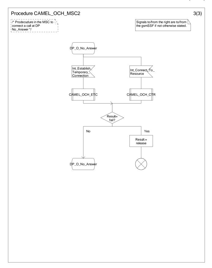
Figure 4.17-3: Procedure CAMEL\_OCH\_MSC2 (sheet 3)
