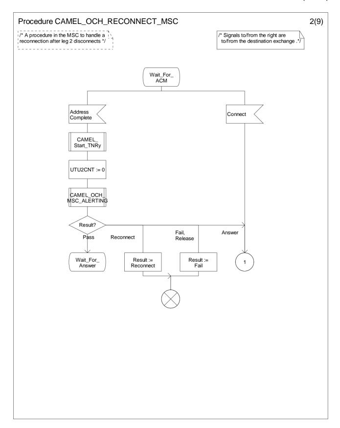
Figure 4.33-2: Procedure CAMEL\_OCH\_RECONNECT\_MSC (sheet 2)
