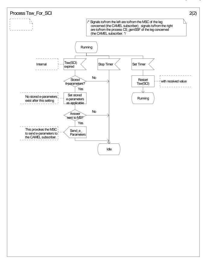
Figure 4.98-2: Process Tsw\_For\_SCI (sheet 2)
