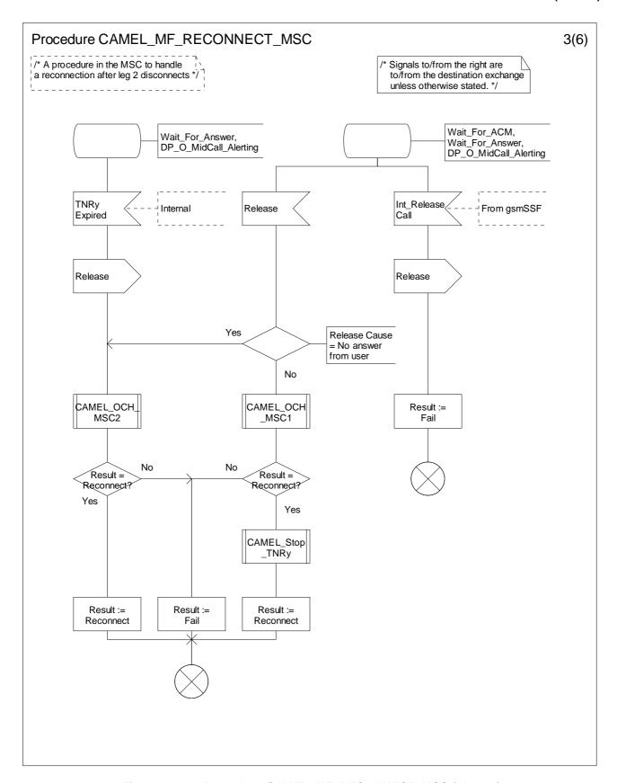
Figure 4.88-3: Procedure CAMEL\_MF\_RECONNECT\_MSC (sheet 3)
