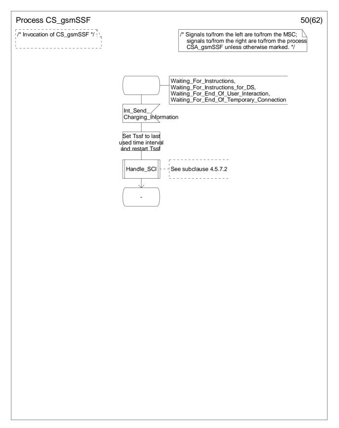
Figure 4.99-50: Process CS\_gsmSSF (sheet 50)
