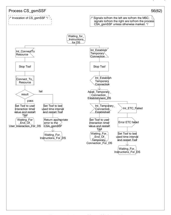
Figure 4.99-56: Process CS\_gsmSSF (sheet 56)
