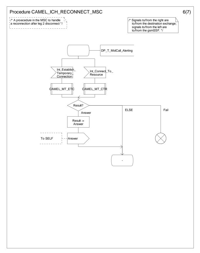
Figure 4.74-6: Procedure CAMEL\_ICH\_RECONNECT\_MSC (sheet 6)
