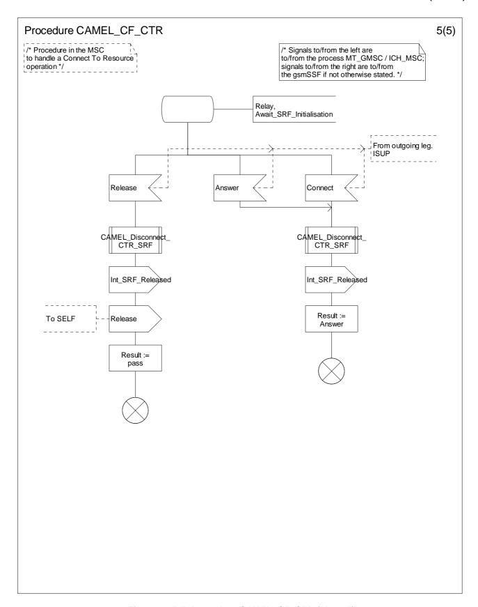
Figure 4.85-5: Procedure CAMEL\_CF\_CTR (sheet 5)
