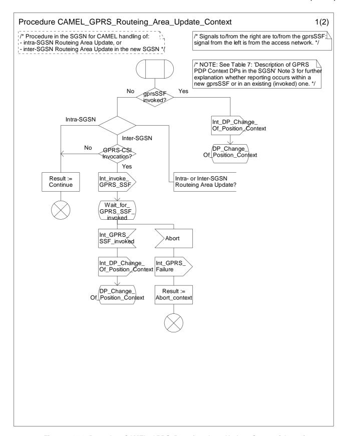
Figure 6.11-1: Procedure CAMEL\_GPRS\_Routeing\_Area\_Update\_Context (sheet 1)
