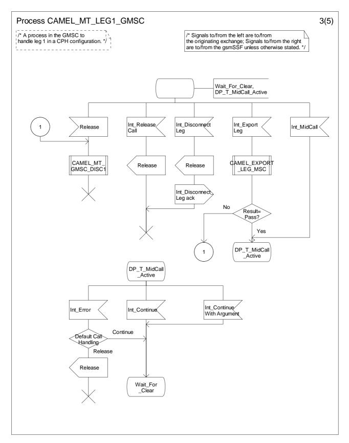
Figure 4.55-3: Process CAMEL\_MT\_LEG1\_GMSC (sheet 3)
