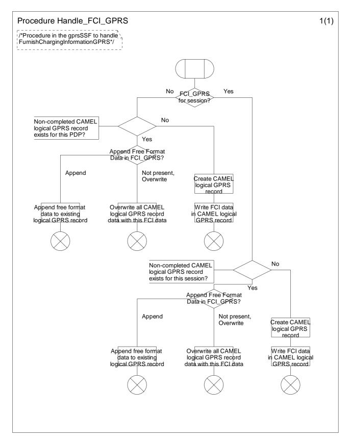
Figure 6.21-1: Procedure Handle\_FCI\_GPRS (sheet 1)
