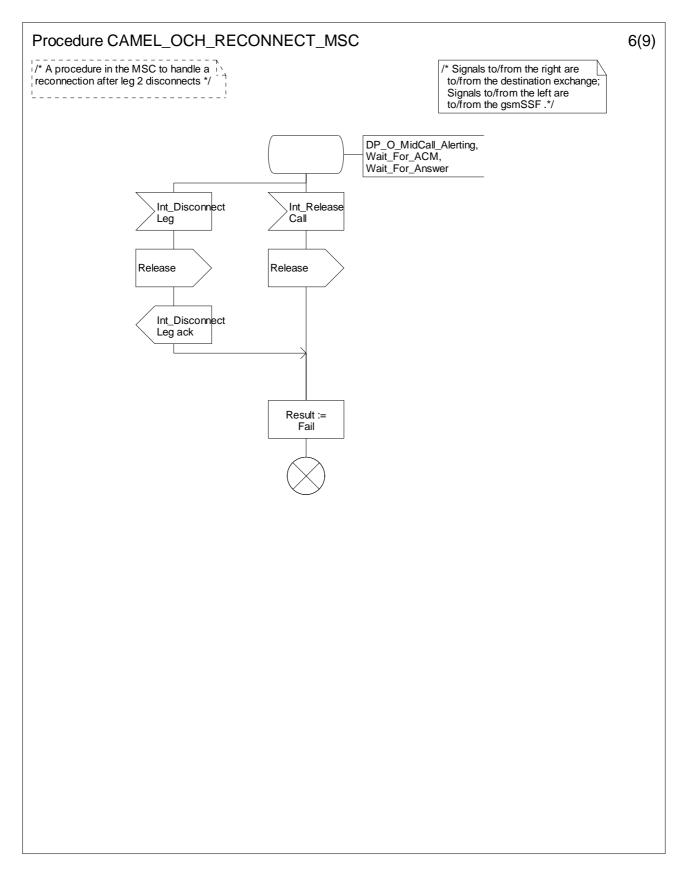
Figure 4.33-6: Procedure CAMEL\_OCH\_RECONNECT\_MSC (sheet 6)
