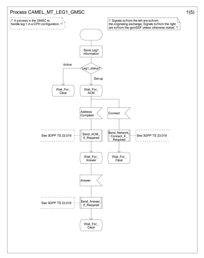
Figure 4.55-1: Process CAMEL\_MT\_LEG1\_GMSC (sheet 1)
