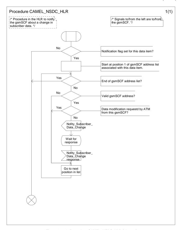
Figure 10.9-1: Procedure CAMEL\_NSDC\_HLR (sheet 1)
