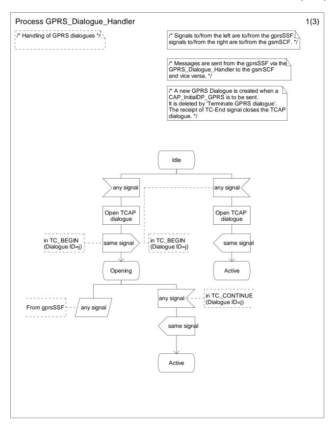
Figure 6.18-1: Process GPRS\_Dialogue\_Handler (sheet 1)
