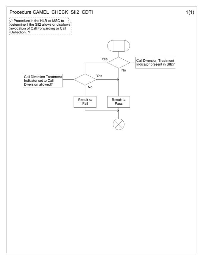
Figure 4.63-1: Procedure CAMEL\_CHECK\_SII2\_CDTI (sheet 1)
