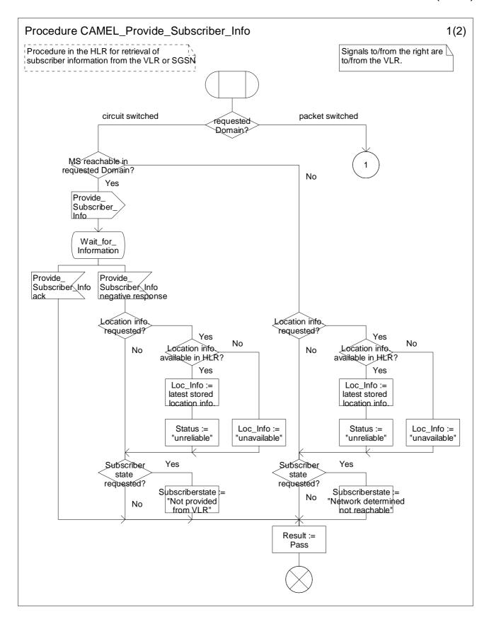
Figure 4.119-1: Procedure CAMEL\_Provide\_Subscriber\_Info (sheet 1)
