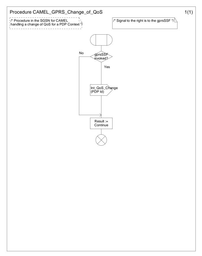
Figure 6.14-1: Procedure CAMEL\_GPRS\_Change\_Of\_QoS (sheet 1)
