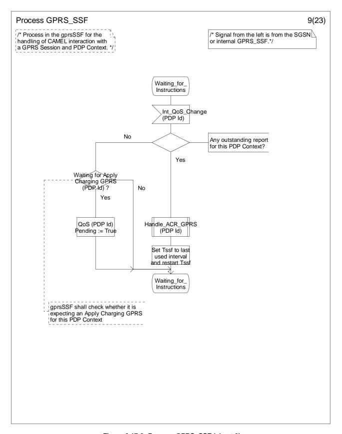
Figure 6.17-9: Process GPRS\_SSF (sheet 9)
