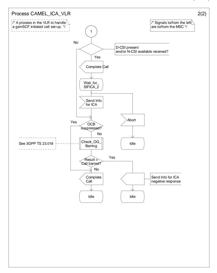
Figure 4.95-2: Process CAMEL\_ICA\_VLR (sheet 2)
