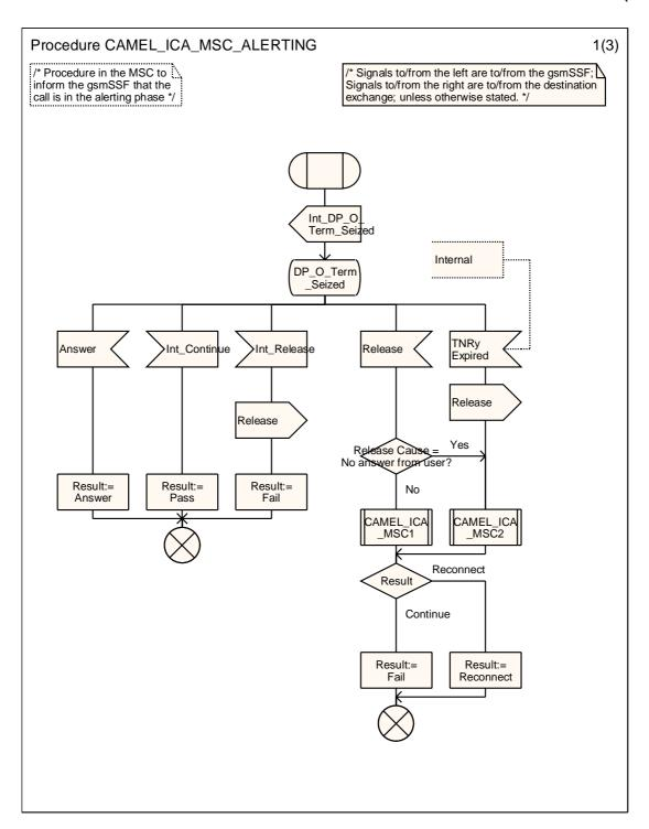
Figure 4.90-1: Procedure CAMEL\_ICA\_MSC\_ALERTING (sheet 1)
