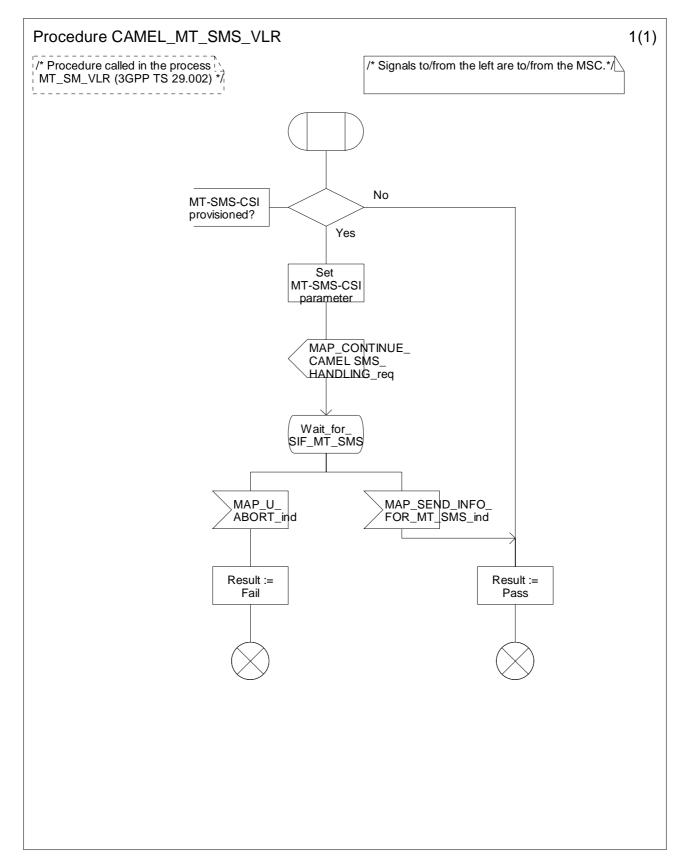
Figure 7.13-1: Procedure CAMEL\_MT\_SMS\_VLR (sheet 1)
