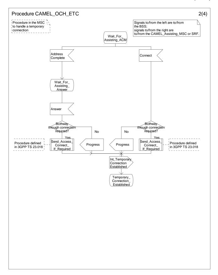
Figure 4.23-2: Procedure CAMEL\_OCH\_ETC (sheet 2)
