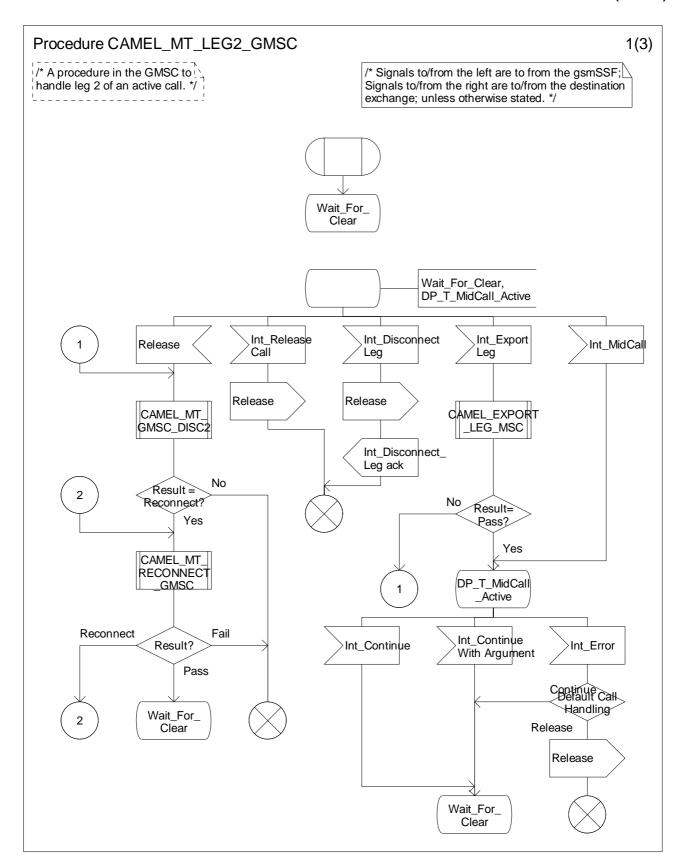
Figure 4.54-1: Procedure CAMEL\_MT\_LEG2\_GMSC (sheet 1)
