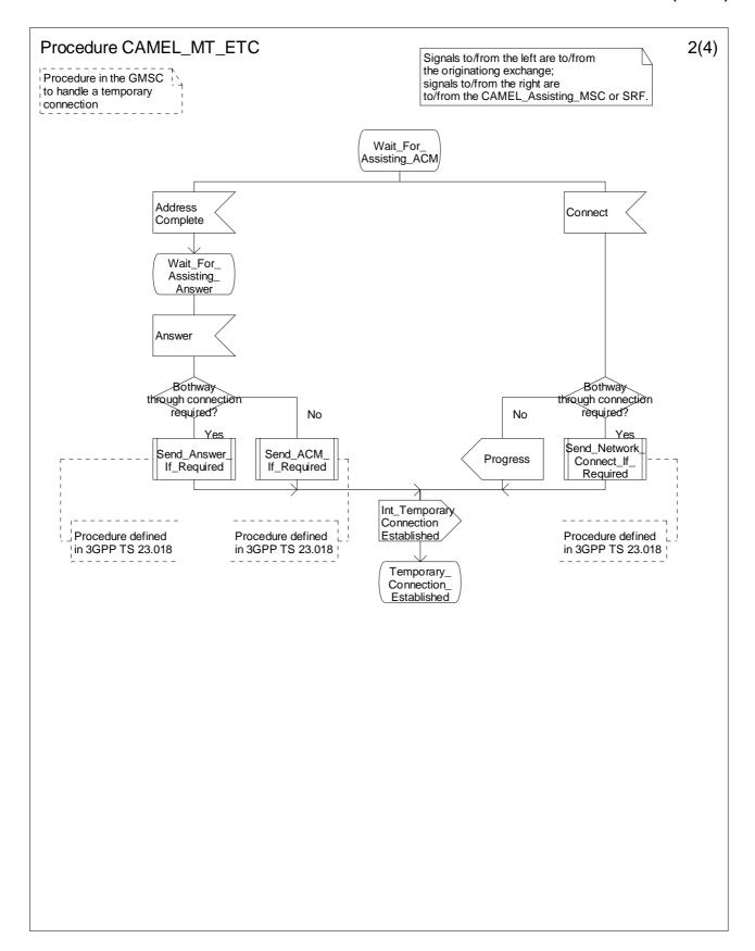
Figure 4.51-2: Procedure CAMEL\_MT\_ETC (sheet 2)
