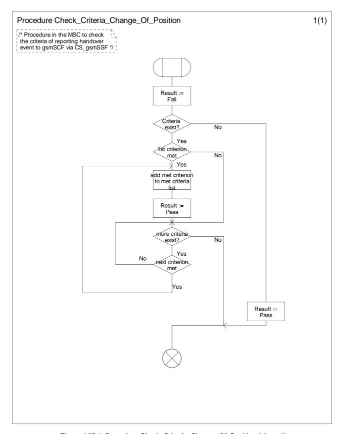
Figure 4.37-1: Procedure Check\_Criteria\_Change\_Of\_Position (sheet 1)
