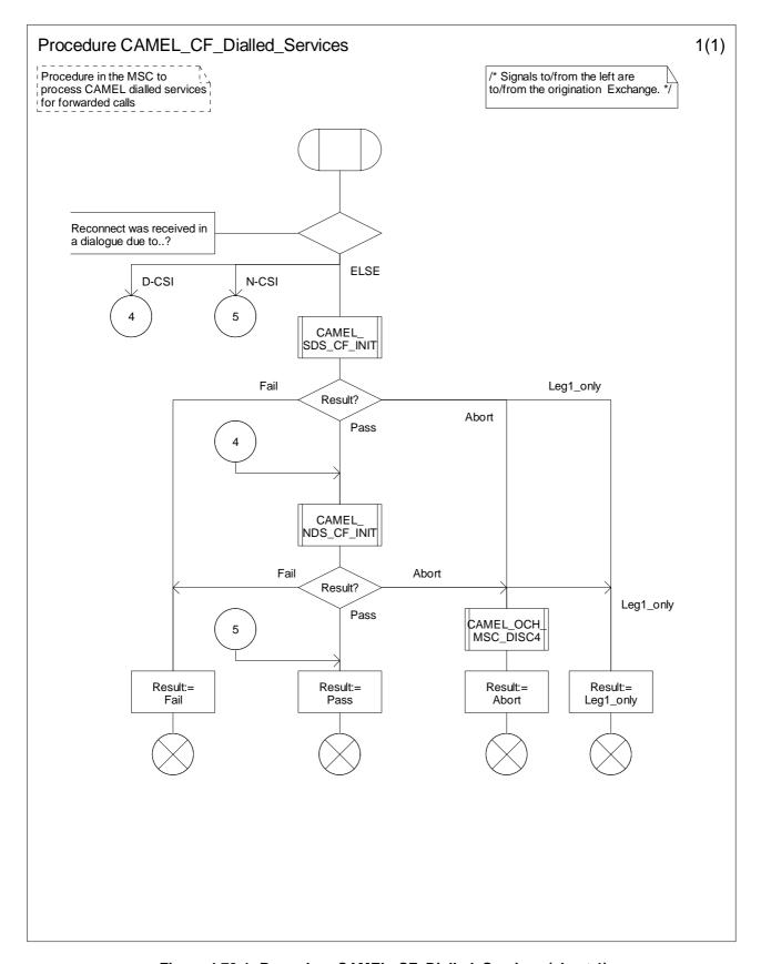
Figure 4.78-1: Procedure CAMEL\_CF\_Dialled\_Services (sheet 1)
