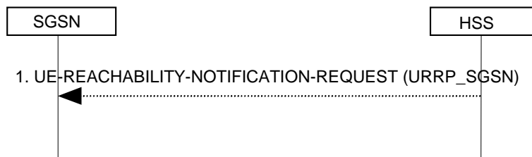
Figure 6.15-1: UE Reachability Notification Request Procedure
