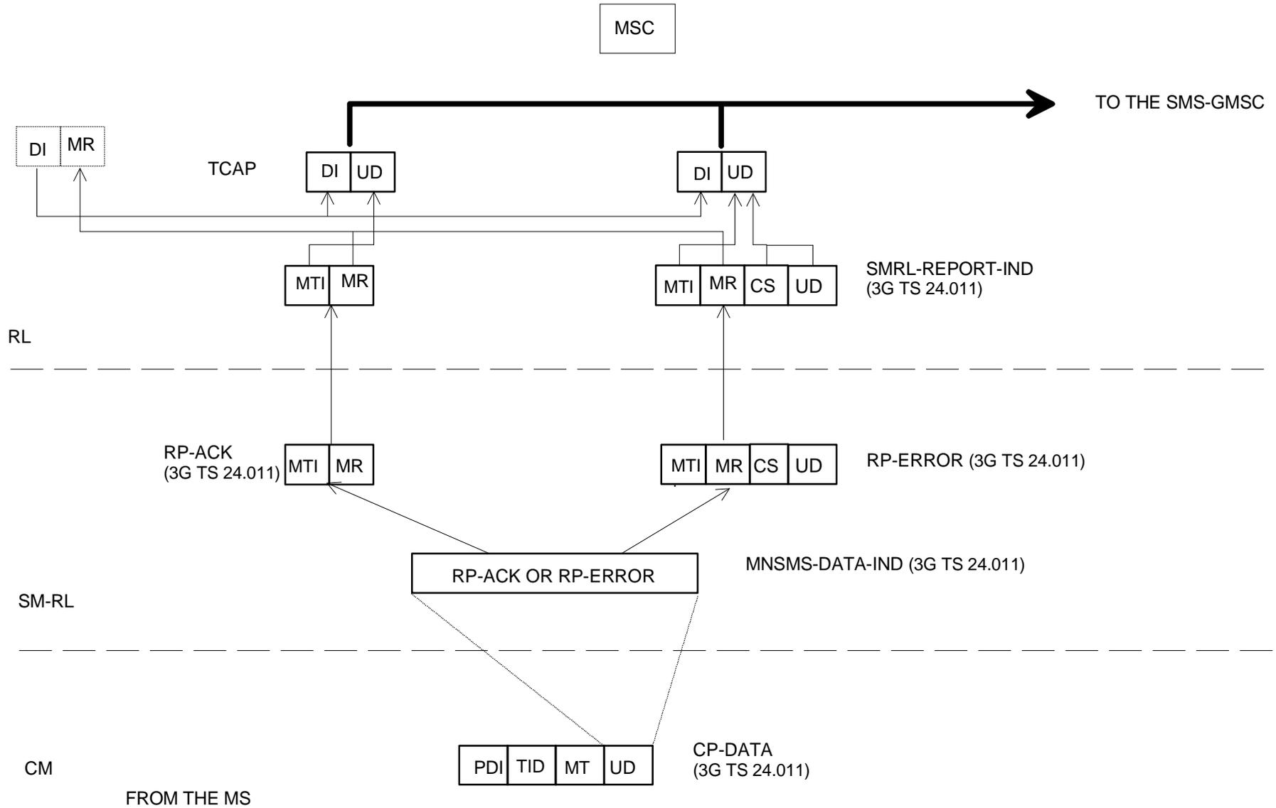
NOTE: The cause carried via UD of TCAP is not the cause supplied via RP-ERROR but is the cause resulting from application of the mapping specified by table 8.5 of 24.011[13].
