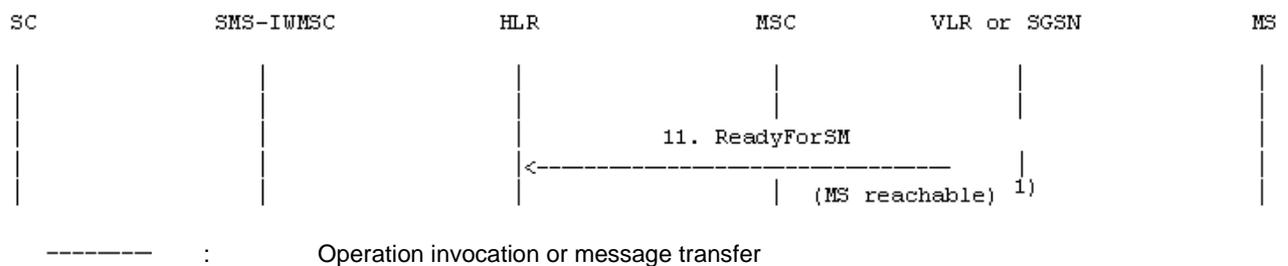
NOTE 1): In case ReadyForSM is sent by the SGSN, the reason may be MS reachable via the SGSN, or MS reachable via the SGSN and the MSC (see 3GPP TS 23.060 [27]).
