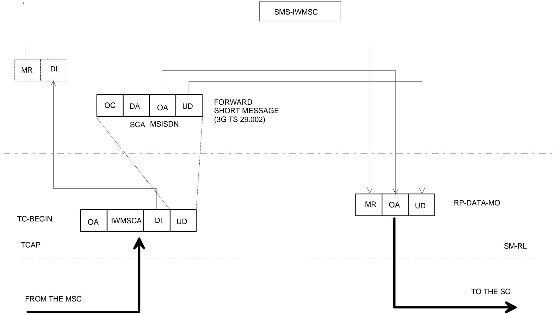
NOTE: MR is of local significance to the IW MSC/SC interface and is not the value supplied by the MS via the MS/MSC interface.
