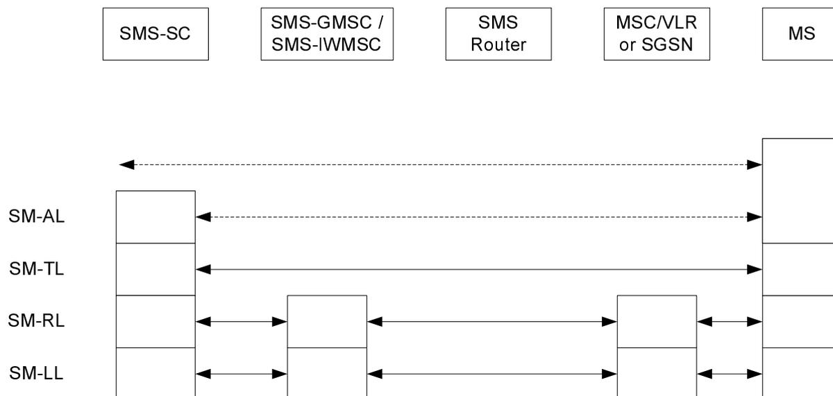
NOTE: The SMS Router is an optional functional entity, and is used only in the MT case.
