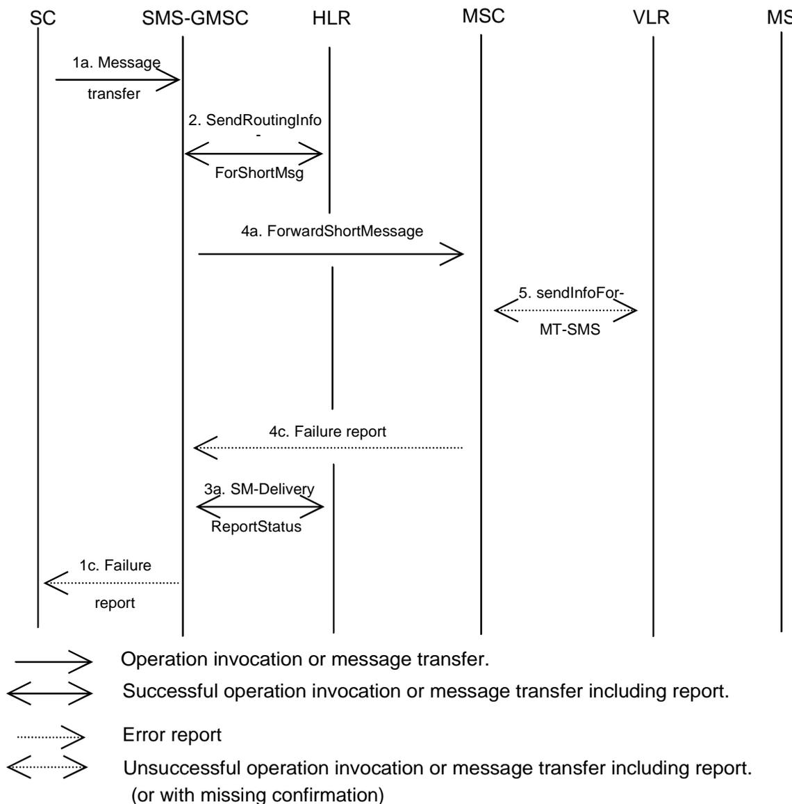
NOTE: If an SMS Router is present, the message flow in 15aa is used, except that a 4c Failure Report message is transparently transferred to the SMS-GMSC from the MSC or SGSN by the SMS Router instead of a 4b Delivery Report.
