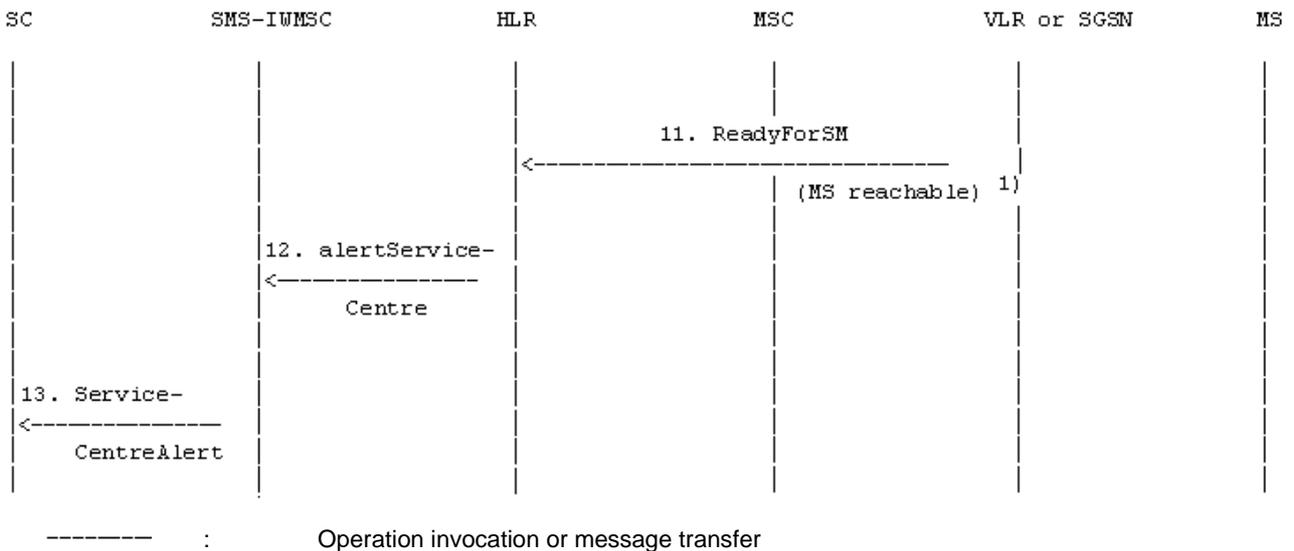
NOTE 1): In case ReadyForSM is sent by the SGSN, the reason may be MS reachable via the SGSN, or MS reachable via the SGSN and the MSC (see 3GPP TS 23.060 [27]).
