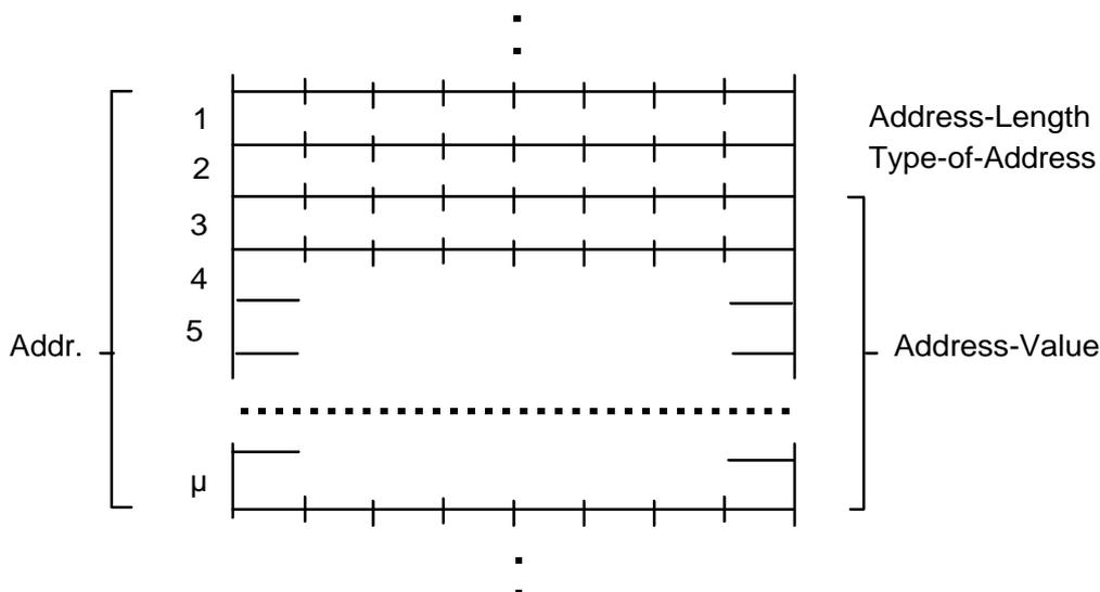
The Address-Length field is an integer representation of the number of useful semi-octets within the Address-Value field, i.e. excludes any semi octet containing only fill bits.
