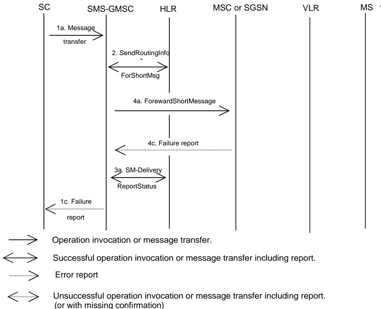
NOTE: If an SMS Router is present, the message flow in 15aa is used, except that a 4c Failure Report message is transparently transferred to the SMS-GMSC from the MSC or SGSN by the SMS Router instead of a 4b Delivery Report.
