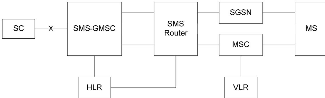
NOTE 1: The SMS Router is an optional entity. If it is not present, the two interfaces extending from the right side of the SMS-GMSC extend directly to the SGSN and MSC, respectively.
