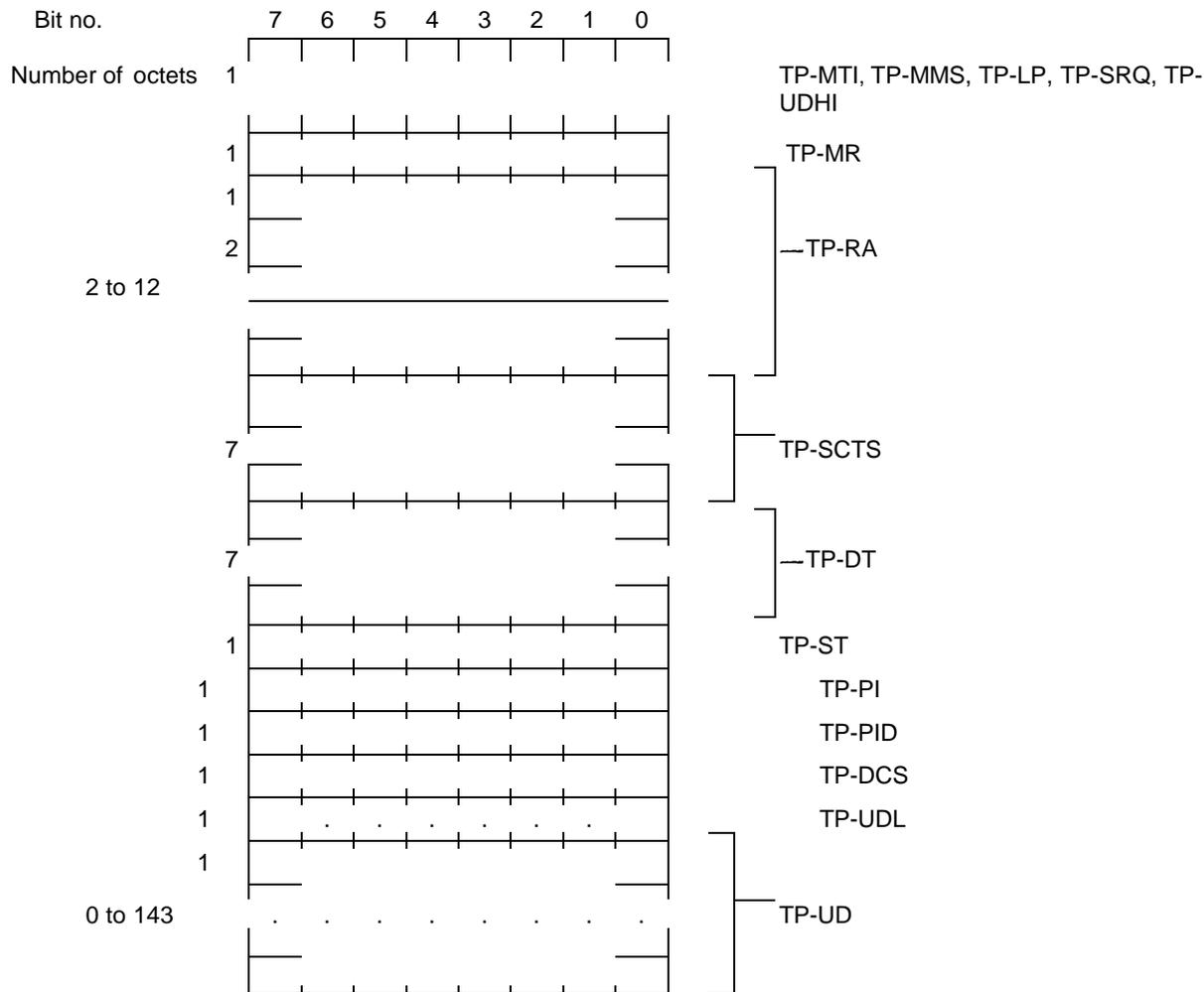
NOTE: Any unused bits shall be set to zero by the sending entity and shall be ignored by the receiving entity.
