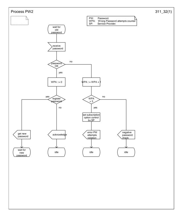
Figure 3.2: PW2; Check of password input (HLR)
