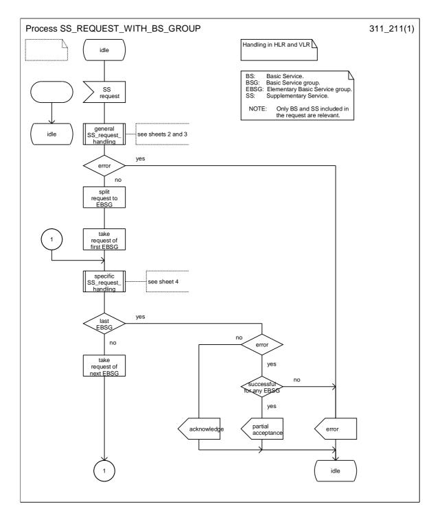
Figure 2.1 (sheet 1 of 4): Handling of call independent SS procedures with respect to basic service groups
