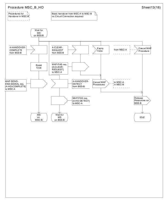
Figure 42 (Sheet 13 of 18): Handover control procedure in MSC-B
