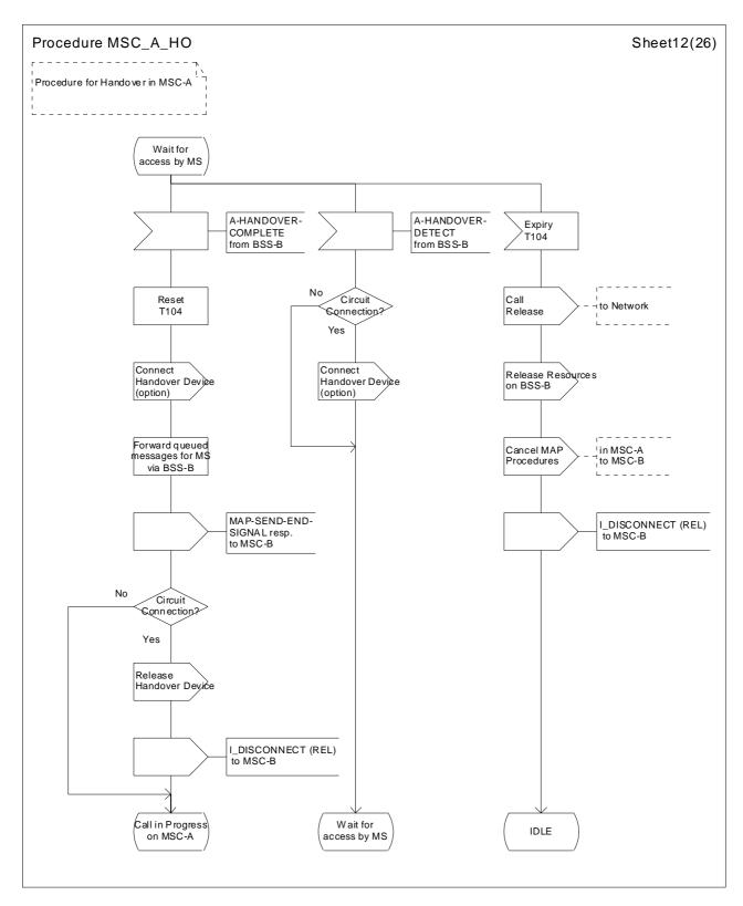
Figure 41 (Sheet 12 of 26): Handover control procedure in MSC-A
