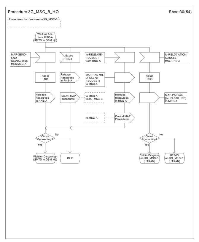
Figure 44 (sheet 30 of 54): Handover control procedure in 3G\_MSC-B
