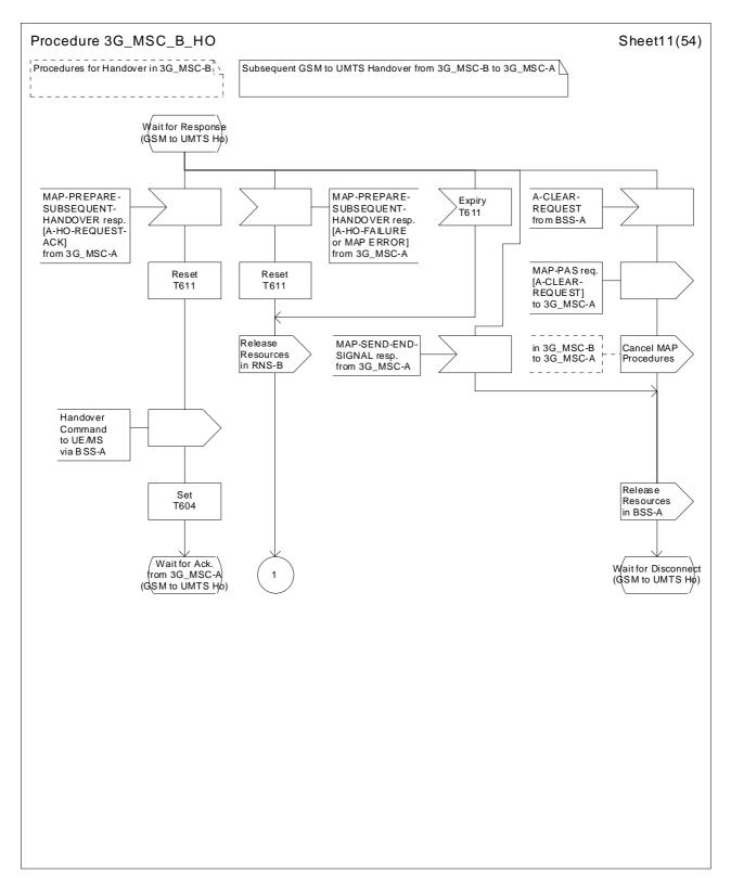
Figure 44 (sheet 11 of 54): Handover control procedure in 3G\_MSC-B
