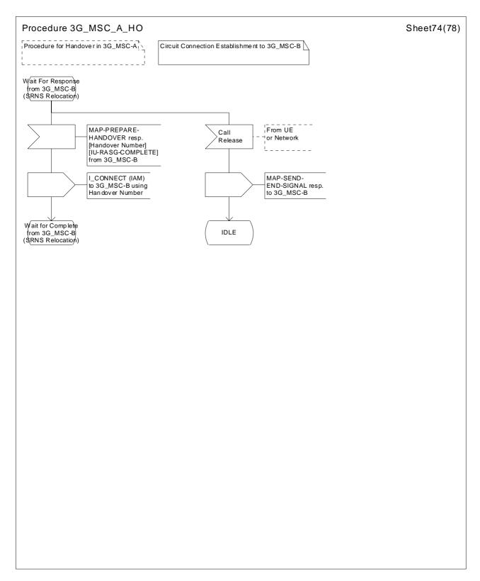
Figure 43 (sheet 74 of 78): Handover control procedure in 3G\_MSC-A
