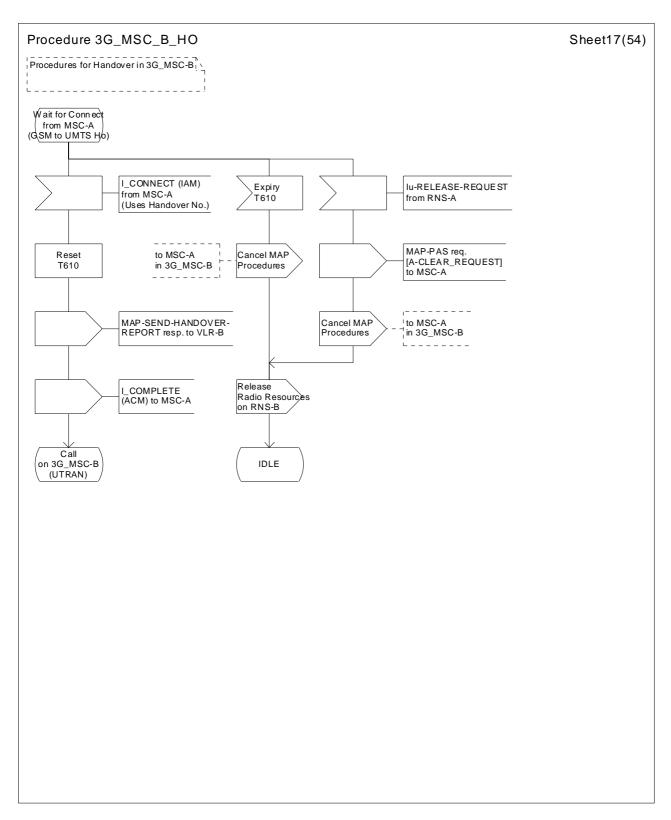
Figure 44 (sheet 17 of 54): Handover control procedure in 3G\_MSC-B
