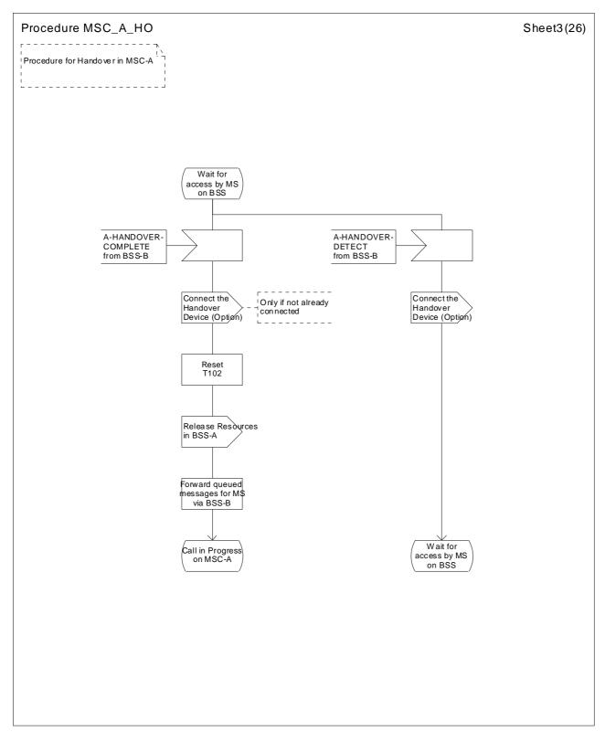
Figure 41 (Sheet 3 of 26): Handover control procedure in MSC-A
