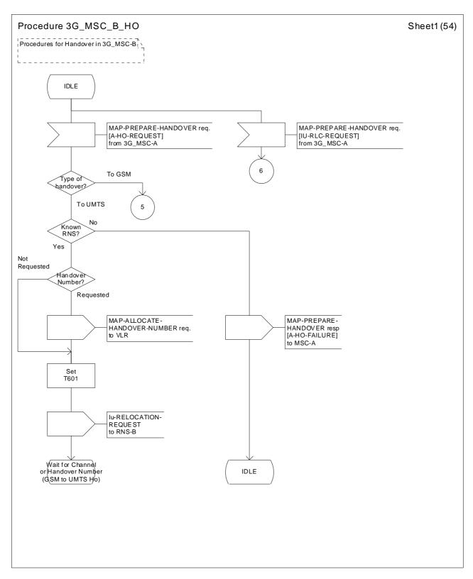
Figure 44 (sheet 1 of 54): Handover control procedure in 3G\_MSC-B
