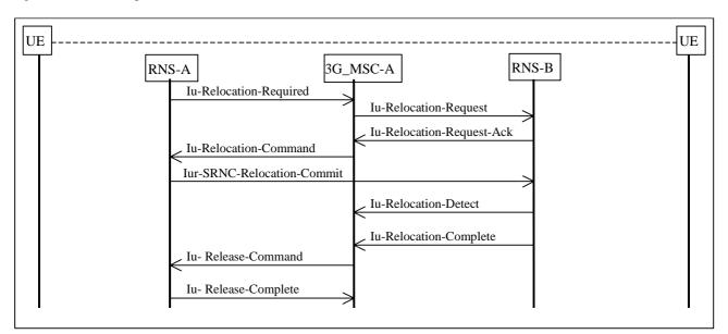
Figure 10 Basic intra-3G\_MSC SRNS Relocation Procedure
