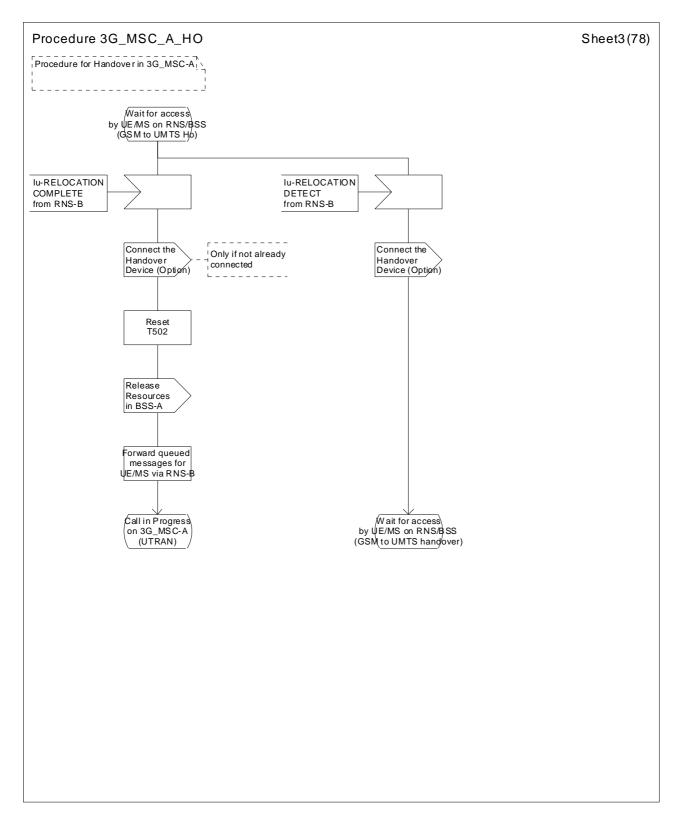
Figure 43 (sheet 3 of 78): Handover control procedure in 3G\_MSC-A
