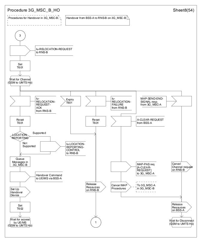
Figure 44 (sheet 8 of 54): Handover control procedure in 3G\_MSC-B
