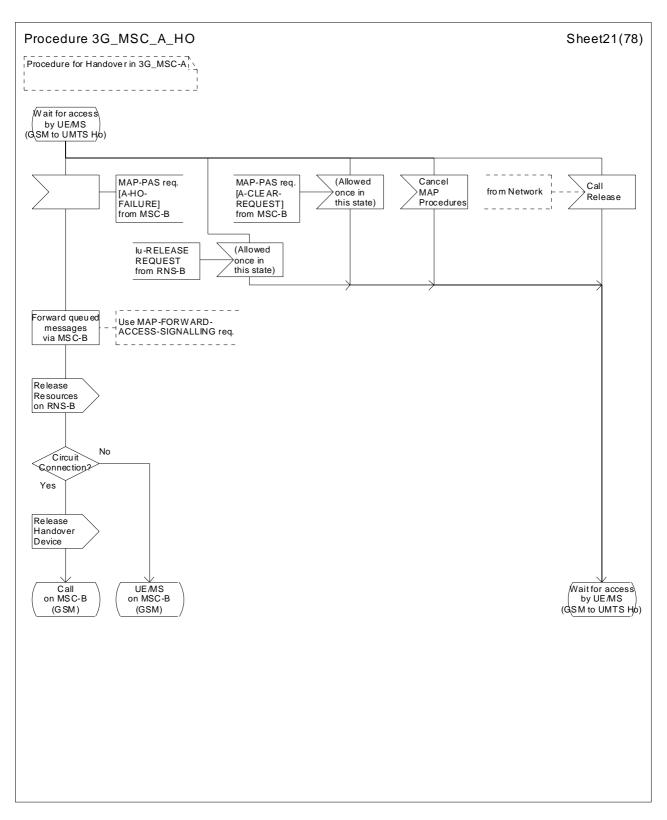
Figure 43 (sheet 21 of 78): Handover control procedure in 3G\_MSC-A
