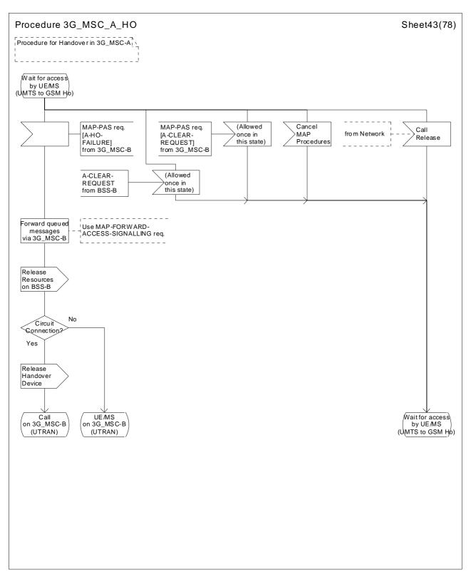
Figure 43 (sheet 43 of 78): Handover control procedure in 3G\_MSC-A
