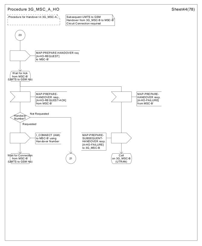
Figure 43 (sheet 44 of 78): Handover control procedure in 3G\_MSC-A
