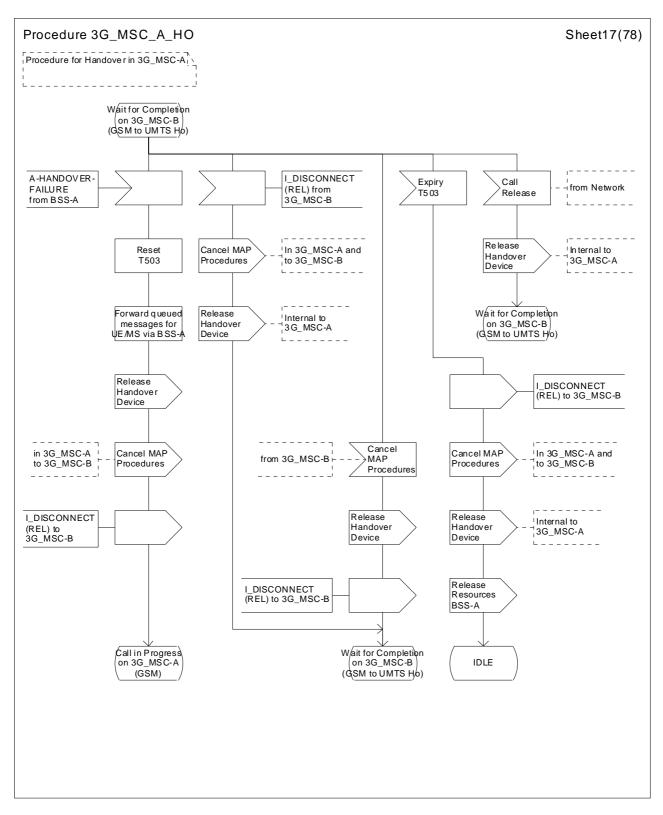
Figure 43 (sheet 17 of 78): Handover control procedure in 3G\_MSC-A
