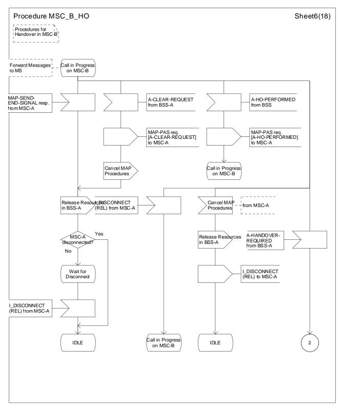
Figure 42 (Sheet 6 of 18): Handover control procedure in MSC-B
