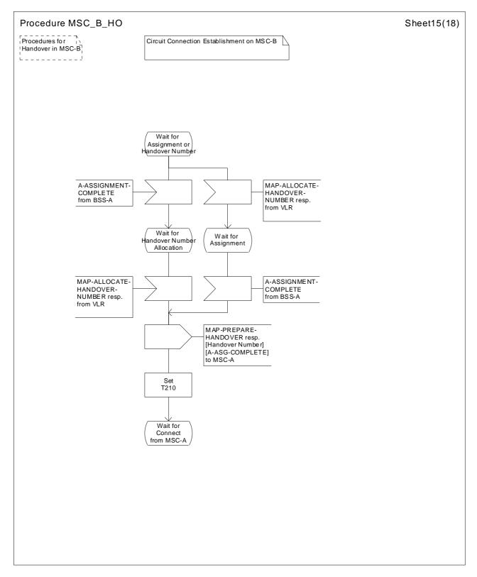
Figure 42 (Sheet 15 of 18): Handover control procedure in MSC-B
