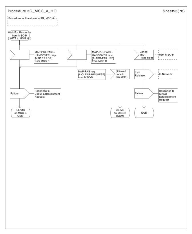
Figure 43 (sheet 53 of 78): Handover control procedure in 3G\_MSC-A
