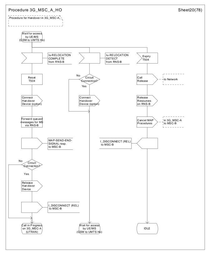
Figure 43 (sheet 20 of 78): Handover control procedure in 3G\_MSC-A
