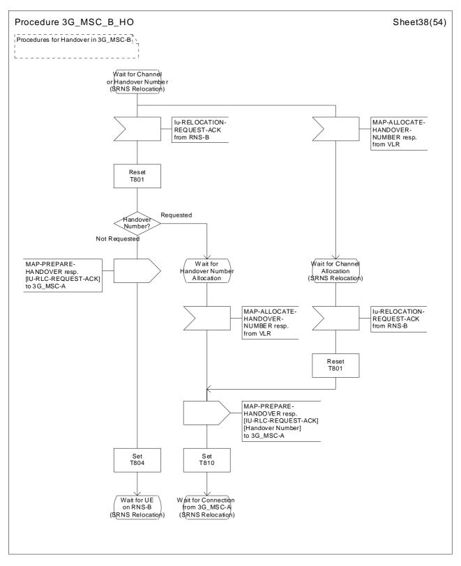
Figure 44 (sheet 38 of 54): Handover control procedure in 3G\_MSC-B
