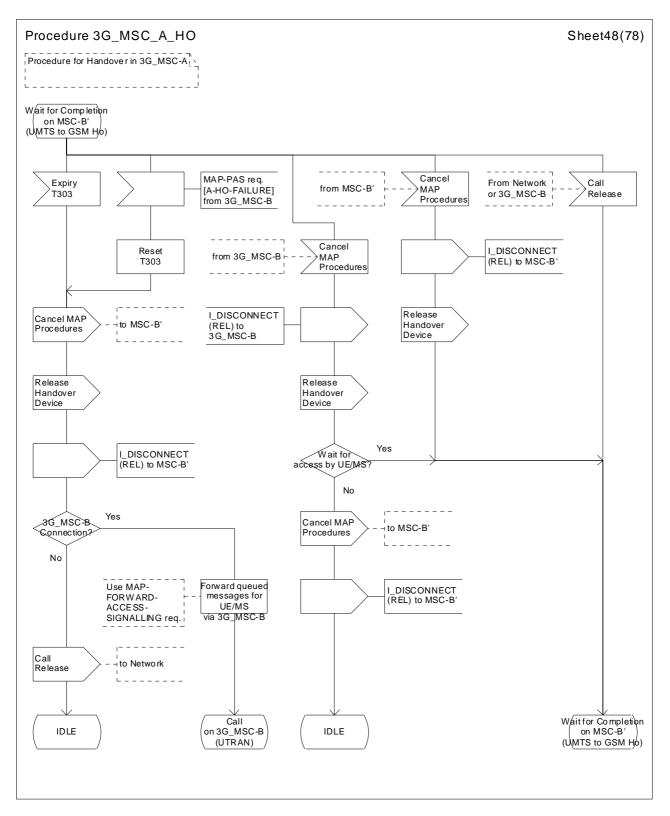
Figure 43 (sheet 48 of 78): Handover control procedure in 3G\_MSC-A
