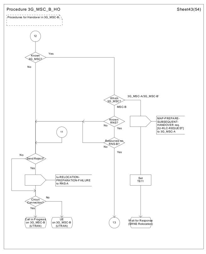
Figure 44 (sheet 43 of 54): Handover control procedure in 3G\_MSC-B
