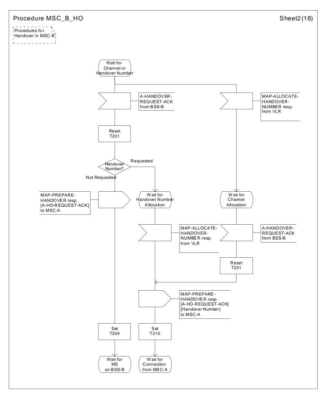
Figure 42 (Sheet 2 of 18): Handover control procedure in MSC-B
