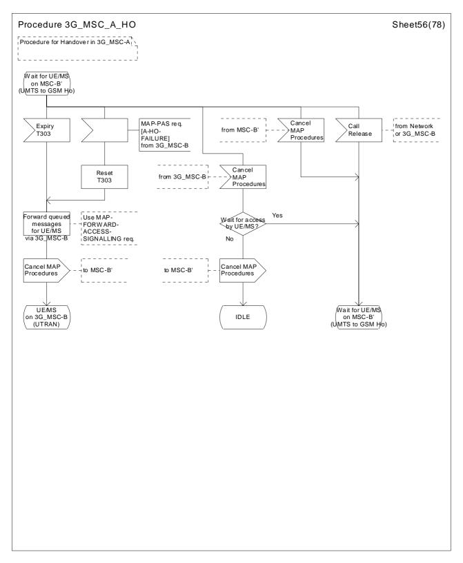
Figure 43 (sheet 56 of 78): Handover control procedure in 3G\_MSC-A
