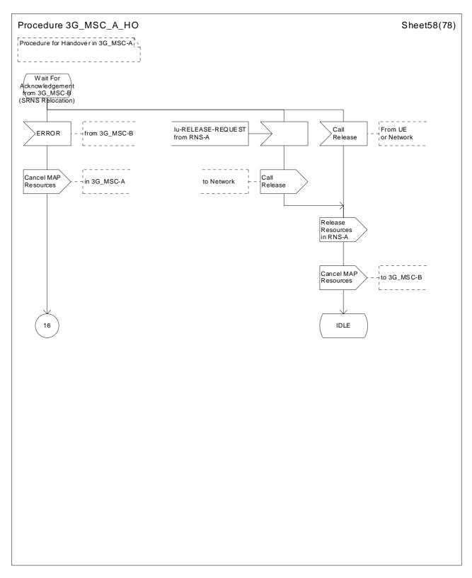
Figure 43 (sheet 58 of 78): Handover control procedure in 3G\_MSC-A
