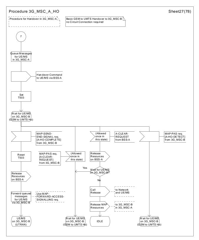
Figure 43 (sheet 27 of 78): Handover control procedure in 3G\_MSC-A
