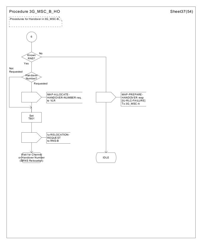
Figure 44 (sheet 37 of 54): Handover control procedure in 3G\_MSC-B
