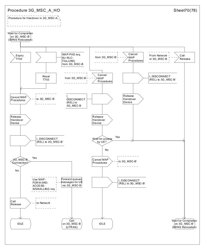
Figure 43 (sheet 70 of 78): Handover control procedure in 3G\_MSC-A
