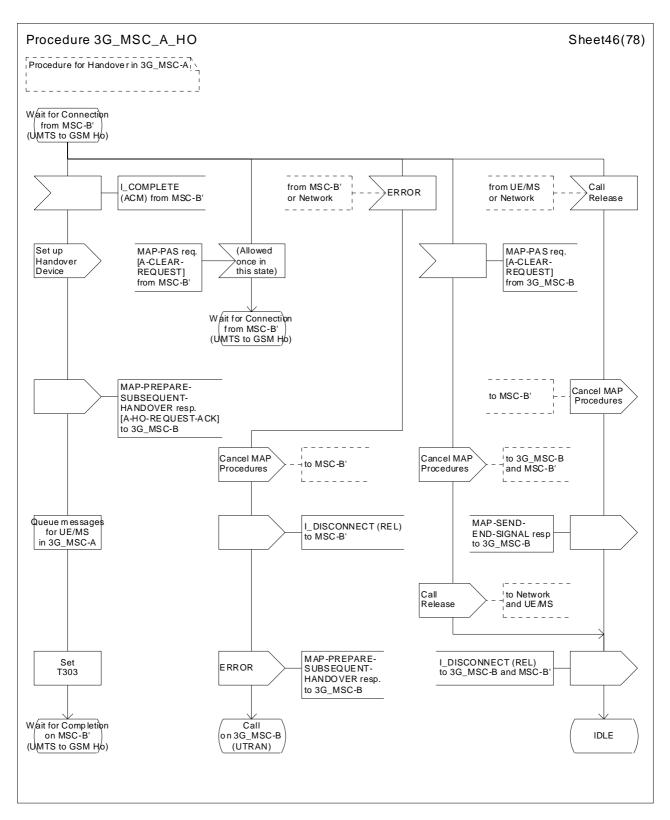
Figure 43 (sheet 46 of 78): Handover control procedure in 3G\_MSC-A
