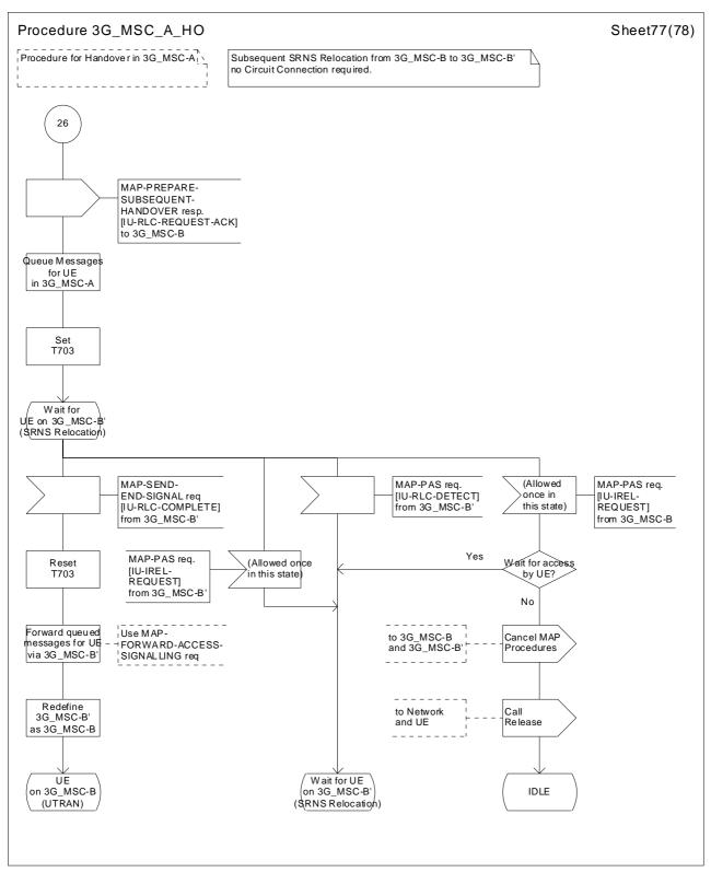
Figure 43 (sheet 77 of 78): Handover control procedure in 3G\_MSC-A
