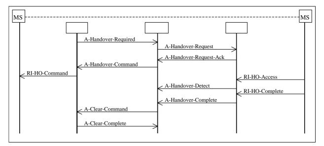
Figure 7: Basic External Intra-MSC Handover Procedure
