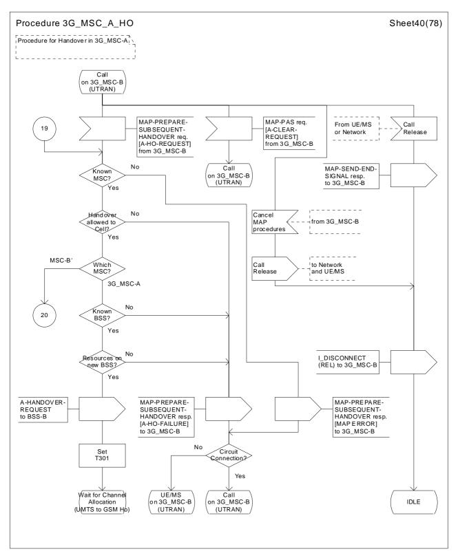
Figure 43 (sheet 40 of 78): Handover control procedure in 3G\_MSC-A
