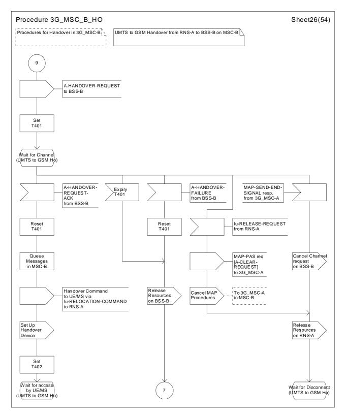
Figure 44 (sheet 26 of 54): Handover control procedure in 3G\_MSC-B
