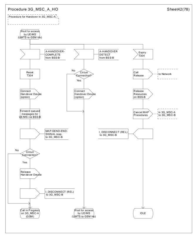
Figure 43 (sheet 42 of 78): Handover control procedure in 3G\_MSC-A
