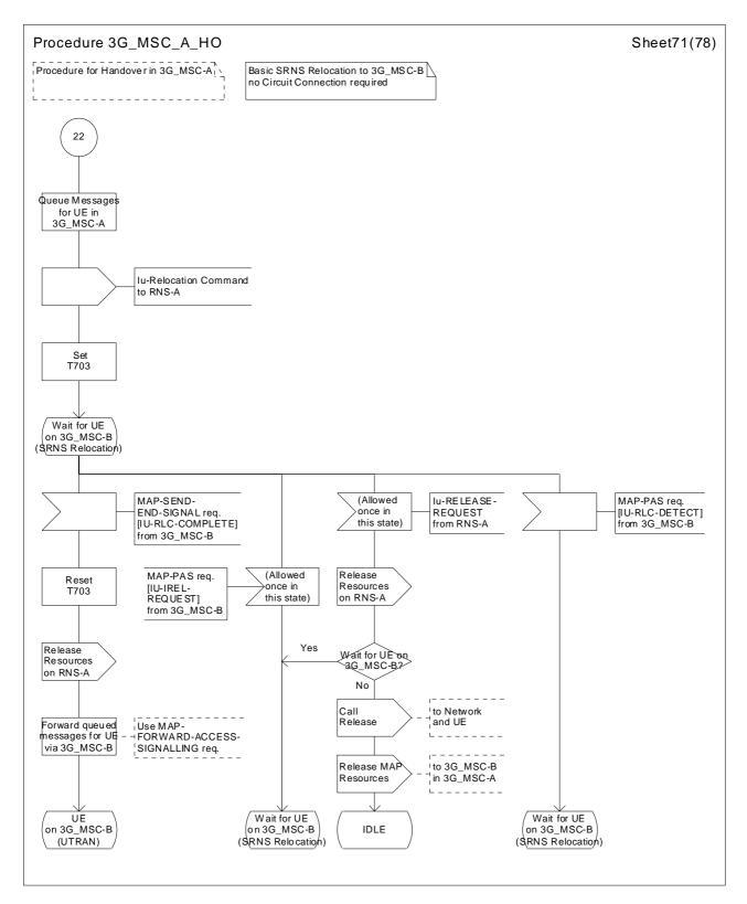
Figure 43 (sheet 71 of 78): Handover control procedure in 3G\_MSC-A
