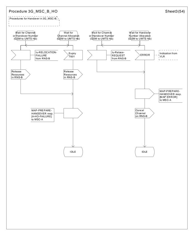
Figure 44 (sheet 3 of 54): Handover control procedure in 3G\_MSC-B
