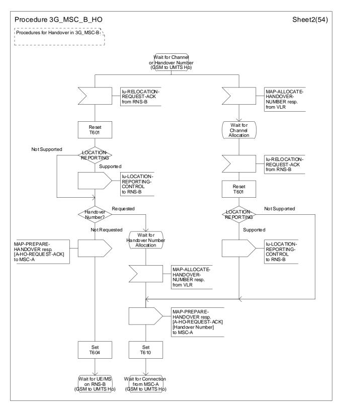
Figure 44 (sheet 2 of 54): Handover control procedure in 3G\_MSC-B
