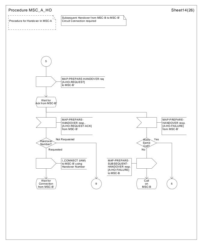
Figure 41 (Sheet 14 of 26): Handover control procedure in MSC-A
