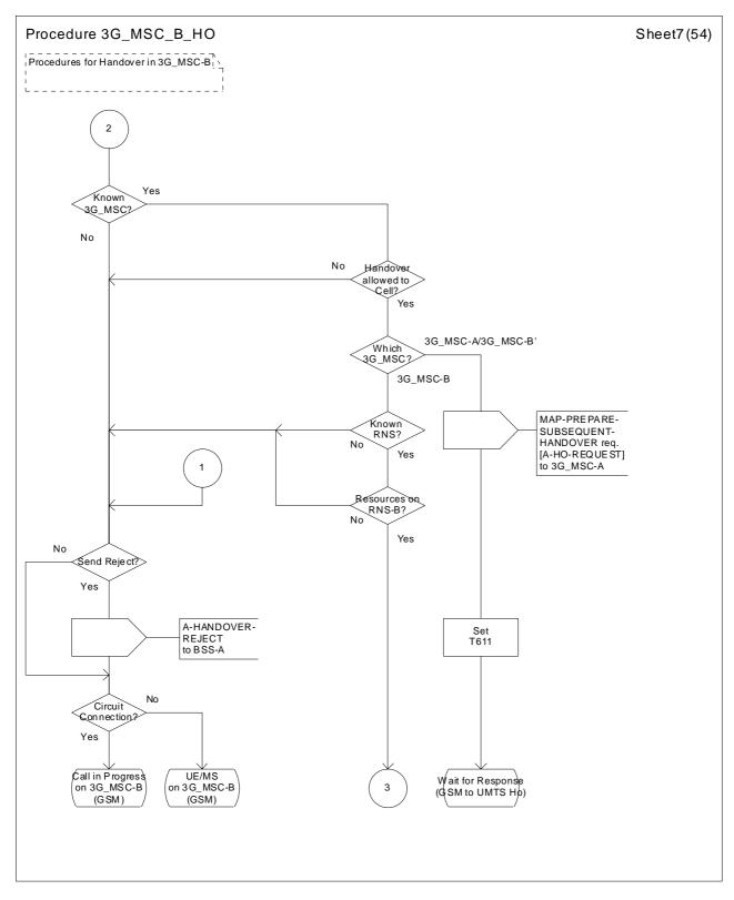
Figure 44 (sheet 7 of 54): Handover control procedure in 3G\_MSC-B
