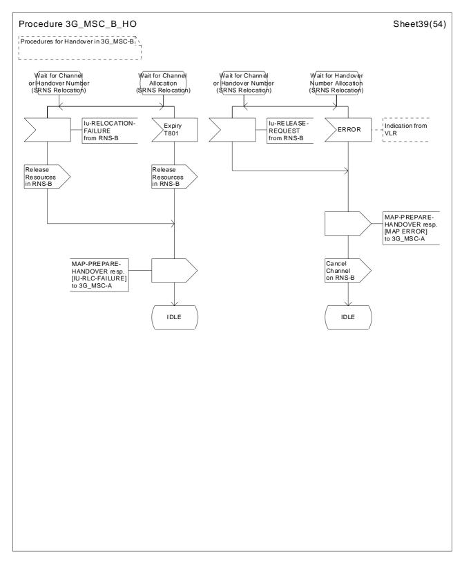
Figure 44 (sheet 39 of 54): Handover control procedure in 3G\_MSC-B
