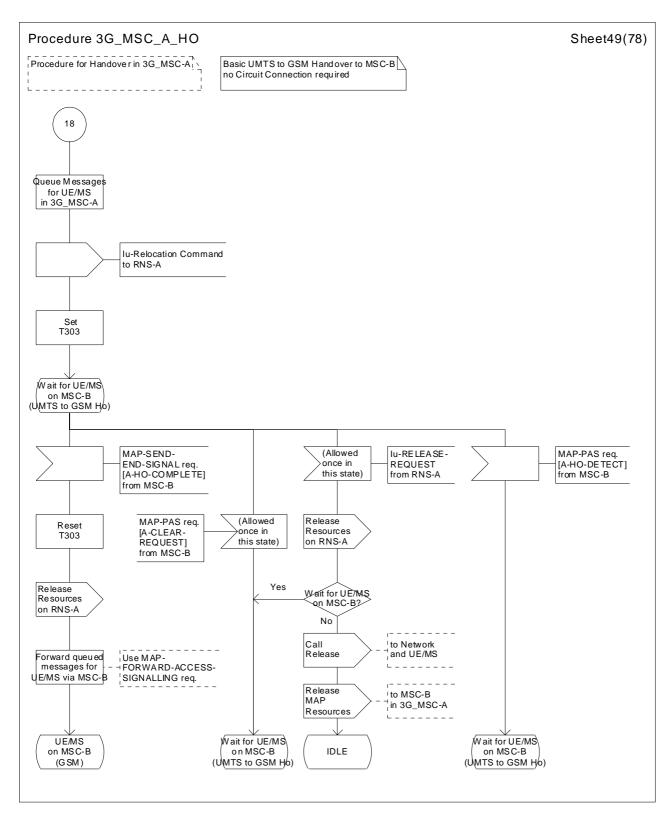
Figure 43 (sheet 49 of 78): Handover control procedure in 3G\_MSC-A
