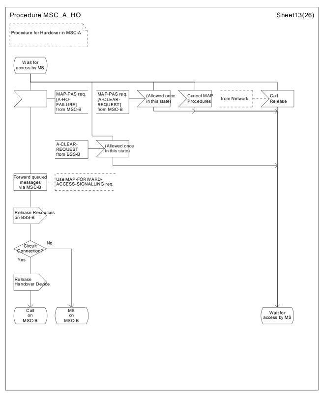
Figure 41 (Sheet 13 of 26): Handover control procedure in MSC-A
