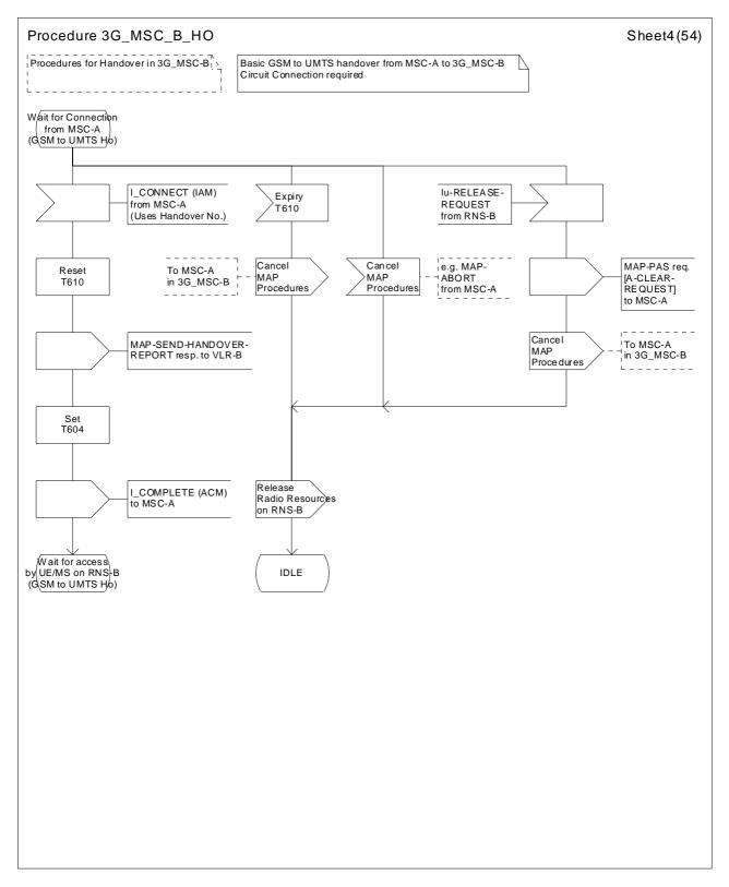
Figure 44 (sheet 4 of 54): Handover control procedure in 3G\_MSC-B
