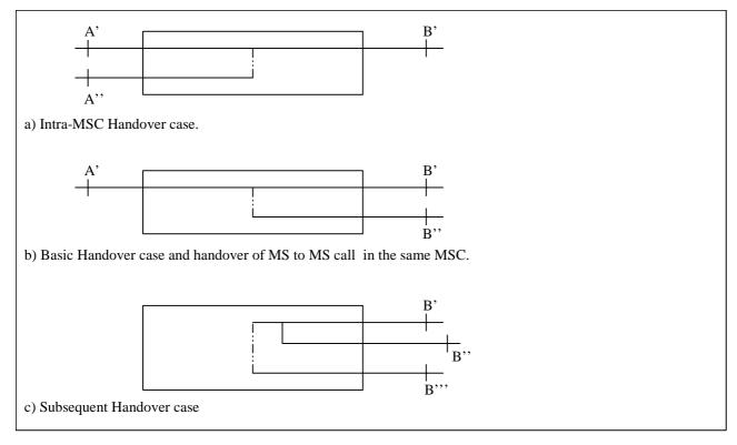
NOTE: In a) and b) A' is released after handover; In c) B" is released after handover.
