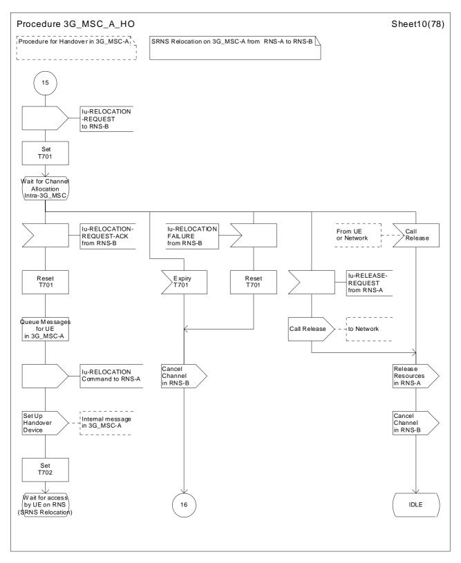
Figure 43 (sheet 10 of 78): Handover control procedure in 3G\_MSC-A
