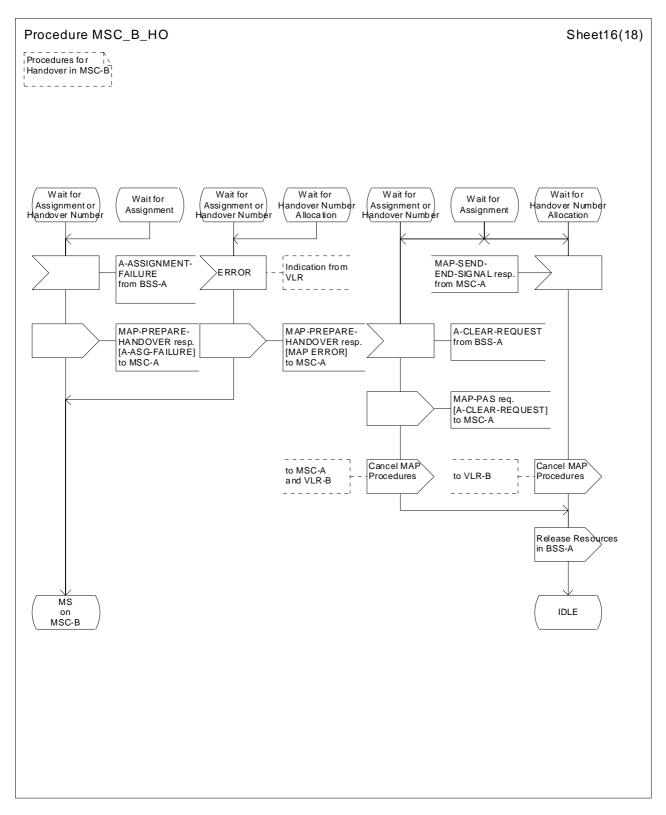
Figure 42 (Sheet 16 of 18): Handover control procedure in MSC-B
