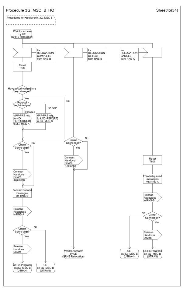
Figure 44 (sheet 45 of 54): Handover control procedure in 3G\_MSC-B
