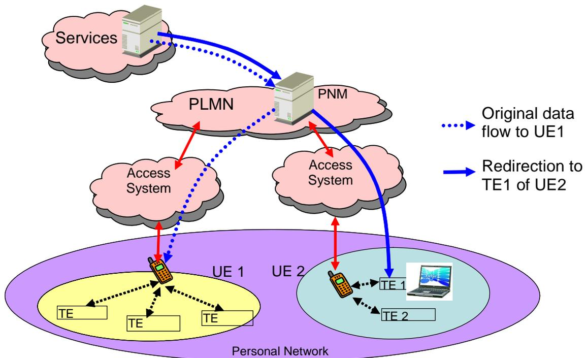
Figure 12: Activating a particular device of a UE or PAN for service termination
