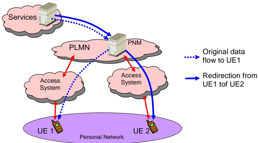
Figure 11: Activation of UE 2 for directing service termination to UE 2
