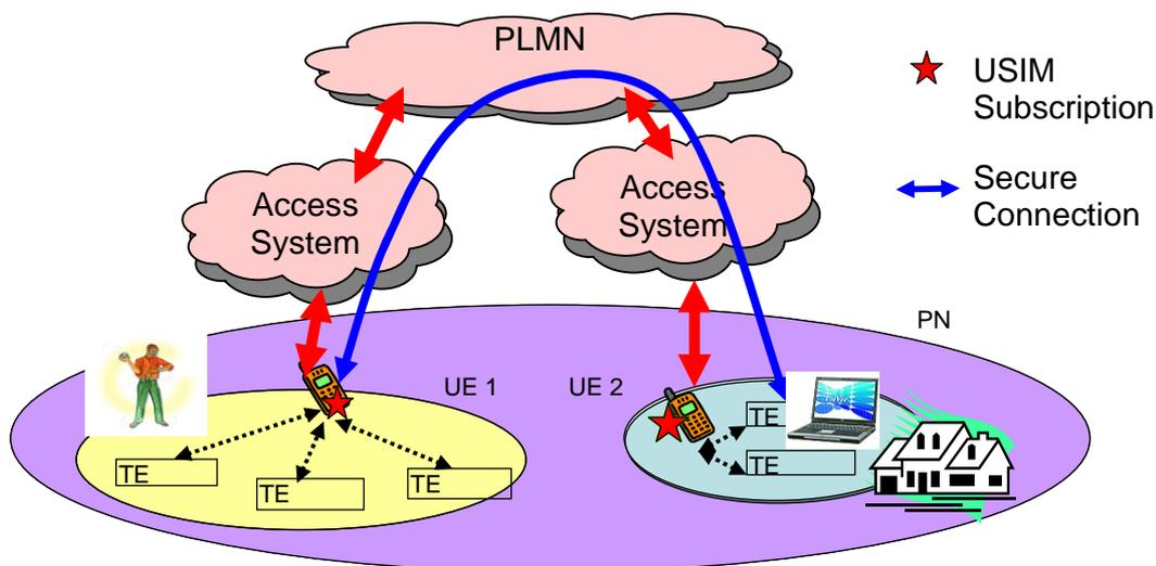
Figure 4: Use case for connection between the devices of a PN
