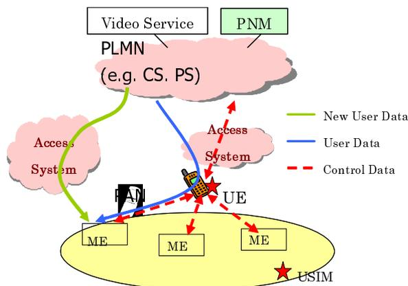
**Figure 9: Multiple network connections through other access system**
