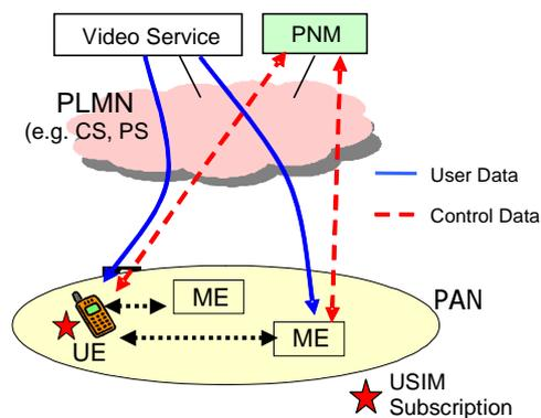
**Figure 8: Multiple network connections through 3GPP access systems**
