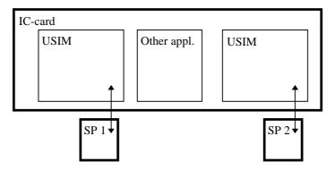
Figure 3 Example of a Multifunction UICC
