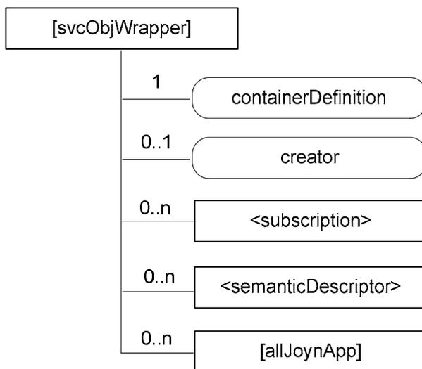
**Figure B.2-1: Structure of [svcObjWrapper] resource**
