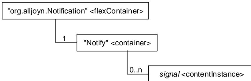
**Figure C.1.1-1: Structure of Notification interface mapping**
