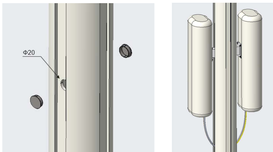
Figure C.4: Side-mounted Schematic Diagram
