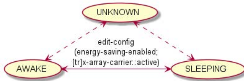
Figure 9.1.3-3: Transition diagram for power-state node
