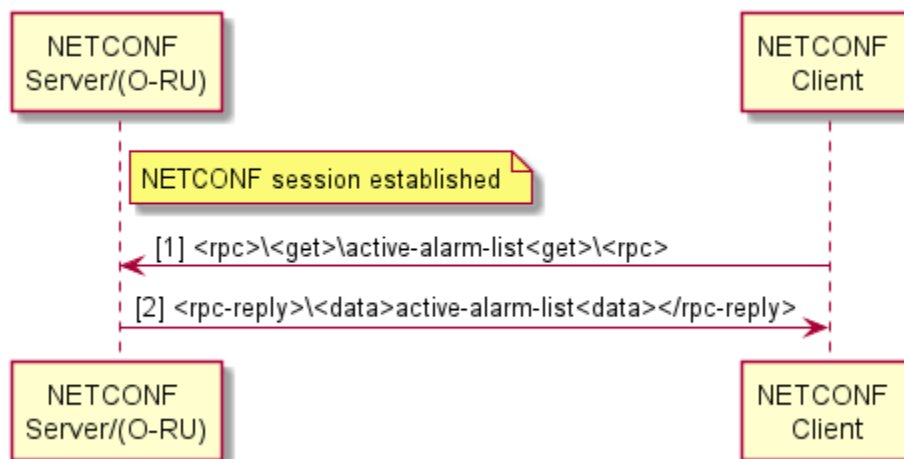
Figure 11.1-1: Read Active Alarms
