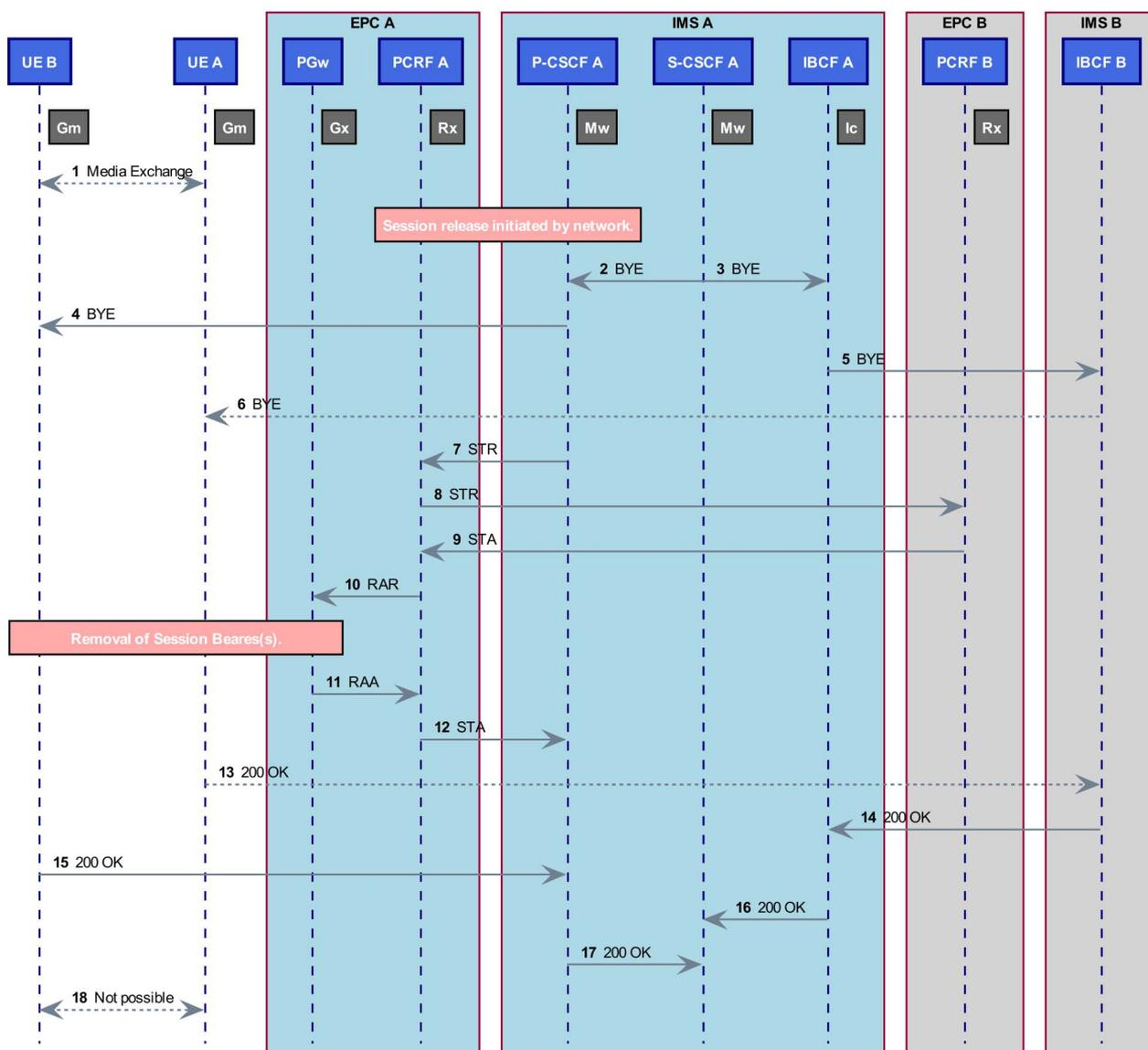
NOTE 1: The Rx exchange need not wait for the Gx exchange to complete.
