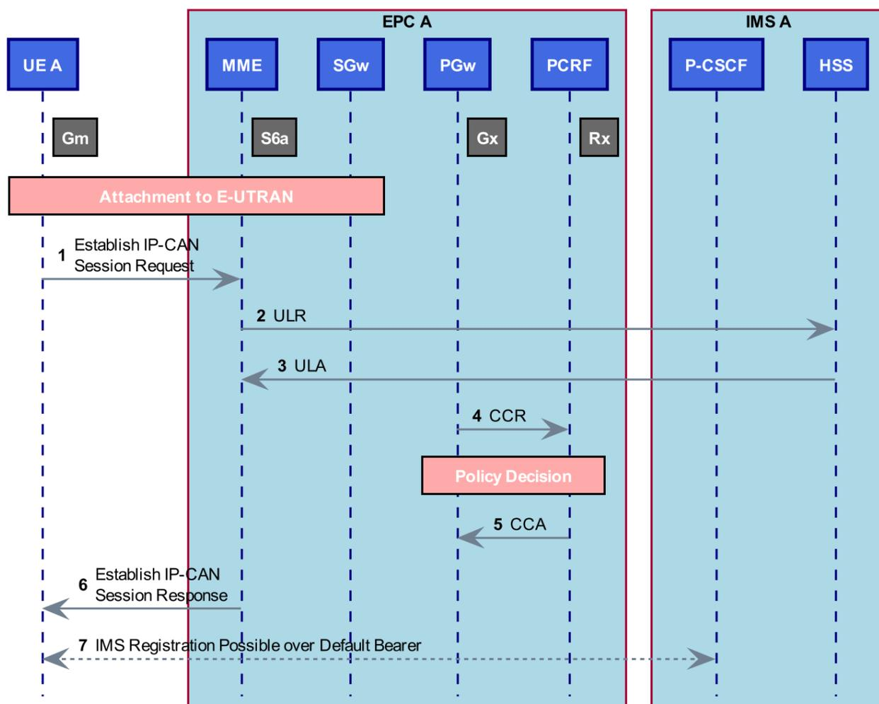
**Figure 5: Initial network attachment**
