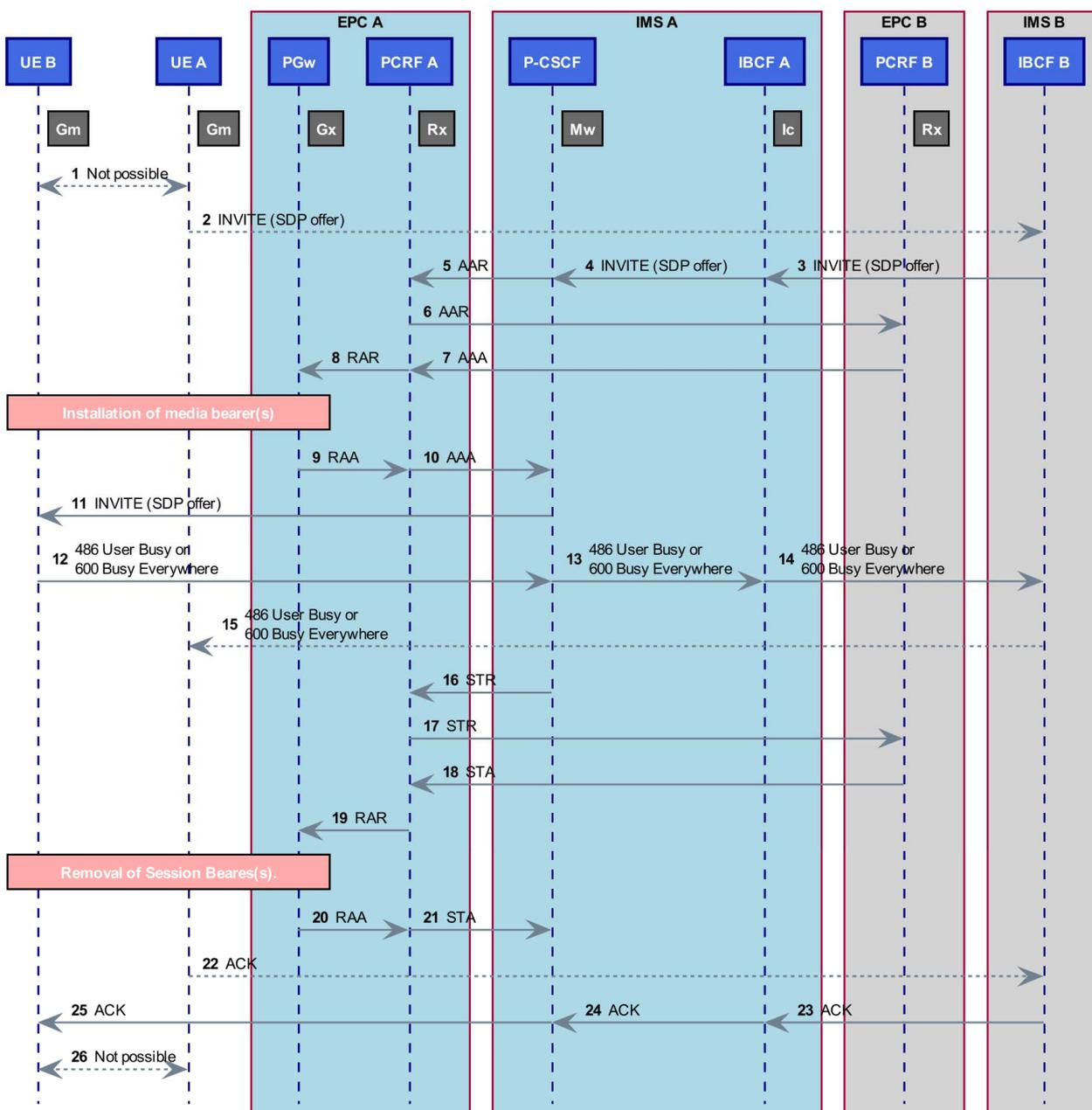
NOTE: Dashed connections between UE A and IBCF B represent the signalling which passes different entities but due to the scope of TD those are not points of observation.
