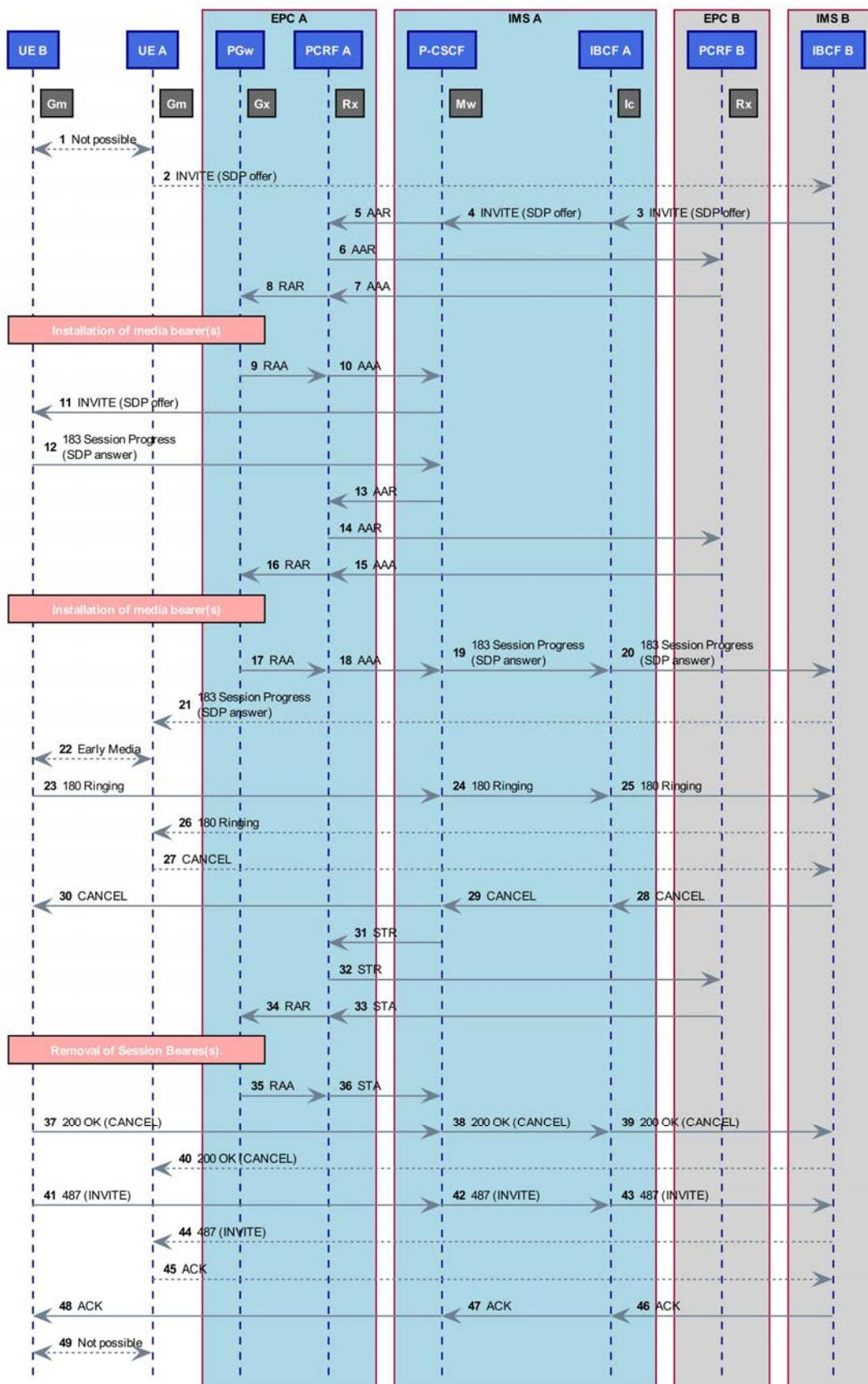
NOTE: Dashed connections between UE A and IBCF B represent the signalling which passes different entities but due to the scope of TD those are not points of observation.
