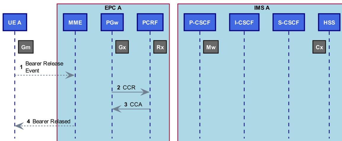
Figure 24: UE Initiated Network Detachment (not IMS Registered)
