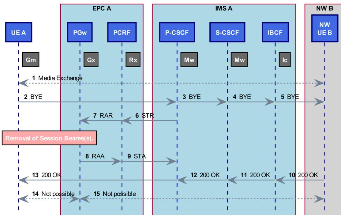
NOTE: In the above figure, the Gx interaction may take place after completion of the Rx interaction.
