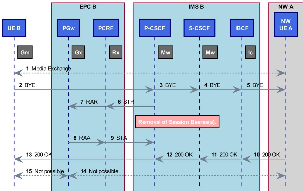
NOTE: The Rx exchange need not wait for the Gx exchange to complete.
