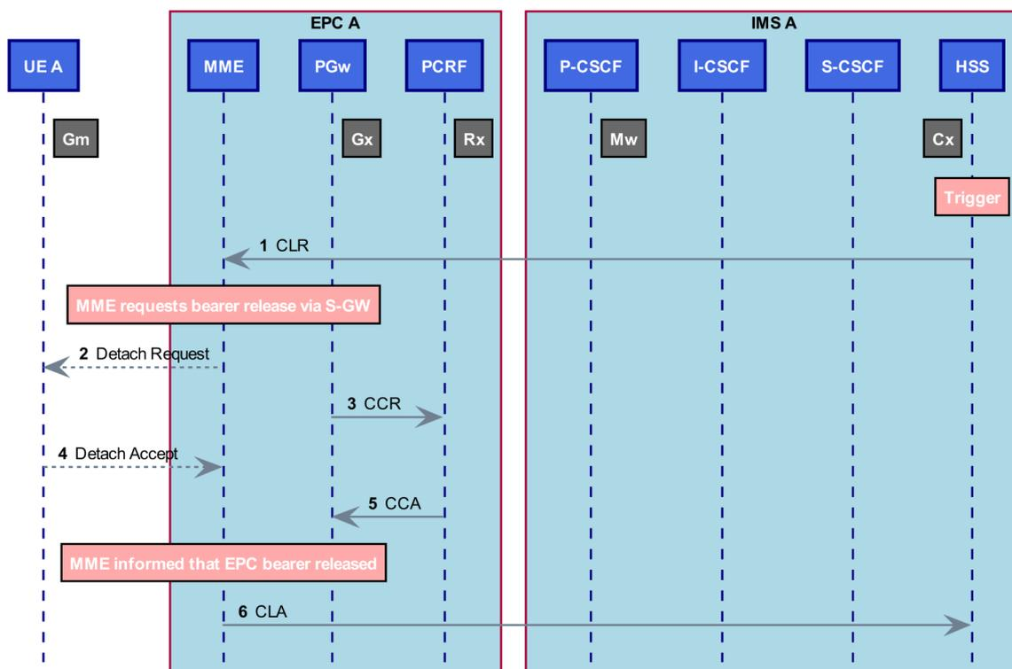
**Figure 27: HSS Initiated Network Detachment (not IMS Registered)**
