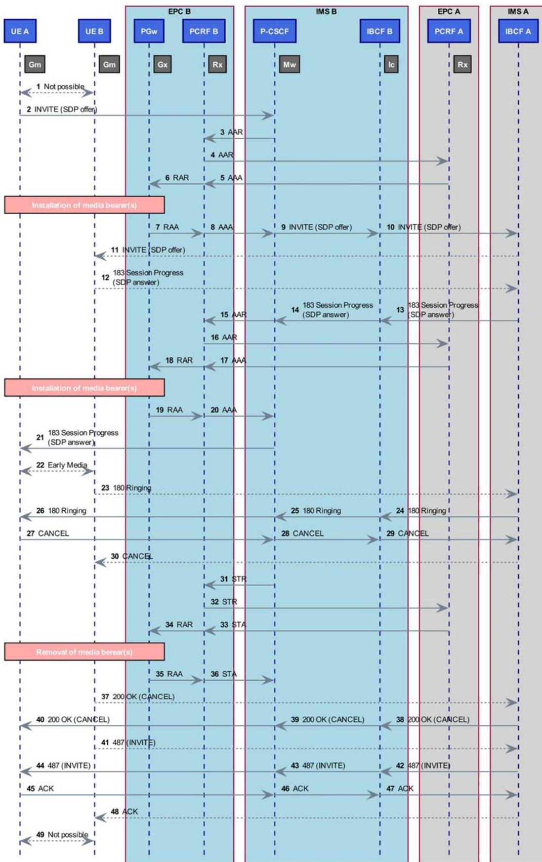
NOTE: Dashed connections between UE B and IBCF A represent the signalling which passes different entities but due to the scope of TD those are not points of observation.
