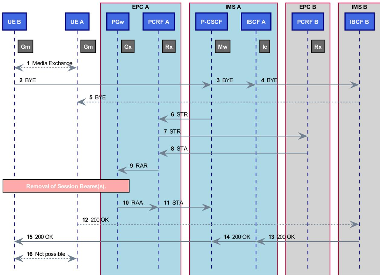
NOTE 1: The Rx exchange need not wait for the Gx exchange to complete.
