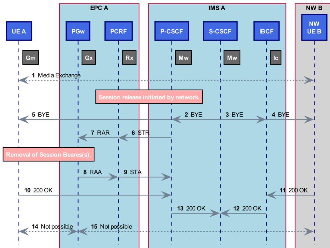
NOTE: In the above figure, the Gx interaction may take place after completion of the Rx interaction.
