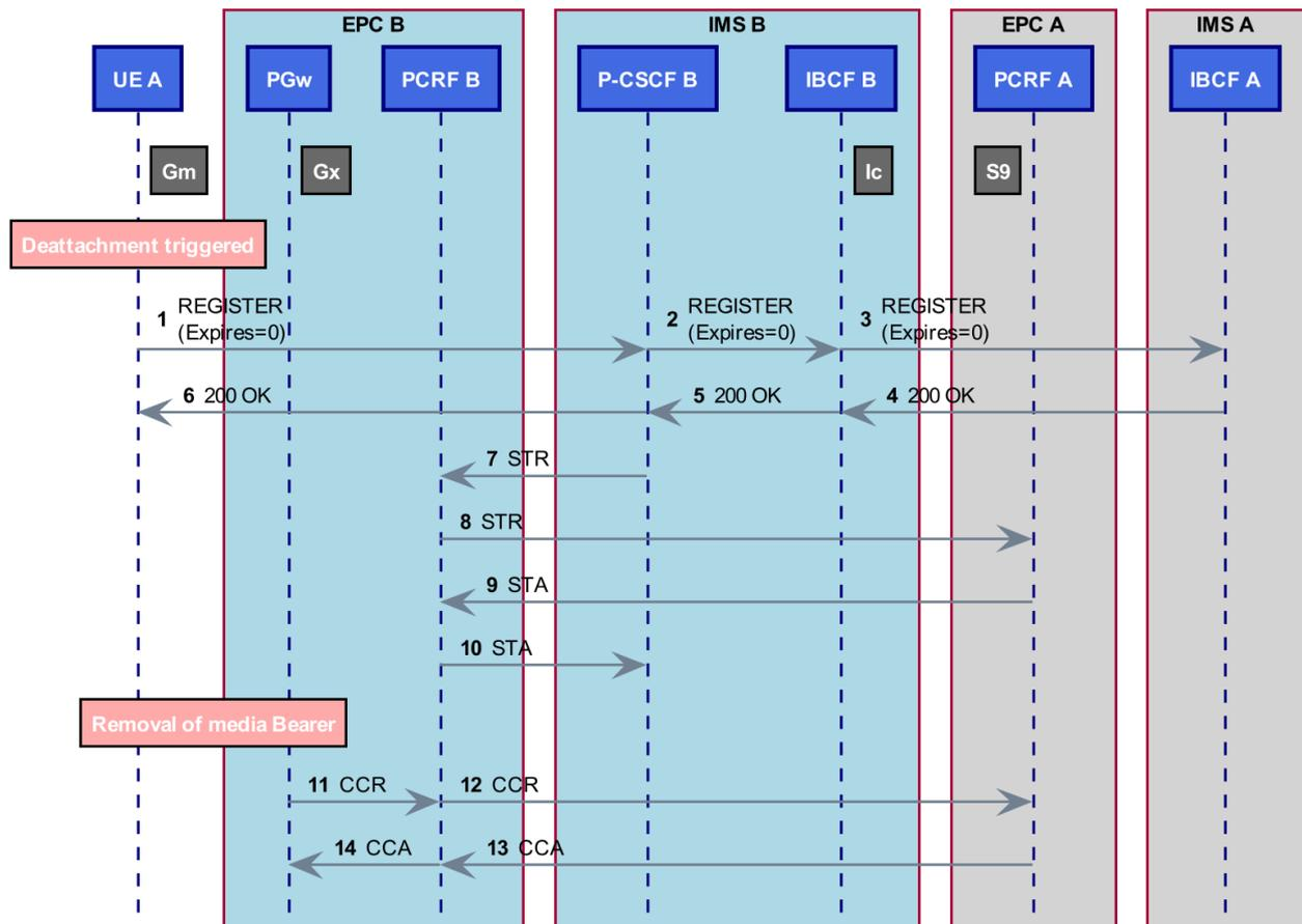
**Figure 48: UE Initiated Network Detachment - IMS Registered (Roaming)**
