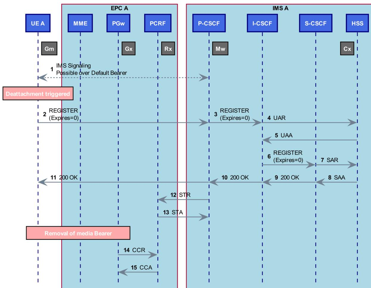
**Figure 25: UE Initiated Network Detachment (IMS Registered)**
