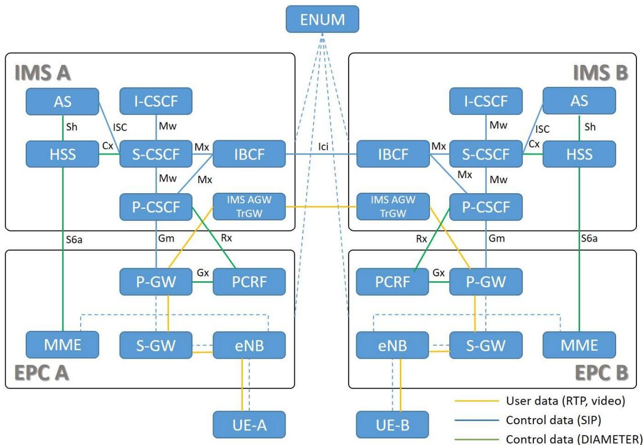
Figure 1: Configuration CF\_VxLTE\_INT
