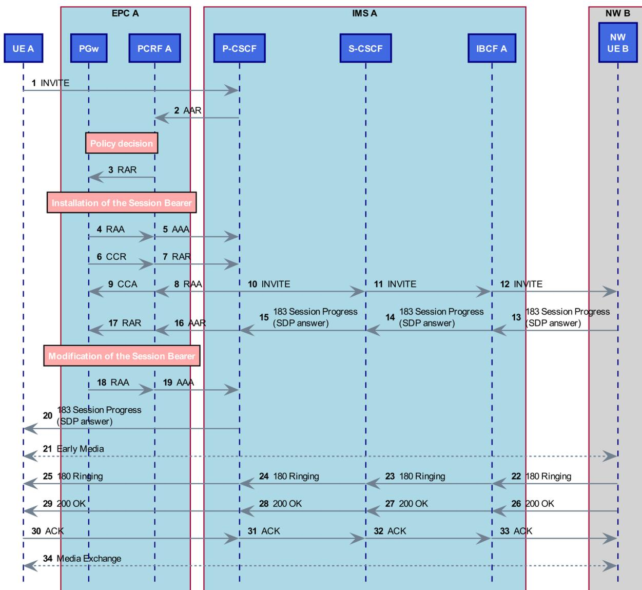
NOTE 1: In the above figure, the Gx interaction may take place after completion of the Rx interaction.
