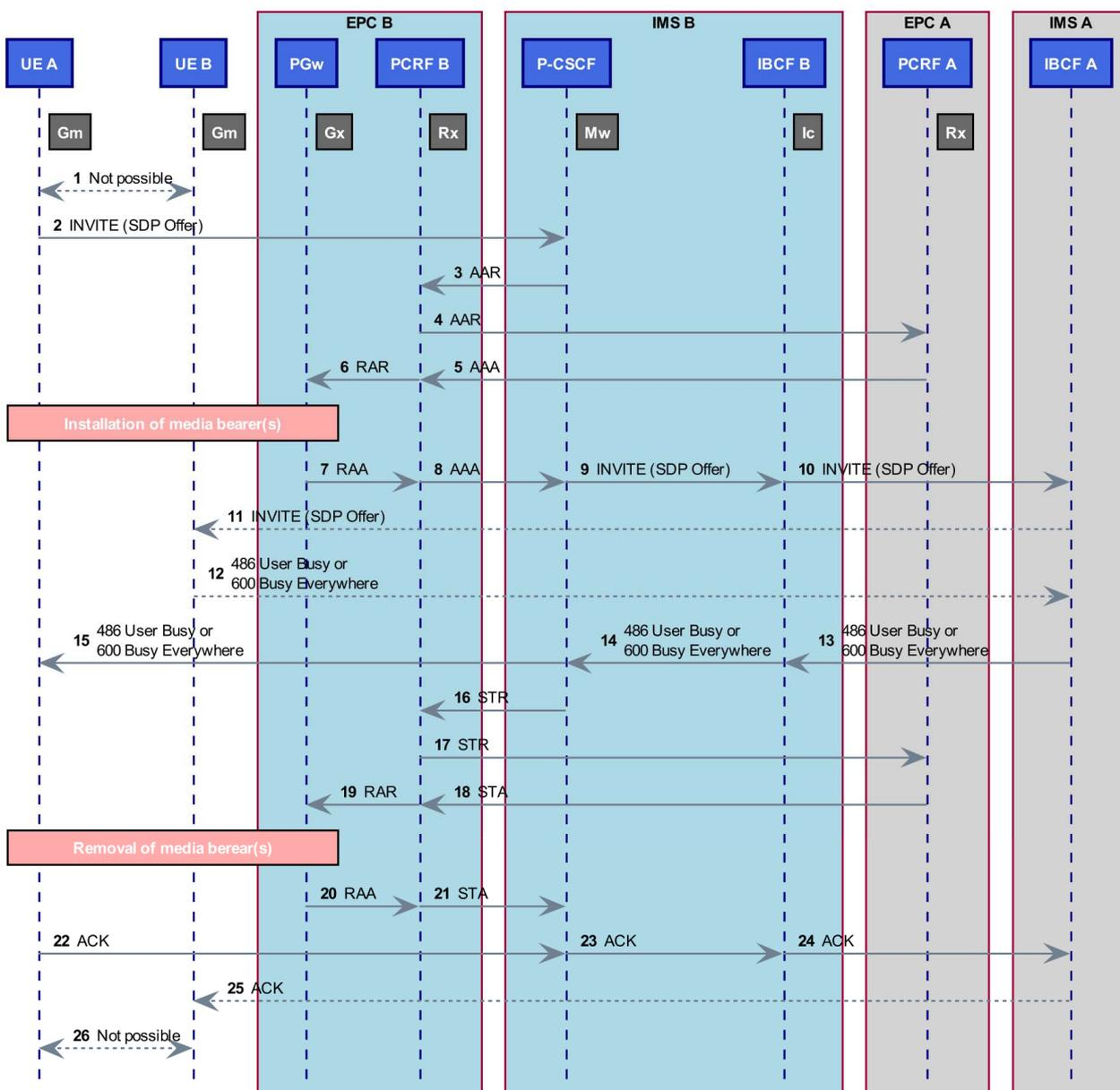
NOTE: Dashed connections between UE B and IBCF A represent the signalling which passes different entities but due to the scope of TD those are not points of observation.
