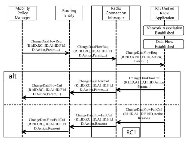
Figure 6.8-1: Flexible data flow
