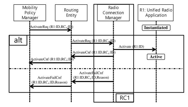
Figure 6.3-1 illustrates a signalling diagram related to the activation of an URA.
