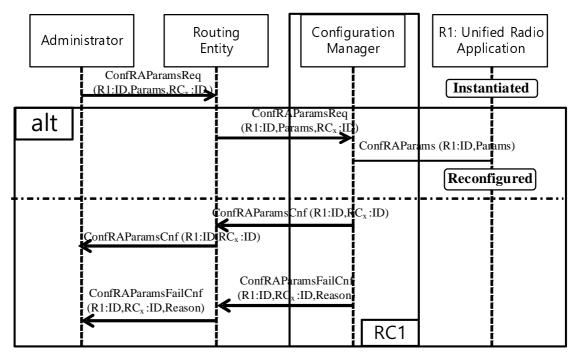
Figure 6.2-3: Configuring URA parameters
