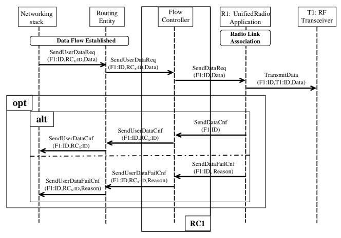
Figure 6.5-4: Signalling Diagram of sending data
