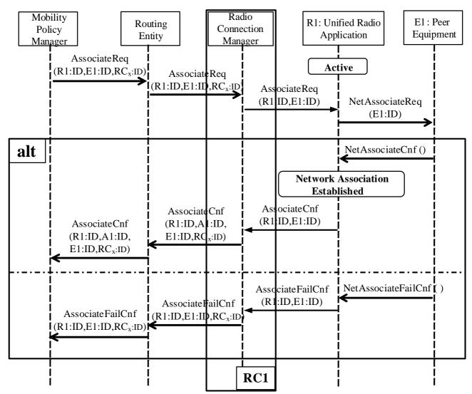
Figure 6.5-1 illustrates a signalling diagram related to the creation of a network association.
