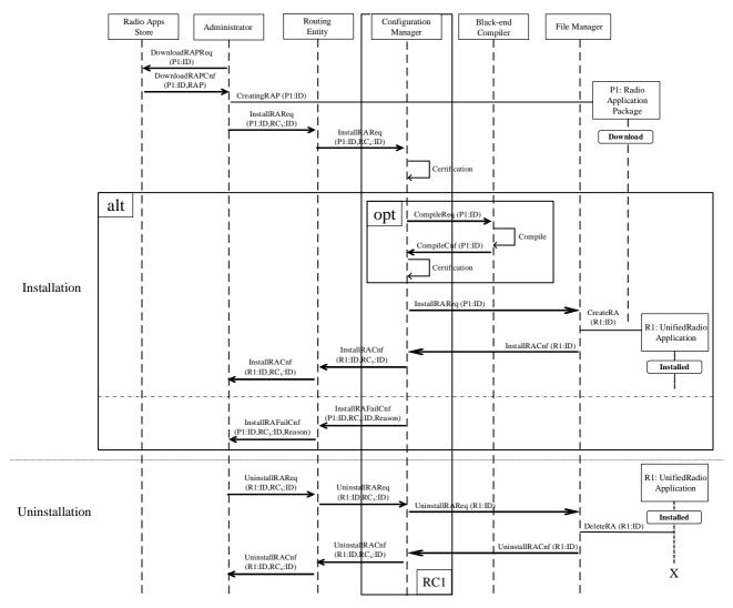
Figure 6.1-1: URA (un)installation
