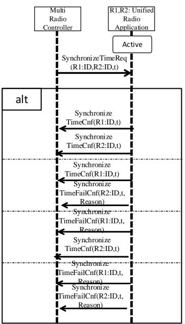
Figure 6.10-1: Synchronizing radio time
