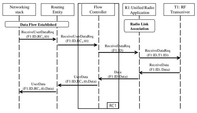
Figure 6.5-5: Signalling diagram of receiving data
