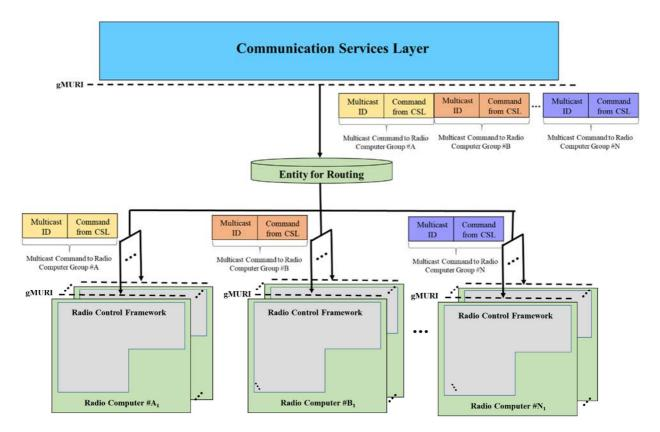
Figure 4.2.2-2: Conceptual diagram showing the routing of the CSL message(s) to the corresponding radio computer(s) in the case of multicast transmission
