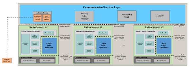
Figure 4.7.1-1: Reconfigurable Radio Equipment Architecture with security components
