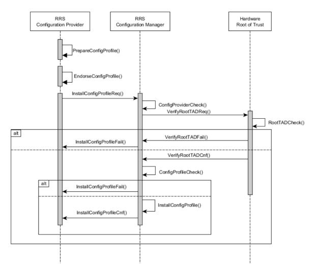
Figure 6.14-3: Signalling diagram for distributing RRS Configuration Profiles
