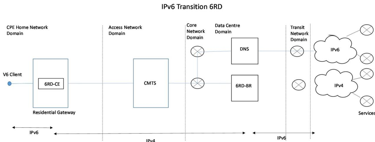
**Figure 1: Illustration of network elements to support IPv6 transition technology 6RD across Cable Network Domains**
