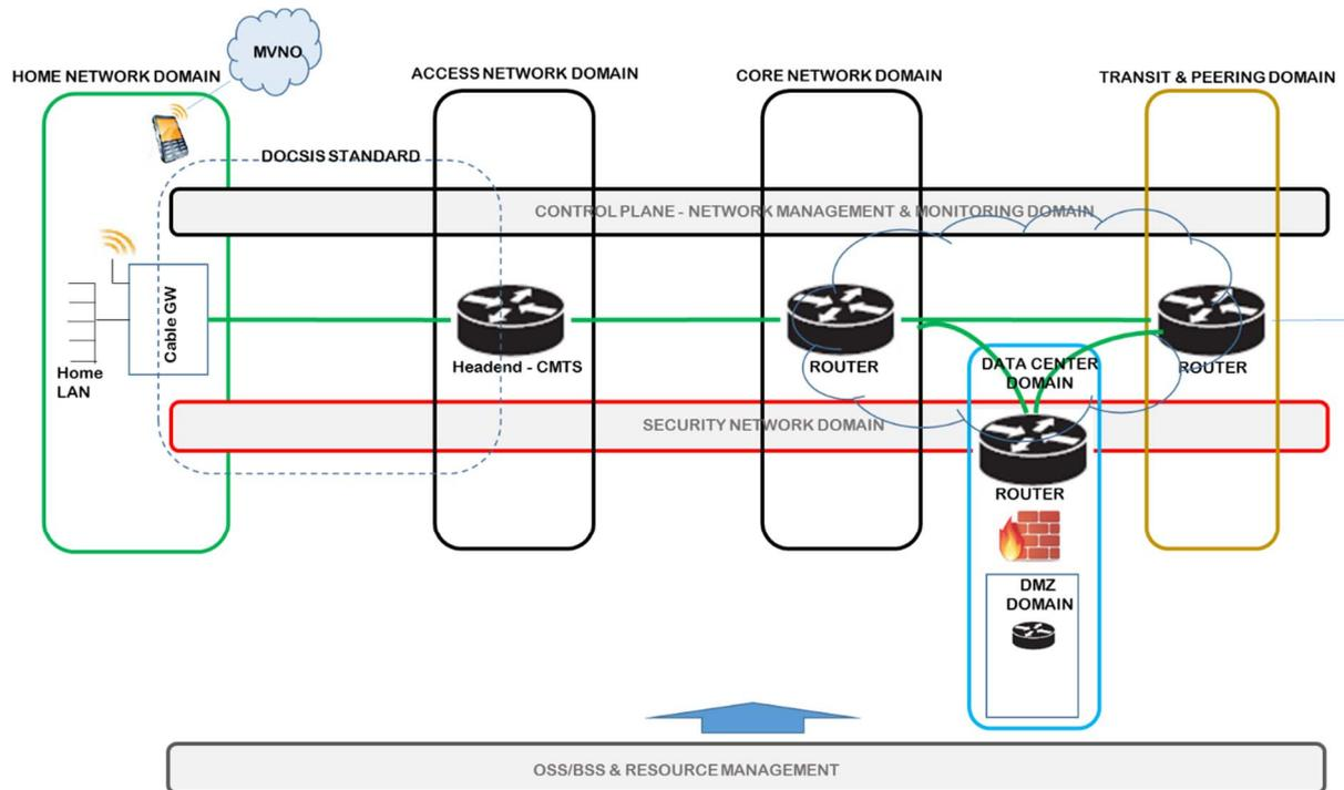
Figure 2: Illustration of the Cable Broadband Network Domains
