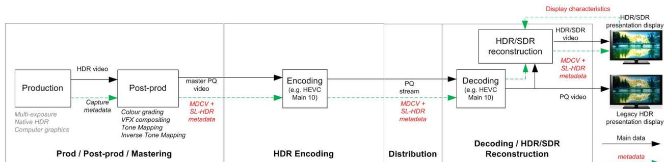
Figure 1: Example of an HDR end-to-end system
