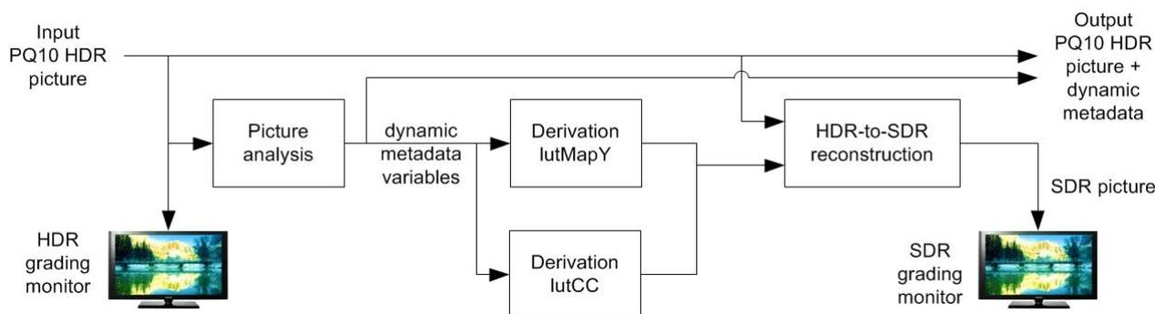
**Figure C.1: synopsis of the HDR-to-SDR decomposition process**
