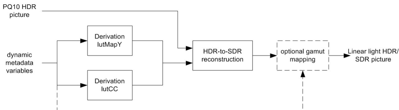
**Figure 3: Overview of the SDR reconstruction process.**
