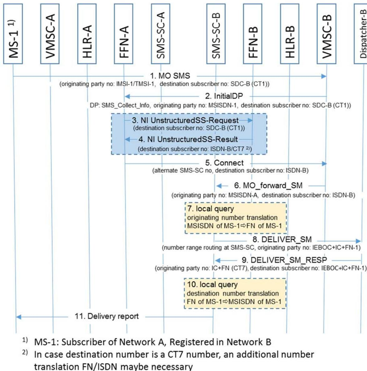
**Figure 3: Message flow smsFN to CT-1, stationary dispatcher as part of the FTS**
