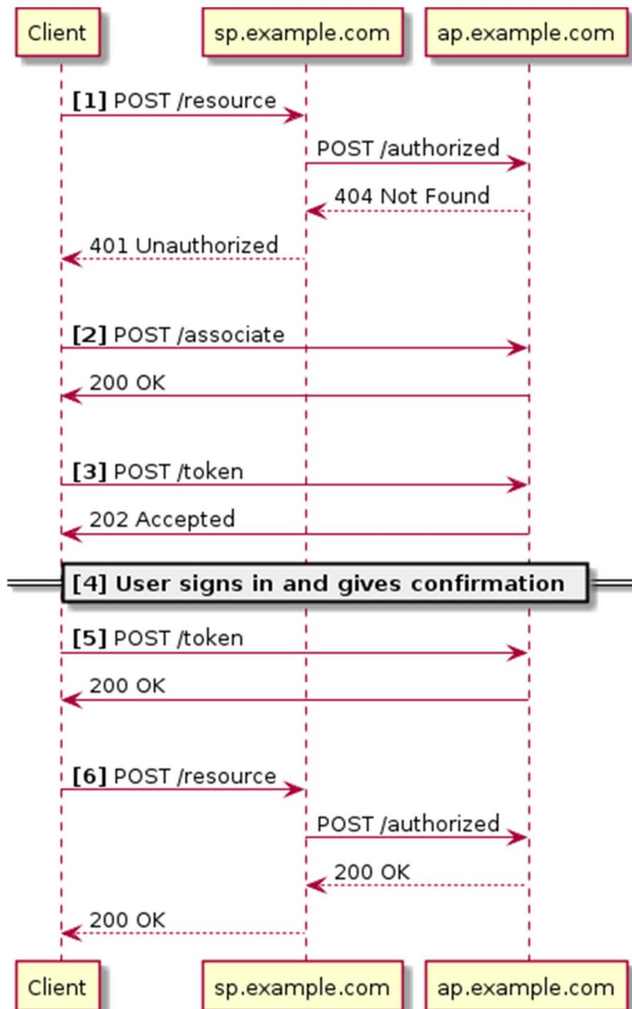
**Figure 4: Provision of token for an existing client with a new service provider with user confirmation**
