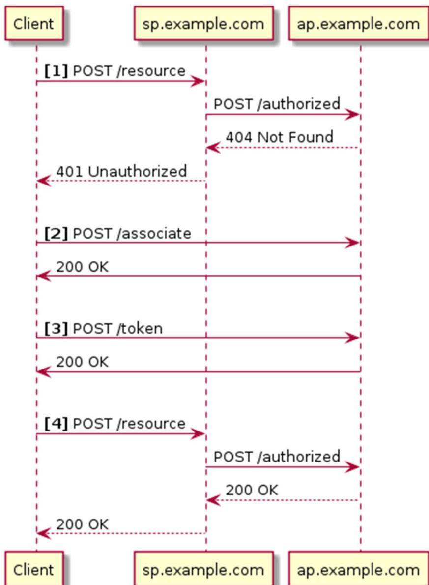
Figure 5: Automatic provision of token for an existing client
