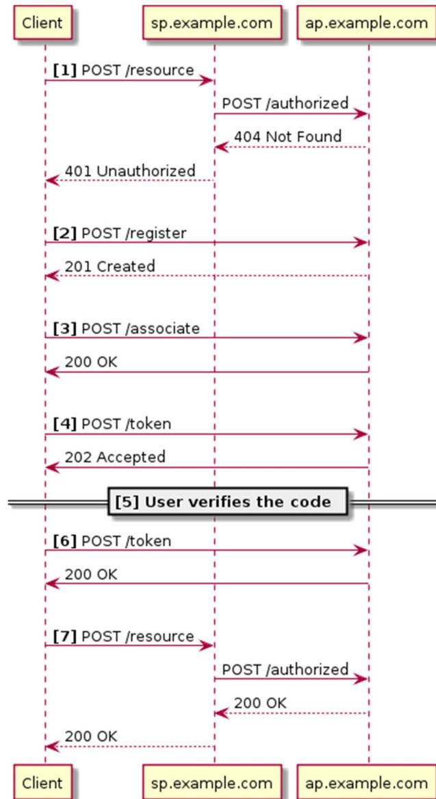
Figure 1: Overview of CPA user mode device flow
