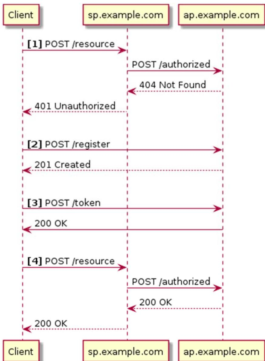
Figure 2: Overview of CPA client mode device flow
