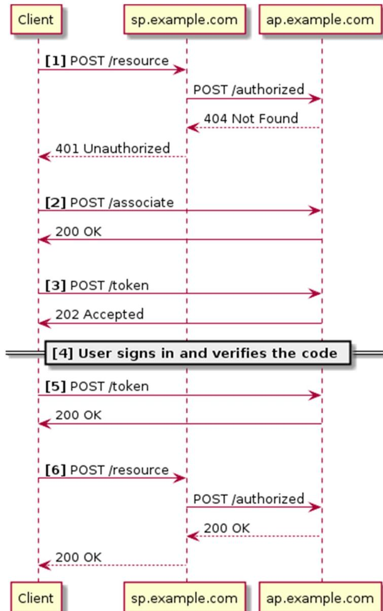
**Figure 3: Provision of token for an existing client with a new service provider with pairing code input**
