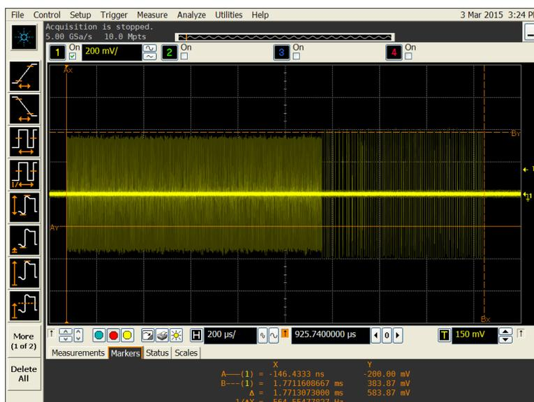
**Figure A.6: "Active period" of a packet transmission captured by the Oscilloscope**
