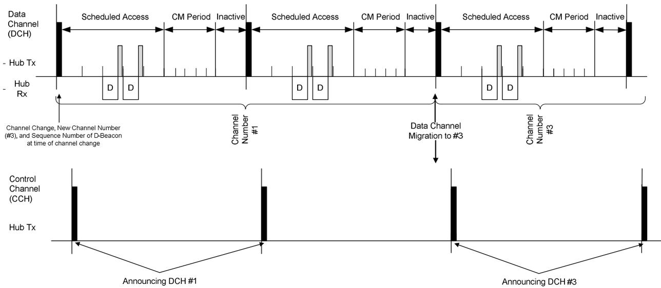
Figure 21: Example of Data Channel Migration (from #1 to #3)
