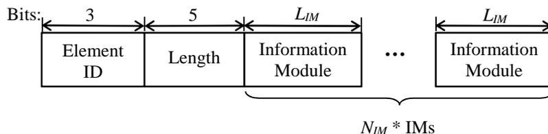
**Figure 7: Structure of an Information Unit**
