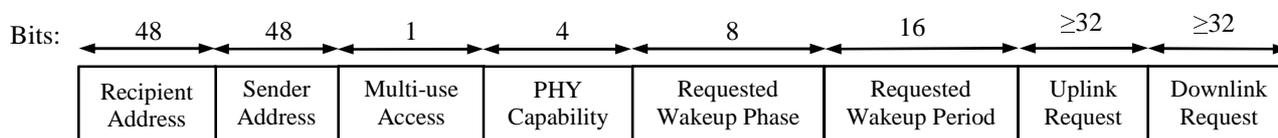
**Figure 13: Connection Request Frame Format**
