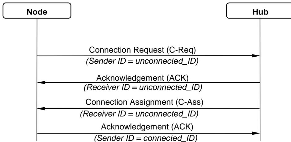
Figure 16: Connection procedure
