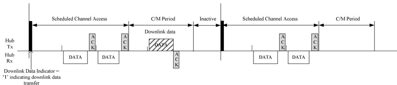
Figure 18: Downlink Data Transmission Illustration
