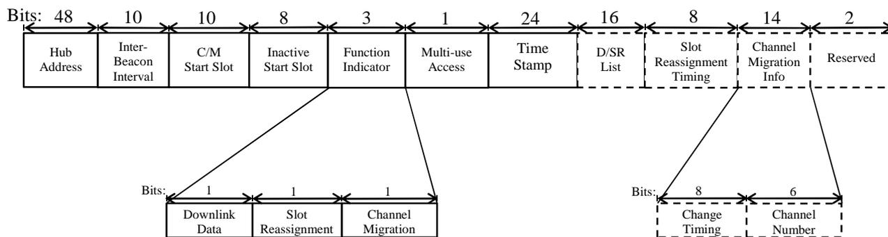
**Figure 12: Data Channel Beacon Frame Format**
