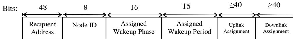
**Figure 14: Connection Assignment Frame Format**
