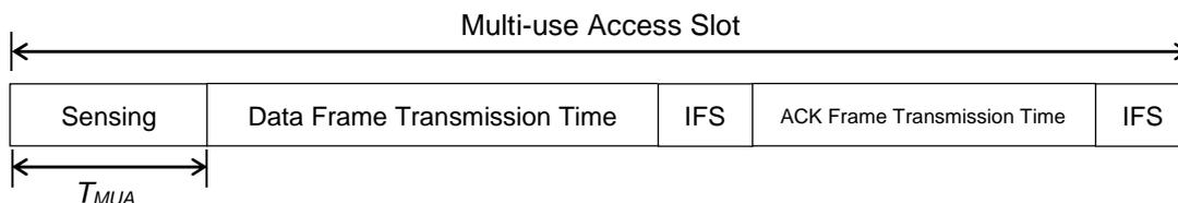
**Figure 6: Multi-use Access Slot Structure**
