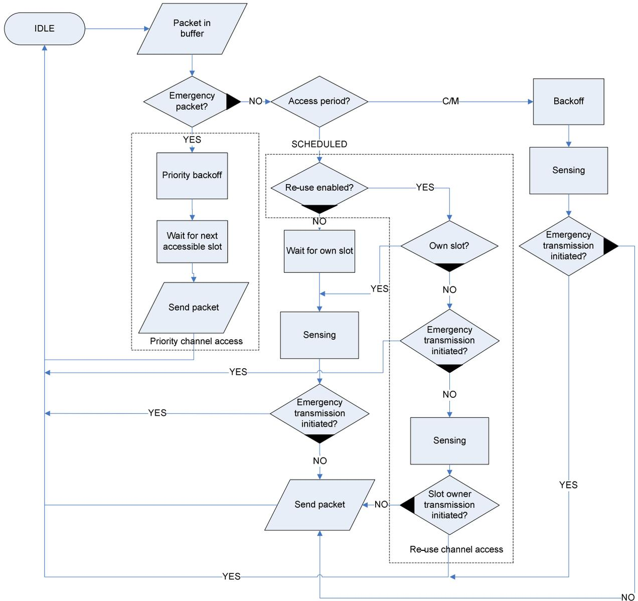
Figure A.1: Flowchart of Multi-use Channel Access
