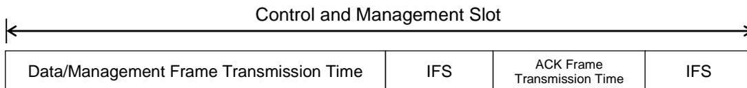
**Figure 5: Control and Management Slot Structure**
