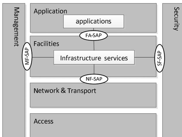
Figure 1: Infrastructure services within the ITS-S architecture
