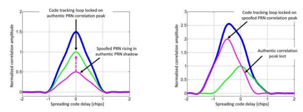
Figure A.7: Effects of shadowed spoofing on correlation functions
