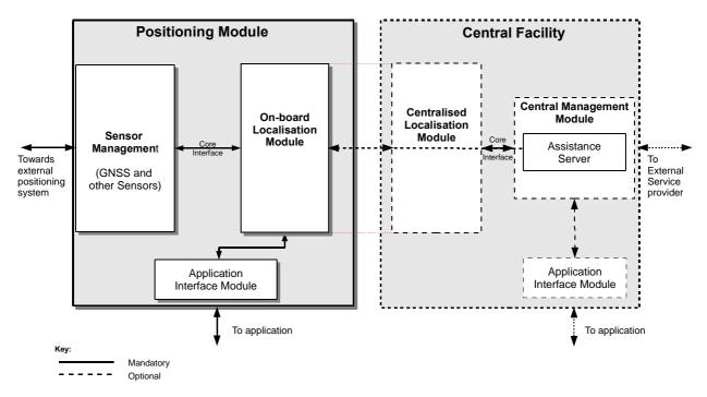
Figure 1: GNSS-based Location System (GBLS) Architecture
