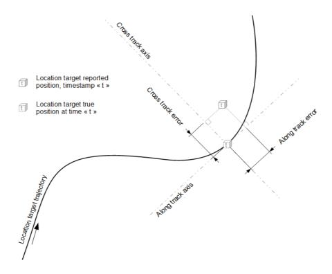
Figure 2: Definition of Cross-Track and Along-Track Position Errors
