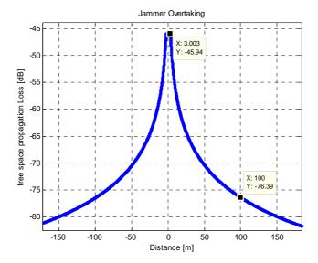
Figure A.6: Free space propagation loss with respect to the jammer distance
