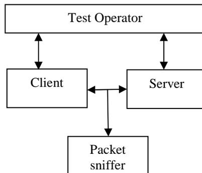
Figure 3: Basic One-2-One CoAP client/server Configuration
