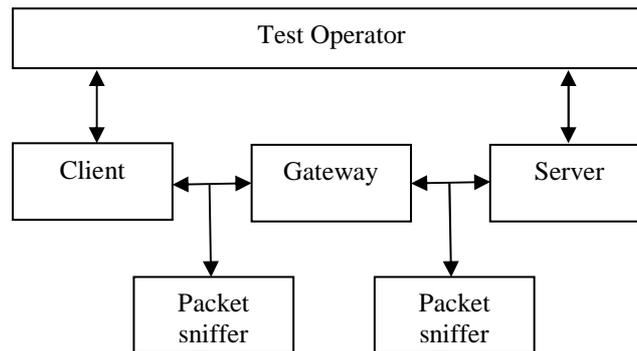
**Figure 4: Basic One-2-One CoAP client/server Configuration in lossy context**
