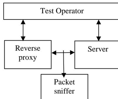
**Figure 5: Basic One-2-One CoAP proxy/server Configuration**
