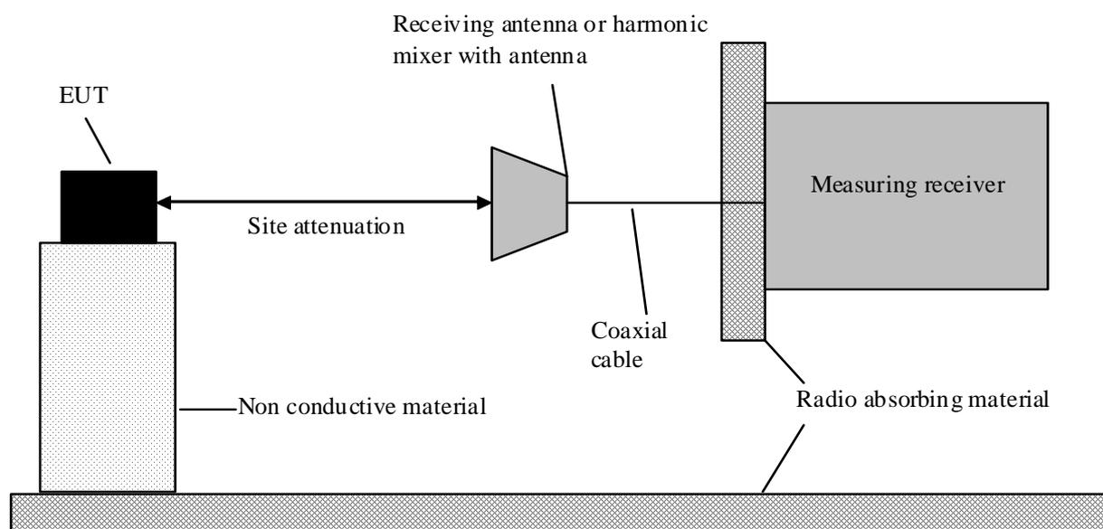
**Figure 1: Example of a test site above 18 GHz with one reflecting surface**
