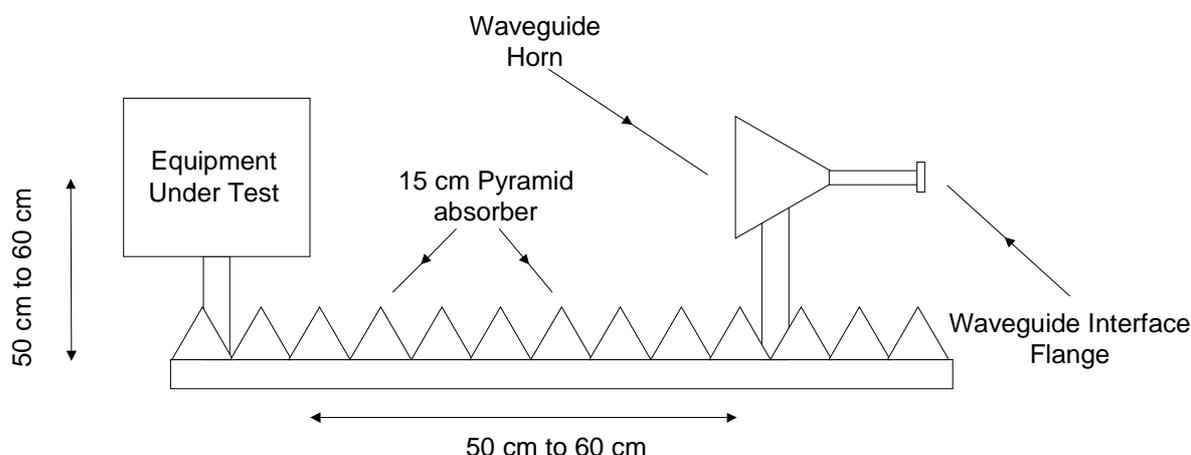
**Figure 3: Example of a test fixture**
