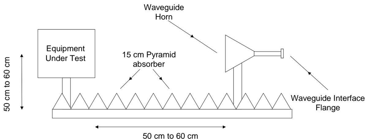
**Figure 3: Example of a test fixture**
