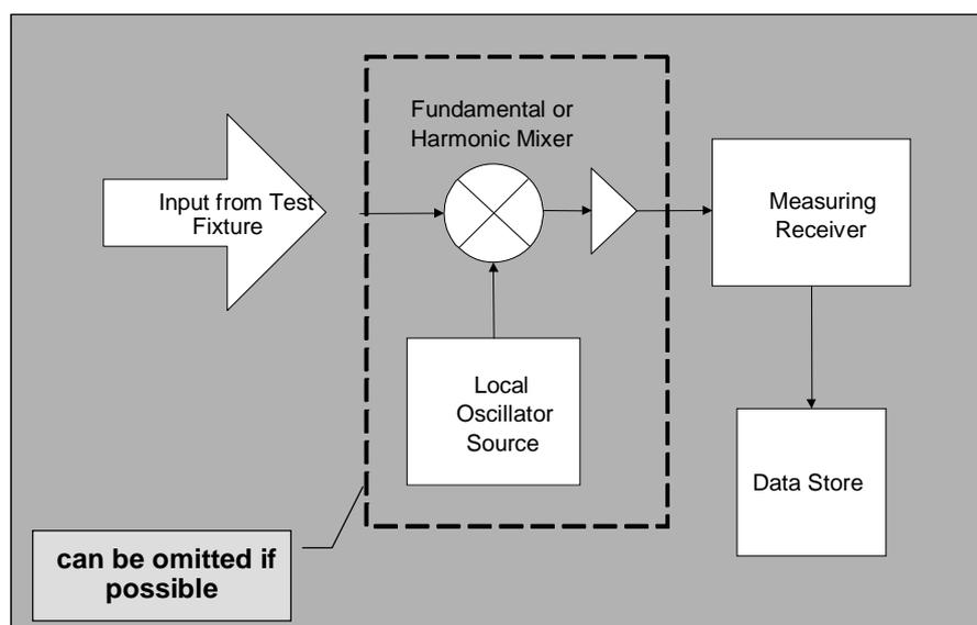
**Figure 2: Test equipment using a mixer for measuring emissions in the EHF frequency range**
