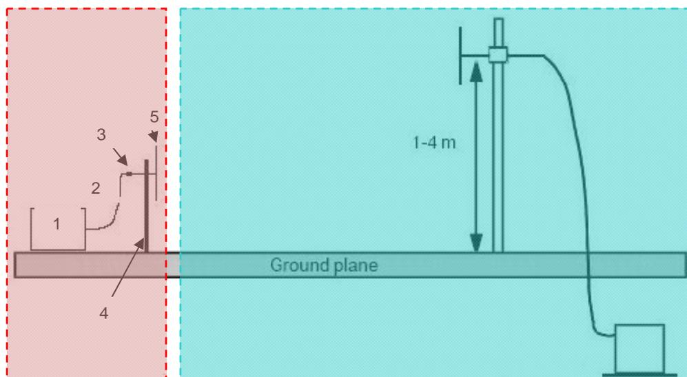
NOTE: Right box of figure B.4: Statistical evaluation/Repetition measurement uncertainty (Type A evaluation). Left box of figure B.4: Measurement uncertainty of the measurement chain consisting of a generator, conductors and the K-factor of the reference antenna (as well as attenuators used for coercive adaptation if necessary) can be summed up by determination of the substitution power with a reference power meter.
