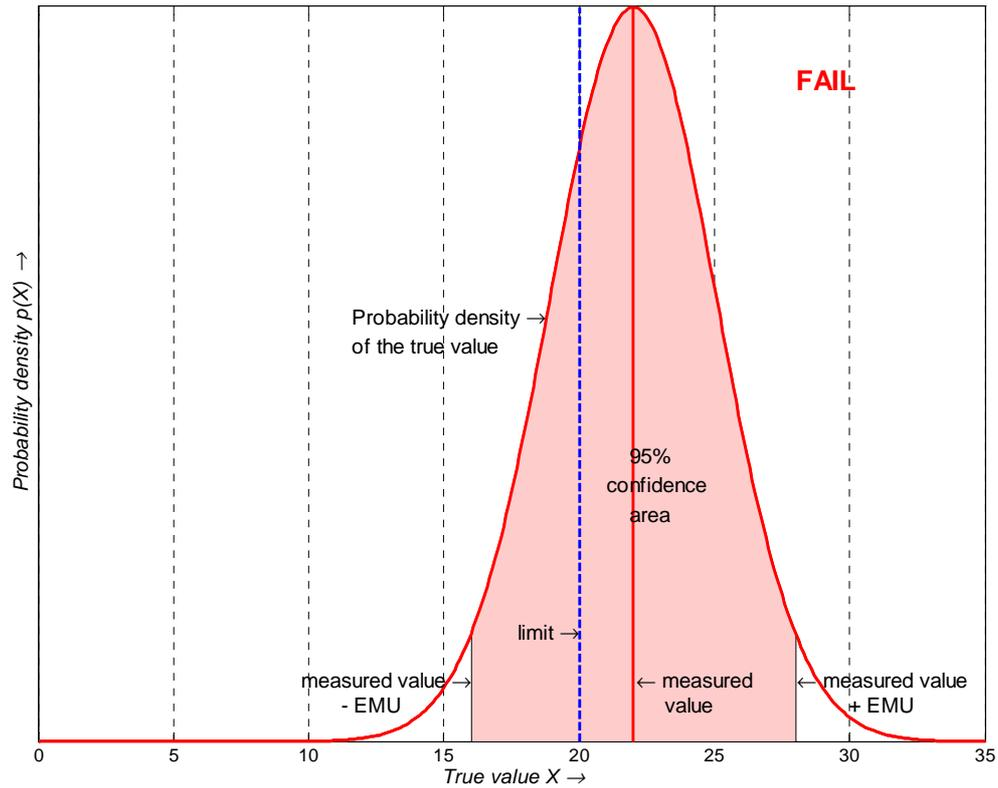
Figure A.1: Equipment does not meet the requirement
