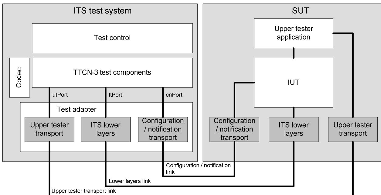
**Figure 1: General conformance test system architecture for SUTs**
