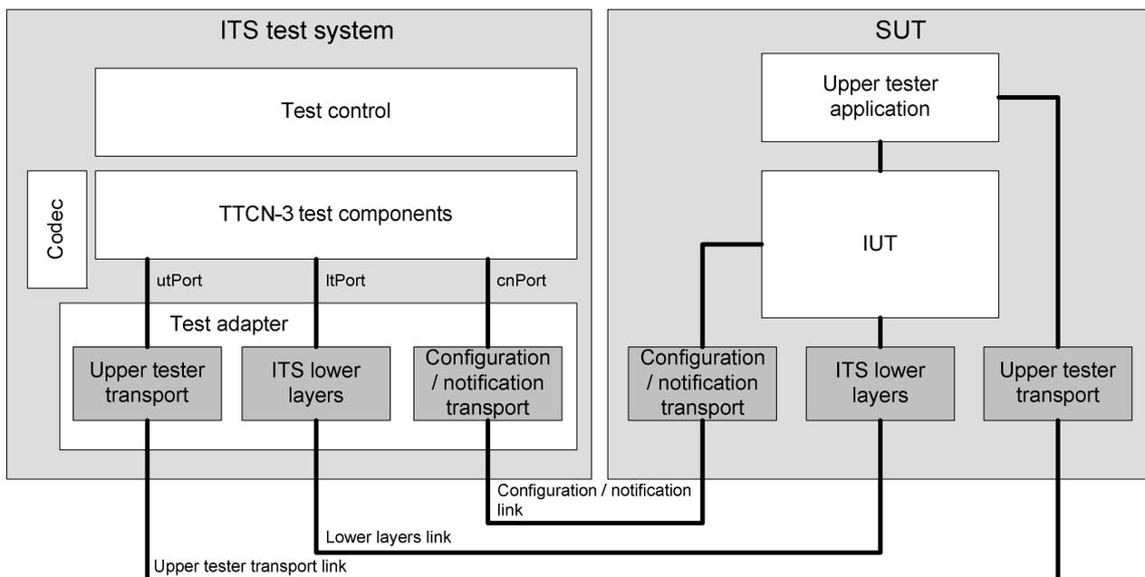
**Figure 1: General conformance test system architecture for SUTs**
