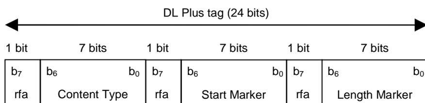
**Figure 5: Structure of the DL Plus tag**
