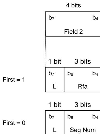
**Figure 6: Structure of Field 2 for DL Plus**
