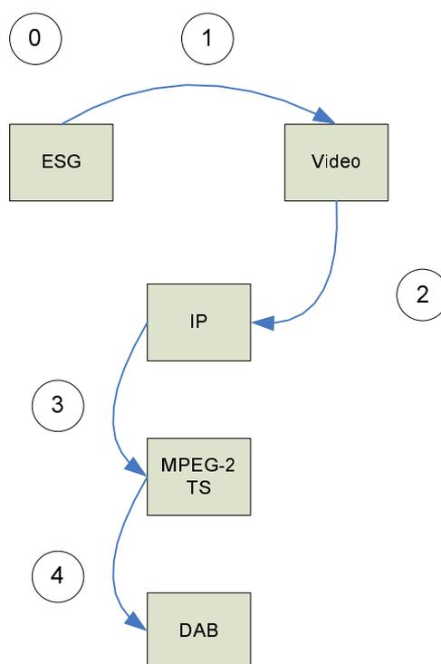
**Figure C.1: Discovery of an Video Service on DAB IPDC Systems**
