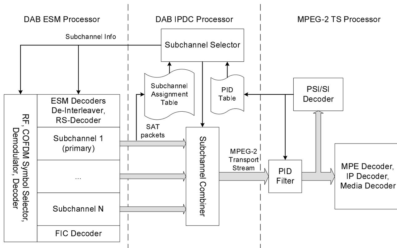
**Figure A.1: DAB IPDC reference receiver model**
