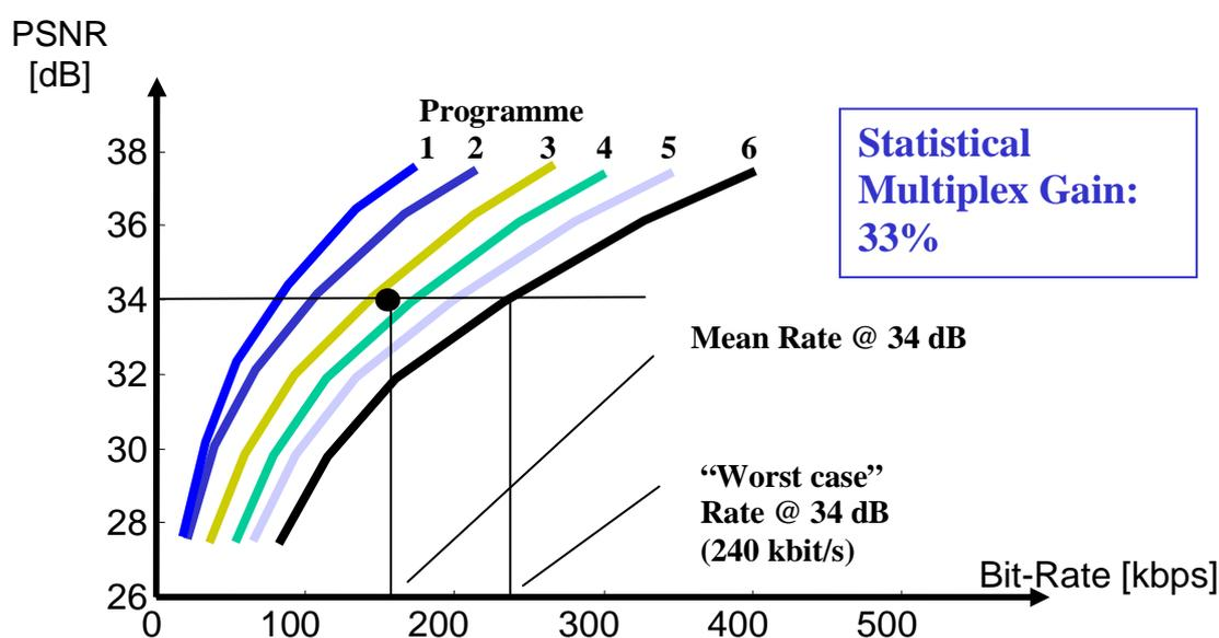
**Figure D.1: Rate distortion curves for different programmes with worst case and mean data rate per programme**
