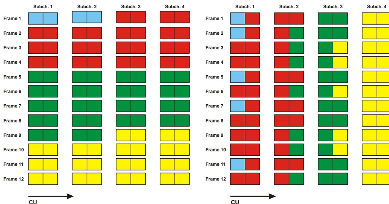
Figure 5: Macro time slicing (left) and micro time slicing (right)
