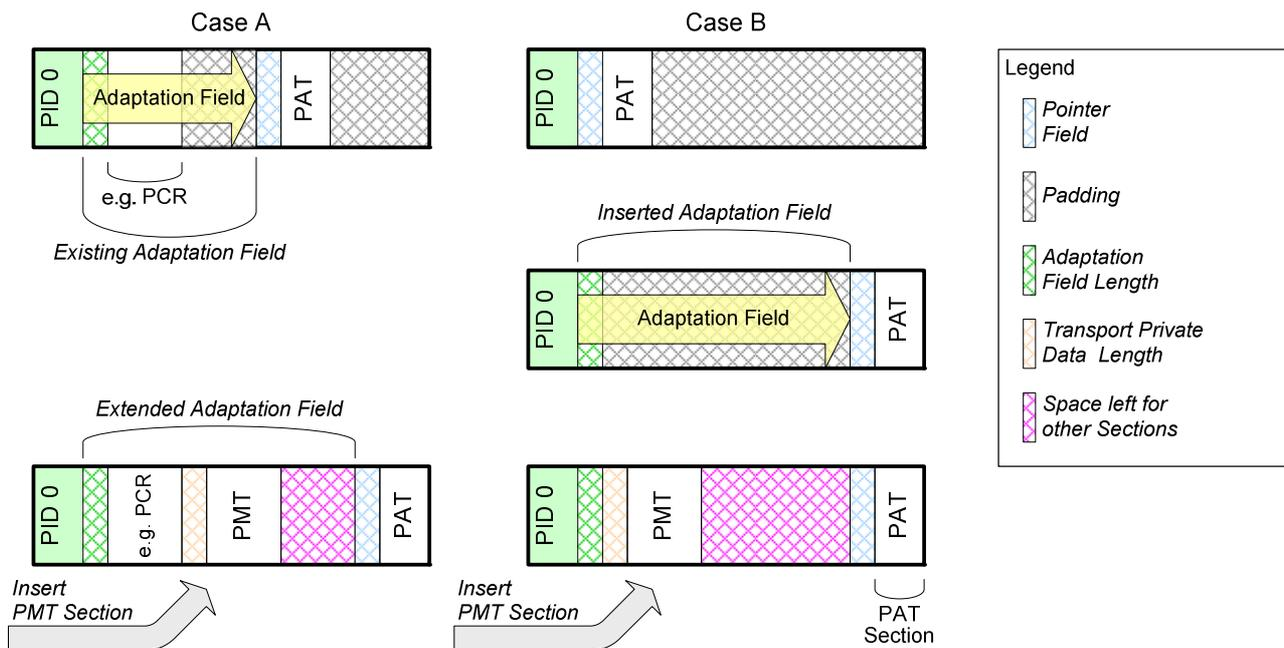
**Figure 6: Transport of PMT section in private data block of adaptation field in PAT packet**
