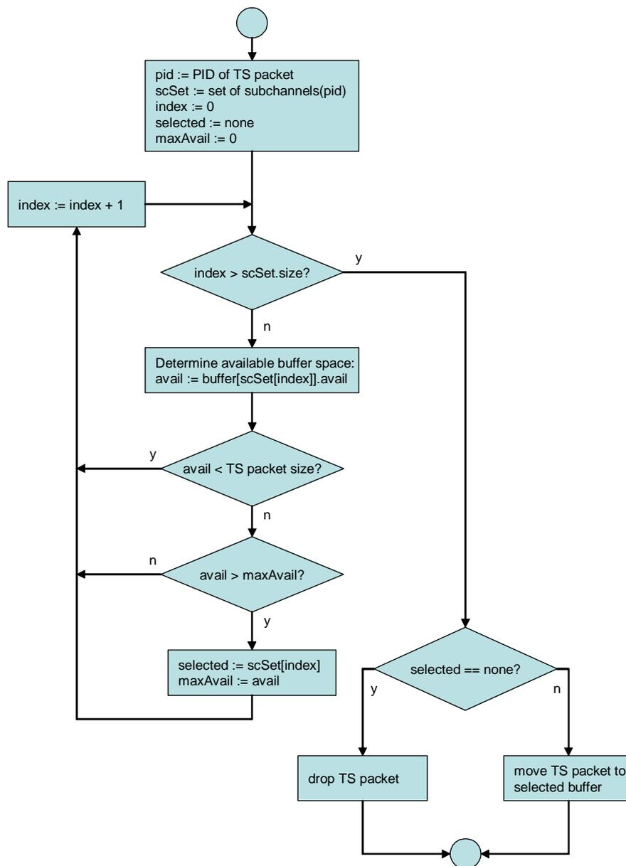
**Figure 9: Transmitter TS-packet sub-channel selection process**
