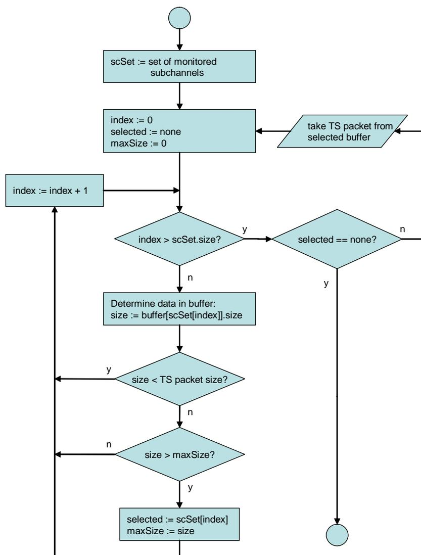
**Figure 10: Receiver TS-packet extraction process**
