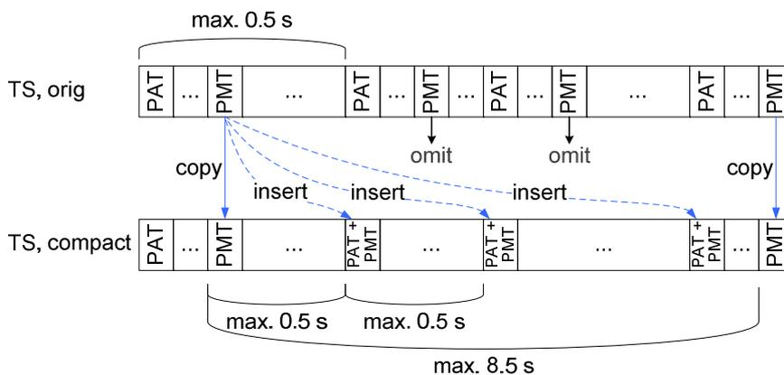
**Figure 7: Transmission period of PSI packets in original TS and using efficient PMT transmission as specified in clause 5.3.1**
