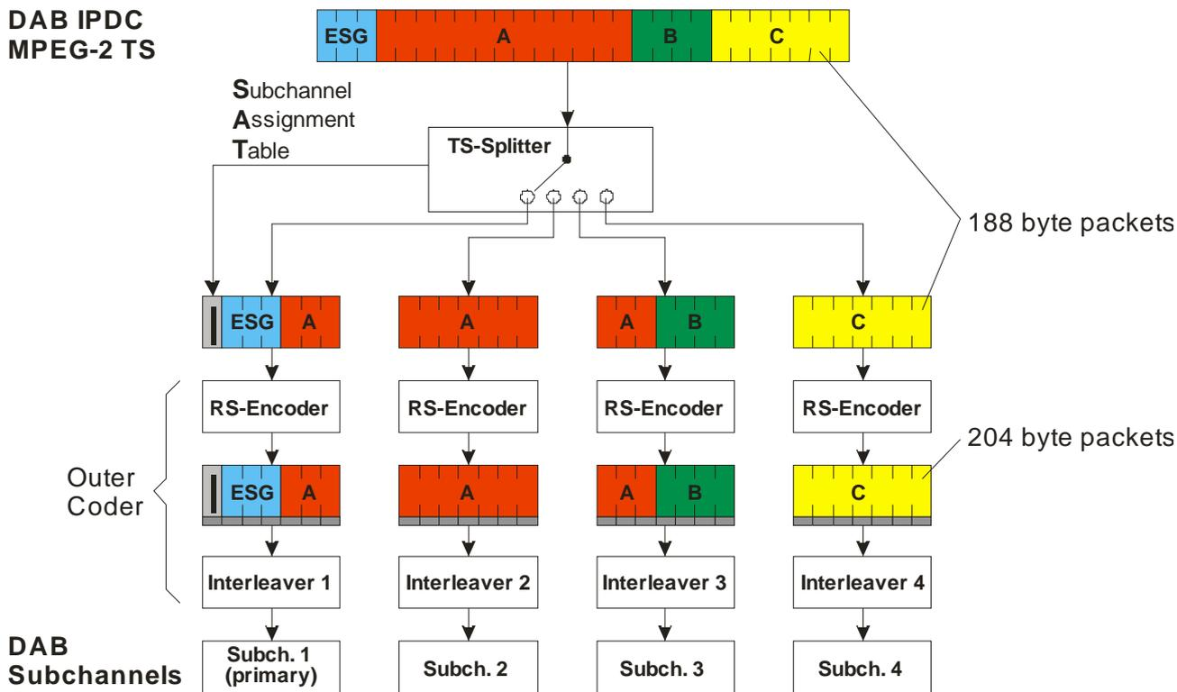
Figure 4: DAB IPDC transport mechanism for MPEG-2 transport streams
