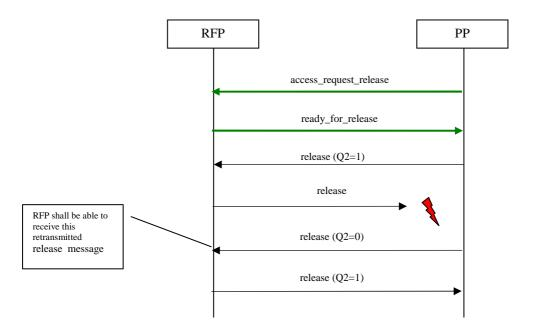
Figure 32: Two-way Single Packet Mode Connection (release retransmitted)
