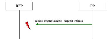
Figure 27: Packet Mode Connection setup fail (access message wrong)
