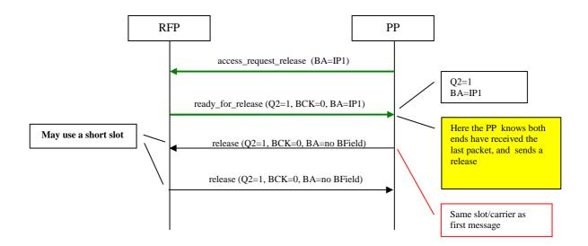
Figure 14: Two-way Single Packet Data Transfer
