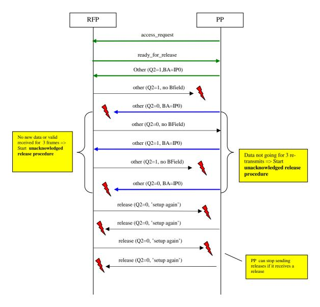
Figure 35: Packet Mode Connection fails (retransmission abandoned)
