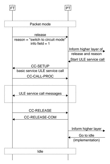
Figure 48: Use of reason code "switch to circuit mode" and setup ULE service call
