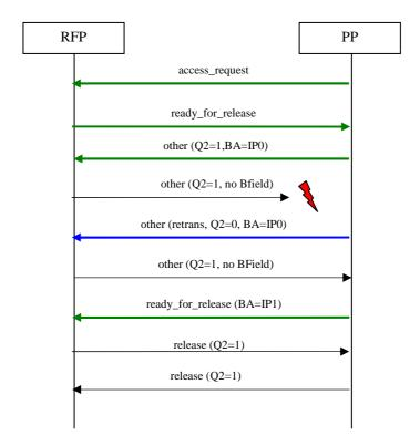
Figure 30: Packet Mode Connection success (2<sup>nd</sup> other message retransmitted)
