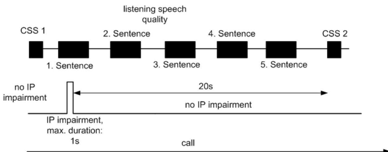
**Figure 12: Test sequence to measure quality of jitter buffer adjustment (with 1 of 8 sentences)**
