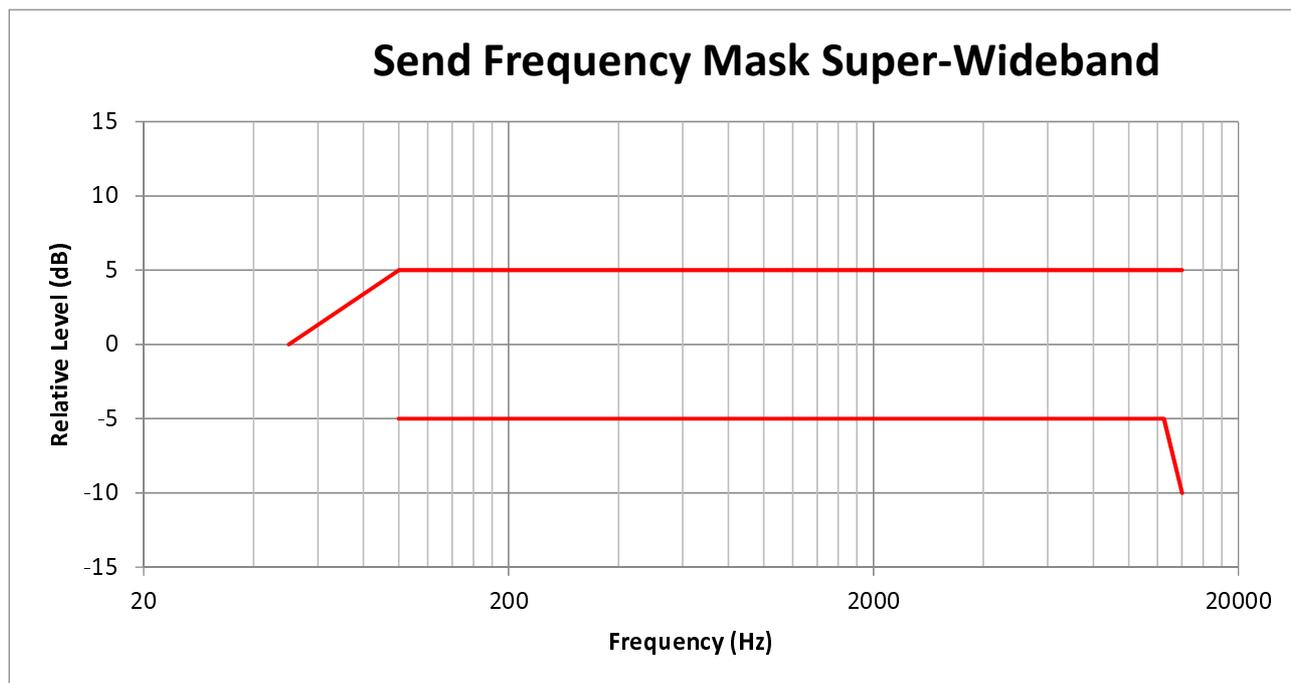
Figure 4: Send frequency response mask for super-wideband
