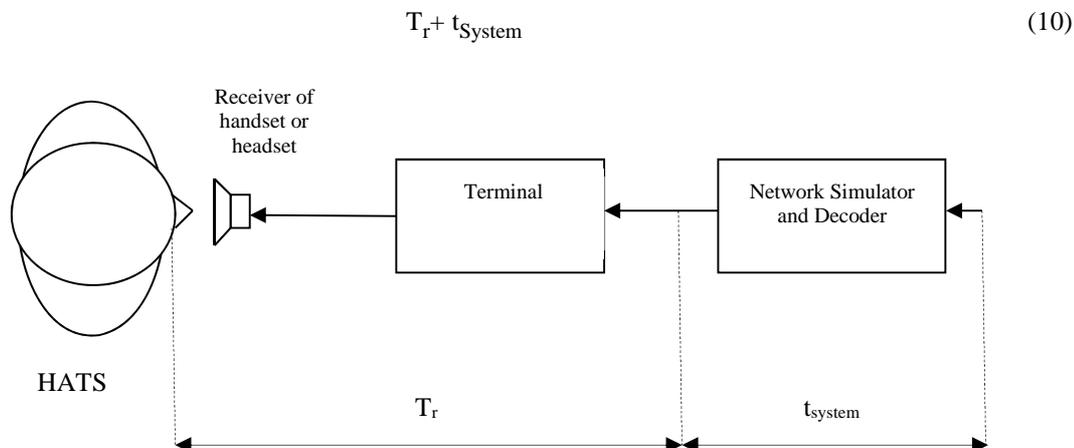
**Figure 11: Different blocks contributing to the delay in receive direction**
