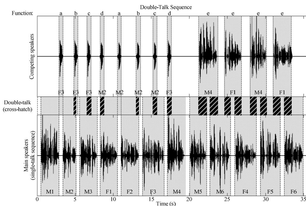
Figure 9: Double talk test sequence with overlapping speech sequences in send and receive direction
