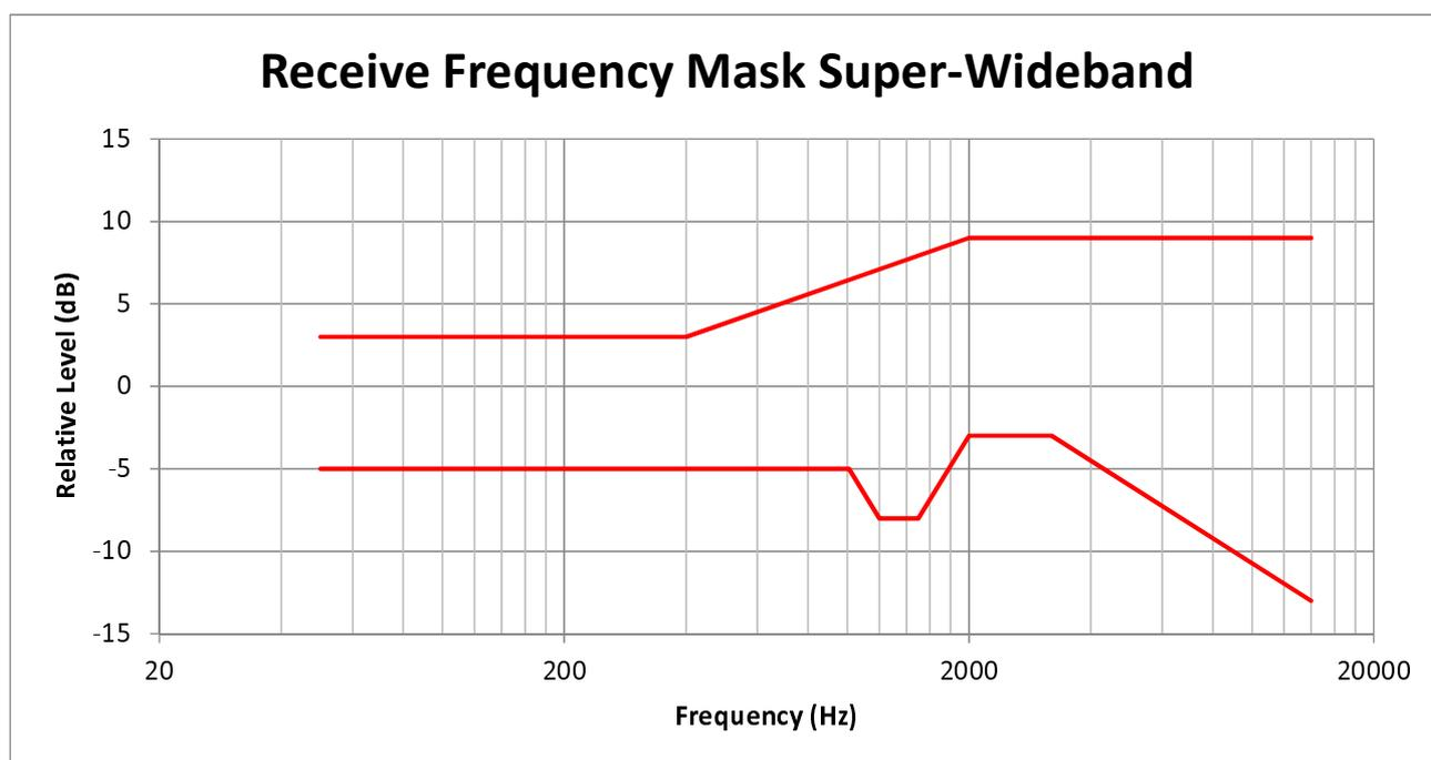
**Figure 7: Receive frequency response mask for Super-Wideband**
