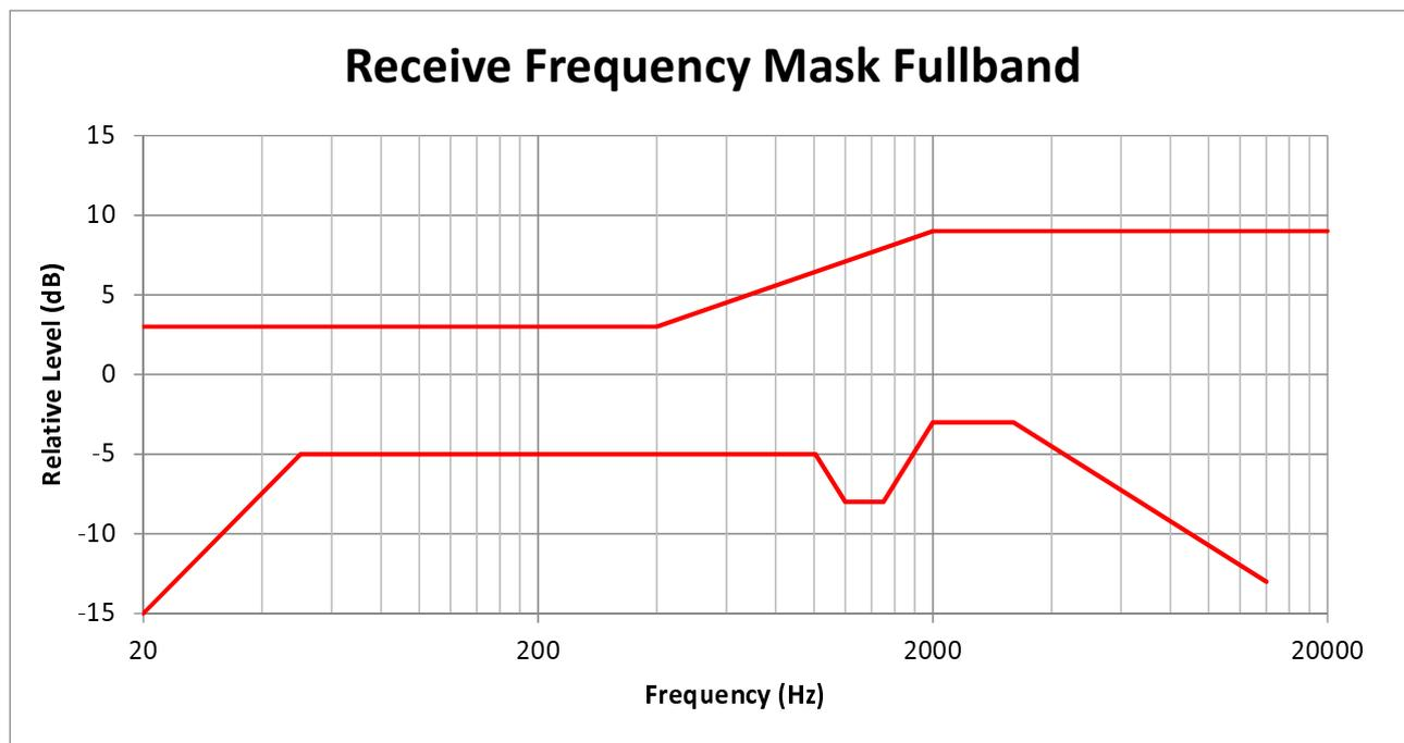
**Figure 8: Receive frequency response mask for Fullband**
