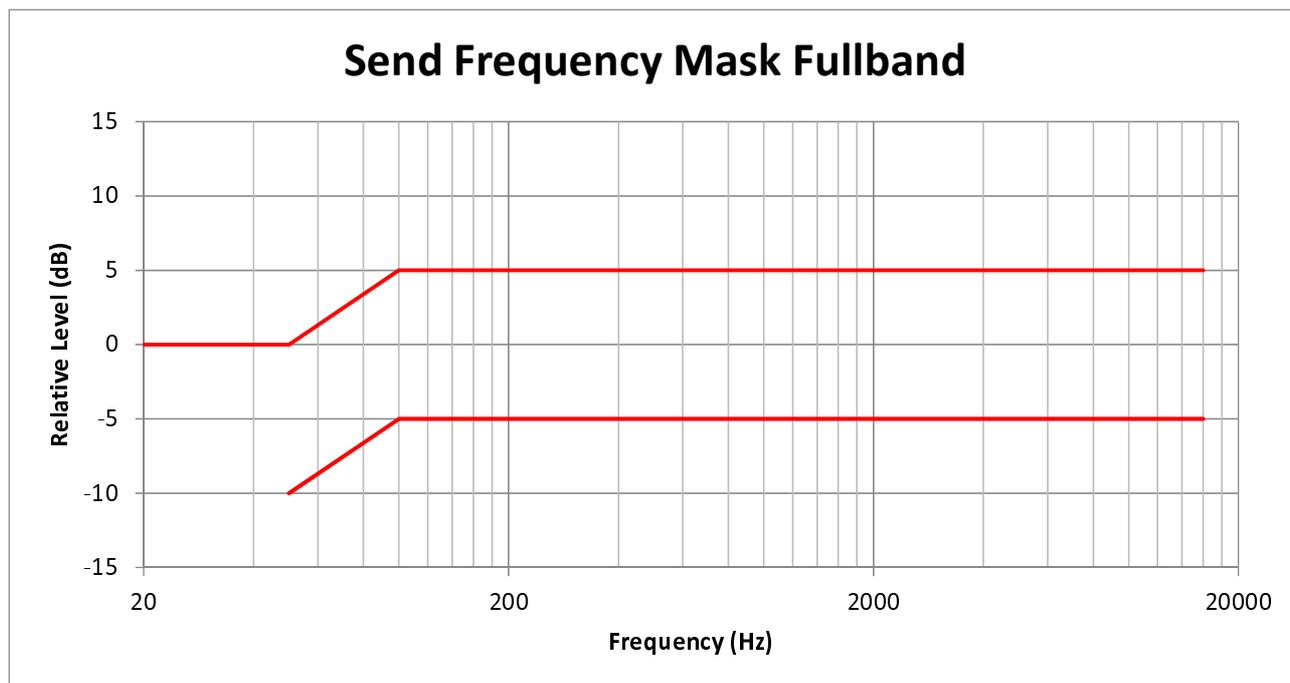
**Figure 5: Send frequency response mask for Fullband**
