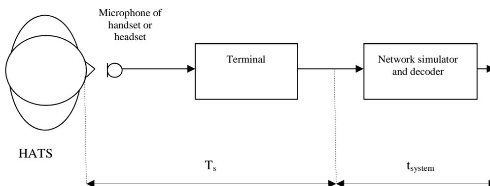
**Figure 10: Different blocks contributing to the delay in send direction**
