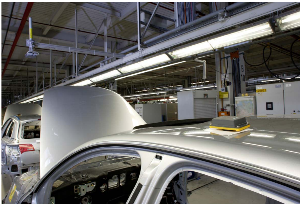
Figure 9: Typical production scenario in automotive industry with read range 1 metre to 2 metres
