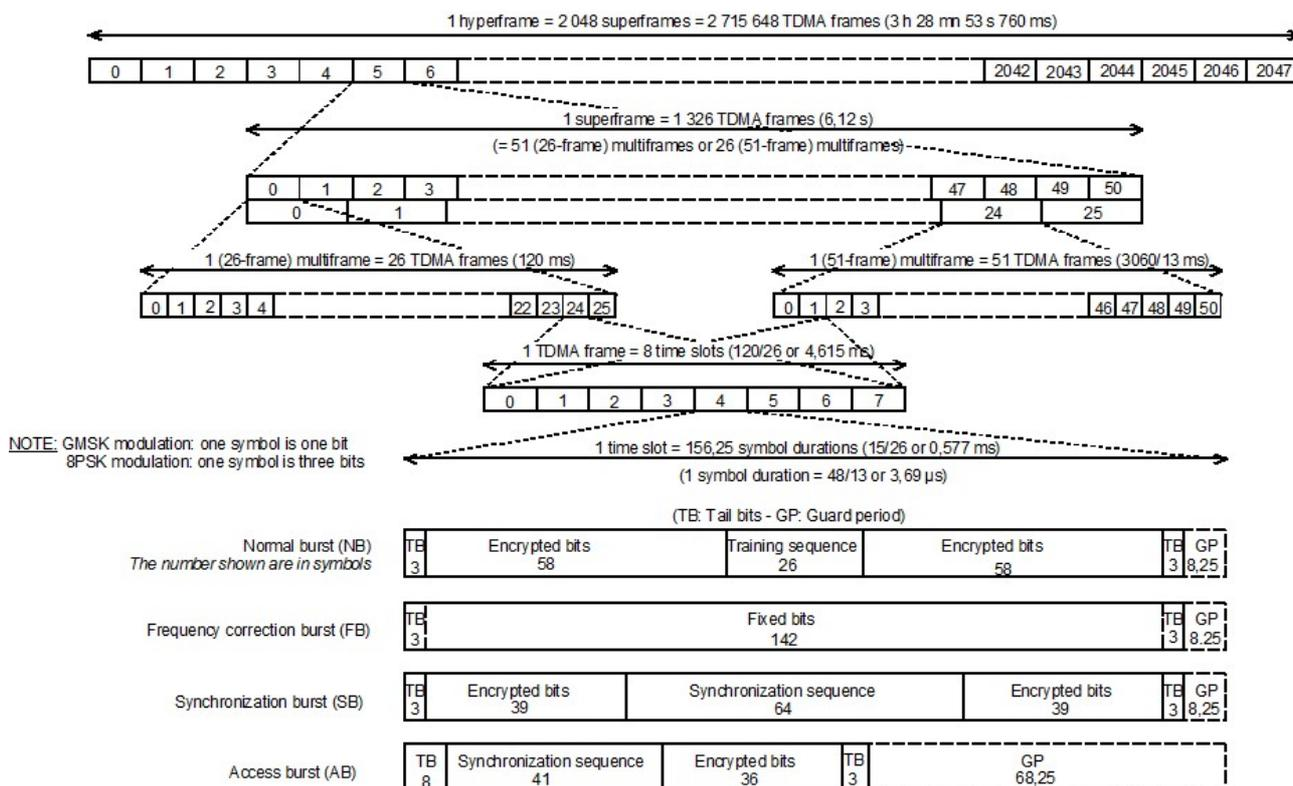
Figure 10: Overall Burst structure of a GSM System
