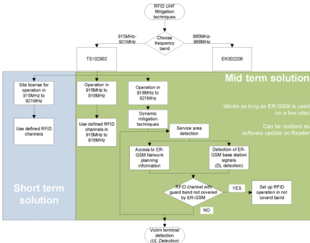
Figure 15: Short term and midterm solution for the sharing in the band 918 MHz to 921 MHz
