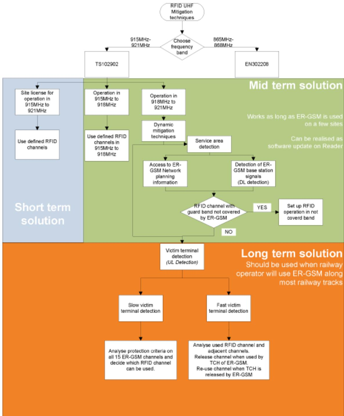
Figure 18: Overall coexistence strategy between ER-GSM and RFID
