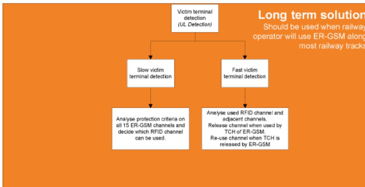
**Figure 17: Additional mechanisms for the long term solution for the sharing in the band 918 MHz and 921 MHz**
