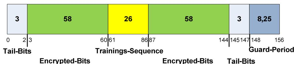
Figure 11: Burst structure of Normal Burst TCH and BCH
