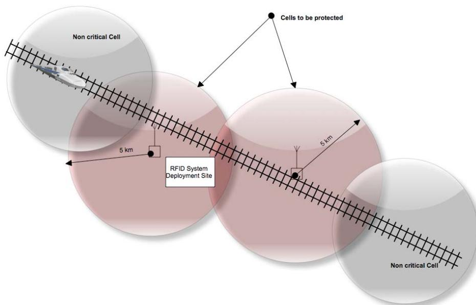
**Figure 16: ER-GSM network coverage**
