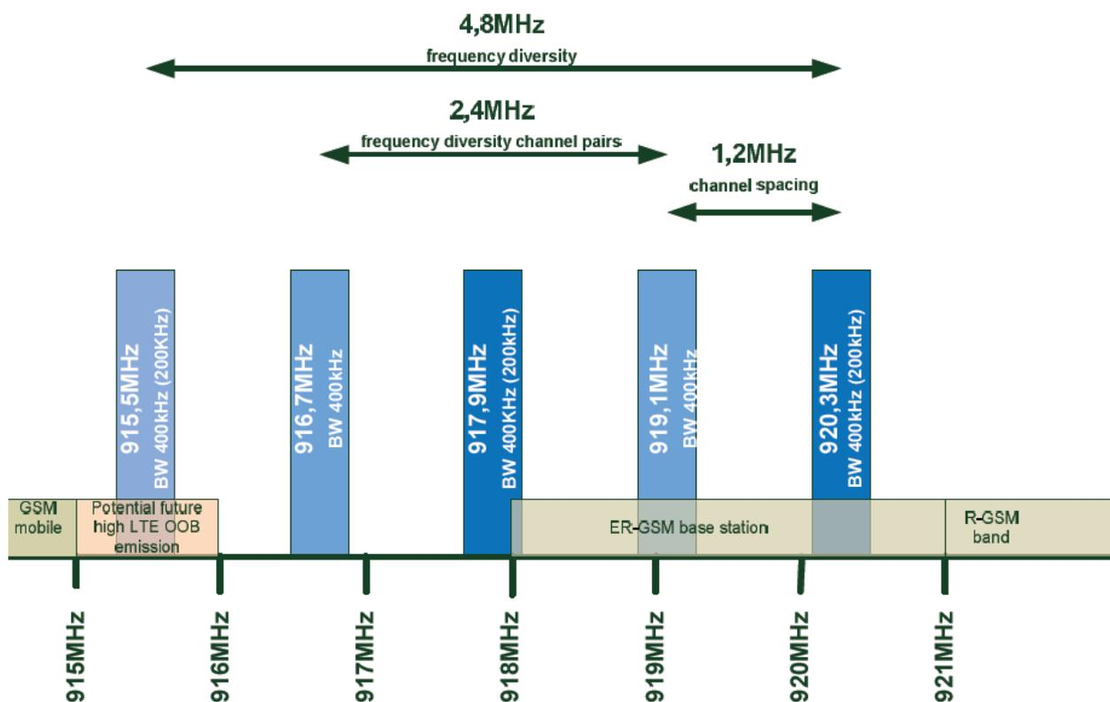
**Figure 1: Revised proposal for high performance RFID applications**
