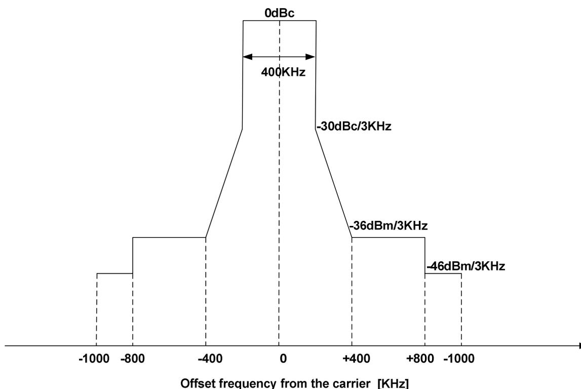
**Figure C.2: High performance interrogator channel mask**
