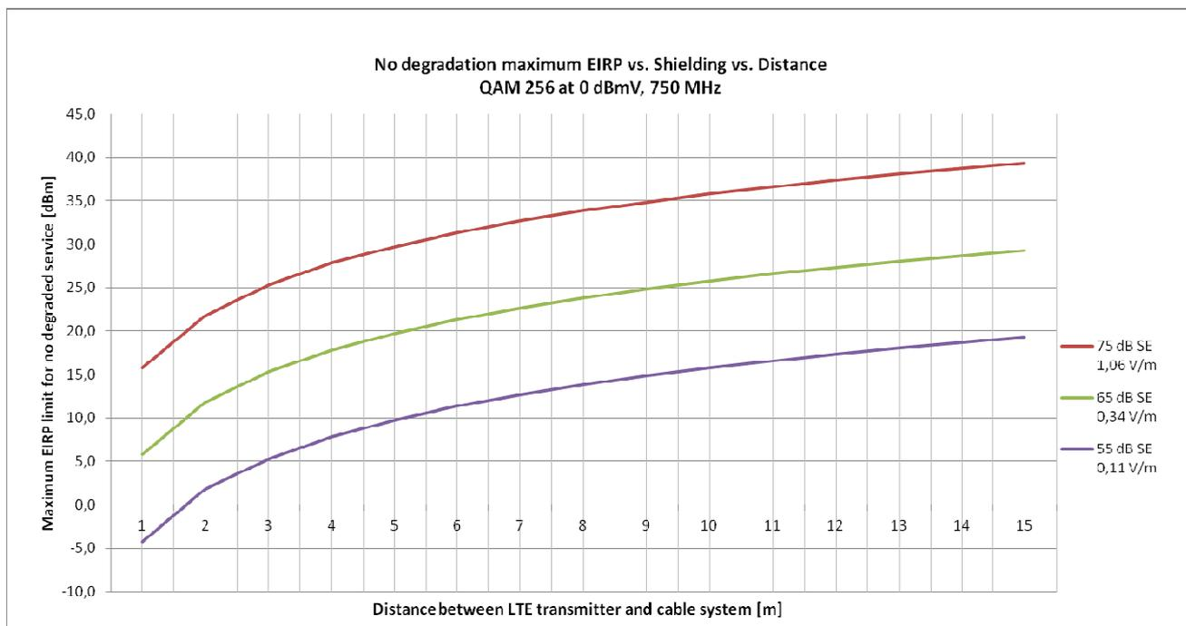
Figure 4a: Typical QAM 256 operation combined with low, medium and high shielding factors
