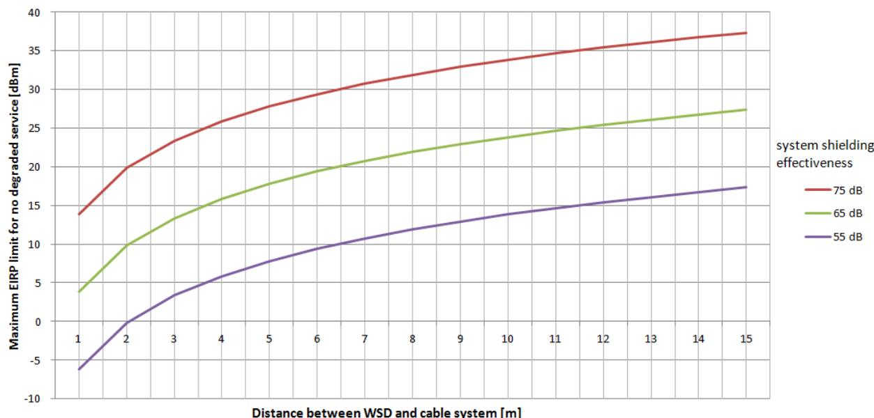
Figure 4b : Typical QAM 256 operation combined with low, medium and high shielding factors
