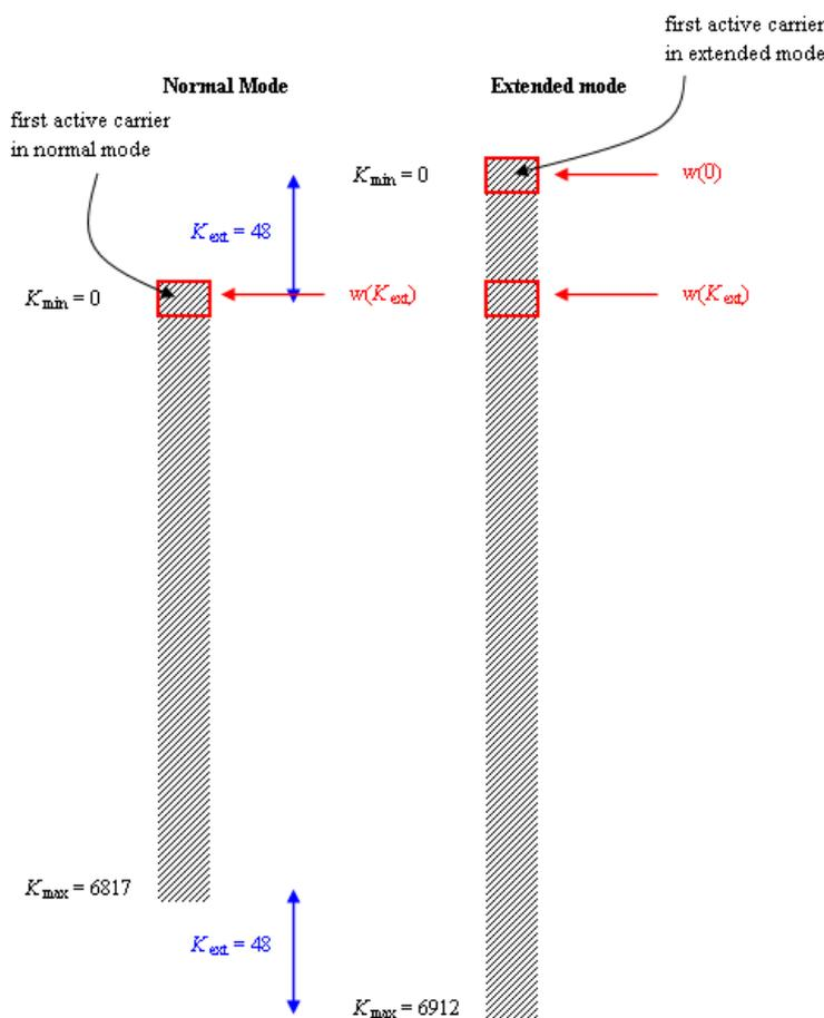
Figure 71: Modulation of the carriers in extended mode
