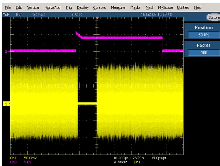
**Figure 55: Absolute timing test showing the zero P1 symbol in relation to the 1PPS edge**
