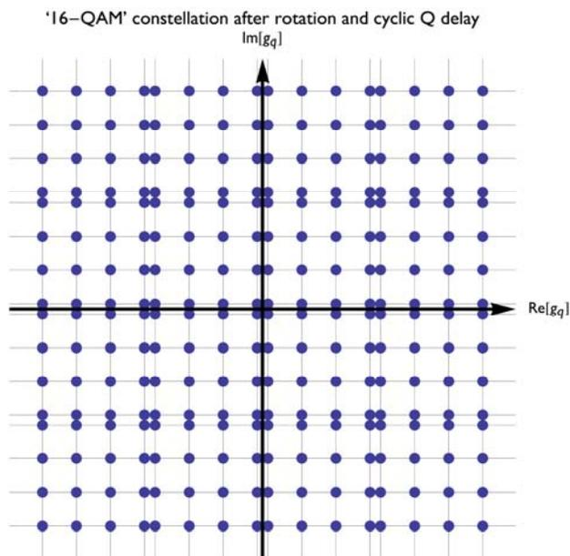
Figure 67: Resulting "virtual" 16-QAM constellation after rotation and cyclic delay
