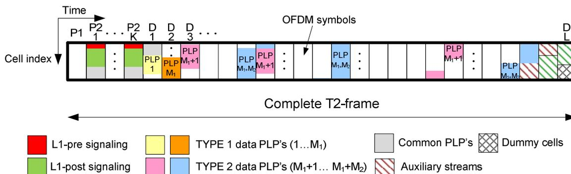
**Figure 19: Mapping of the L1 signalling, PLPs and auxiliary streams into the T2-frame**
