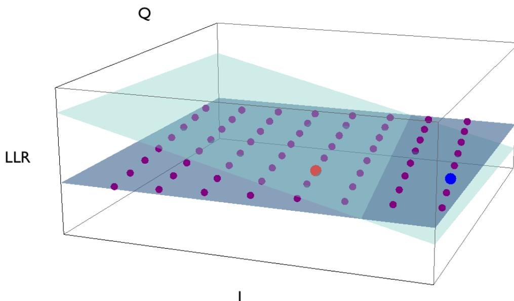
**Figure 99: an example of the 'Genie-aided' LLR calculation for rotated-64-QAM.**
