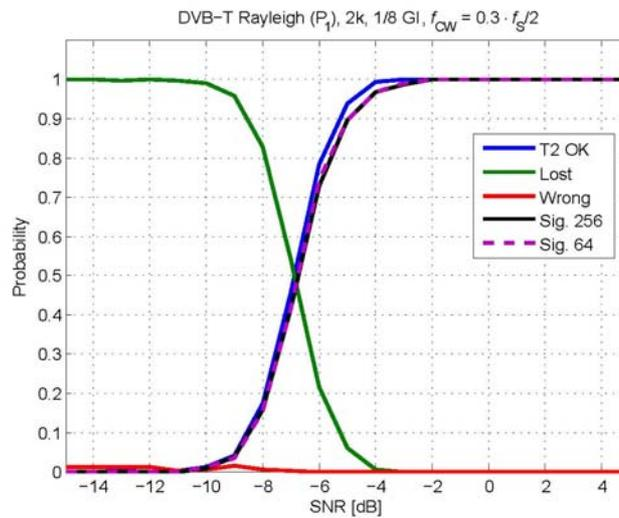
Figure 107: P1 robustness in Rayleigh channel (P1)
