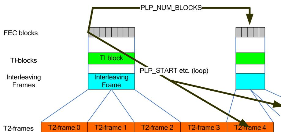
Figure 46(b): In-band signalling for  $P_1 = 2$ ,  $I_{\text{JUMP}} = 2$ ,  $N_{\text{TI}} = 1$
