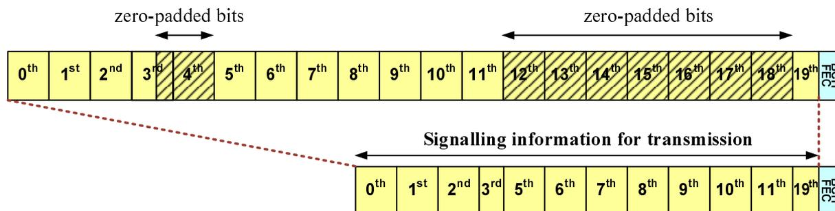
Figure 65: Example of removal of zero-padding bits
