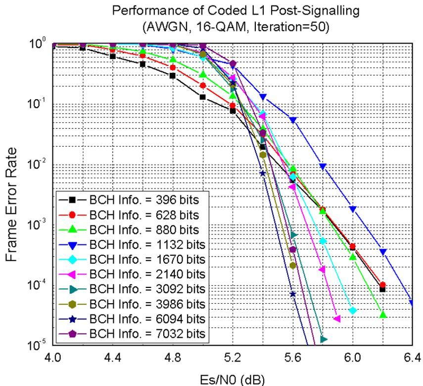
Figure 112: Performance of L1 Post (16QAM, AWGN channel)
