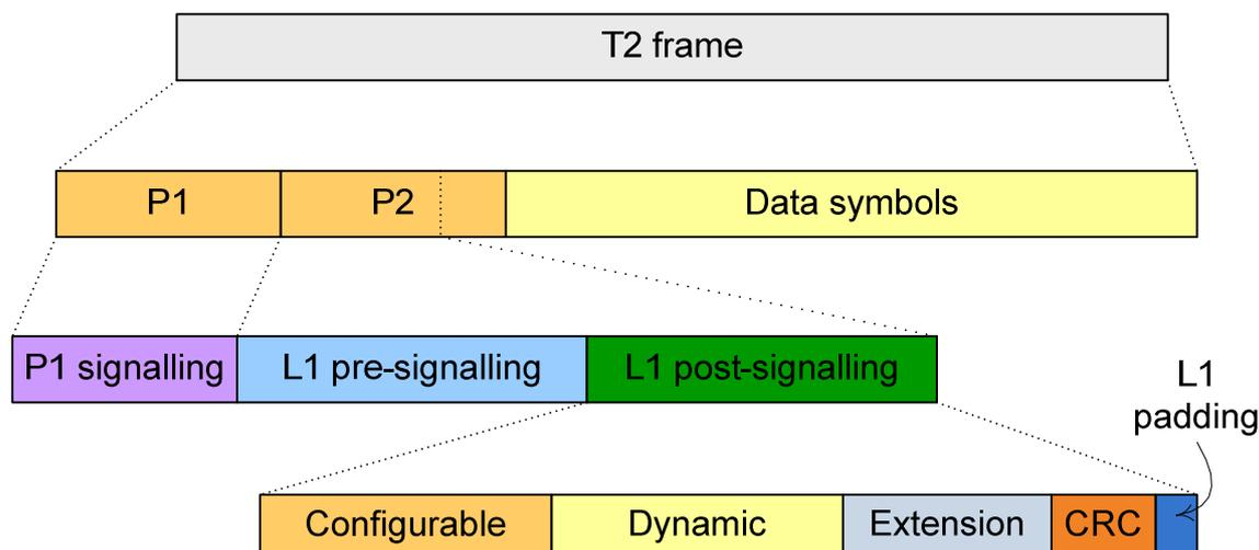
**Figure 43: The L1 signalling structure**
