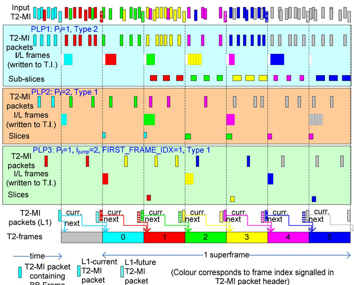
NOTE: The PLPs in figure 52 belong to different PLP groups. The transmission delay for all three PLPs, as discussed in 8.6.1.2.5, is equal to  $T_F$ .
