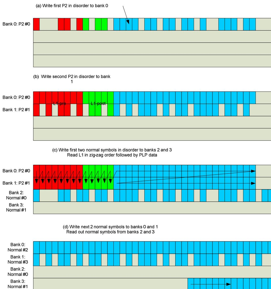
Figure 91: Combined L1/Frequency de-interleaver
