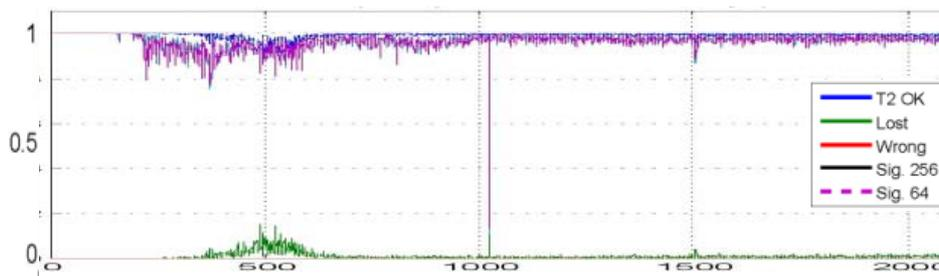
Figure 109: P1 robustness in 0 dB 180° Echo channel (SNR=0 dB)
