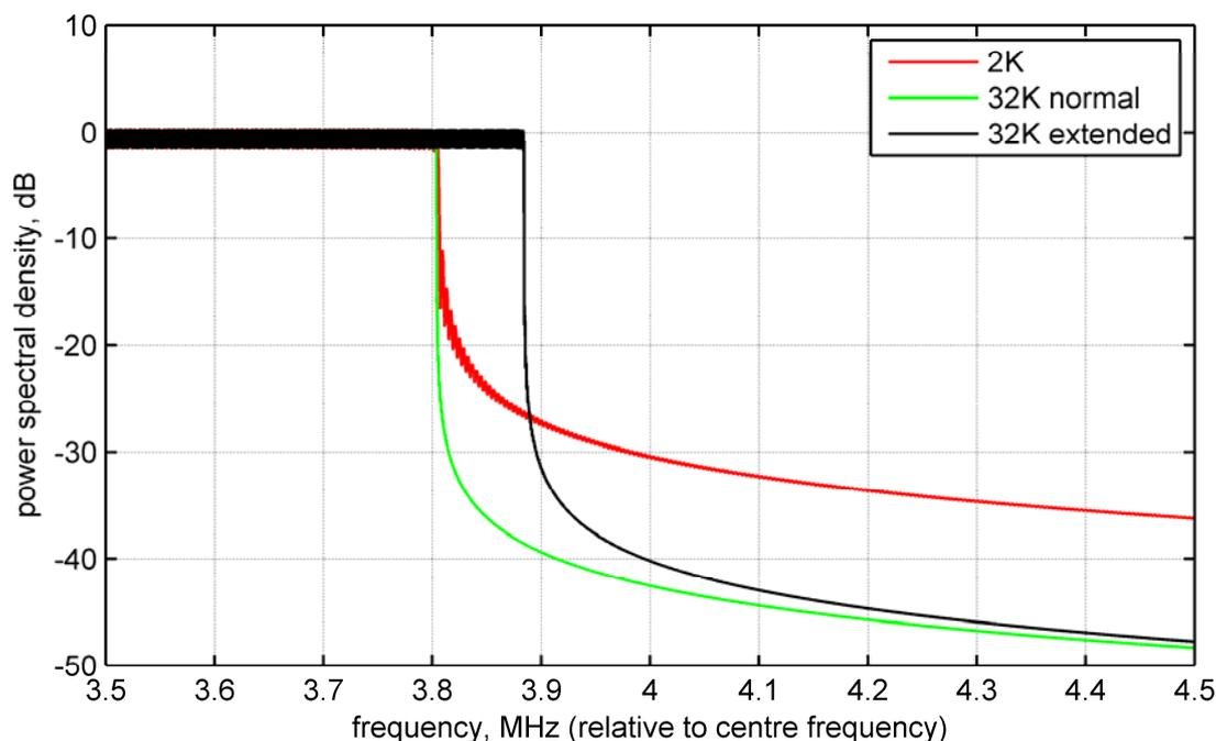
NOTE 1: The spectrum shown in figure 15 assumes that random data is sent in every OFDM cell. The presence of pilot information will cause some fine-detail variations in the wanted signal band. The choice of guard-interval fraction will affect the depth of the ripple in the wanted band (it increases as the guard-interval fraction increases) and also the ripples at the band edge.
