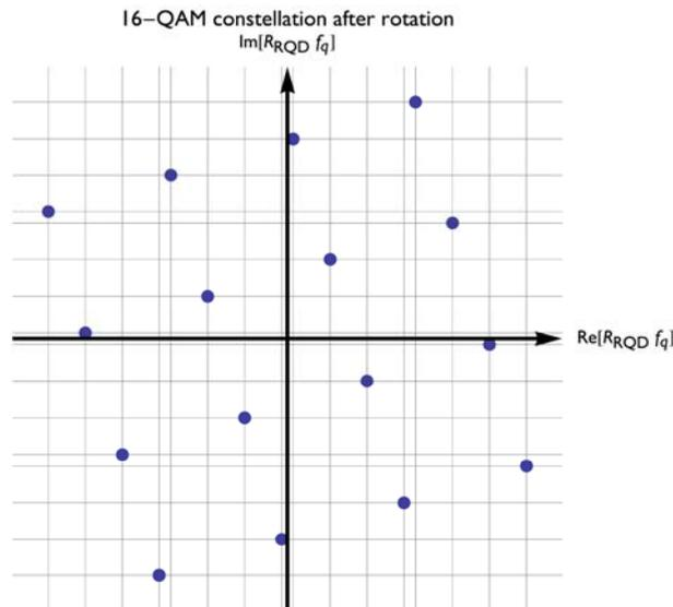
Figure 10: Rotated 16-QAM constellation
