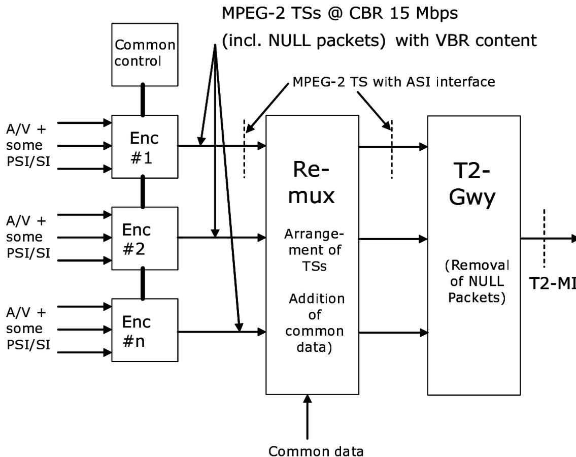
**Figure 30: Example of separate TSs with common control**
