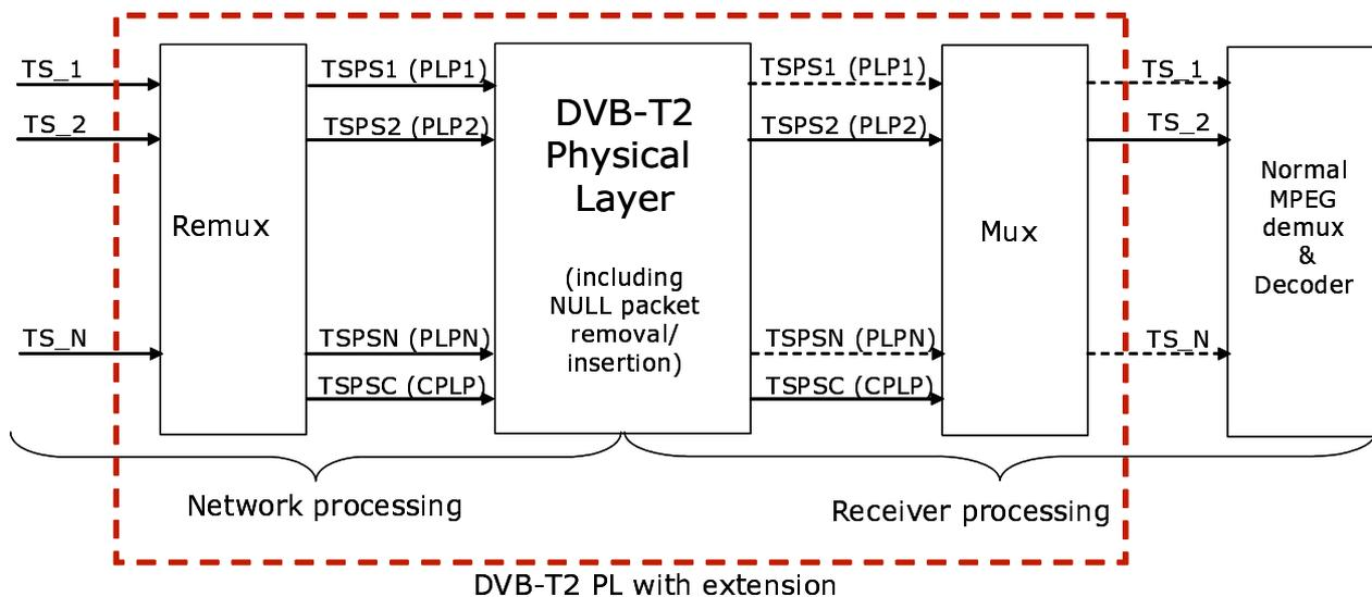
**Figure 31: Multiple TS input/output to/from the extended DVB-T2 PL**
