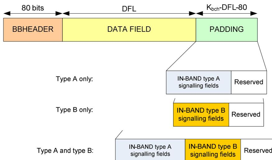
**Figure 45: PADDING format at the output of the STREAM ADAPTER for in-band type A**
