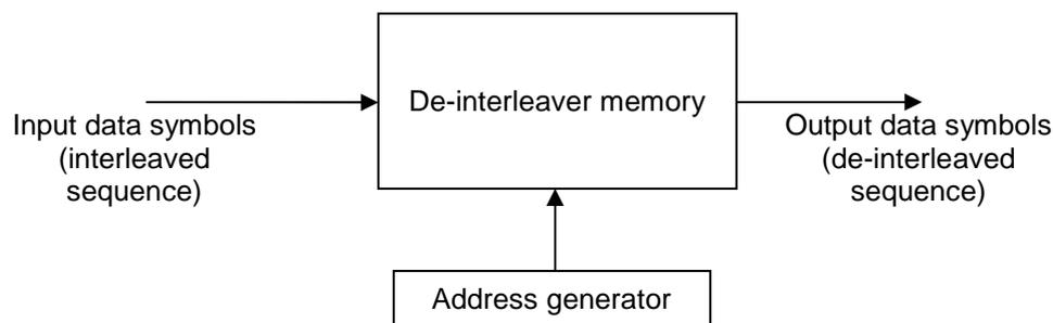
**Figure 93: De-interleaver block diagram**
