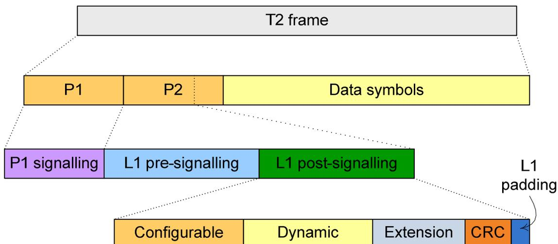
**Figure 101: The L1-signalling structure**
