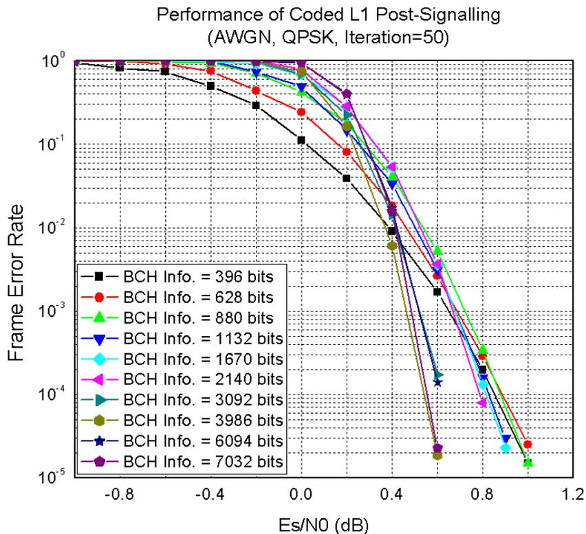
Figure 111: Performance of L1 Post (QPSK, AWGN channel)
