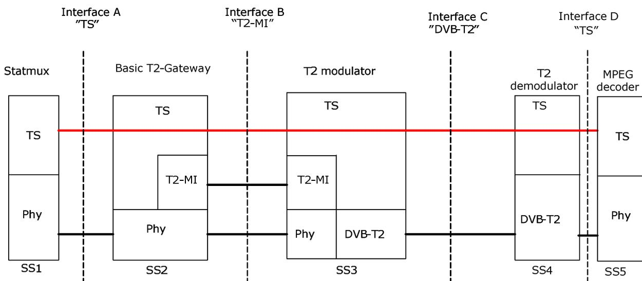
Figure 2: Reference protocol stacks for DVB-T2 (MPEG-2 TS case)
