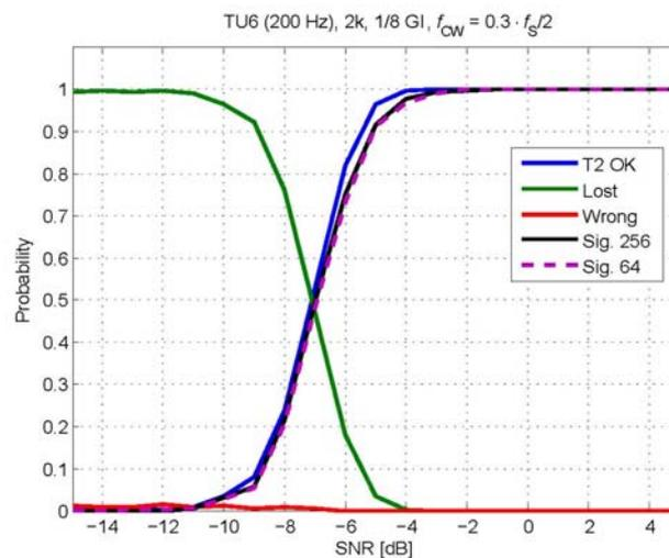
Figure 108: P1 robustness in Tu-6@200Hz channel
