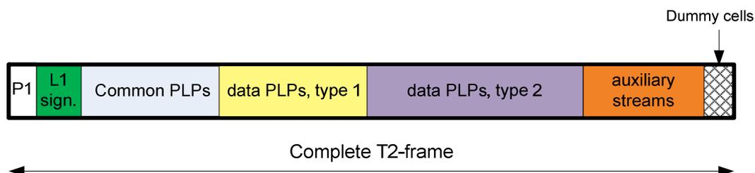
**Figure 18: Structure of the T2-frame**
