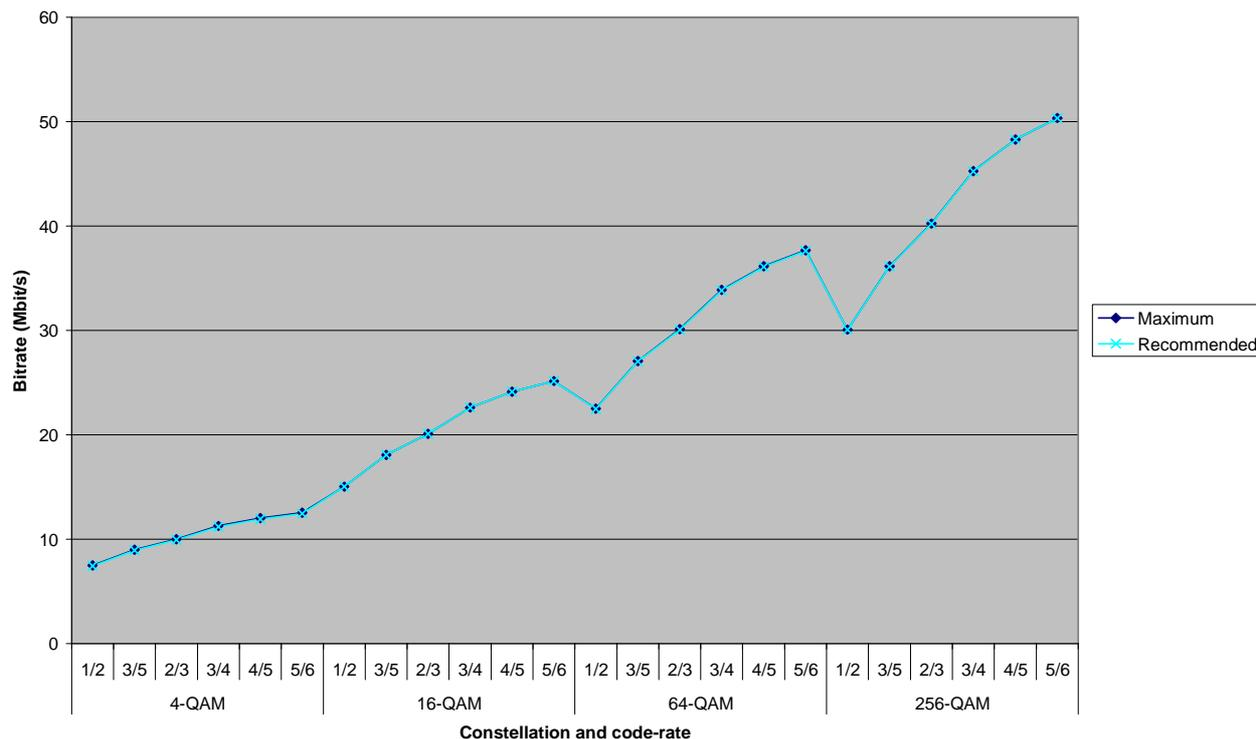
**Figure 27: Maximum bitrate and bitrate for recommended configuration with 8 MHz bandwidth and 32 K PP7**
