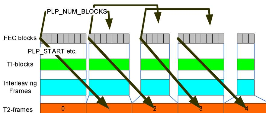
Figure 46(a): In-band signalling for  $P_1 = 1$ ,  $I_{\text{JUMP}} = 1$ ,  $N_{\text{TI}} = 1$
