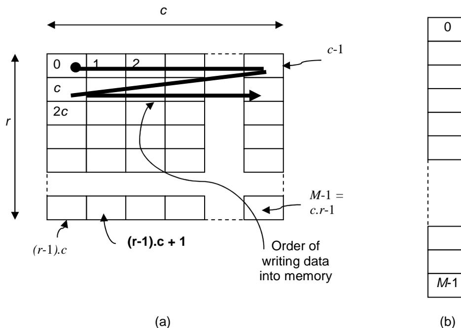
**Figure 94: Implementation of de-interleaver memory, showing (a) the conceptual implementation with rows and columns which defines the de-interleaving sequence and (b) the actual implementation as a sequential block of memory**
