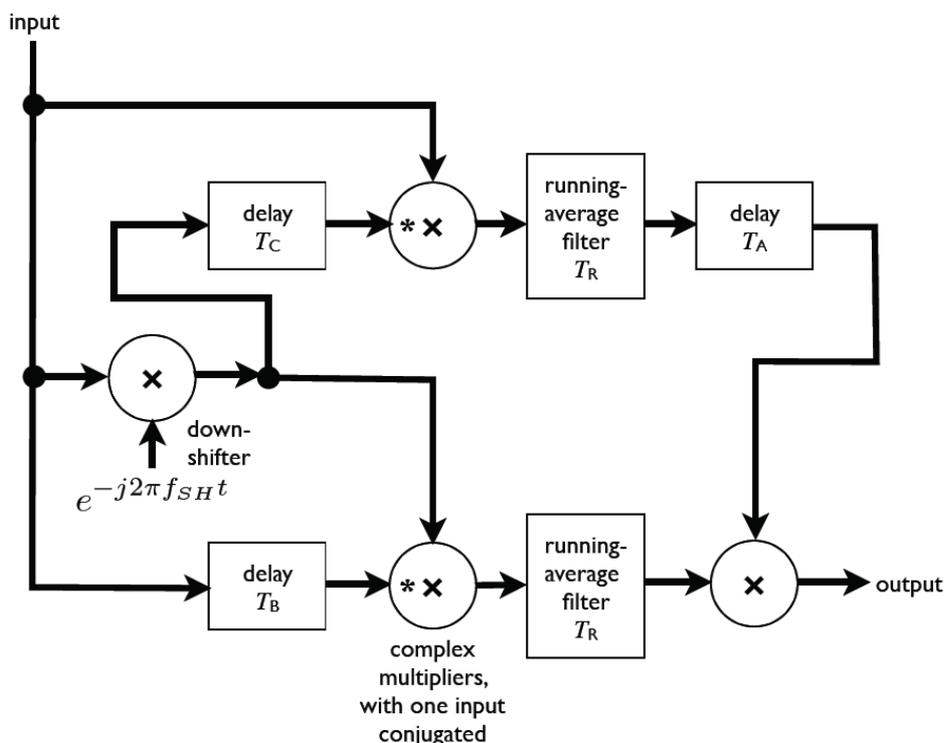
**Figure 81: Correlation for the P1 Detection (Block diagram)**
