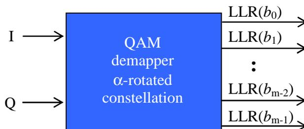
Figure 96: 2D LLR demapper for rotated constellations
