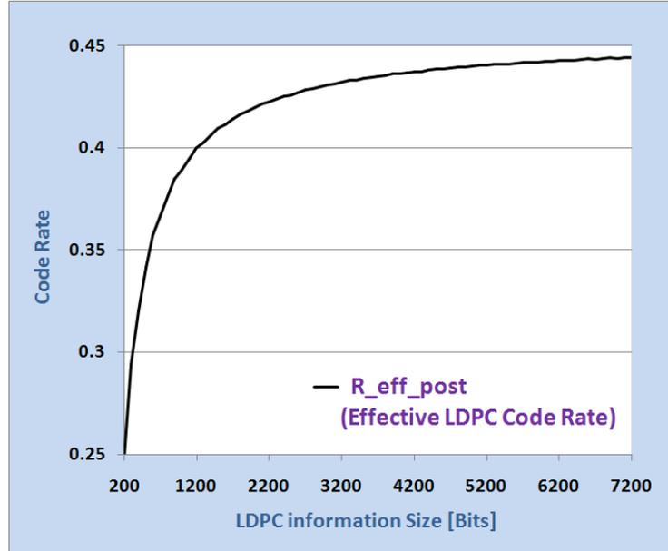
**Figure 64: Effective LDPC code rate  $R_{\text{eff\_post}}$  with  $(N_{P2} = 2, \eta_{\text{MOD}} = 6)$**
