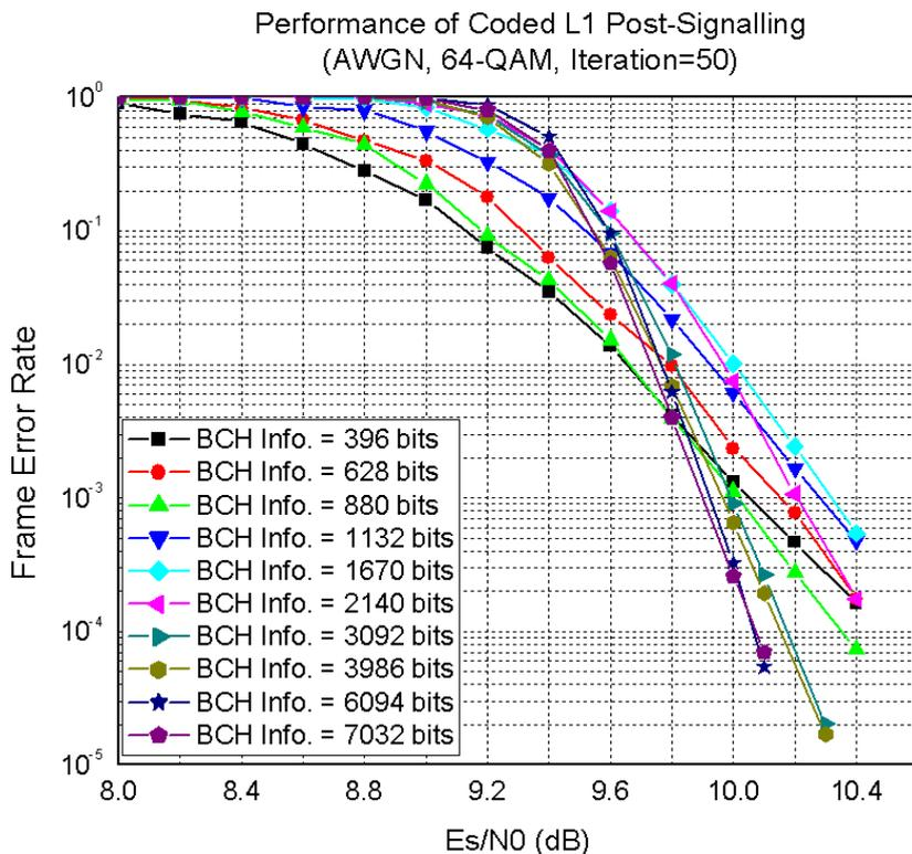
Figure 113: Performance of L1 Post (64QAM, AWGN channel)
