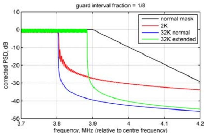
Figure 6: Power-spectral-density roll-off at the band edges for 2 K and 32 K
