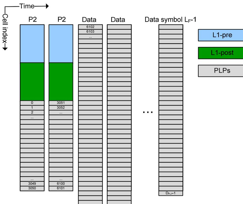
**Figure 24: Addressing of the OFDM cells for common PLPs and data PLPs**
