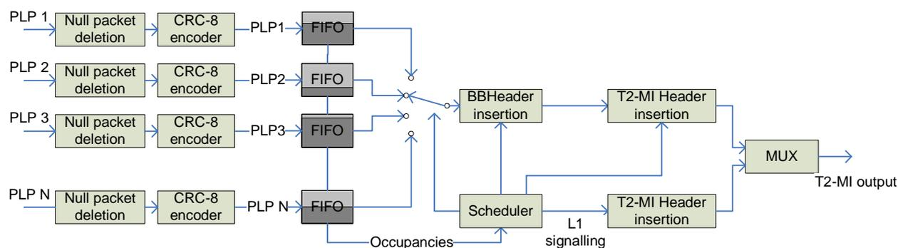
Figure 35: Block diagram for FEC block allocation models
