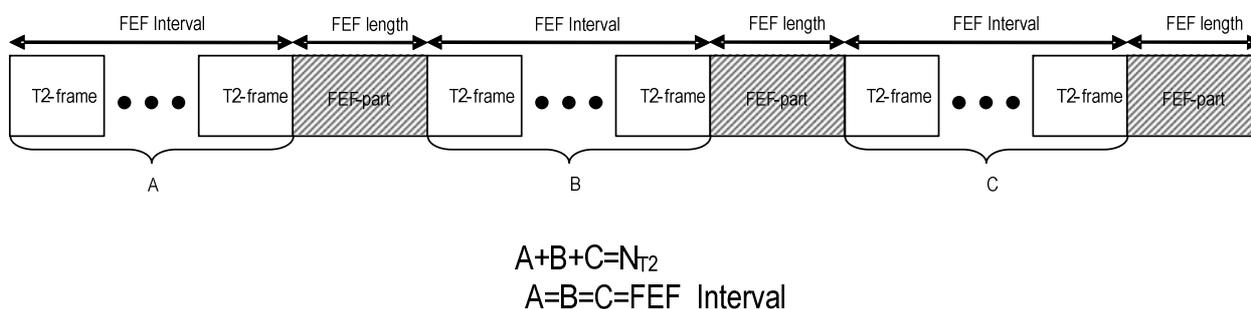
**Figure 25: The super-frame, including T2-frames and FEF parts**
