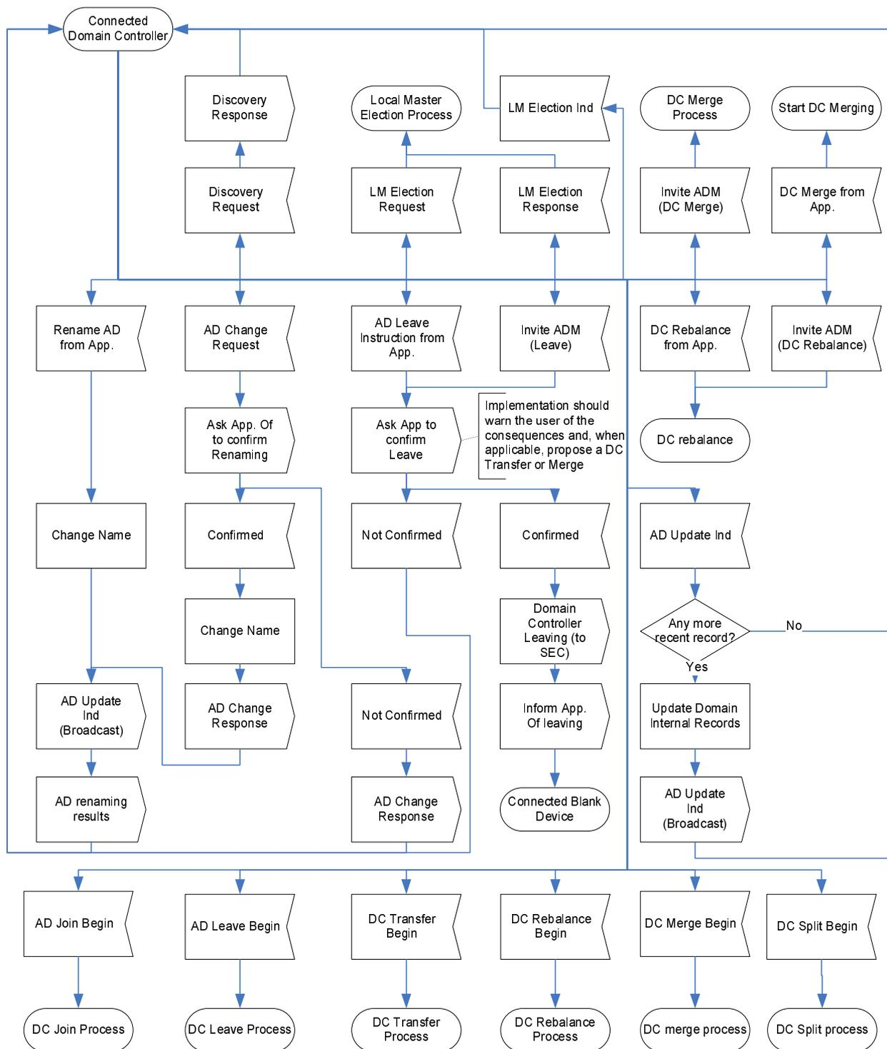
Figure 9: Connected Domain Controller State Machine
