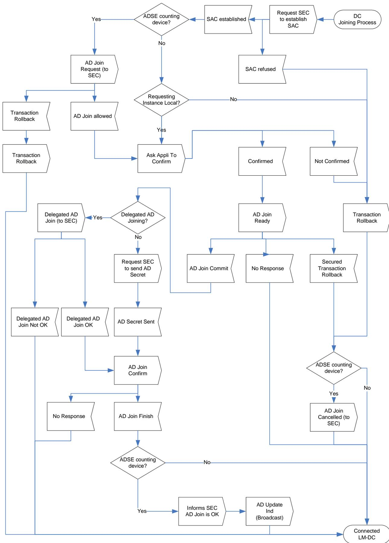
Figure 17: Domain Controller in AD Joining Process
