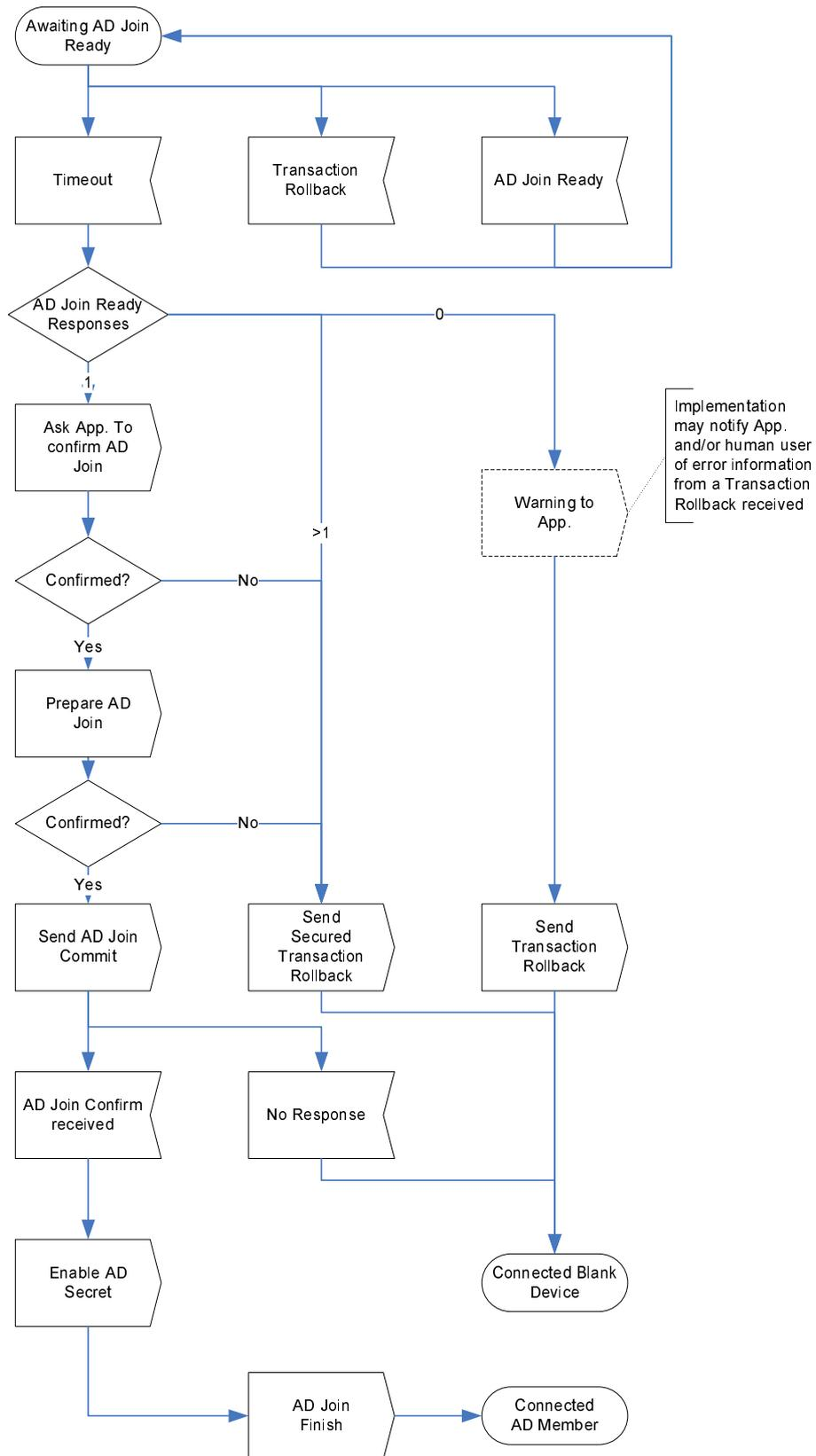
Figure 15: Blank Instance Joining an AD
