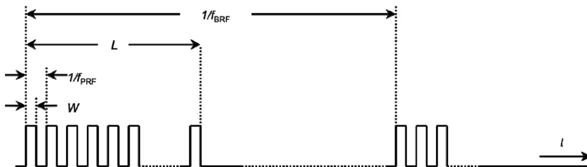
**Figure D.5: General structure of the bursts for DAA radiolocation test transmissions**
