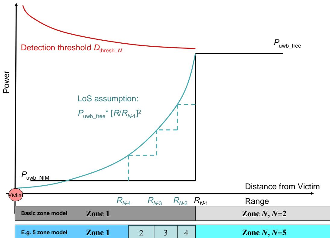
**Figure 3: Illustration of multi zone concept based on equivalent protection levels**
