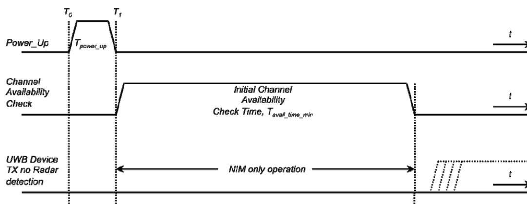
Figure D.1: Example of timing for radiolocation testing of the Minimum Initial Channel Availability Check Time  $T_{\text{avail\_time}}$ , UWB DAA device intent to operate in a non NIM mode
