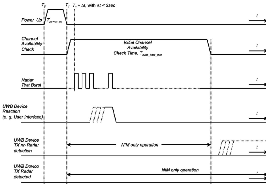
Figure D.2: Example of timing for radiolocation testing at the beginning of the Minimum Initial Channel Availability Check Time, UWB DAA radio device intent to operate in a non-NIM mode
