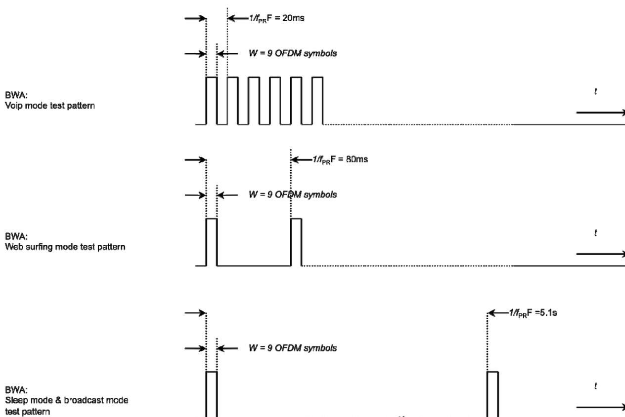
Figure E.1: Timing of BWA test signals
