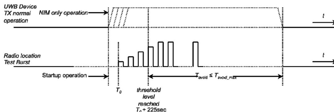
**Figure D.4: Example of timing for radiolocation signal in-operation testing of the Detect and Avoid Time, here with increasing Radiolocation test signal level larger than the threshold**
