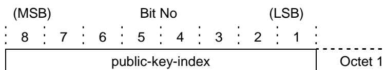
Figure 6.38: UEPositionRequest Signalling PDU (with PublicKeyIndex)
