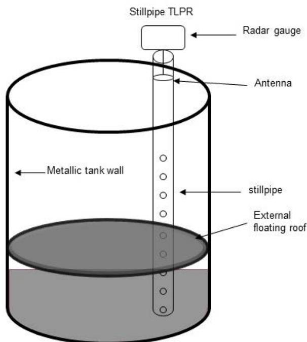
**Figure 2: Stillpipe TLPR installed on external floating roof tank to measure the level inside the tank**
