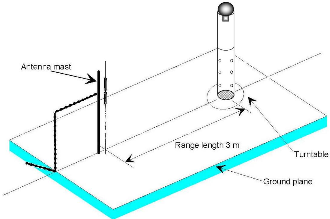
NOTE: Should the sensitivity not be sufficient, the measurement distance can be reduced to 1 m.
