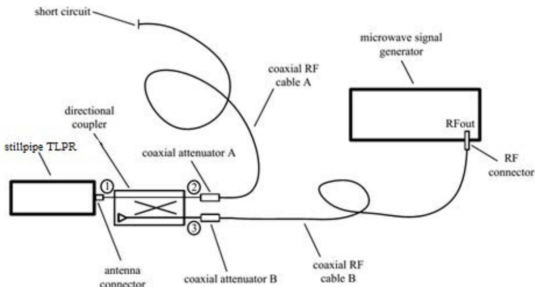
Figure 4: Conducted test setup for the equivalent scenario using coaxial components
