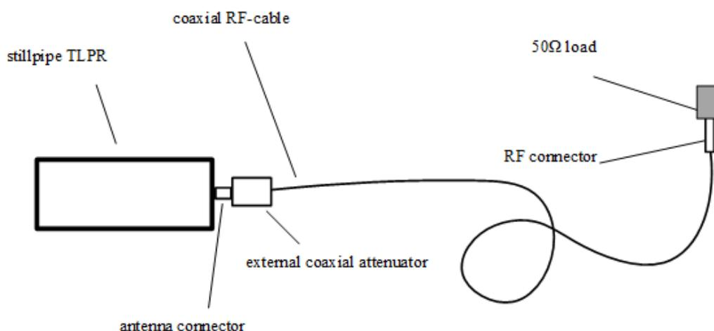
**Figure 6: Conducted test setup for Rx noise floor measurement without injection of interference signal**
