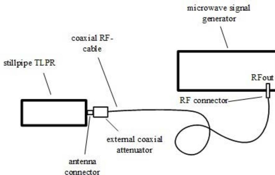
**Figure 5: Conducted test setup for Rx noise floor measurement with injection of interference signal**
