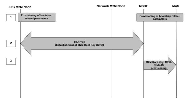
Figure 8.8: M2M Service Bootstrap using EAP-TLS over PANA
