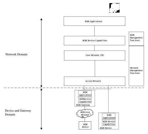
Figure 4.1: High level architecture for M2M
