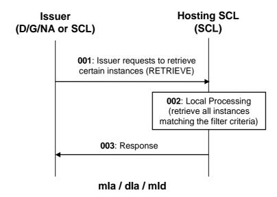
Figure 9.67: Message flow of procedure to read all instances matching filter criteria in a *<container>* resource
