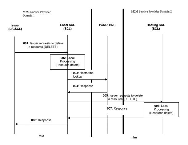
Figure 9.130: Message flow of procedure to delete a resource in another M2M Service Provider domain
