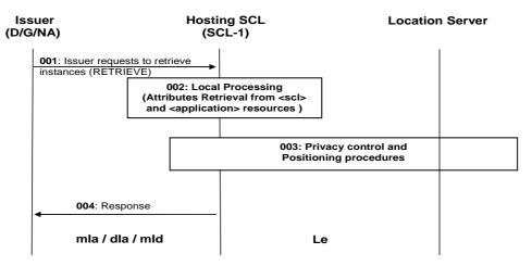
Figure 9.68: Illustration of Procedures for the case of location server based to read all instances in a < locationContainer > resource
