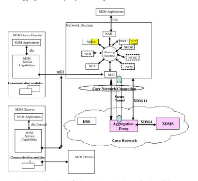
Figure D.1: Option 1 - Interworking XDMS- M2M Network Domain for different service providers
