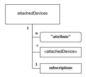
Figure 9.32: Structure of attachedDevices resource
