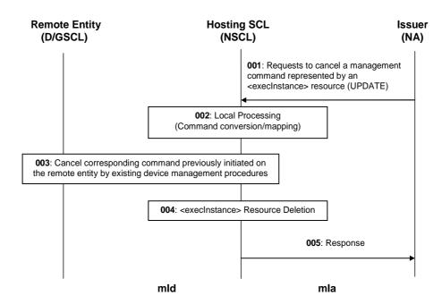
Figure 9.112: Illustration of procedures to cancel a management command execution instance on a remote entity
