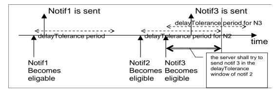
Figure 9.84: Notification mechanism, conflict resolution when multiple delayTolerance are used
