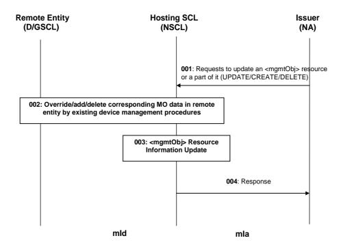
Figure 9.99: Illustration of procedures to update an <mgmtObj> resource or its sub-resource by an M2M NA
