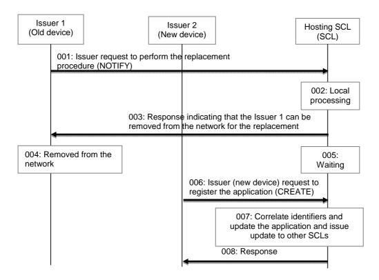
Figure 9.126: Procedures for application replacement initiated from the device
