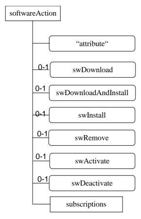
Figure B.23: Structure of the softwareAction resource
