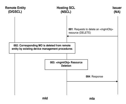
Figure 9.101: Illustration of procedures to delete an <mgmtObj> resource by NA
