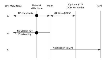
Figure 8.9: Call flow for Automated Bootstrapping using Device-Certificate TLS over TCP
