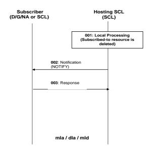
Figure 9.89: Procedures for asynchronous notification in case of deletion of subscribed resource
