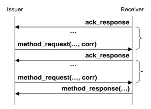
Figure 9.42: Client-2-server mode delayed Response
