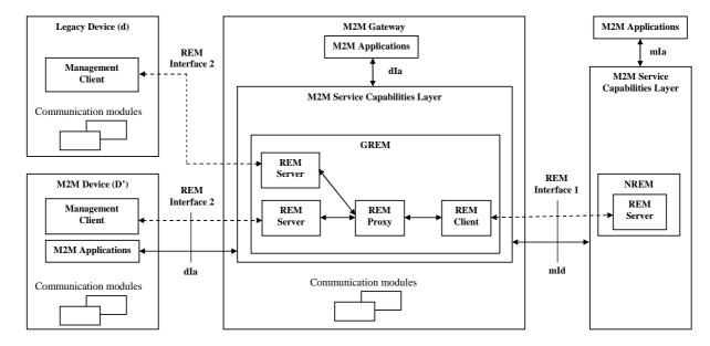
Figure E.2: Integrated Reference Architecture for Managing M2M Devices behind M2M Gateway
