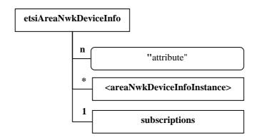
Figure B.28: Structure of the etsiAreaNwkDeviceInfo resource
