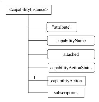
Figure B.8: Structure of the <capabilityInstance> resource
