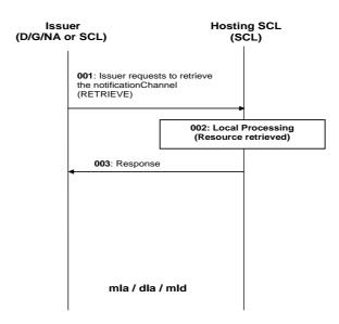
Figure 9.114: Procedures for <notificationChannel> retrieve
