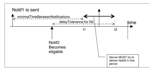
Figure 9.86: Notification mechanism, no conflict between the subscription minimalTimeBetweenNotification and the resource instance delayTolerance
