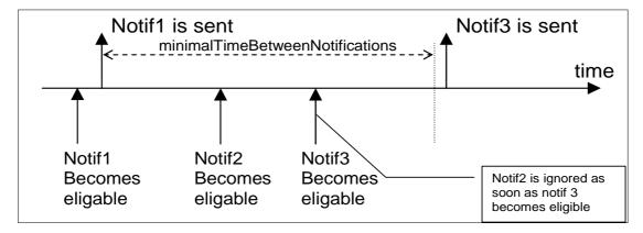
Figure 9.82: Notification mechanism when minimalTimeBetweenNotifications is used, the case when more than one notification become eligible
