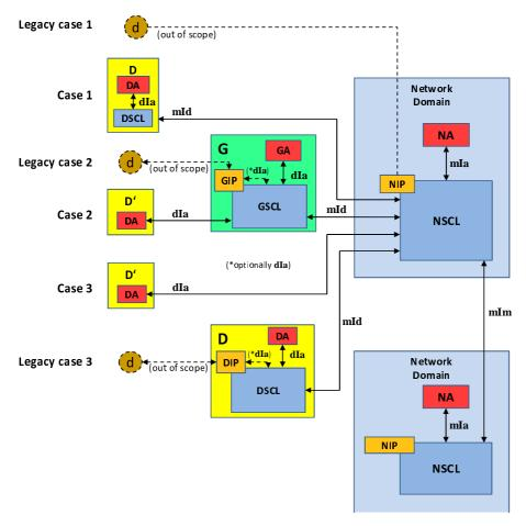
Figure 6.1: Mapping of reference points to different deployment scenarios
