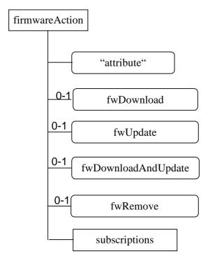
Figure B.20: Structure of the firmwareAction resource
