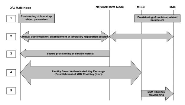
Figure 8.7: M2M Service Bootstrap using IBAKE over EAP over PANA
