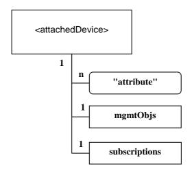
Figure 9.33: Structure of <attachedDevice> resource
