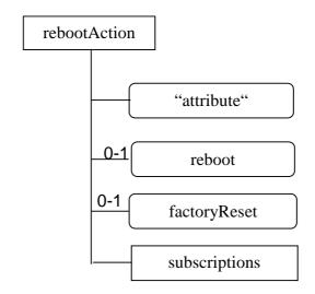
Figure B.25: Structure of the rebootAction resource
