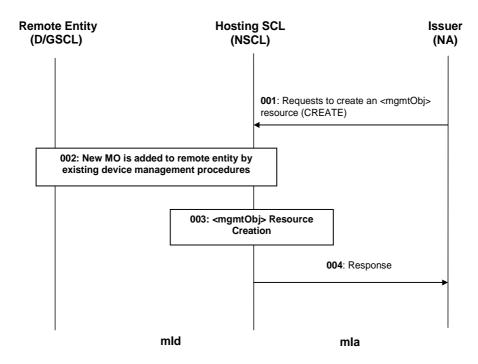
Figure 9.95: Illustration of procedures to create an <mgmtObj> resource by NA
