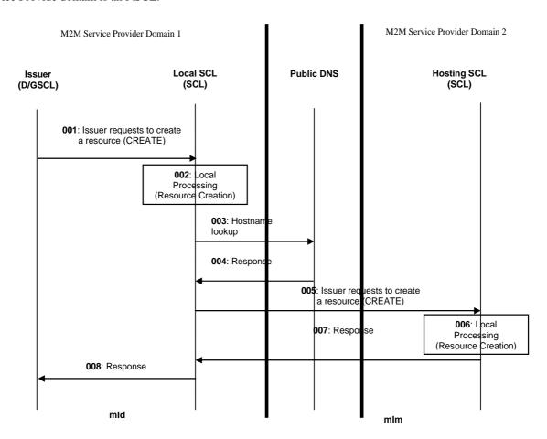
Figure 9.127: Message flow of procedure to create a resource in another M2M Service Provider domain
