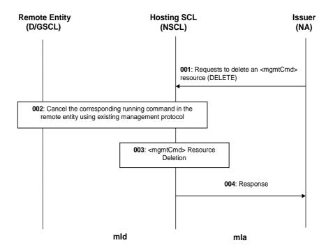
Figure 9.108: Illustration of procedures to delete an <mgmtCmd> resource by NA
