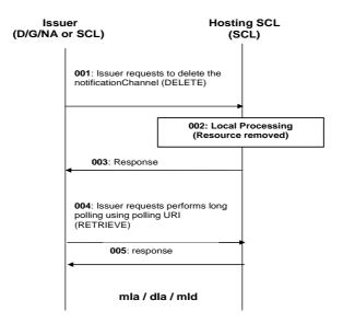
Figure 9.115: Procedures for <notificationChannel> delete
