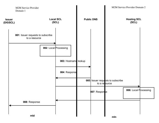
Figure 9.131: Message flow of procedure to subscribe to a resource in another M2M Service Provider domain
