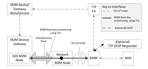
NOTE: The line through the Network M2M Node indicates that the Network M2M Node passes messages between D/G M2M Node and MSBF with some procedure-dependent processing at the Network M2M Node.
