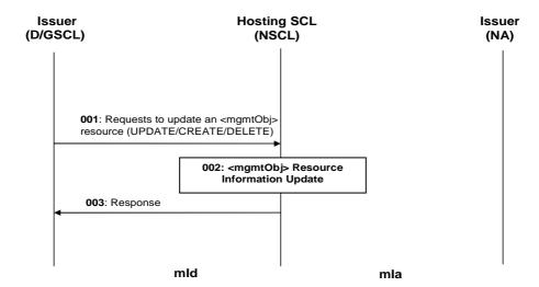
Figure 9.98: Illustration of procedures to update an <mgmtObj> resource by a D/GSCL
