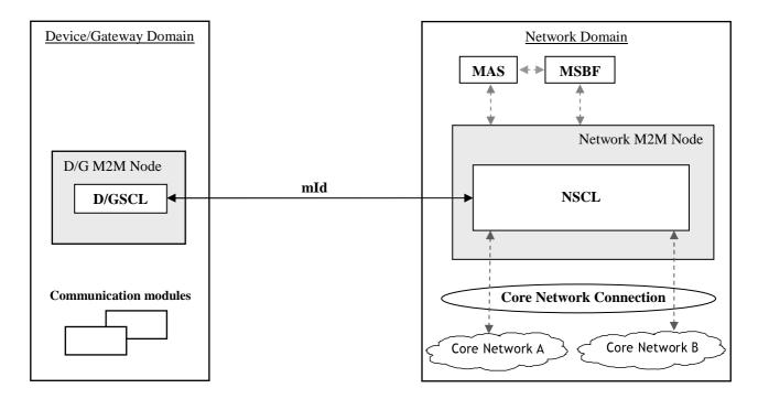
Figure 8.1: Functional architecture elements for bootstrapping
