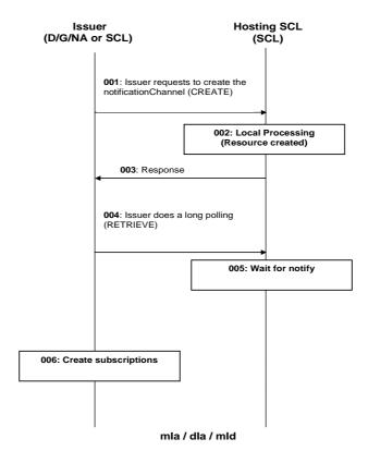
Figure 9.113: Procedures for <notificationChannel> create
