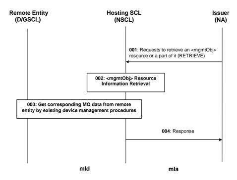
Figure 9.97: Illustration of procedures to retrieve an <mgmtObj> resource by an M2M NA
