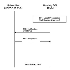
Figure 9.88: Procedures for asynchronous notification
