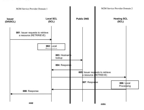
Figure 9.128: Message flow of procedure to retrieve a resource in another M2M Service Provider domain
