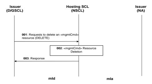
Figure 9.107: Illustration of procedures to delete an <mgmtCmd> resource by D/GSCL
