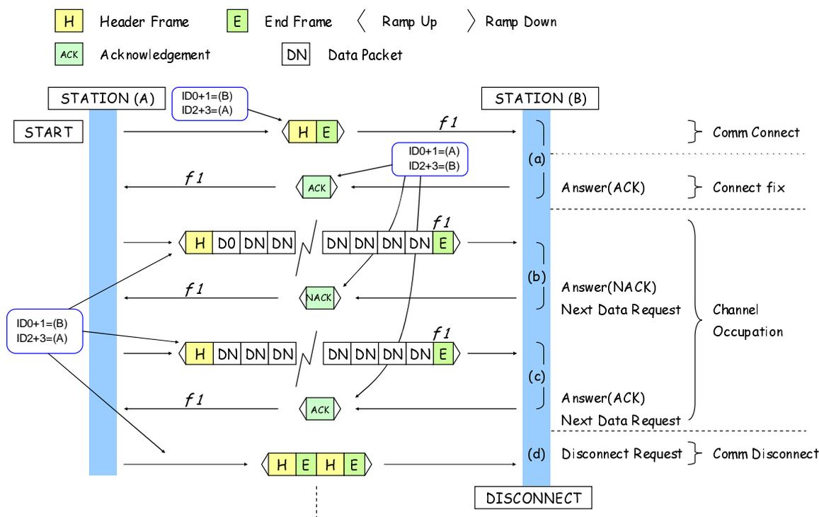
**Figure 9.3: Packet exchanges**
