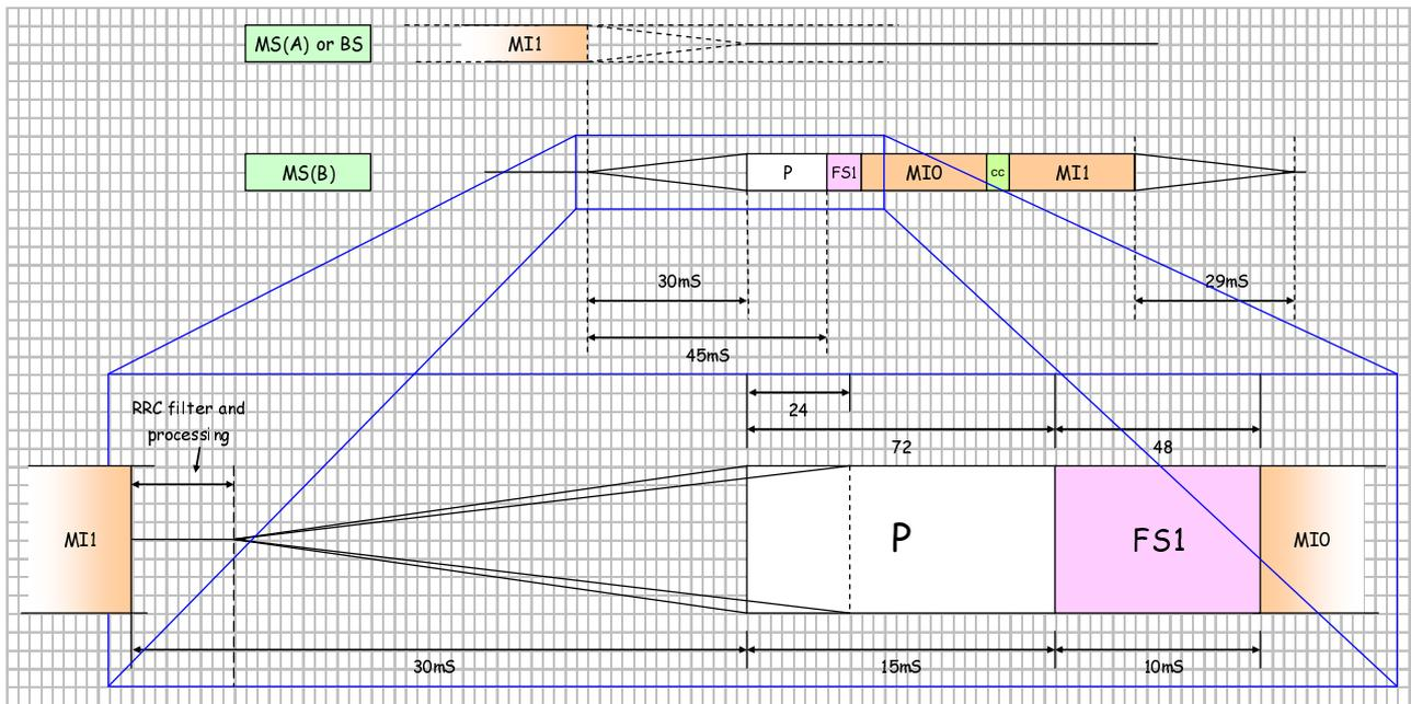
Figure 12.1: Preamble Timing
