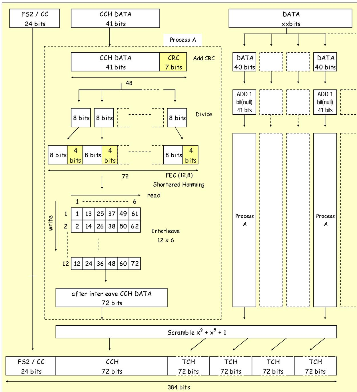
Figure 11.6: Type 2 data frame coding
