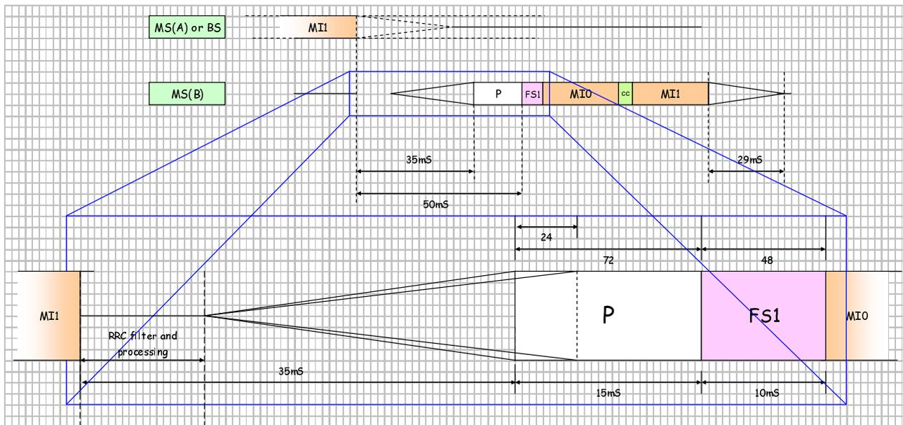
Figure 12.2: Message Profile for latest timing
