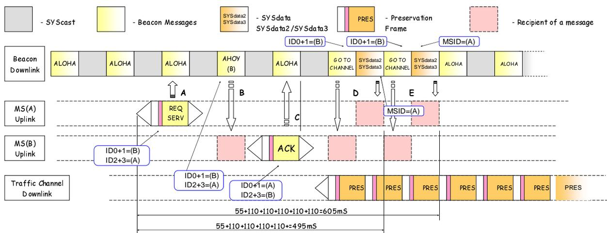
**Figure 4.25: Mode 3 Beacon Channel Individual Voice Call Set-up**
