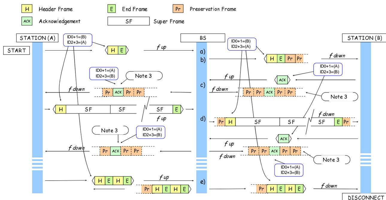
Figure 10.15: Mode 2 Individual data call exchanges
