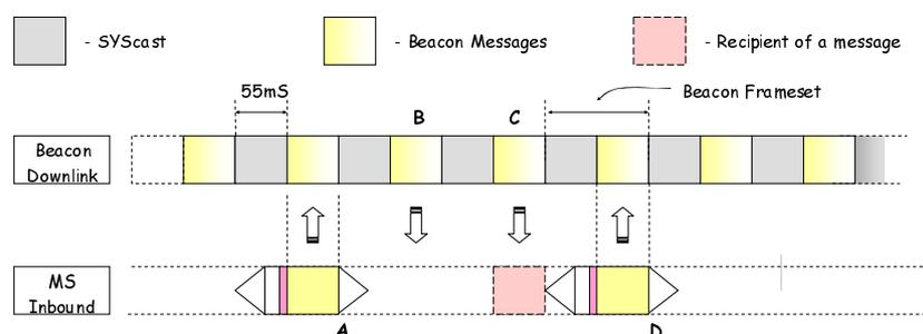
**Figure 12.6: Key points for a Mode 3 beacon channel**
