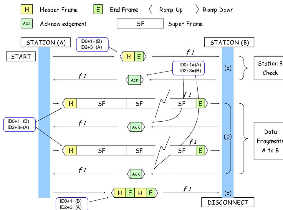
Figure 4.22: Mode 1 Individual data call exchanges
