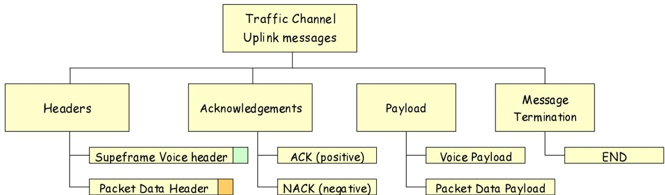
Figure 8.2: Uplink Traffic Channel Messages
