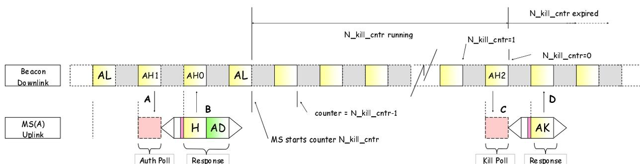
**Figure 10.46: Example of unsuccessful kill procedure**
