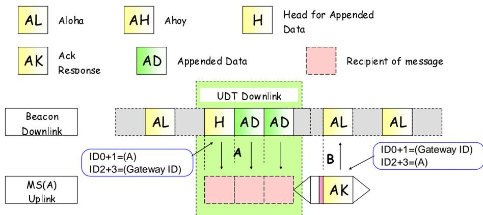
**Figure 10.48: Example of a Gateway/MS Dynamic Regroup Transaction**
