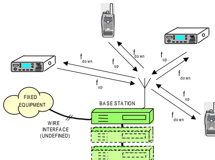
**Figure 4.4: Managed Centralized Repeater Network (Mode 3)**
