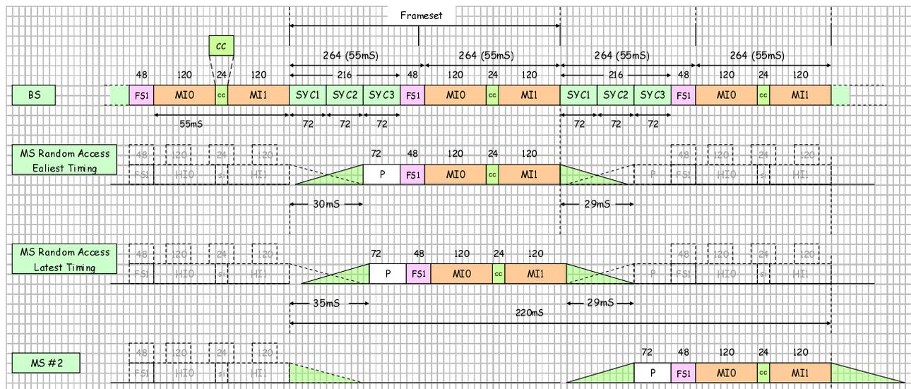
Figure 12.3: Message Timing Profile for Mode 3
