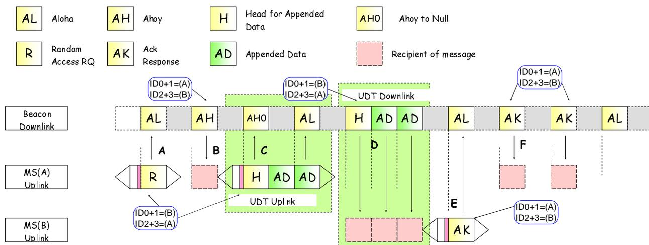
**Figure 10.47: Example of a MS/MS Dynamic Regroup Transaction**
