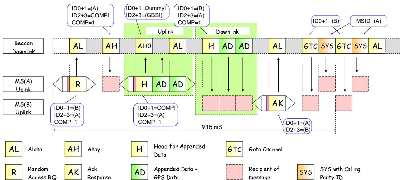
Figure 10.32: UDT mechanism carrying complementary data
