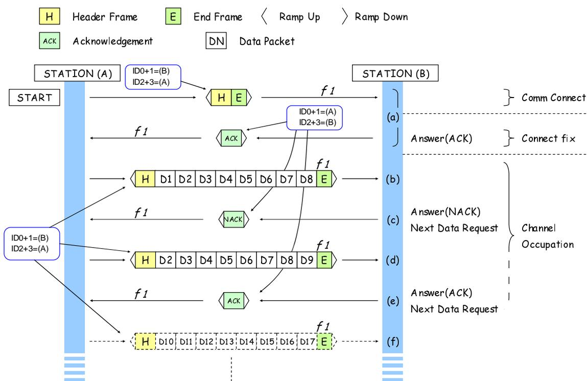
Figure 10.7: Packet Retransmissions
