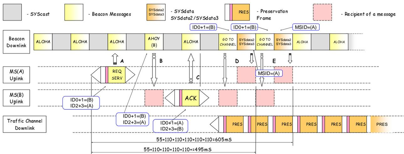
**Figure 10.27: Individual Call Set-up example**
