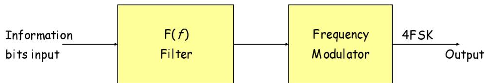
Figure 14.1: 4FSK Modulator
