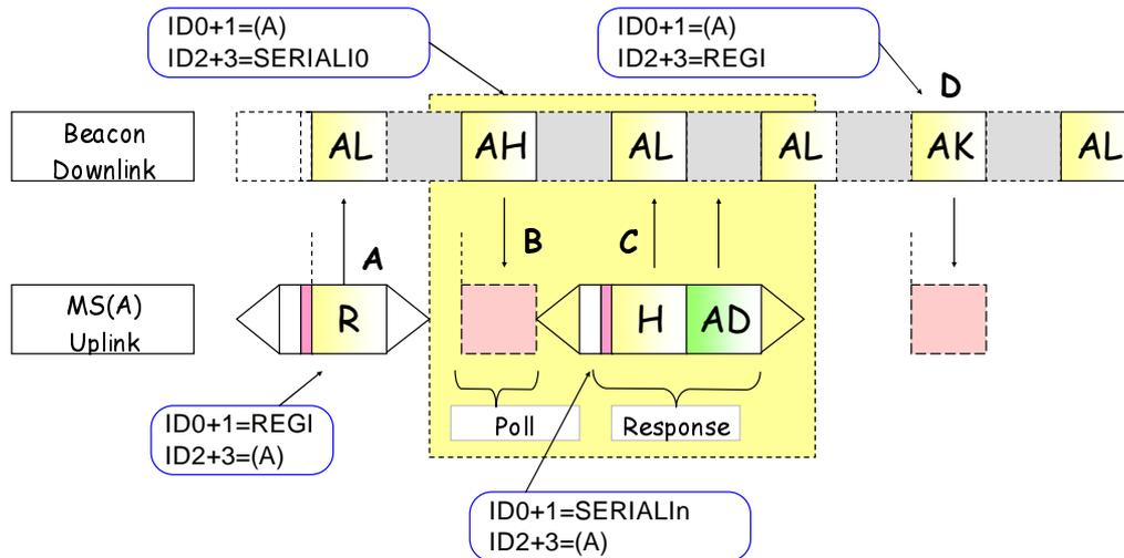
**Figure 12.32: Registration with serial check**
