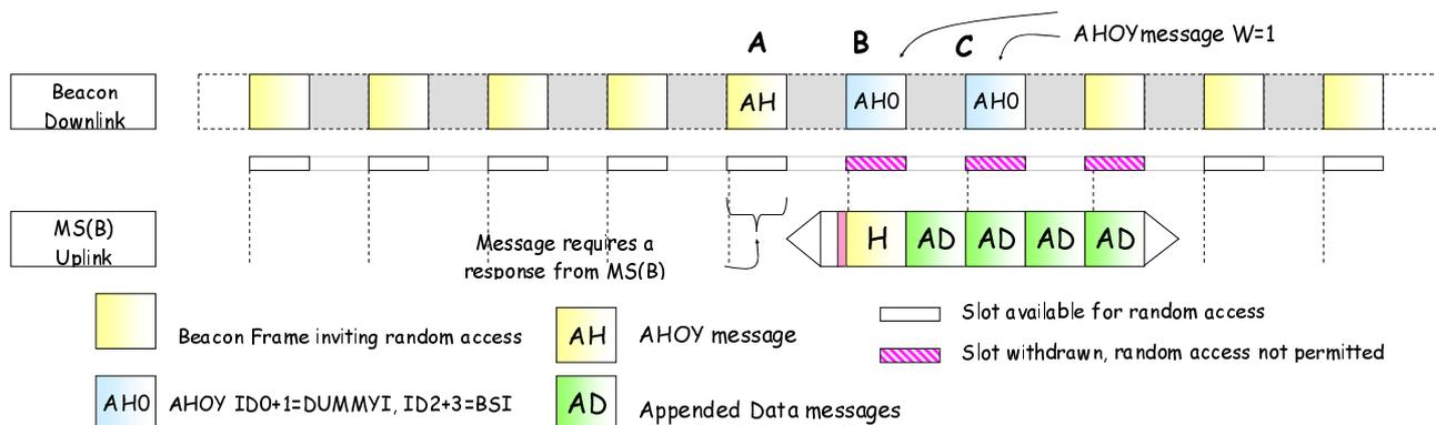
Figure 12.16: Withdrawn Framesets Example #3
