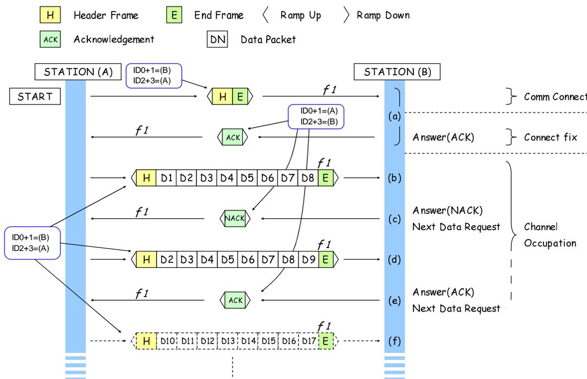
Figure 9.4: Packet retractions
