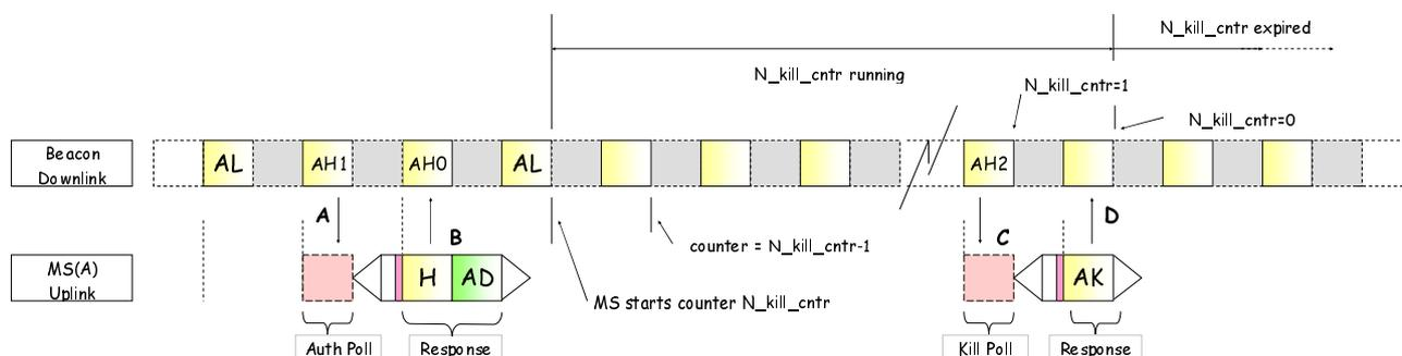
**Figure 10.45: Example of successful kill procedure**
