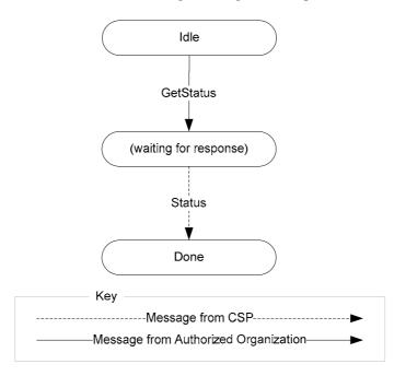
Figure 6: State diagram for GetStatus
