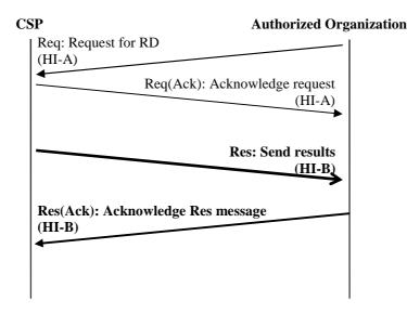
Figure 7: Message flow Successful delivery
