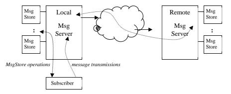
Figure C.1: Schematic overview of message handling
