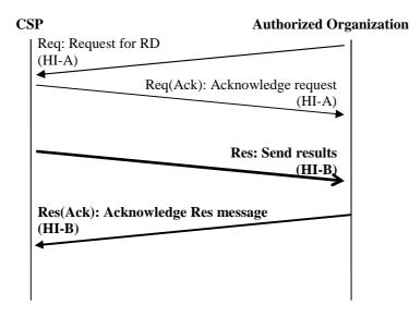
Figure 7: Message flow Successful delivery
