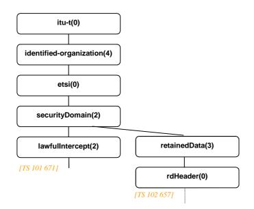
Figure A.1: Object identifier tree
