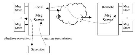
Figure C.1: Schematic overview of message handling
