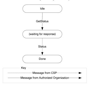
Figure 6: State diagram for GetStatus
