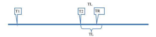
Figure J.2: TR occurs earlier than T2+TL, so a multi-part delivery should be applied
