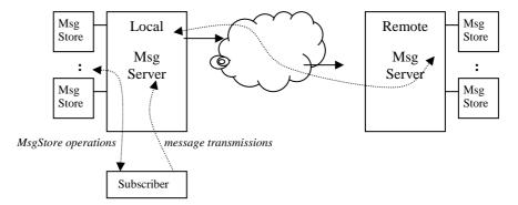
Figure C.1: Schematic overview of message handling
