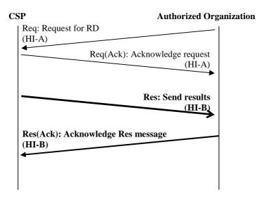
Figure 7: Message flow Successful delivery
