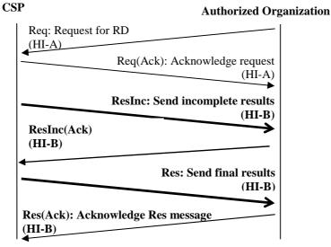
Figure 9: Message flow multi-part delivery
