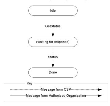
Figure 6: State diagram for GetStatus
