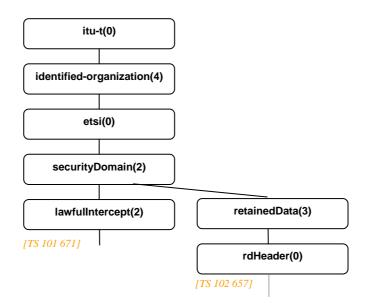
Figure A.1: Object identifier tree
