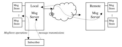
Figure C.1: Schematic overview of message handling
