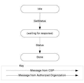
Figure 6: State diagram for GetStatus
