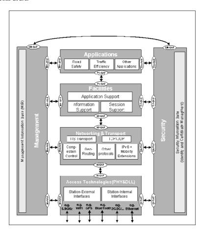
Figure 1: ITS Station Reference Architecture
