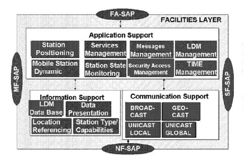
Figure 2: Facilities Layer Architecture
