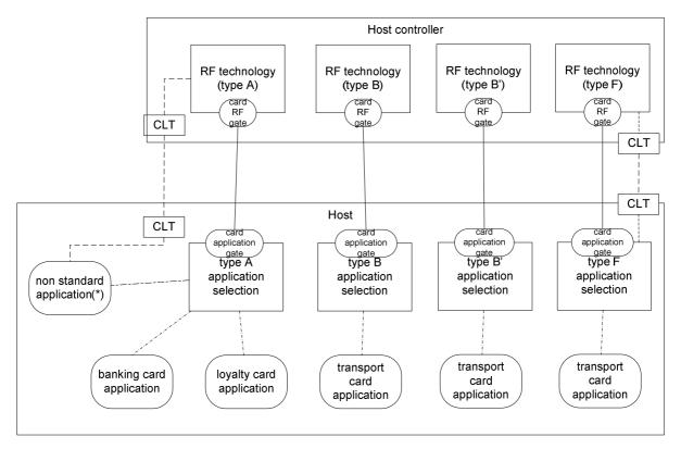
NOTE: Non-standard applications refer to type A contactless card applications that that do not use the transmission protocol defined in ISO/IEC 14443-4 [7].
